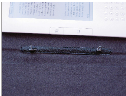
Figure 6. The way the Kindle 2 attaches to the covers is more secure than it was with the original Kindle.
