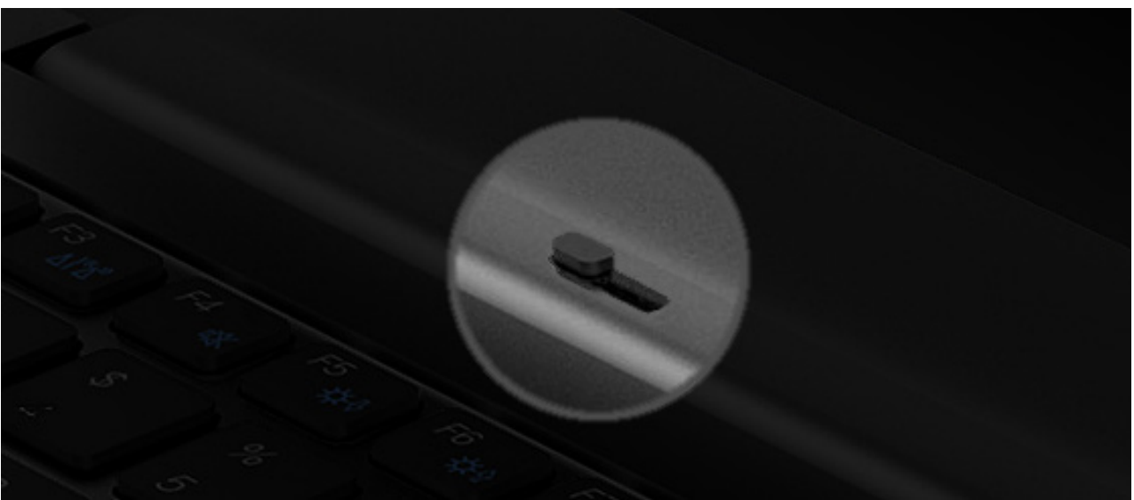
Figure 6. It's not possible to accidentally turn these switches on or off, which is awesome (photo from Purism ).
