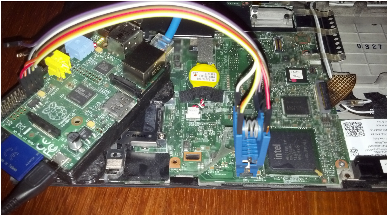
Figure 2. Hardware Flashing a BIOS with a Raspberry Pi
