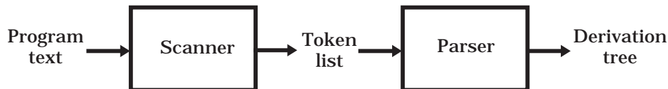
Figure 1.15: The Scanner and Parser
