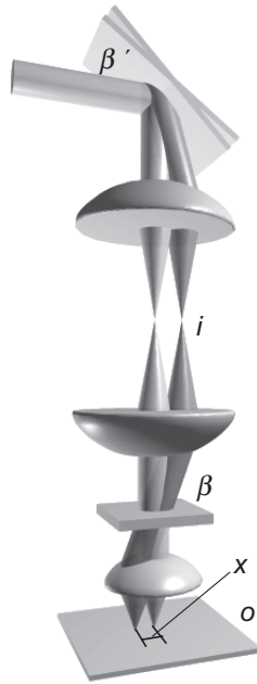
Figure 21.5: Location of the scan unit in a laser scanning microscope. In a confocal beam scanning microscope, mirrors located in planes conjugate to the telecentric system are tilted and thus deviate the beam by an angle \beta' that is proportional to \beta . This causes a light spot to move in the image plane i .
