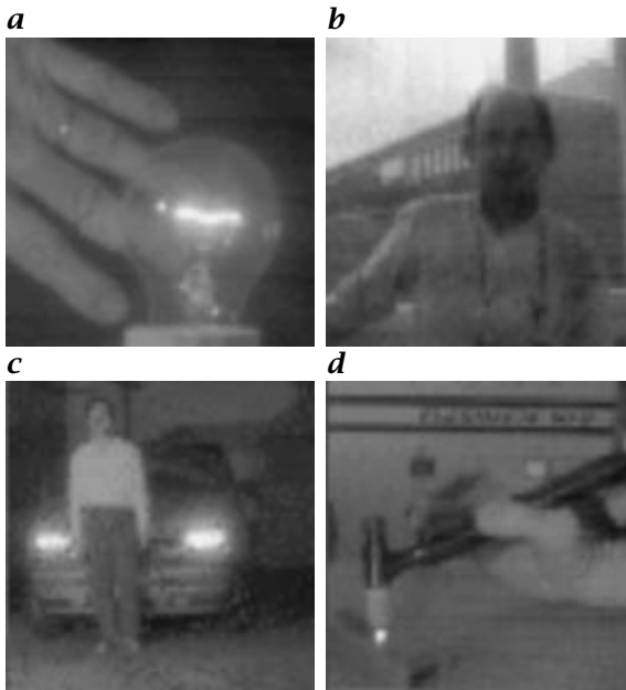
Figure 7.12: Four examples of pictures taken with a small-area logarithmic image sensor with 64 \times 64 pixels, illustrating the large dynamic range of \geq 120 dB: a electric light bulb where the glowing filament and the background are visible simultaneously; b back-illuminated scene of a portrait in front of a window; c parking garage application with its notoriously high dynamic range (headlights compared to dark corners) and low average light levels; d welding application in which the object and the welding arc can be observed at the same time without blooming.
