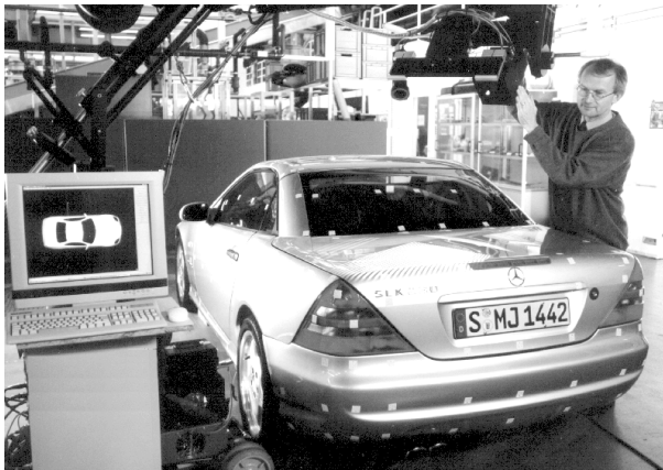
Figure 20.26: “Free-flying” sensor Ganymed in use.
