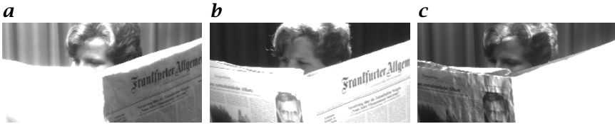
Figure 8.2: CCD image of a left side; b top; c right side; illuminated newspaper reader, showing saturation effects typical for linear responding cameras.
