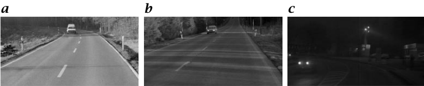
Figure 8.5: HDRC2 Traffic scenes a in bright sunlight; b at dawn; c by night.
