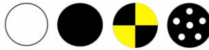
Figure 15.2: Typical markers: White or black circles for fast detection; more complex shaped markers for offline analysis.
