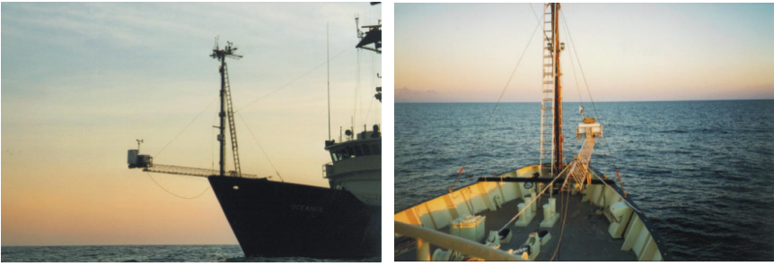
Figure 35.6: The CFT instrument is mounted on a 7-m long boom at the bow of the Research Vessel Oceanus during the cruise in the North Atlantic, July 1997; (see also Plate 11).
