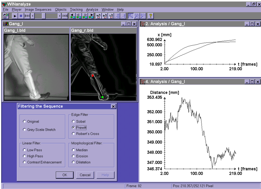
Figure 15.8: WINAnalyze—realization under Windows 95/NT. A stereo image sequence for gait analysis is shown, partially filtered with a high-pass filter. Two points were tracked on the leg. The chart on the upper right shows the horizontal trajectory of both points. In the lower right, the distance of both points along time is shown.
