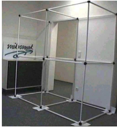
Figure 15.7: Example of a noncoplanar calibration model; calibration points are the spheres on the stick crosses. This model spans a room of 2 \times 2 \times 1 \text{ m}^3 , which are the minimum requirements for human gait analysis.
