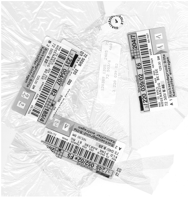
Figure 14.10: Example of package labels, which are processed in any given orientation at a conveyor belt speed of 0.5 m/s.
