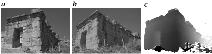
Figure 20.13: a Image 3 and b image 6 of the Roman bath sequence; c estimated depth map for image 6 (near = dark, far = light).
