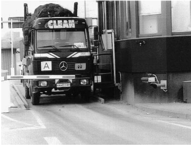
Figure 14.7: The OCR system VICODE identifies the license plate of the garbage truck at the entrance. Simultaneously the truck is weighed and the driver has to identify himself. The camera system can be seen on the right-hand side of the image.
