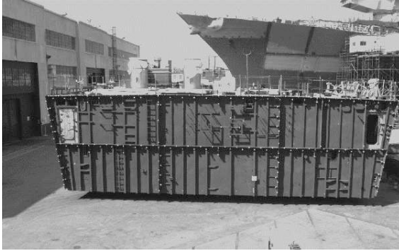
Figure 16.2: Typical unit with targets applied to section. All five faces of this unit are measured in one operation. The background shows the units on the assembled ship (Photography courtesy of Bath Iron Works).
