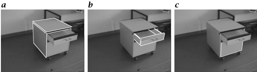
Figure 23.10: Recognition of an articulated object: Guided by the hierarchical structure of the object model the unknown joint configuration of the drawer cabinet is determined recursively.
