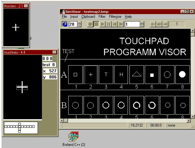
Figure 26.7: Screenshot of the PC running the VISOR program. The displays show computer-generated patterns. The left-bottom window indicates the area displayed by the piezoelectric actuators (dotted rectangle) as well as their actual pattern (square dots).
