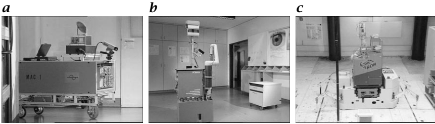
Figure 23.11: Different AMS used for the experiments. Note that in the AMS shown in the camera is mounted at the robot hand.
