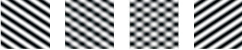
Figure 10.3: Four texture patterns. Left and right: pure 1-D signals, embedded into 2-D; middle: weighted superpositions to true 2-D signals.
