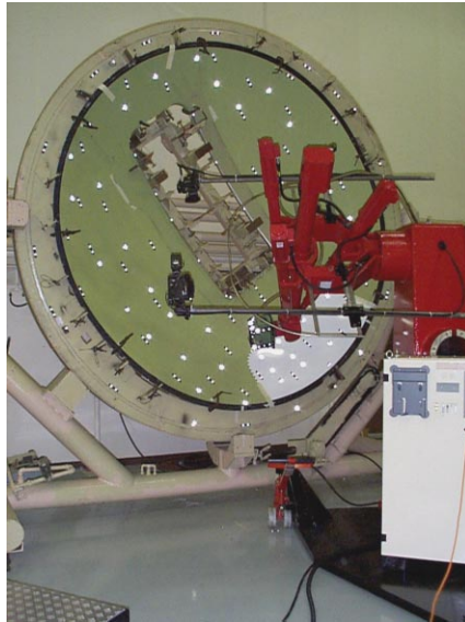
Figure 16.4: Bulkhead of an airplane with TI^2 system (Image courtesy of Boeing).
