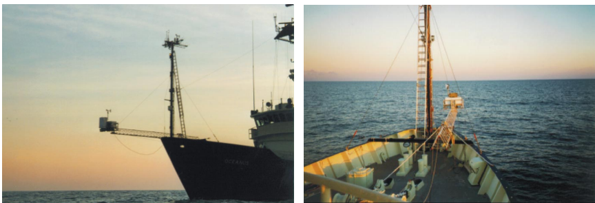
Plate 11: The CFT instrument is mounted on a 7-m long boom at the bow of the Research Vessel Oceanus during the cruise in the North Atlantic, July 1997; (see also Fig. 35.6, p. 757)
