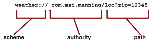
Figure 4.2 The portions of a Uri that are used in Android, showing scheme, authority, and path
