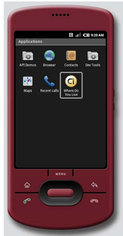
Figure 1.6 Applications are listed in the launcher based on their IntentFilter . In this example, the application Where Do You Live is available in the LAUNCHER category.
