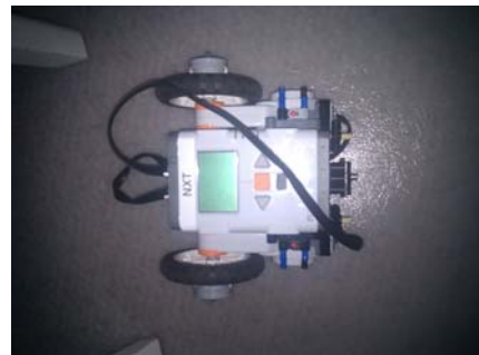
Figure 14.5 Simple LEGO NXT robot with motors connected to B and C ports
