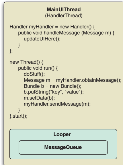
Figure 3.5 Using the Handler class with separate threads, and the relationship among HandlerThread , Looper , and MessageQueue
