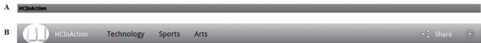
Figure 21.10 (A) Pre-Android 3.0 title bar with no action bar. (B) Android 3.0 title bar with fully customized action bar including tab-based navigation and action items, with the look and feel driven by simple styling.
