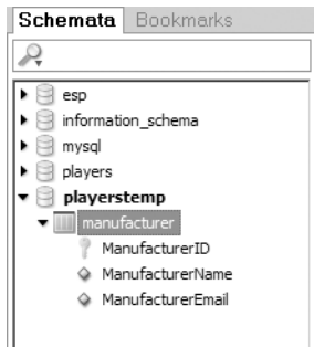
Figure 11-11. In MySQL Query Browser, you can verify that a table has been created correctly.
