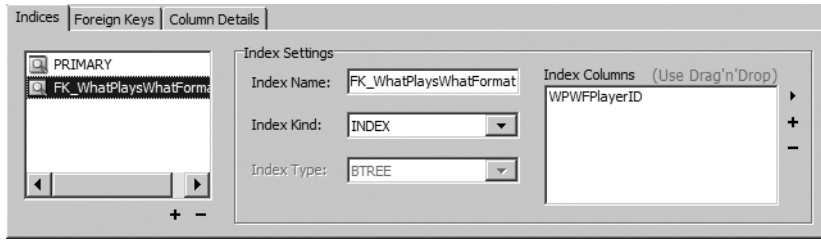
Figure 2-38. Composite primary keys require a separate index when they are in a relationship.
