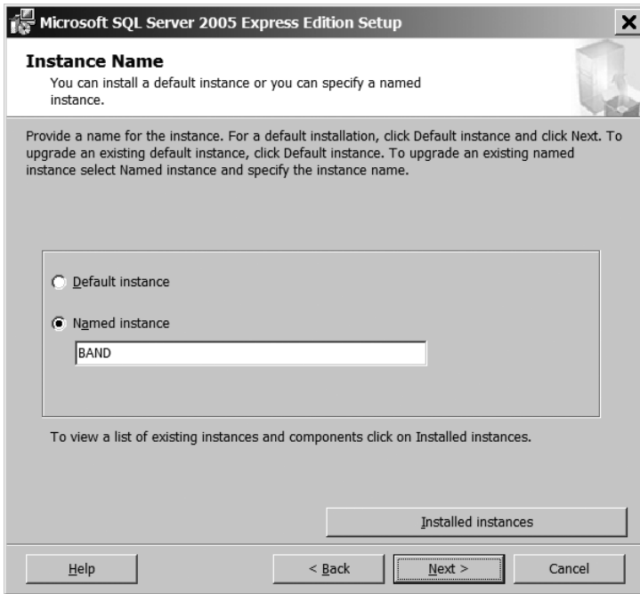
Figure A-1. Specifying the name of the SQL Server instance to create
