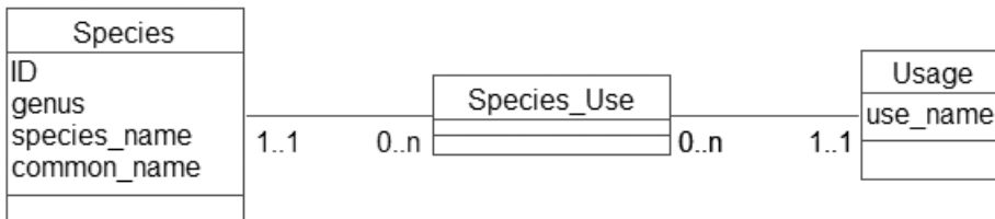
Figure 7-18. Adding another class to deal with a Many–Many relationship in a relational database
