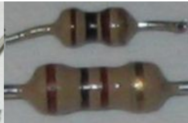
The 1/10th watt resistors used in this circuit, compared with 0.25watt resistors.
