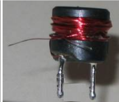
The transformer consists of 50 turns 0.25mm wire connected to the pins. The feedback winding is 20 turns 0.095mm wire with "fly-leads."
