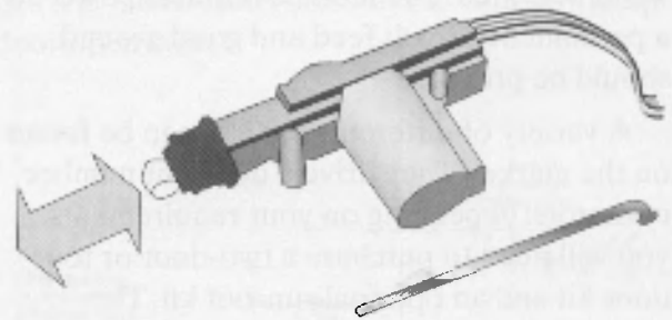
Figure 4-5 Central-locking motor and actuator rod
