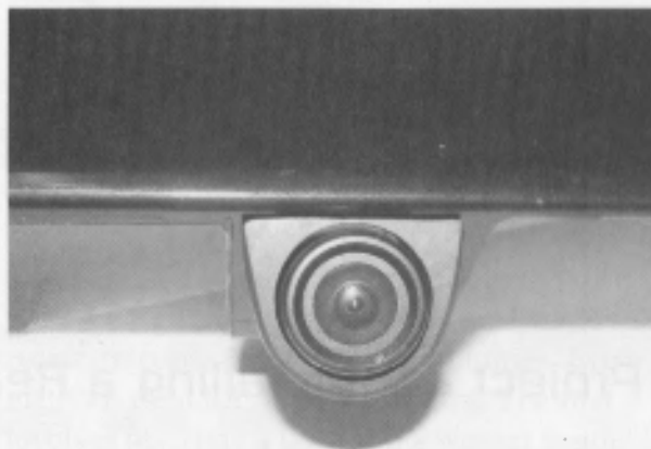
Figure 4-18 Under-bumper camera mounting (Courtesy Rostra Precision Controls)
