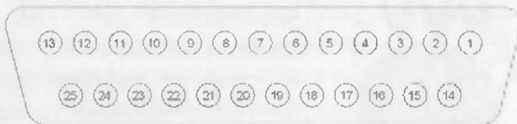
Figure 7-5 DB25 External parallel port connector
