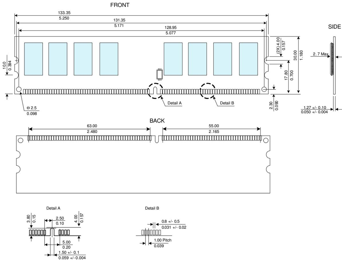
Note: All dimensions are typical with tolerances of +/- 0.15 (0.006) unless otherwise stated
