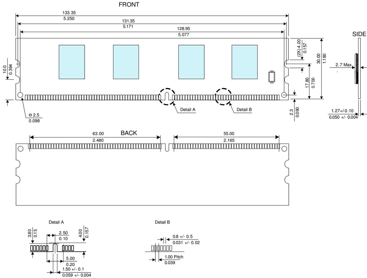
Note: All dimensions are typical with tolerances of +/- 0.15 (0.006) unless otherwise stated
