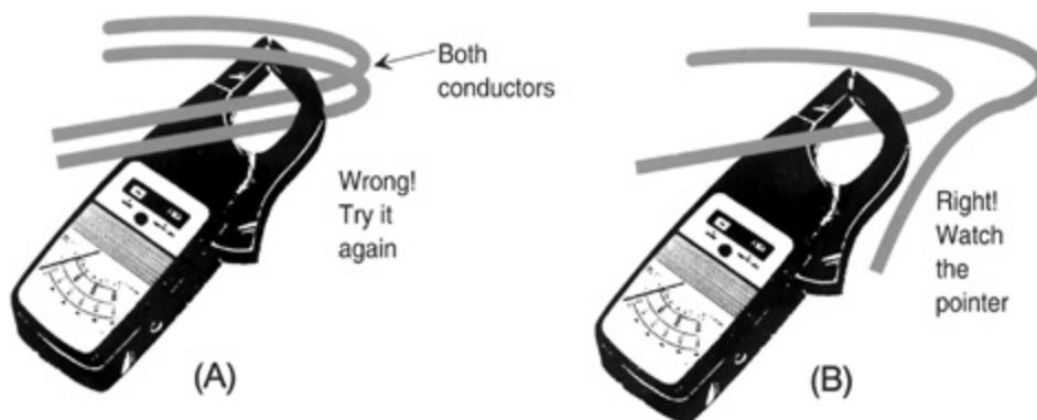
Figure 9.18 Right and wrong way to take current reading with a clamp-on ammeter.
