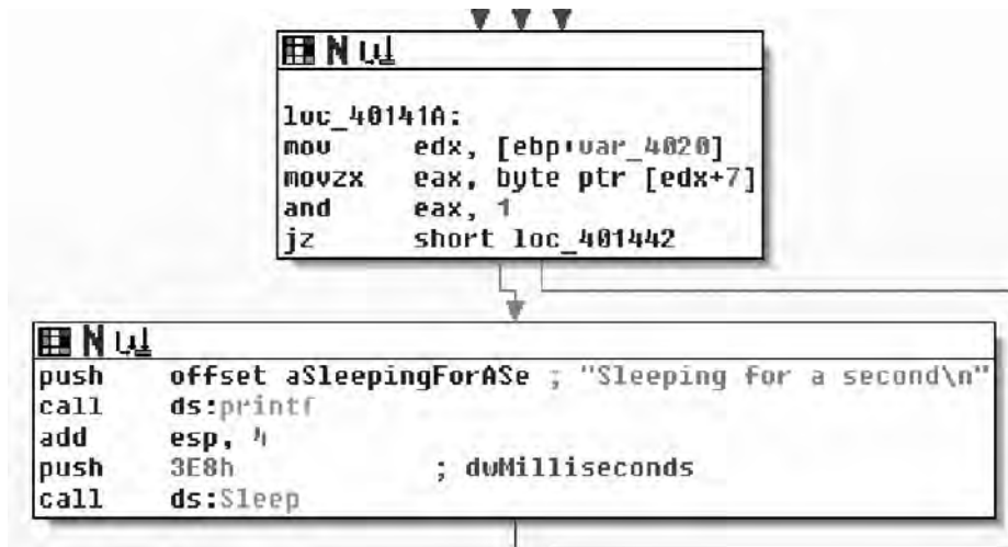
Figure 7.10 If Bit Is Set, Thread Goes to Sleep for 1000 ms
