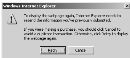
Figure 3-1: Browsers do not automatically reissue POST requests made by users, because these might result in an action being performed more than once
