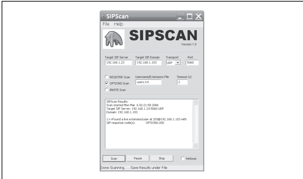
Figure 3-7 Using SIPSCAN against our Cisco IP Phone 7912 to find its extension
