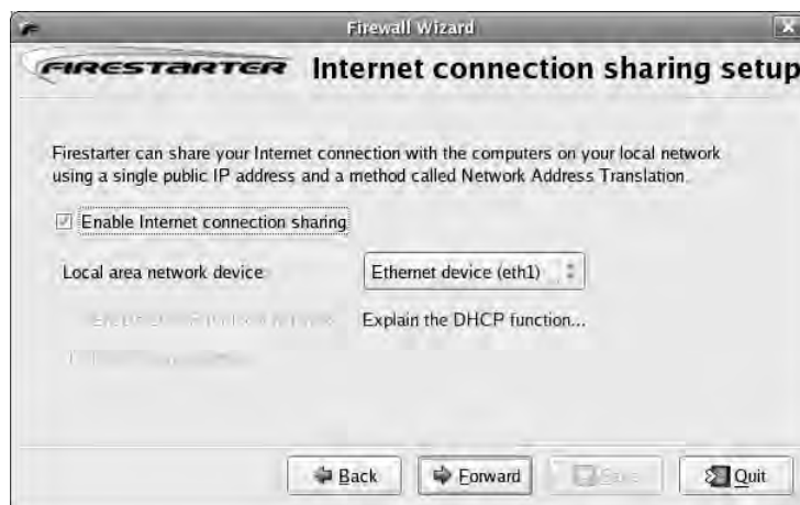
Figure 2.15 Firestarter Internet Connection Sharing Setup
