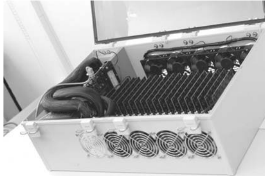
Figure 4.11: The Copacobana DES cracking machine (from www.copacobana.org , Gallery, with the courtesy of the authors).
