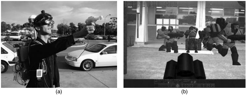
Figure 3.24 ARQuake, with user wearing head-mounted display and holding a gun (a) and game scene depiction (b). Reproduced by permission of Wayne Piekarski.
