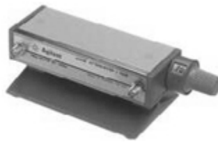
FIGURE 5.23 A sample of a RF step attenuator (variable loss)
