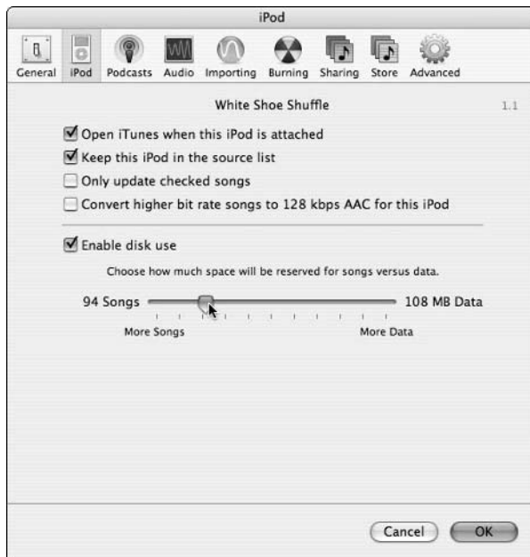
Figure 23-5: Enable the iPod shuffle as a flash memory drive that looks like a hard drive.
