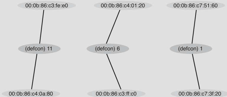
Figure 6-29 This figure shows the access points and the channel and SSID they are using.
