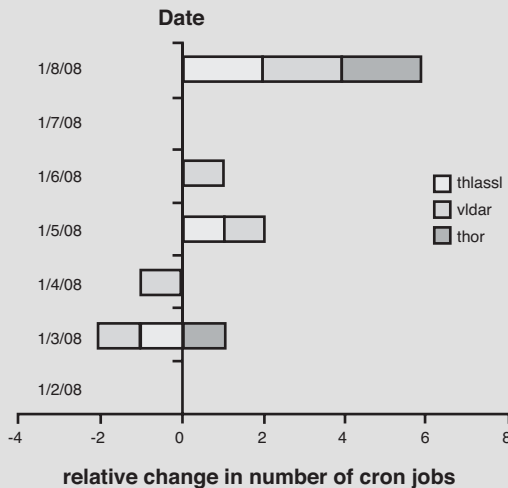
Figure 8-7 For each day, this chart shows the number of added or deleted cron jobs per machine.
