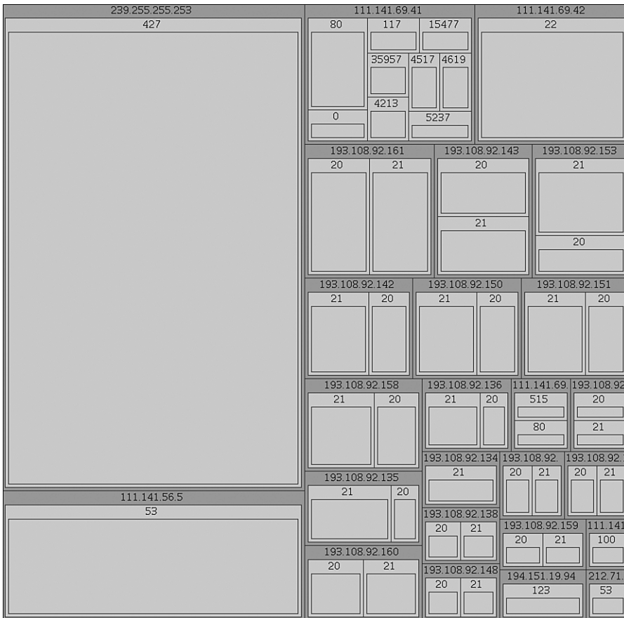
Figure 5-25 Treemap showing machines and their services. This time the dominant machine is filtered to show all other machines.
