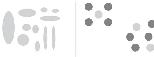
Figure 1-4 The leftmost example shows a graph that uses two integral attributes, width and height, to encode information. The graph on the right uses separable attributes, color and position, to do the same.
