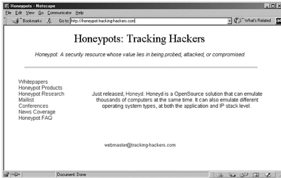
Figure 7-7. The emulated Web server service customized with the Tracking Hackers Web site to create a more realistic honeypot
