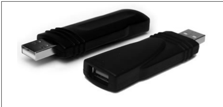
Figure 12.2 KeyGhost with USB Connectors
