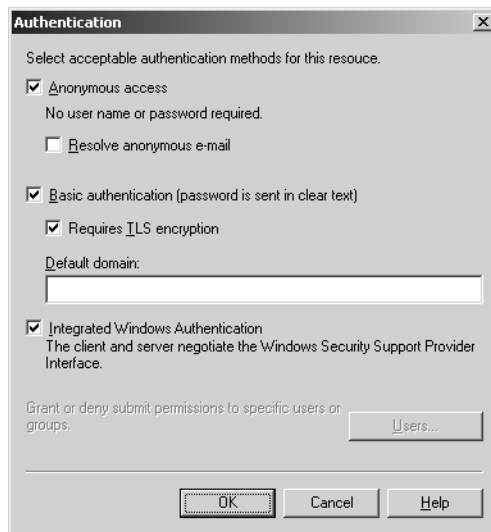
Figure 4.9 Exchange TLS encryption
