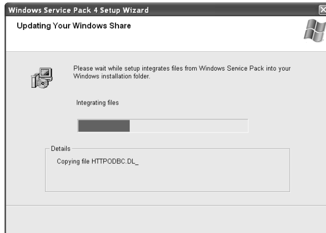
Figure 6.6 Slipstreaming a service pack
