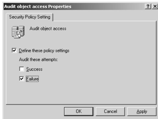
Figure 2.10 Auditing must be enabled for the system before it can be enabled for individual resources
