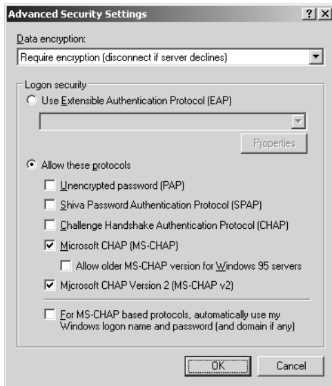
Figure 12.11 Advanced client authentication settings
