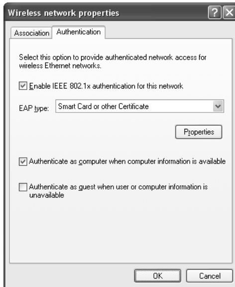
Figure 10.7 Windows XP wireless network authentication configuration
