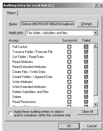
Figure 2.11 Failure auditing causes events to be added to the event log when a user is denied access to a resource
