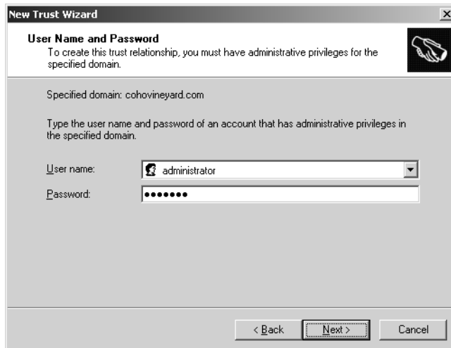
Figure 1.12 The User Name And Password page of the New Trust Wizard
