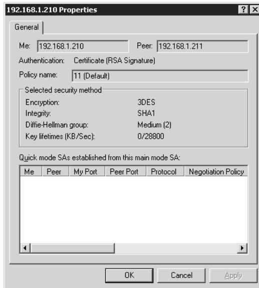
Figure 9.3 Security association authenticated with certificates
