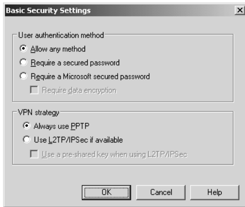
Figure 12.13 Editing basic VPN security settings by using the CMAK wizard
