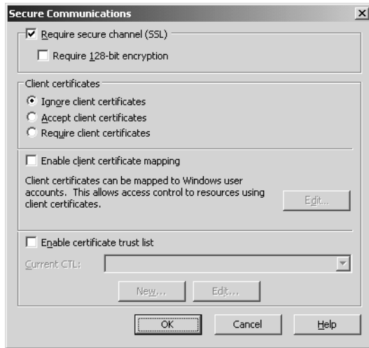
Figure 11.3 Requiring HTTPS for a Web server
