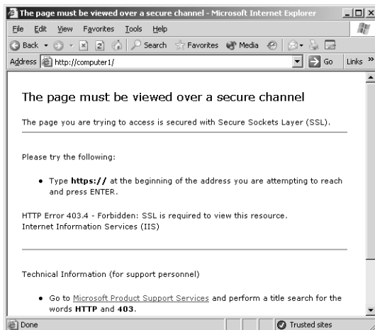
Figure 11.9 IIS configured to require SSL
