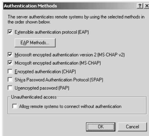
Figure 12.5 Default server authentication methods
