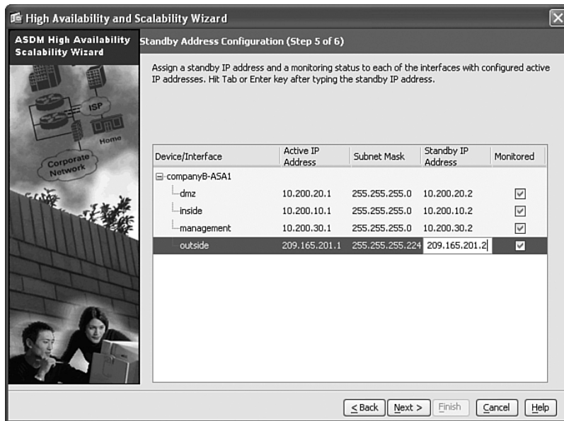
Figure 12-57 Configuring the Standby IP Addresses
