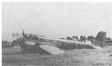
36. A wrecked Ju88G-1, W. Nr 414811, left to the mercy of souvenir hunters, who invariably 'liberated' the fin swastikas. Note the pre-service delivery radio code letters, PW + BC. (Via EJC)
