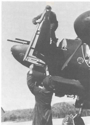
1. Overall black was the finish adopted for night fighters during the early days of the force and the majority of aircraft also sported the 'Englandblitz' badge on both sides of the nose. This Bf110C is having the nose fairing over the four 7.9mm machine guns replaced by the armourers. One of the blast tubes inside the fairing can be seen and the white individual aircraft letter 'F' can just be made out on the extreme tip of the nose.
