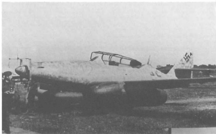
41. 'Red 12' of NJG 11, an Me262B-1a/U1 W. Nr 111980 with black underside paintwork and mottled blue-grey camouflage on top, seen on a Berlin airfield after the war. (Via EJC)
