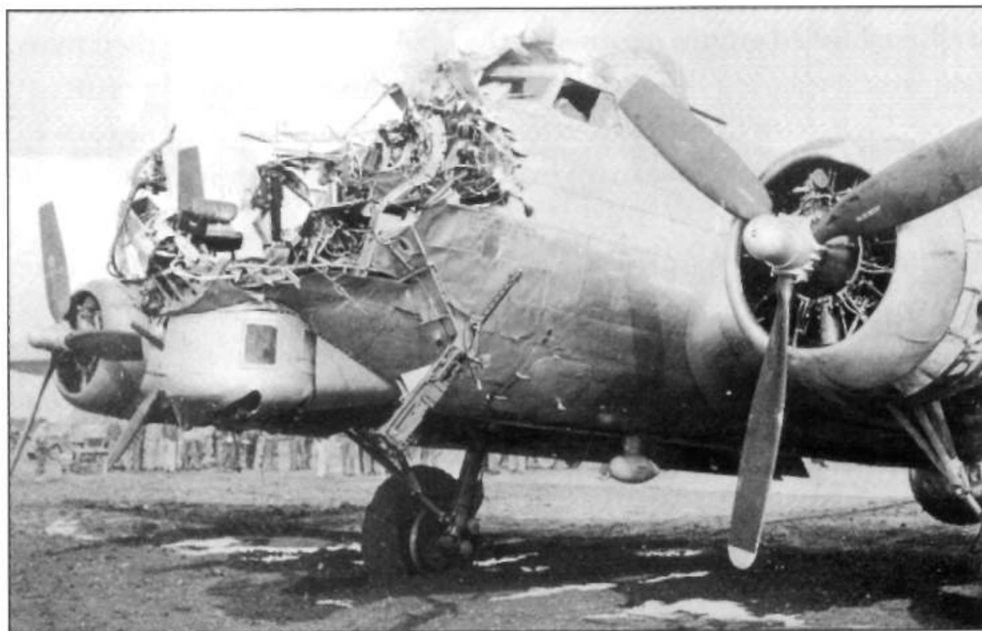
B-17G-80-BO 43-38172 of the 601st BS/398th BG, piloted by 1Lt Lawrence De Lancey, made it back to Nuthampstead from Cologne on 15 October 1944 after losing its nose, and the bombardier, to a direct flak hit over Cologne (USAF)
