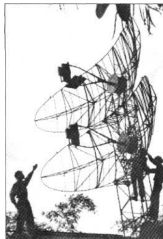
The 'Song Ma' Regiment's P-15 'Flat Face' early-warning radar could detect targets up to 250 km away at a minimum altitude of 300 m. The P-15 was mounted on a ZIL-157K 6x6 truck, which gave it cross-country mobility. Forty 'Flat Faces' were put into operation in North Vietnam ( Tran Dinh Kiem )
