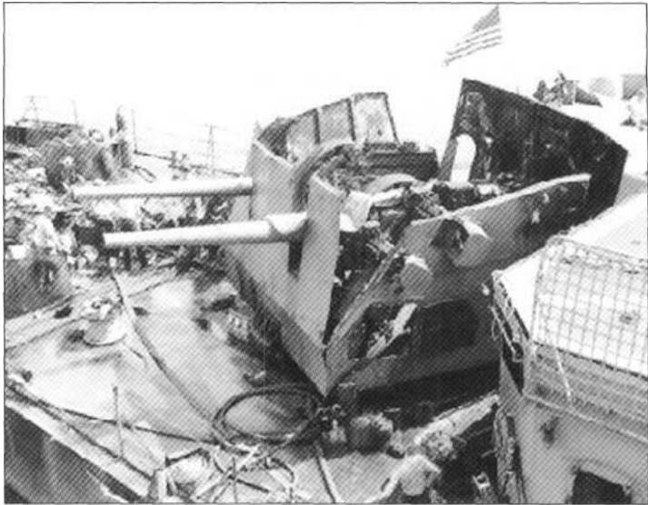
As this photograph graphically shows, the damage inflicted on the stern of the Higbee by Le Xuan Di's solitary 250-kg bomb was severe. It effectively wrecked the destroyer's aft 5-in turret, yet miraculously none of the vessel's crew were killed (via Istvan Toperczér)
