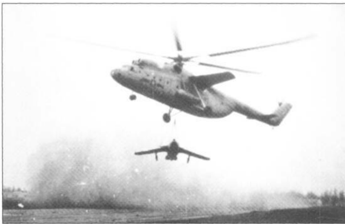
Mil's hugely impressive Mi-6 could easily lift fully-armed and refuelled MiG-17s, and transport them from their dispersals in the mountains to jet-capable airfields. After completing their missions, the fighters would soon be delivered back and hidden from enemy fighter-bombers. The VPAF's modest fleet of Mil-6s transported MiG-17s on approximately 400 occasions to remote mountain shelters up to 30 kms away from operational bases (VPAFMuseum)
