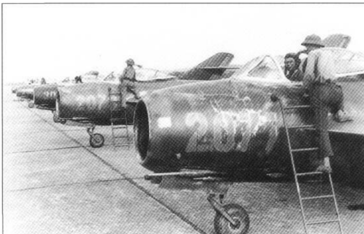
These dark green MiG-17F 'Fresco-Cs' of the 923rd Fighter Regiment are seen on the ramp at Kep. The pilots nicknamed these camouflaged aircraft 'Snakes' because of their colour scheme (VNA)
