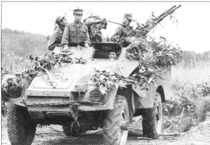
This VPAF-ADF GAZ BTR-40 scout vehicle has been fitted with a 20 mm AAA mounting. The design of the Russian-built BTR-40 was heavily influenced by the American M3A1, 3340 examples of which were supplied to the USSR during World War 2. The vehicle is seen moving to a new site near Noi Bai airfield in September 1967 (Gabor Palfai)
