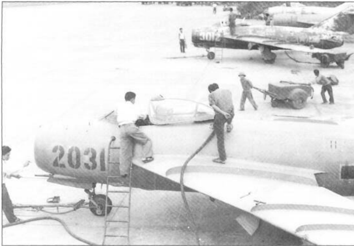
North Vietnamese groundcrews prepare a quartet of MiG-17s for their next mission at Noi Bai. Note the two technicians manhandling the engine starter cart across the apron to a waiting fighter out of a shot (I/AM)
