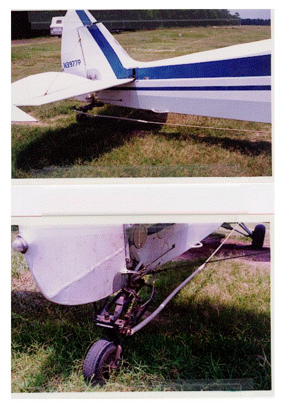
FIGURE 2-2. EXAMPLES OF A VEE BAR
