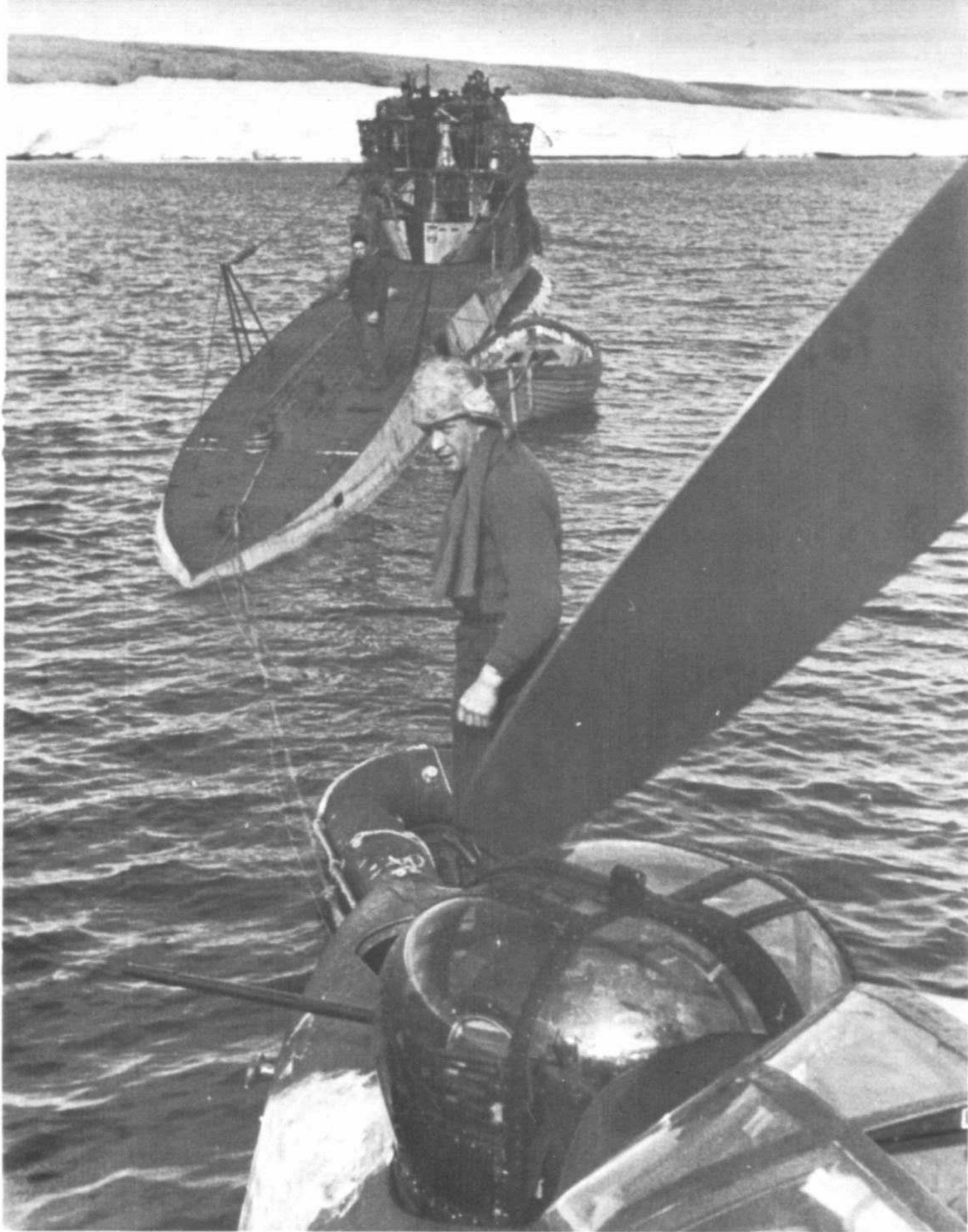
A shortage of fuel or damage to the aircraft caused this towing arrangement. The BV 138 B has a splotched on "iceberg" white camouflage paint over its green surface. The submarine doing the work is a Type VII late model boat mounting much anti aircraft defense.
