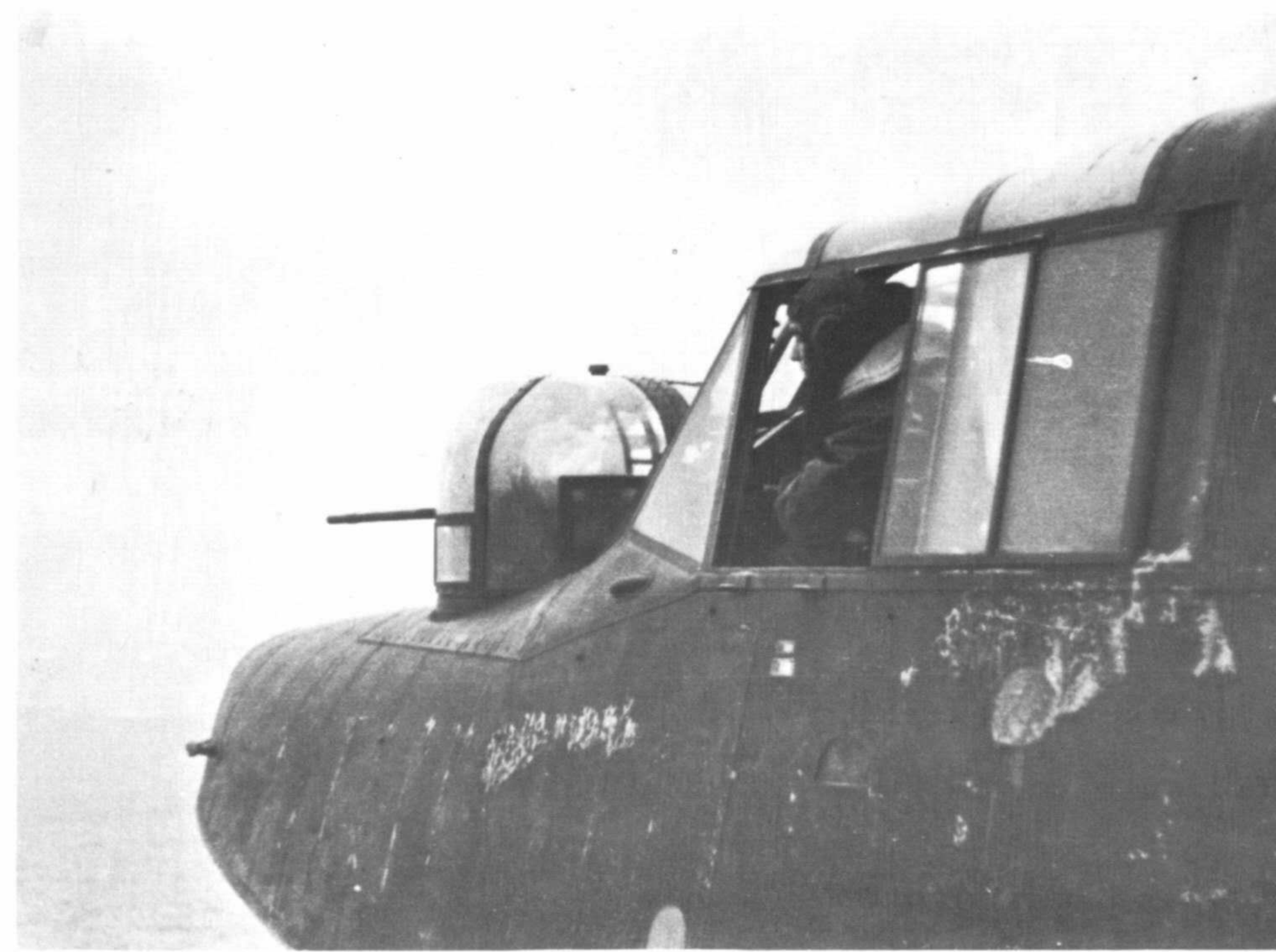
The "office" of a BV 138 as seen from outside. The sliding windows on the canopy were large enough for a man to get out of if necessary. Note the 20 mm MG 151 in its turret.
