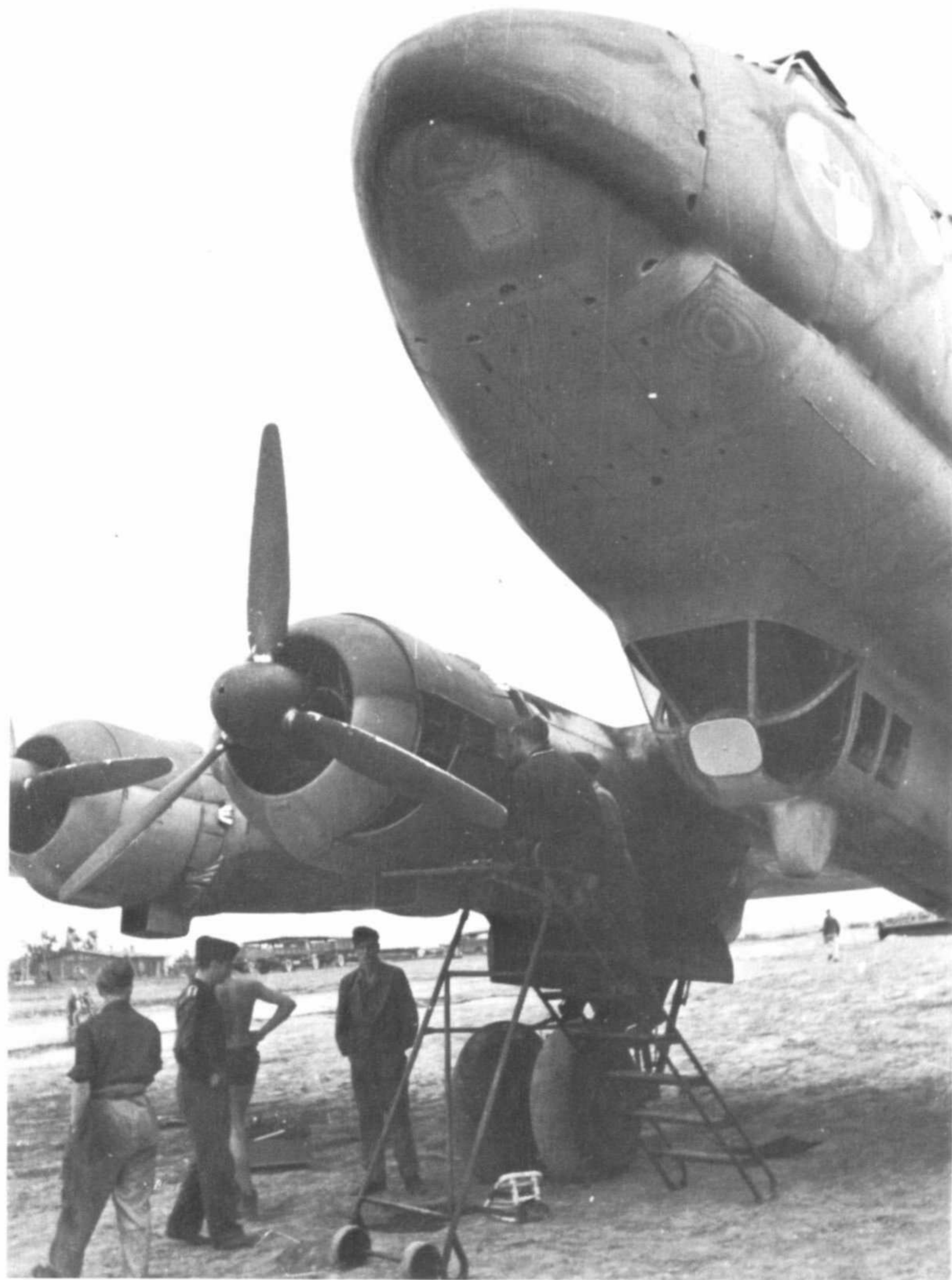
Another view of the FW 200 C-3 of Blindflugschule B-36. Mechanics are preparing to work on one of the four 1,000 hp BMW 323 engines. Note the all-around access panels on the cowl, giving the mechanics ample space to work.
