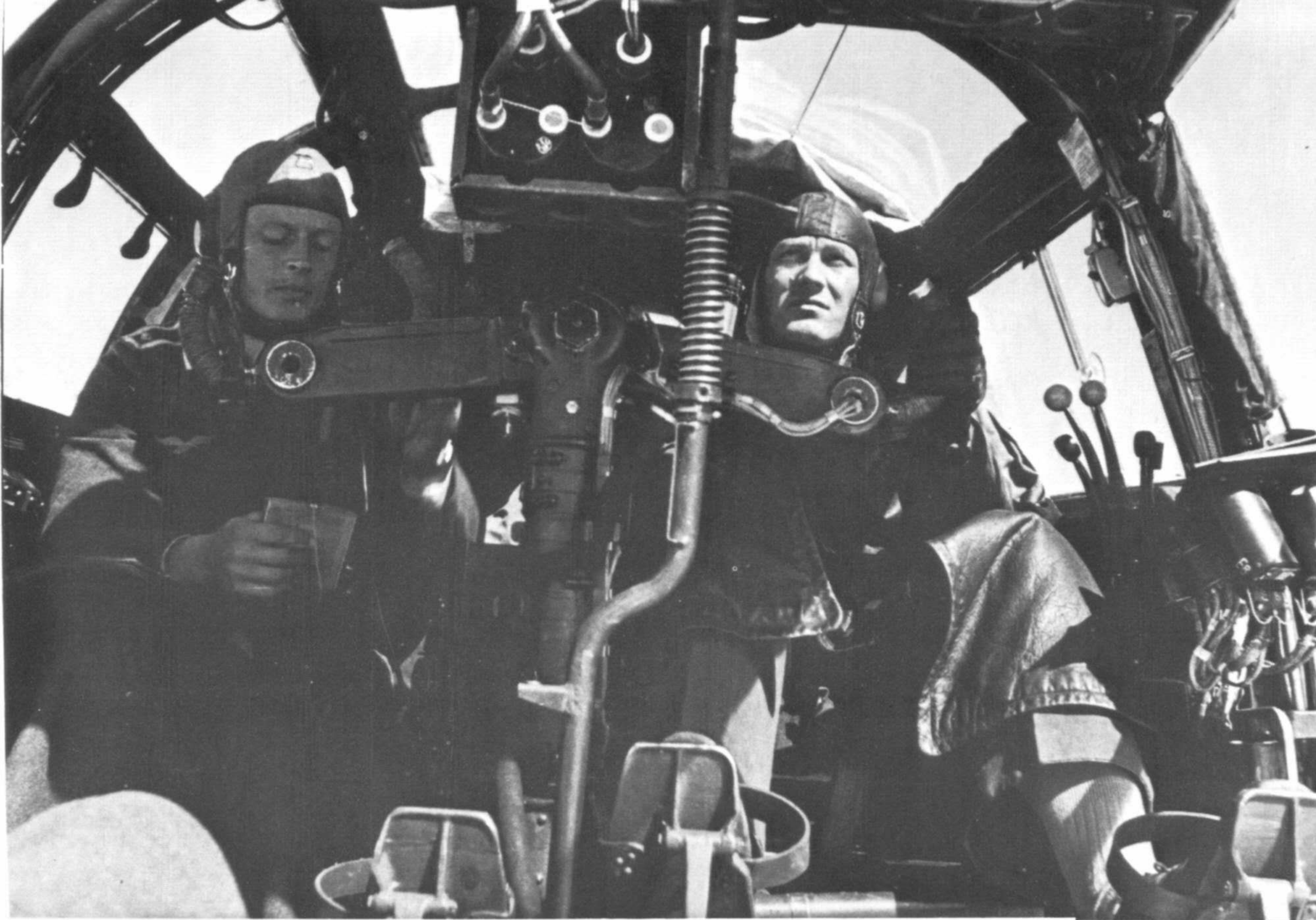
The pilot and co-pilot of a FW 200 during a flight over the Atlantic. Notice that both control yokes are hooked to a common member centrally located between the two crew members.
