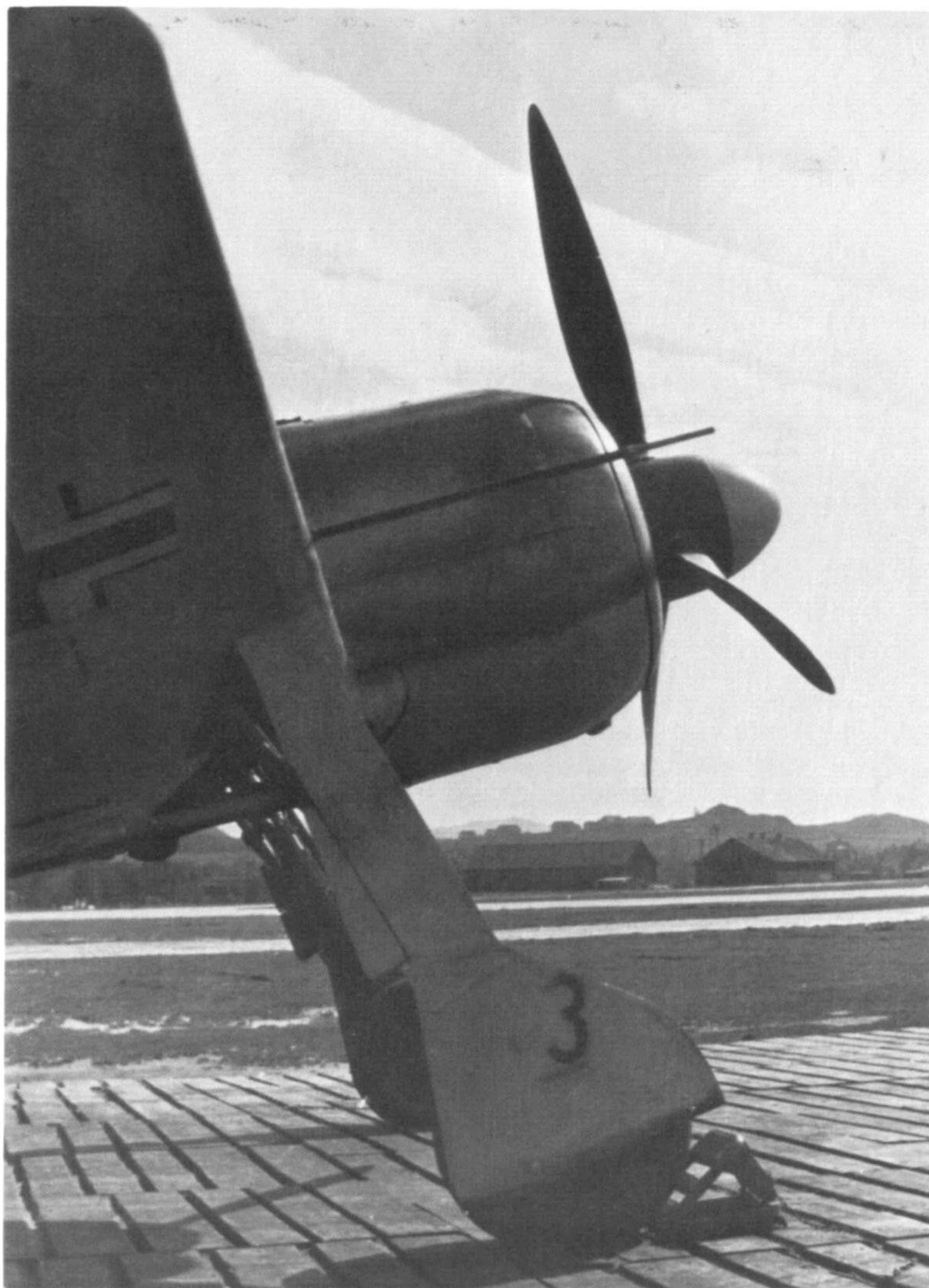
In this side view, one can see the protruding blast tube of the fuselage mounted 13 mm MG 131 that fired through the propeller arc, as well as the sturdy wide tracked landing gear.
