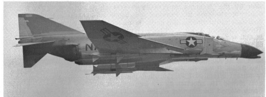
Early production model of the Phantom test firing a Sparrow AAM off Point Mugu, California. F-4Bs were the first models to assume the by now familiar 'droop snoot' appearance, occasioned by the installation of the 32" radar dish and the infra-red heat sensor. (U.S. Navy)
