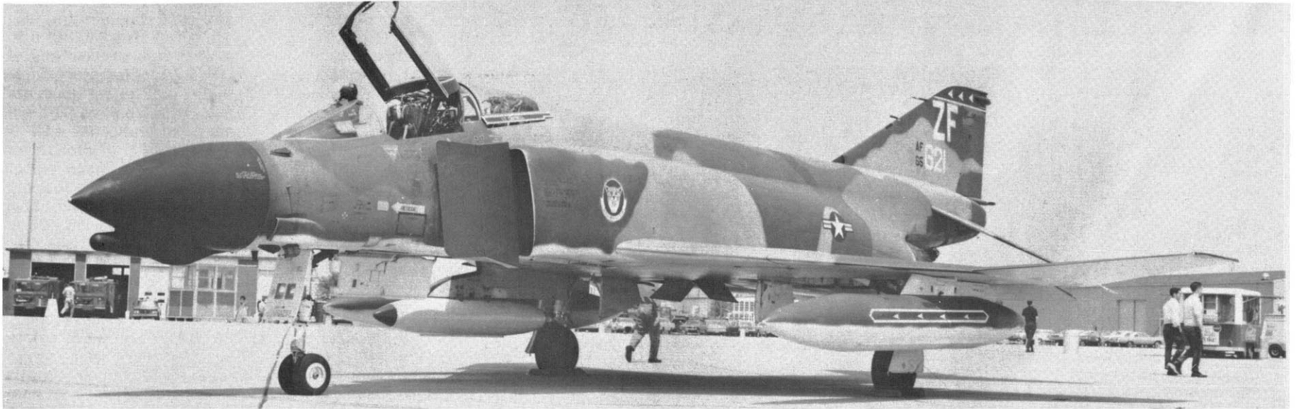
A Later model of the F-4D. Air Force Phantoms are equipped with an explosive cartridge starting system, enabling them to operate from airfields with less exotic maintenance equipment. Navy Phantoms, rarely called upon to operate from forward areas, do not employ this system. (Paul Stevens)
