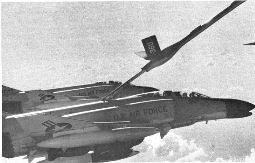
In-flight refueling. USAF strike aircraft would not have been able to carry out their devastating strikes on North Vietnam had it not been for the KC-135 tankers that serviced them inbound and outbound from their targets. (USAF)
