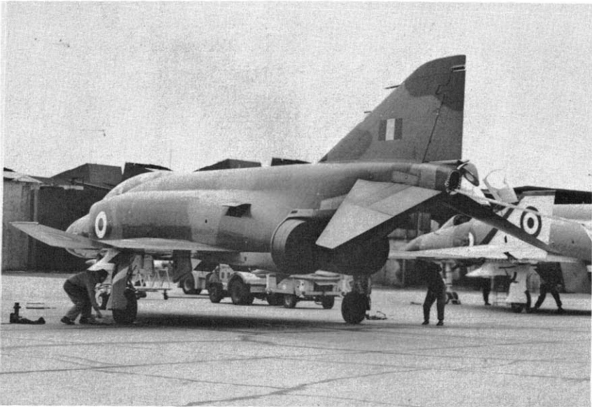
F-4M at the end of a test hop. British Phantoms use the Rolls Royce Spey engine, which results in slightly different lines at intake and exhaust. (McDonnell-Douglas)
