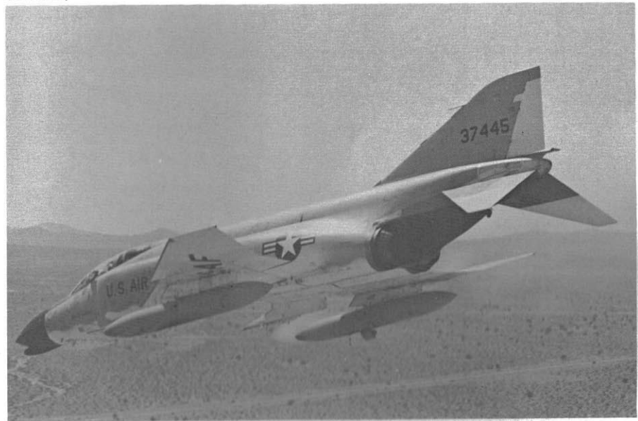
F-4C testing the 20mm Vulcan gunpods on outboard wing stations. (General Electric)
