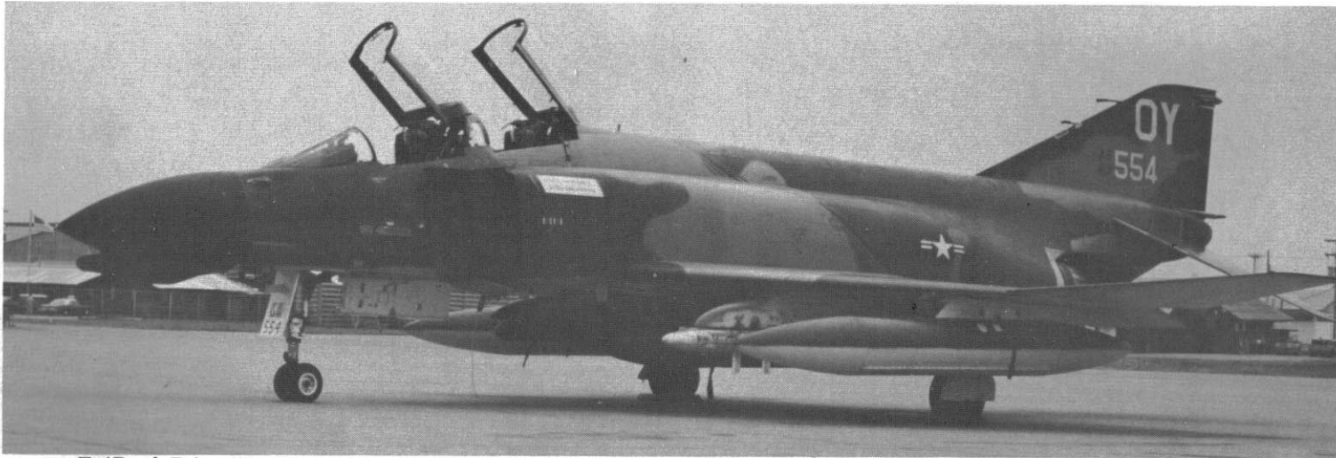
F-4D of Brigadier General Darrell S. Cramer, CO of the 432nd TRW . General Cramer was an ace in World War II, with 13 victories to his credit. Aircraft carries the tail code of the 555th TFS . MiG kill markings on the splitter vane belong to the aircraft, not to General Cramer. Fuselage bands are blue (front) and red. This aircraft carries an ECM pod on the inboard wing pylon. (Capt. Ward Boyce)
