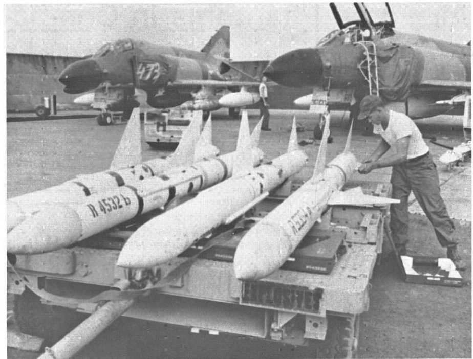
A USAF Weapons Specialist is readying Sparrow IIIB AAMs for loading onto F-4s. The Raytheon Sparrow is the primary armament of the F-4. The missile has a 60 lb HE warhead, and a range of 13 miles. It is radar guided. (USAF)
