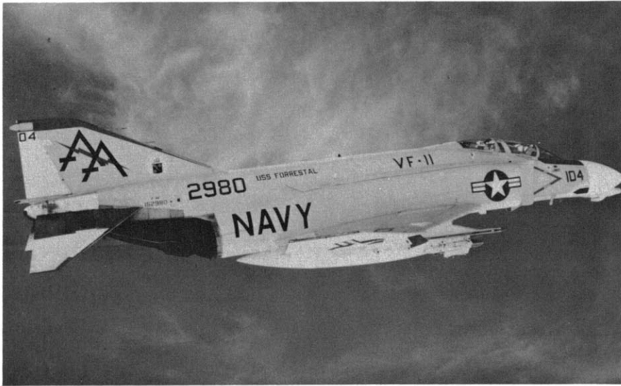
Red Rippers. VF-11 F-4Bs over the Med. 2980 rolls over his wingman (top) and joins up (bottom) for return to the USS Forrestal. Late model F-4Bs retain the infra-red sensor housing beneath the nose, though the sensor has been deleted in favor of avionics antenna. (US Navy)
