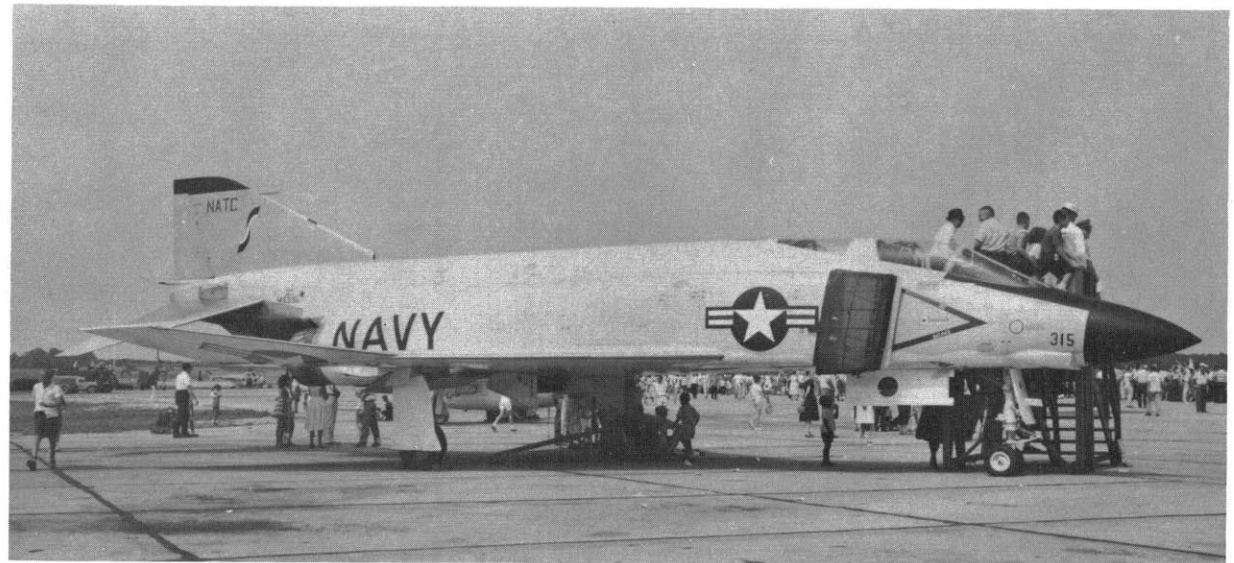
EARLY PHANTOMS—F-4A (top) has faired-in intakes used with lower powered J79-GE-3 engines. More powerful dash 8 engines required redesigned intakes. Both models have smaller nose used with 24" radar dish, and original canopy outline, later changed when seats were raised to provide better over the nose visibility for Pilot and Radar Intercept Officer. (via Paul Stevens)
