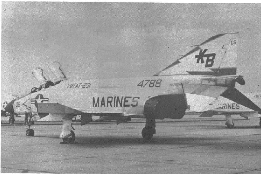
Two views of the late model F-4J for the Marine Corps. The 'J' has numerous improvements over the 'B', including AWG-10 pulse doppler radar fire control, improved AJB-7 bombing system, drooped flaps and slotted leading edges in the stabilator for better control at approach speeds, as well as a slightly larger fuel capacity. Note the position of the open drag chute door under the rudder. (USMC)
