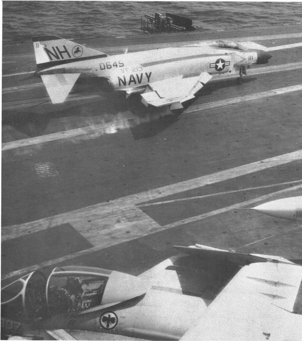
One of only 12 F-4Gs being hauled to a stop by Kitty Hawk's arresting gear. F-4G was actually the F-4B modified by the addition of Automatic Carrier Landing System. VF-213 operated the F-4G over Vietnam in late 1965.
