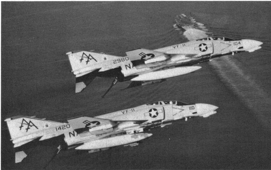
Red Rippers. VF-11 F-4Bs over the Med. 2980 rolls over his wingman (top) and joins up (bottom) for return to the USS Forrestal. Late model F-4Bs retain the infra-red sensor housing beneath the nose, though the sensor has been deleted in favor of avionics antenna. (US Navy)
