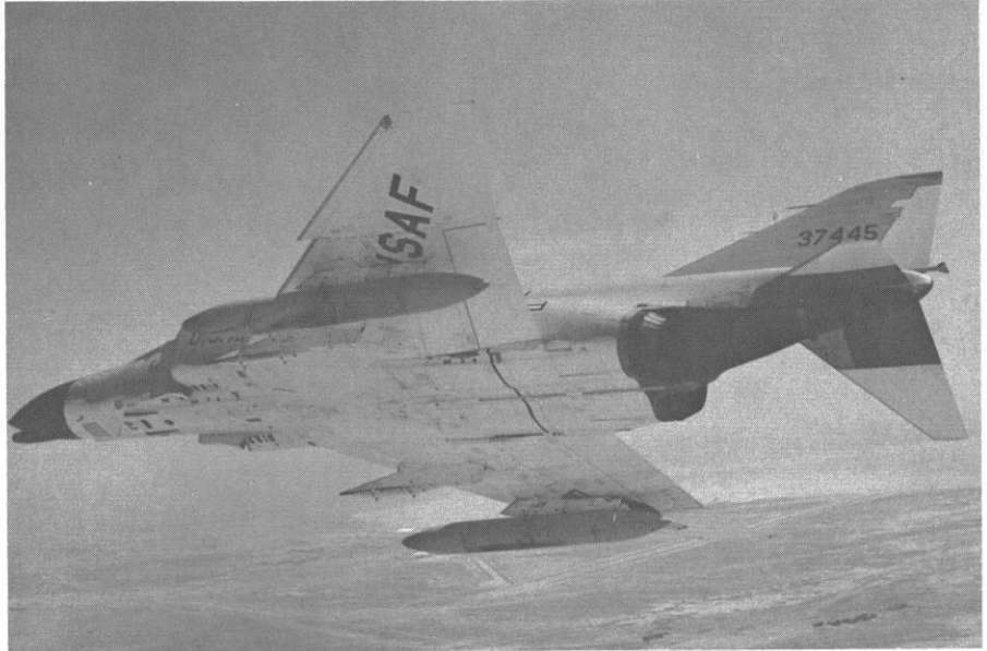
F-4C testing the 20mm Vulcan gunpods on outboard wing stations. (General Electric)
