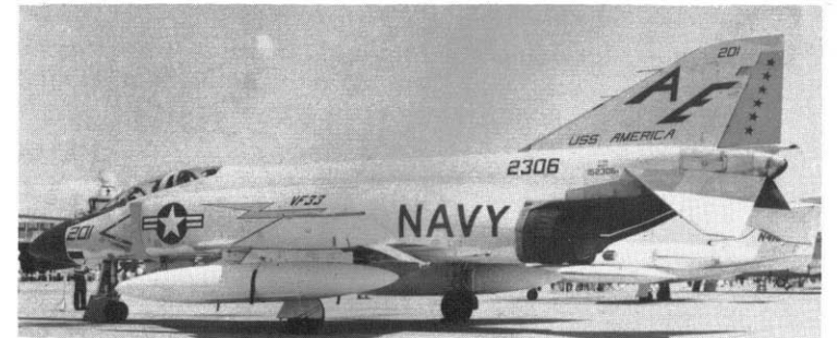
VF-33 Phantom, sans various antennae the F-4B later sprouted as Vietnam war experience was put to use in the development of ECM equipment. (Paul Stevens)
