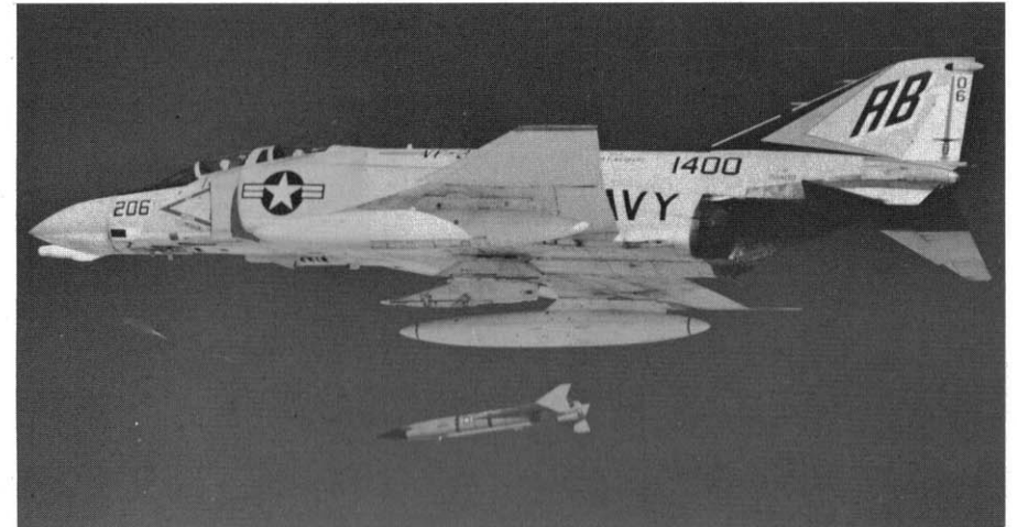
A Phantom from the USS John F Kennedy launching a target drone over the Mediterranean. Following F-4s will track the drone on target acquisition radar and try to shoot it down. (US Navy)
