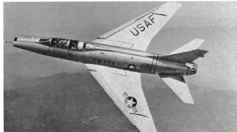
Overhead plan view of F-100F. The opened IFR hood is clearly visible in the rear cockpit. Also note position of split leading edge slats. (North American)
