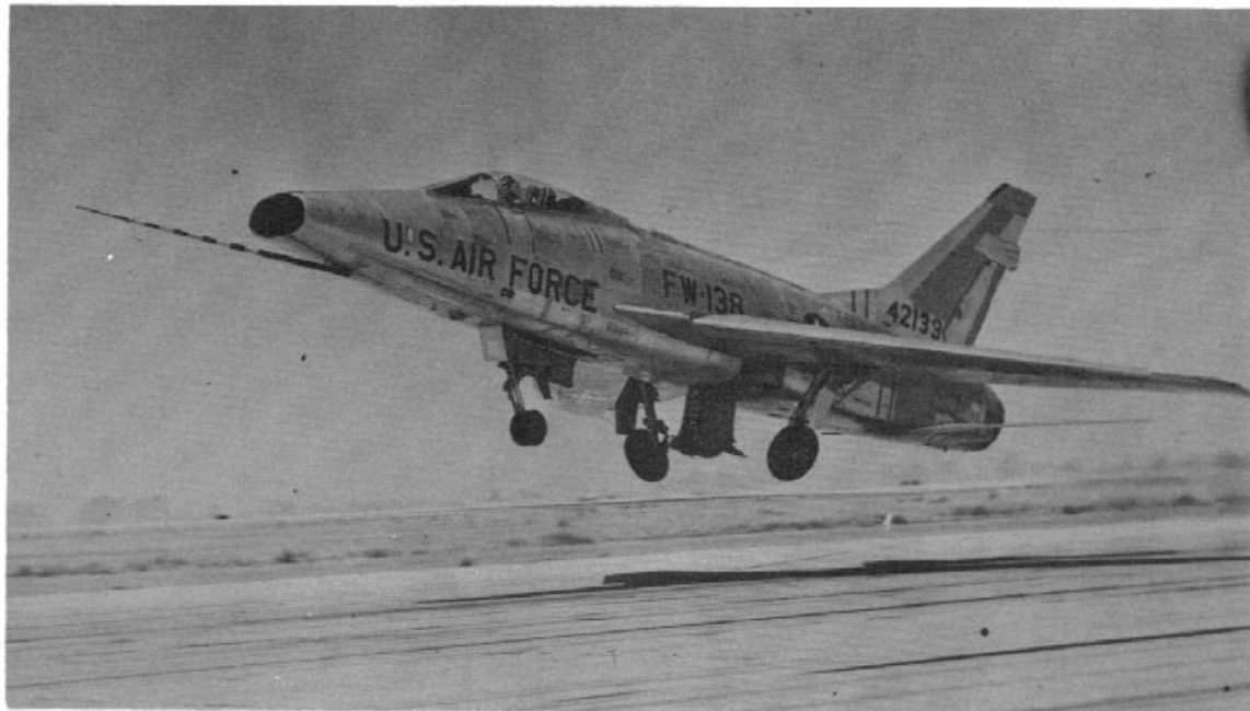
F-100 gear retraction sequence is illustrated as a pair of F-100's leave North American's Palmdale facility. Total time required for gear retraction is six to eight seconds. (North American)
