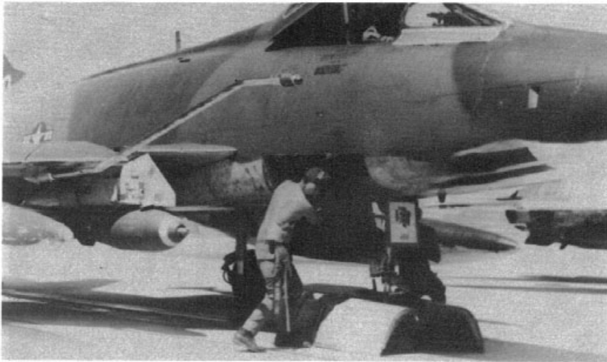
Hun pauses at arming pit, while munitions men manually charge the 20mm cannon, before taking off for a strike. When guns are fired, expended cartridge cases will be jettisoned through chutes in the underside of the fuselage, while belt links are retained internally. (USAF)
