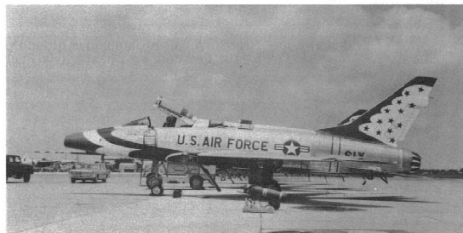
F-100D of Capt. Merrill A. McPeak. McPeak was flying this Super Sabre at air show in 1967, when both wings came off during vertical roll. Later investigation indicated fatigue cracks, which were prevalent among most operational 100's, had caused structure to fail. This precipitated grounding of Thunderbirds F-100's, and a 4G limit being placed on all other operational Super Sabres. Modification program which cost $620,000 eventually fixed problem and the F-100 continued to soldier on. (Paul Stevens)
