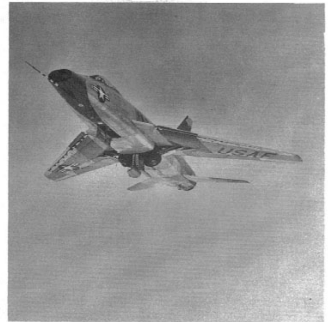
F-100 gear retraction sequence is illustrated as a pair of F-100's leave North American's Palmdale facility. Total time required for gear retraction is six to eight seconds. (North American)
