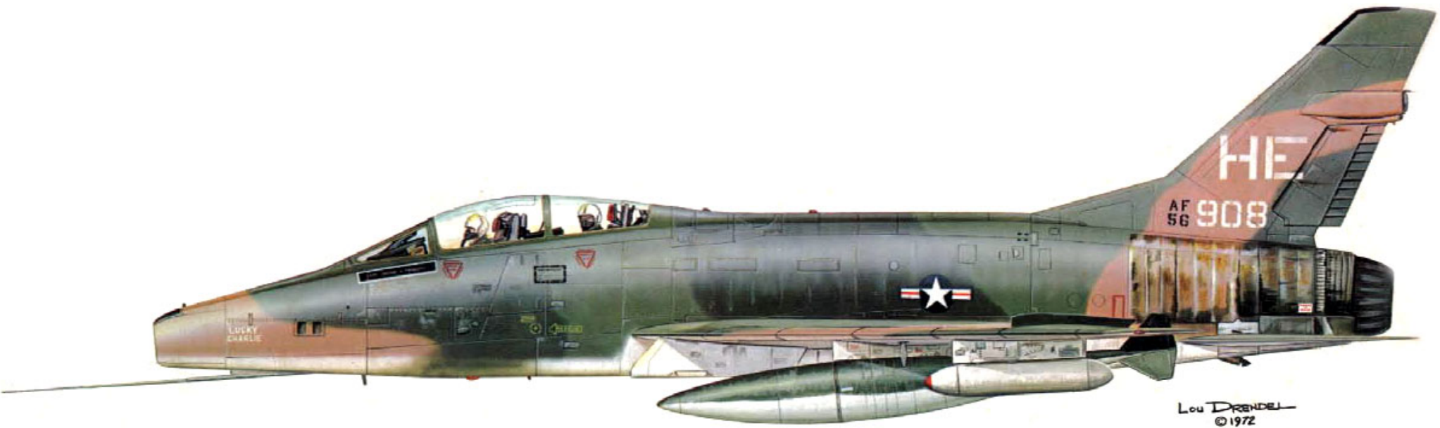
F-100F-10-NA assigned to "Misty FAC" program. Was flown by Capt. George A. Franzer. Standard loading for Misty FACs was LAU-59A rocket pods on outboard stations, 335 gallon drop tanks on intermediate stations. Some carried special fore/aft camera pods mounted inboard of inboard station.
