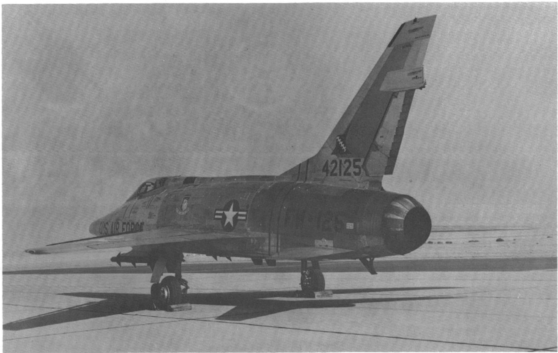
Fourth production example of the F-100D on the ramp at Edwards AFB in 1956. It is shown with four Sidewinder AAM's mounted on underwing pylons. The "D" variant was the first of the Super Sabres to be equipped with landing flaps, a much needed and appreciated improvement over the hot-landing "C". Early production versions also incorporated a lightweight doppler navigation system. (USAF)
