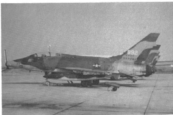
F-100F-11-NA of the Iowa Air National Guard at Des Moines in 1972. Note the variations in camouflage colors, and how the paint has been effectively removed from rear of fuselage by heat. (Douglas Slowiak)
