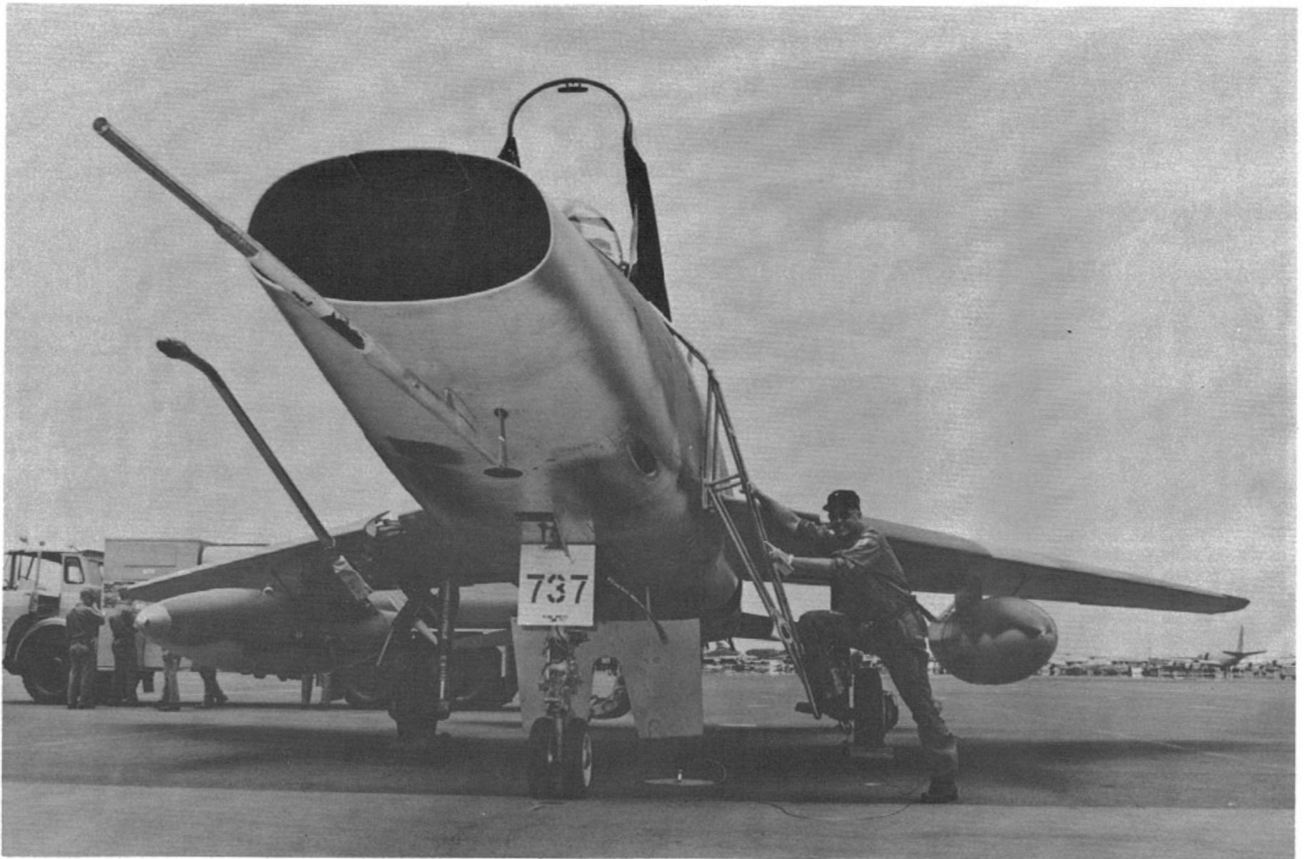
Hun driver about to check into his office. Super Sabre configured as this one would carry 12,000 lbs. of fuel. Note full open position of speed brake, which can be used at any speed. (Relief valve prevents structural damage if speed brake is employed at too high a mach number.) (USAF)
