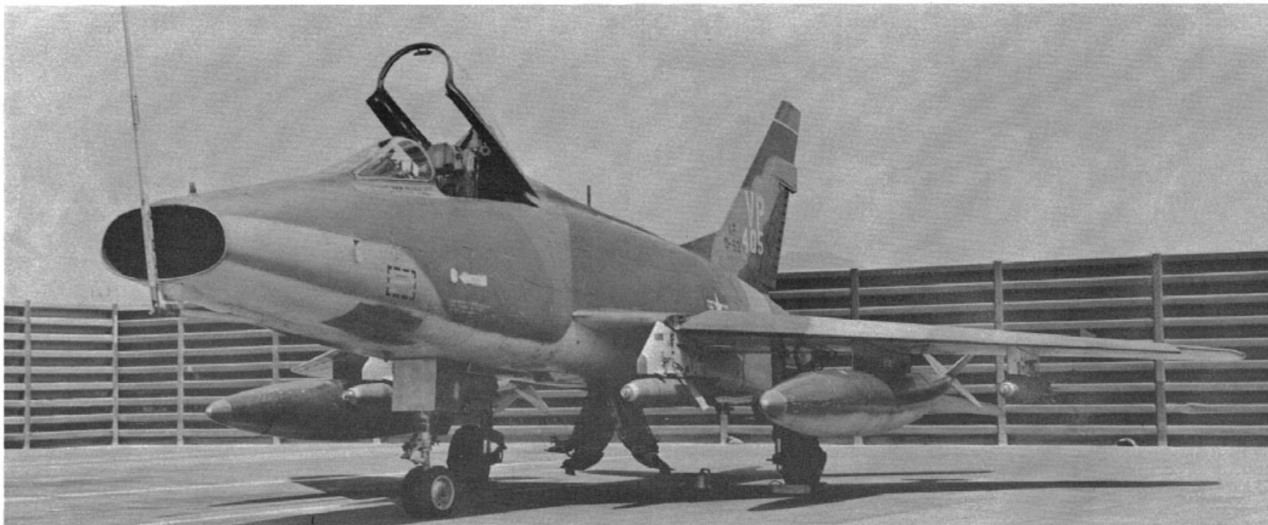
F-100D-86-NH of the 614th TFS , loaded with 500 lb. Snakeye bombs , in revetment at Phu Cat AB. Note detail of nose probe fold. (Norm Taylor)
