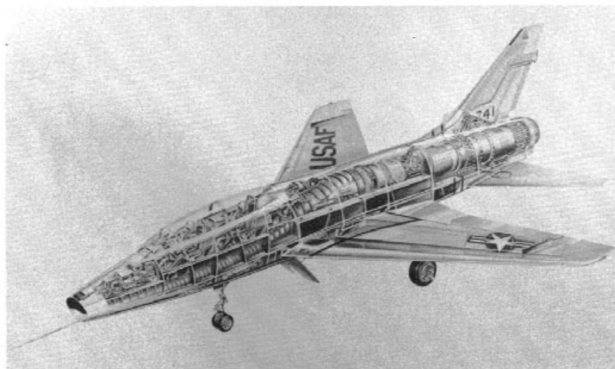
Cutaway view of F-100F, showing principle components. Note fuel cells immediately above and in the wing. (North American)
