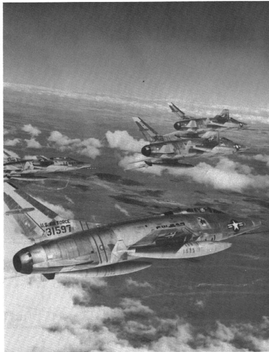
Formation of F-100A's of the 479th Fighter Day Wing , out of George AFB, California. These Super Sabres have been modified with larger vertical fin and wings. (North American)
