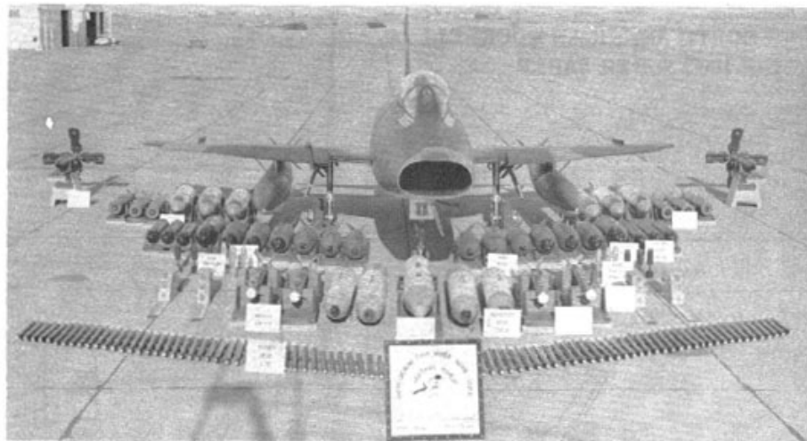
F-100 poses with the various types of ordnance it is capable of delivering. Worthy of note are the Snakeeye high drag bombs, (on either side of the wingtips) with fins extended. (USAF)
