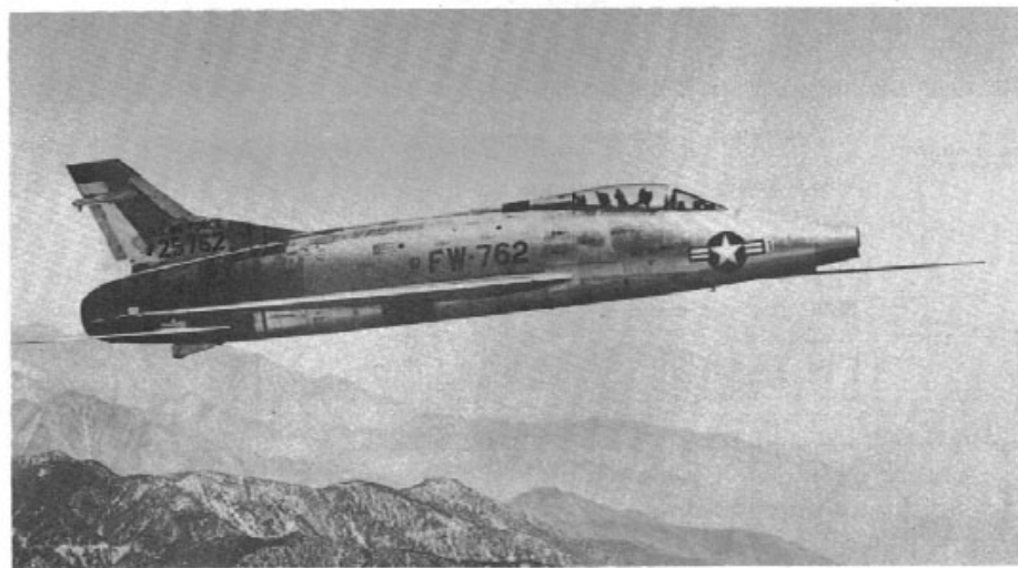
Initial production version of the F-100A , with short vertical fin, in flight over the mountains of Southern California. (USAF)
