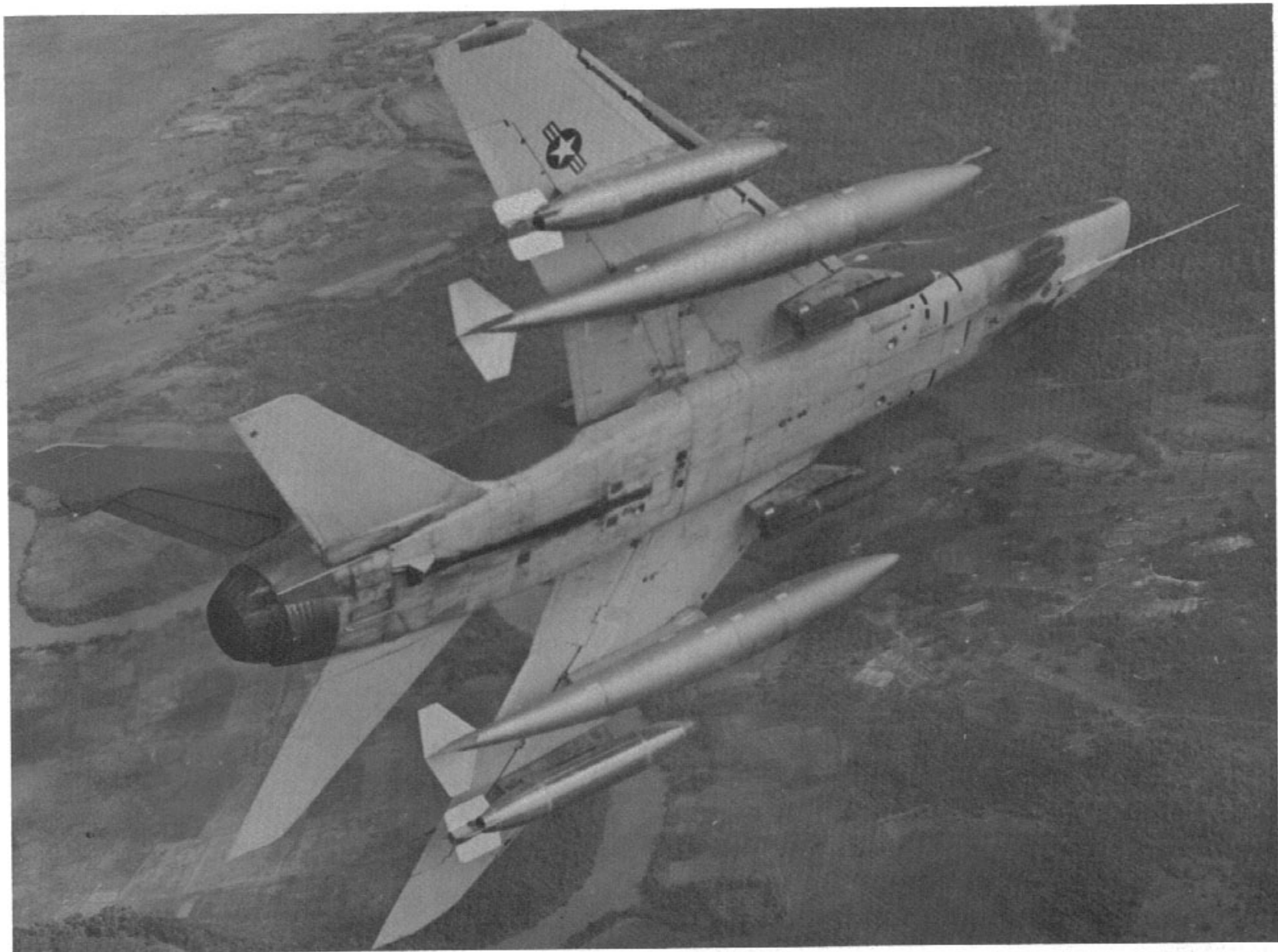
Super Sabre rolls in "hot". Note off-center position of arresting gear hook. The hook itself is flat steel spring which, when released, is held against the runway by spring tension. (USAF)
