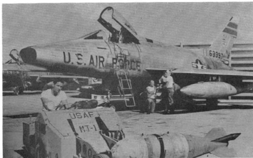
Loading bombs on a Hun of the 307th TFS at Bien Hoa in the fall of 1965. Bands on tail are light blue. (USAF via Dave Menard)
