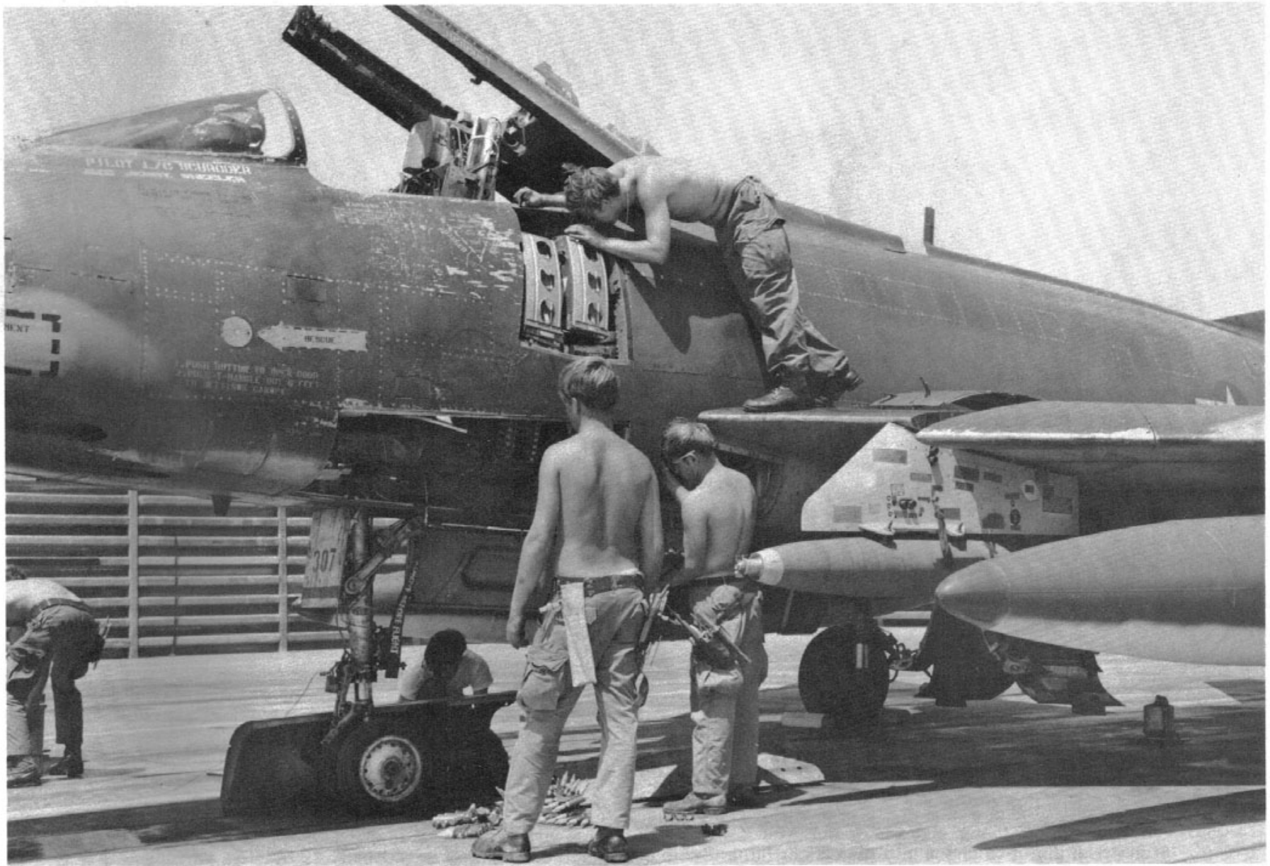
Munitions men loading M-39 cannon of F-100D-91-NA, assigned to 615th TFS, Phu Cat AB, March 1971. Super Sabre is also loaded with four 500 lb. bombs. (Norm Taylor)
