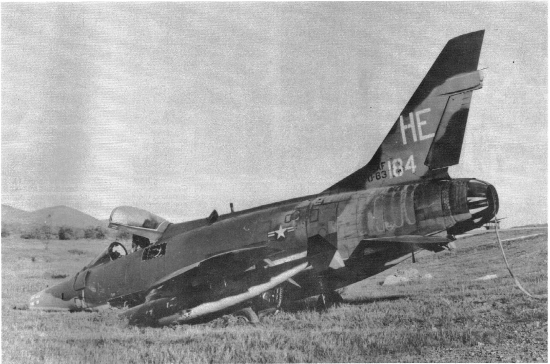
"My Gal Sal III" , an F-100D-71-NA of the 416th TFS came to grief, overrunning the runway at Phu Cat AB, in January of 1969, as a result of a broken hydraulic brake line. (USAF via Norm Taylor)
