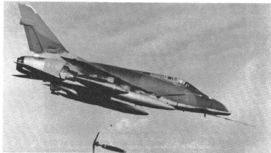
Super Sabre, with Napalm mounted outboard, delivering a high drag bomb from one of the inboard stations. Extended fins will slow descent of the bomb, allowing the F-100 to escape blast at low delivery altitudes. (USAF)
