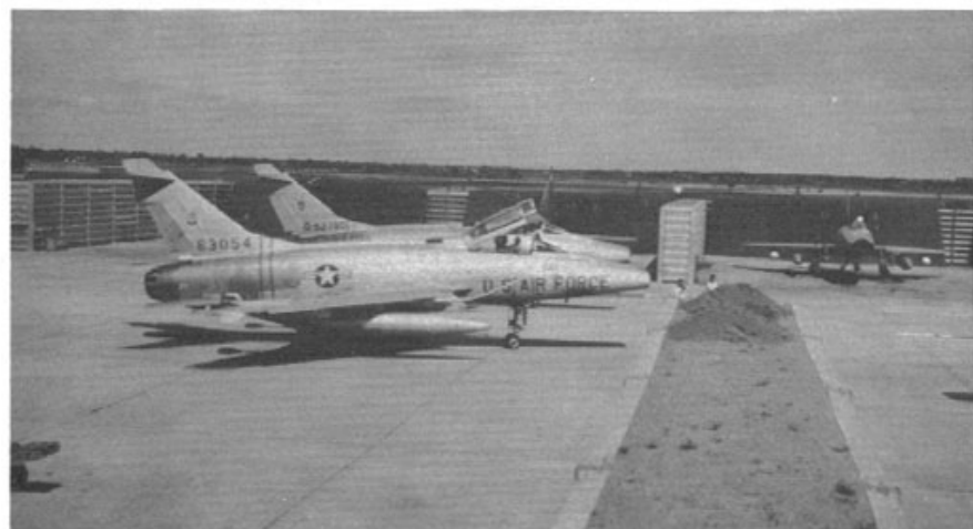
F-100's of the 481st TFS photographed from atop revetment at Bien Hoa AB. Note blast deflectors at rear of revetments in background. (Tom Lowe)
