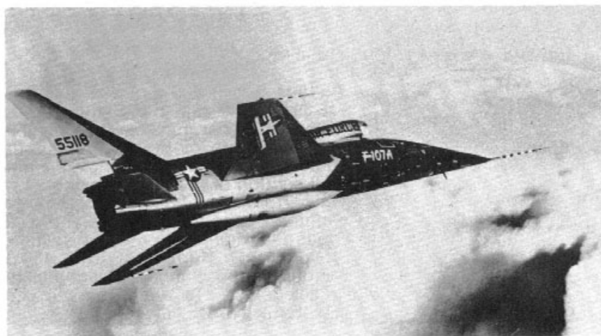
F-100-A's on the flight line at George AFB. (top) (North American) Ill-fated F-107A was begun as the original all-weather version of the F-100. It had a single J-75 engine, which delivered 23,500 lb. of thrust with afterburner. Only three were built. (left) (North American)
