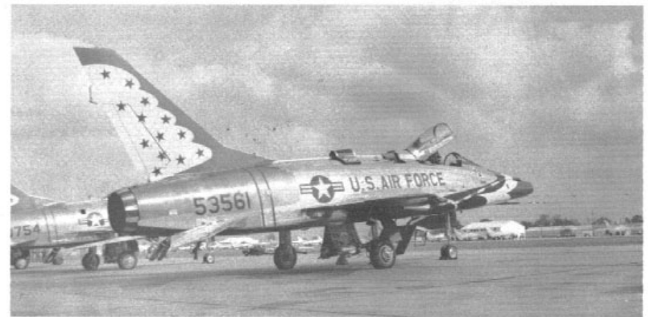
F-100D of Thunderbirds . Note plumbing for smoke system atop fuselage at bottom of vertical fin. (Paul Stevens)
