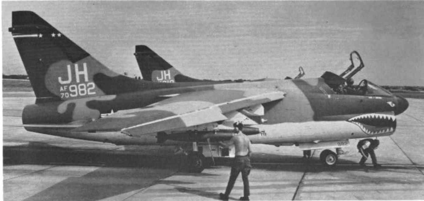
3rd TFS A-7D in the arming pits at Korat RTAFB, Thailand, prior to combat mission. Note that pilot keeps his hands out of the cockpit while arming crew removes safety pins. (greatly adding to their peace of mind.) (USAF)
