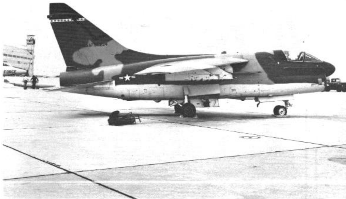
A-7D at Eglin AFB's Armament Development Test Center during weapons tests in 1971. Black outlined area on leading edge of vertical fin is VHF/Loran antenna. Tip of vertical fin carries UHF, Localizer antennas, and ECM Warning pod. (Norman E. Taylor)
