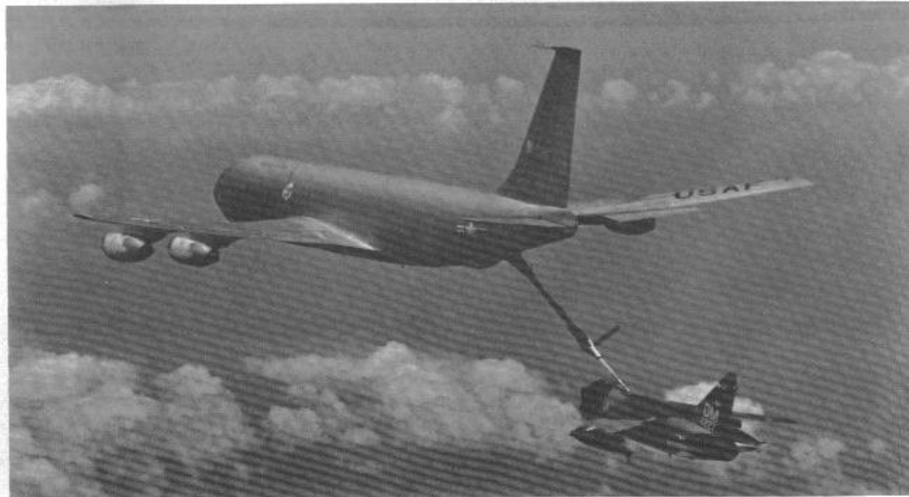
355th TFW A-7 on the tanker. With full external and internal fuel load, (2,625 gallons) A-7 has a range of 2,643 nautical miles. (LTV)
