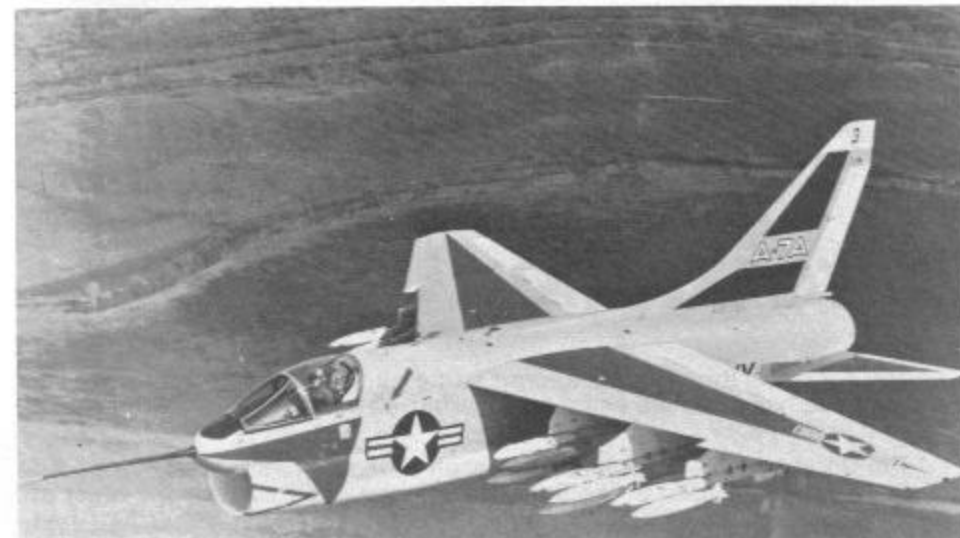
Prototype A-7A loaded with inert bombs on MERs. The Corsair II airframe has a design life of 4,000 hours, and is stressed for 7 G's at combat weight. Some of the black boxes carried by early A-7's included; APN-153 Doppler radar, ASN-41 nav. computer, APN-141 radar altimeter, ASN-50 all-altitude reference, ARN-52 Tacan, APQ-116 forward looking radar, TPQ-10 tracking radar, APN-154 radar beacon, and the CP-741 weapons delivery computer. (USN)
