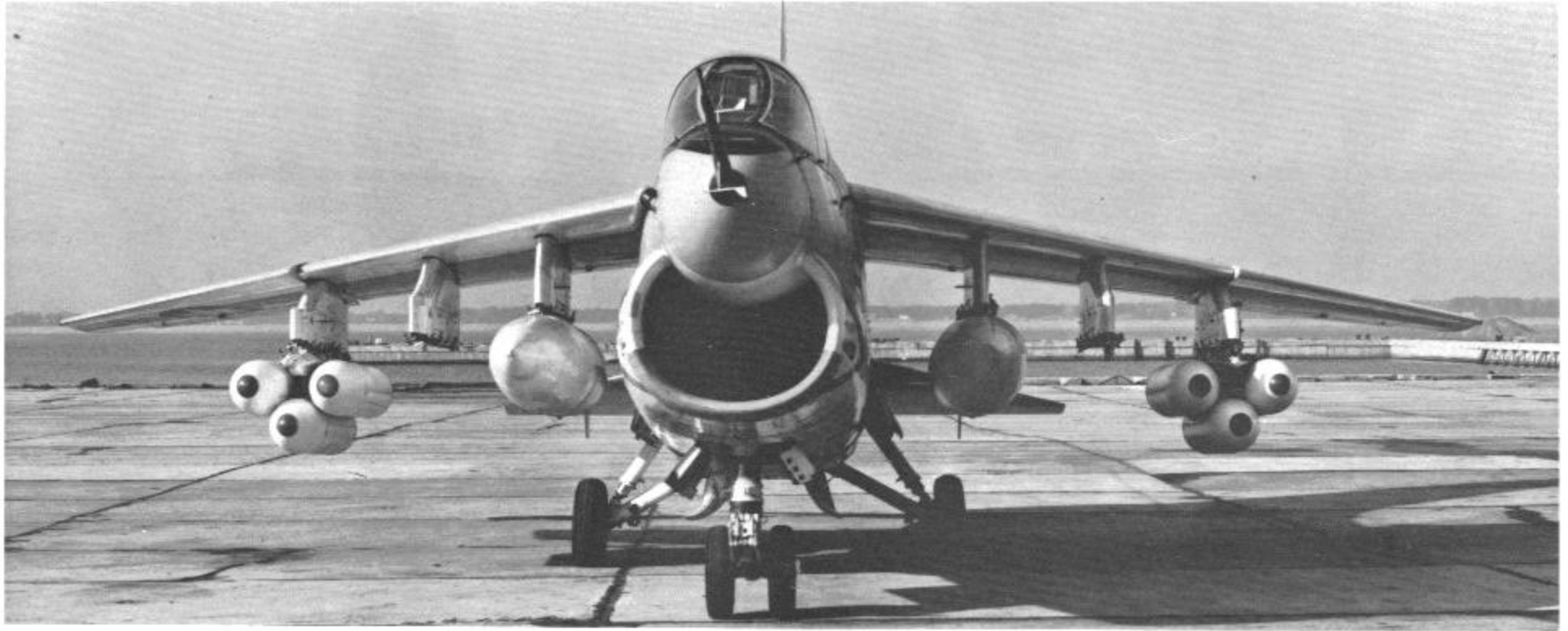
A-7A at NATC Patuxent River for weapons delivery tests in 1968. It is shown with Aero 1D 300 gallon fuel tanks inboard, and LAU-3A rocket pods on TER's outboard. Corsair II is capable of carrying up to 15,000 lbs. on it's six
