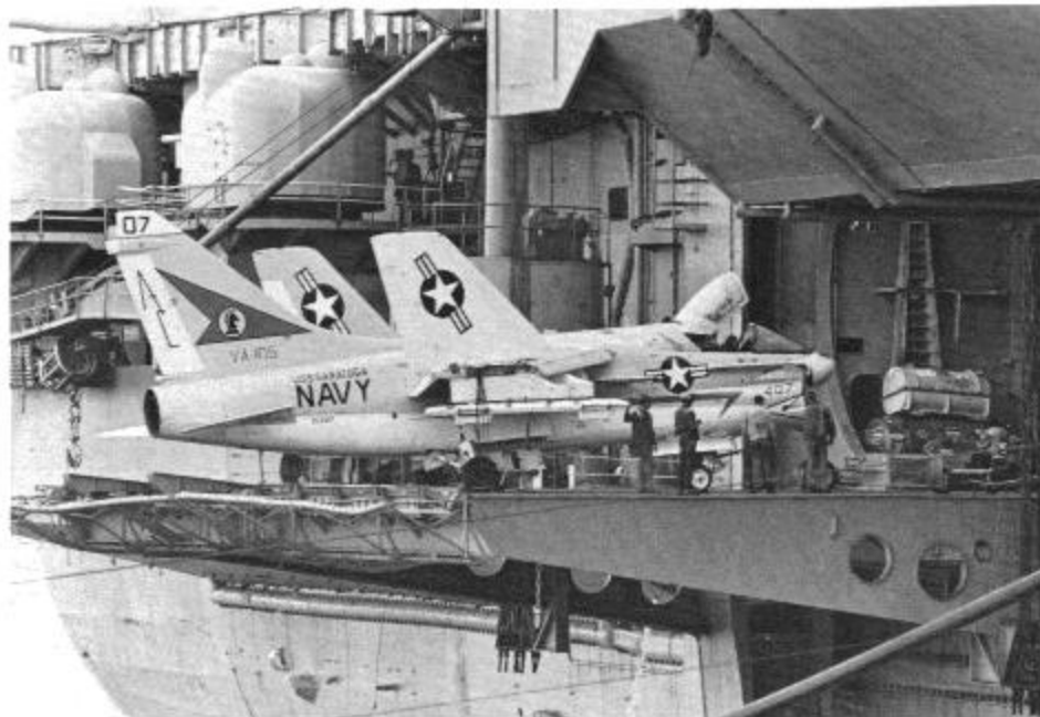
VA-105 Corsair enroute to the flight deck of USS SARATOGA aboard deck-edge elevator. (USN)
