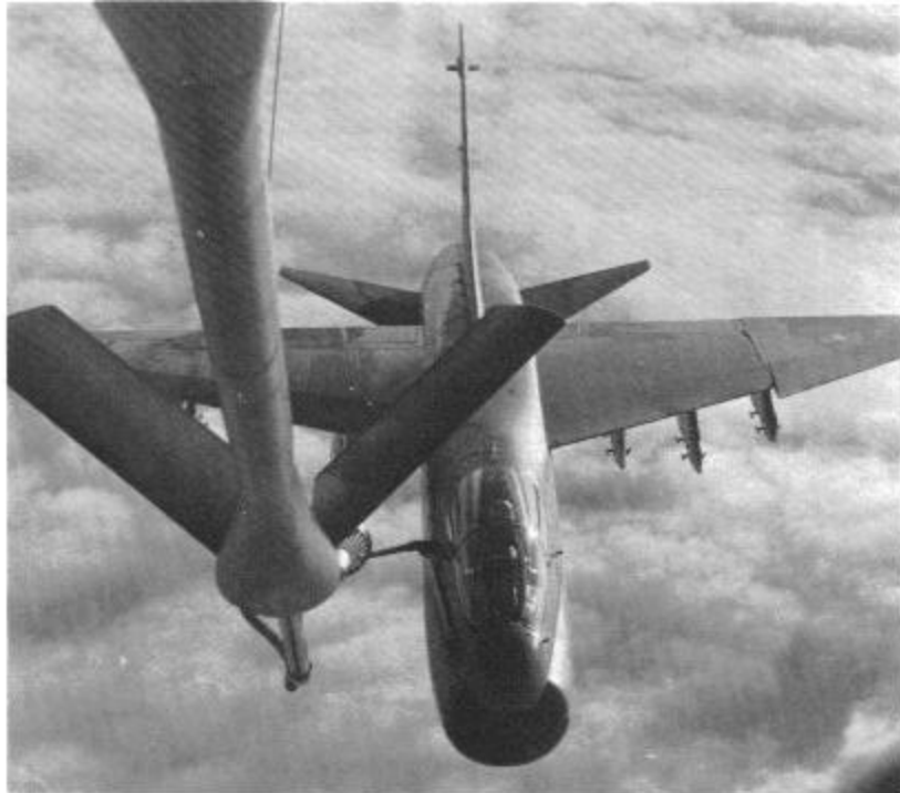
Early test model of the A-7D (AF SerNo 68-8222) during refueling tests over Alaska. Aircraft was flown by Major Robert Lilac, project officer from the 6510th Test Wing, Edwards AFB. First 16 "D" models retained the Navy probe and drogue refueling method. (USAF via Norman E. Taylor)
