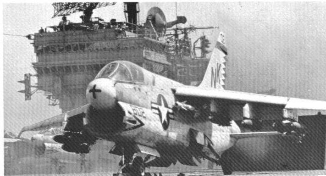
VA-27 Corsair II a split-second before it is launched from Constellation for a 1968 combat mission. Ordnance load consists of 10 500 lb. Snakeye bombs and a pair of Sidewinder AAM's. (USN)
