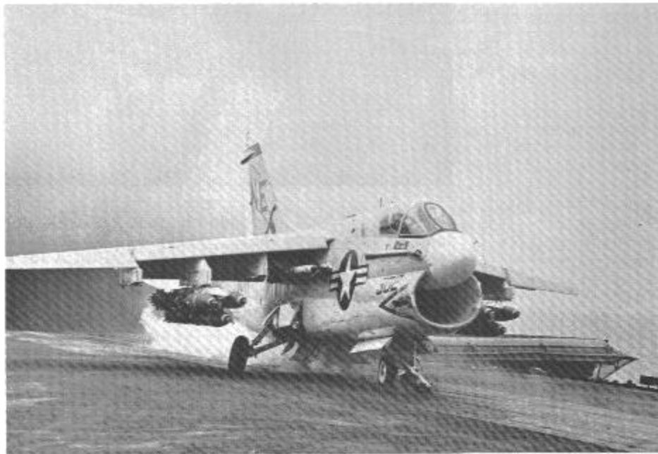
A-7 of VA-147 begins 250 foot trip down the number two catapult of USS Ranger. It is loaded with 12 500 lb. Snakeye bombs on MER's. (USN)
