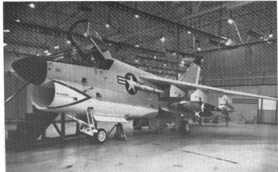
Full size mock-up of the A-7A as it appeared at the LTV plant in 1964. The F-8 nose cone was later eliminated as a space-saving measure. (USN)
