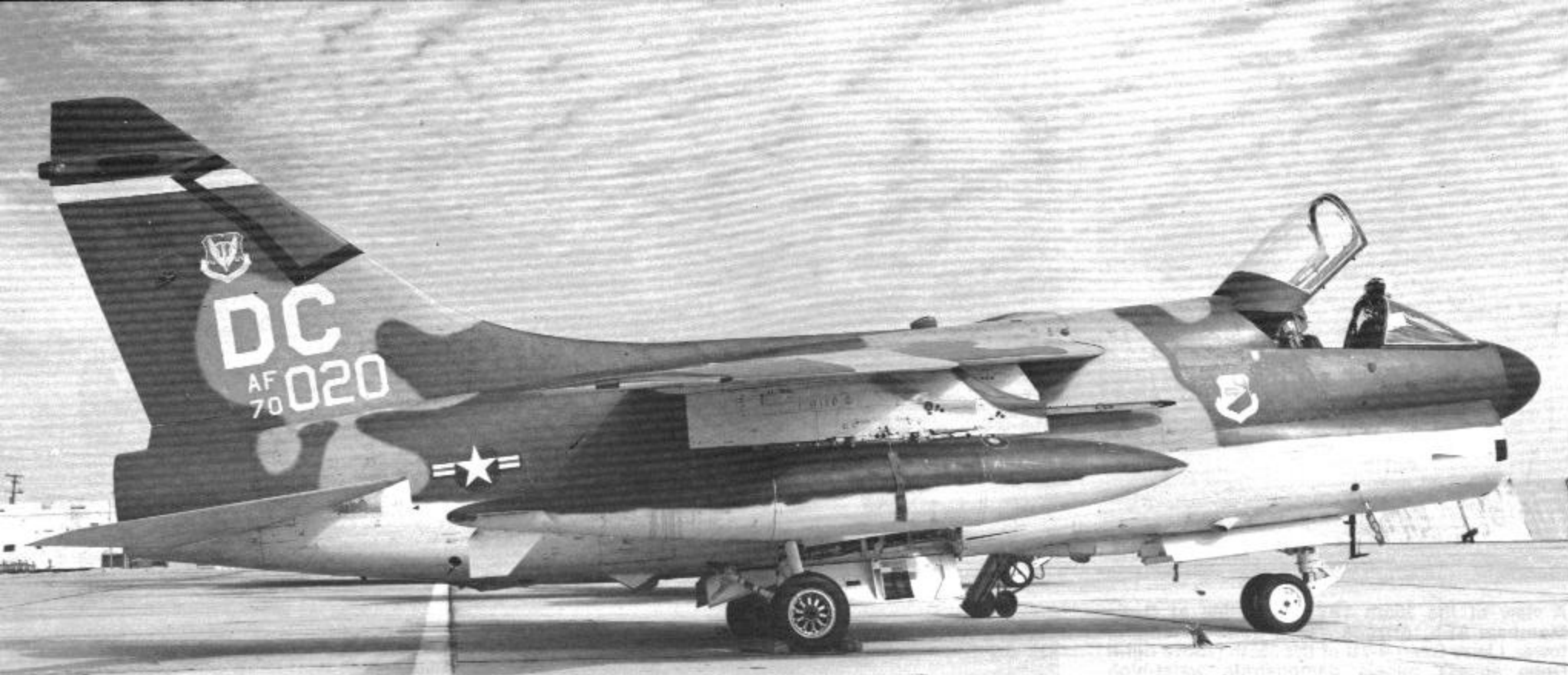
A-7D of the 357th TFS, 355th TFW. (above) (Norman E. Taylor) Avionics bay of A-7D. (left) (Jerry Geer) A-7 has 35 access panels, 90% of which can be reached without use of aircraft stand. Engine change can be accomplished in 30 minutes.
