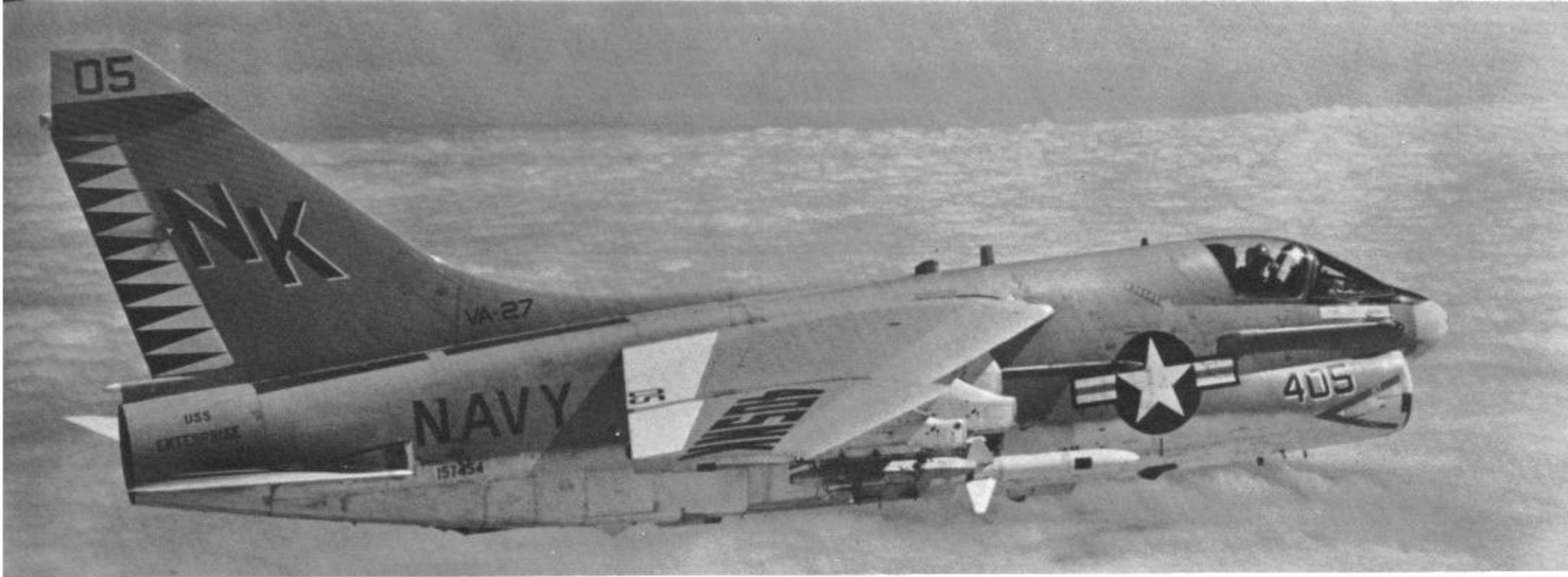
VA-27 A-7E returning to CVAN-65 after a strike on North Vietnam. It carries an unexpended Shrike missile on center pylon. (USN)
