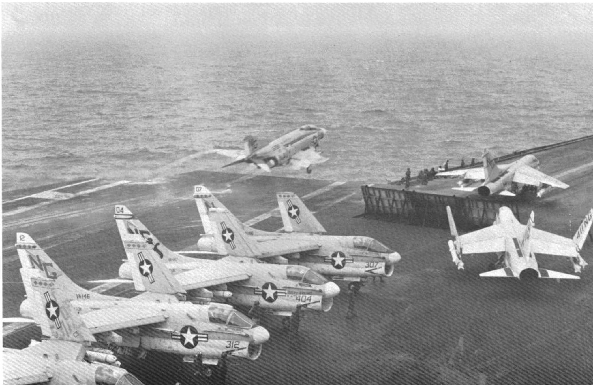
May, 1972: A VF-92 Phantom launches from the waist catapult of the USS CONSTELLATION as A-7's of VA-146 of VA-147 await their turns to launch
