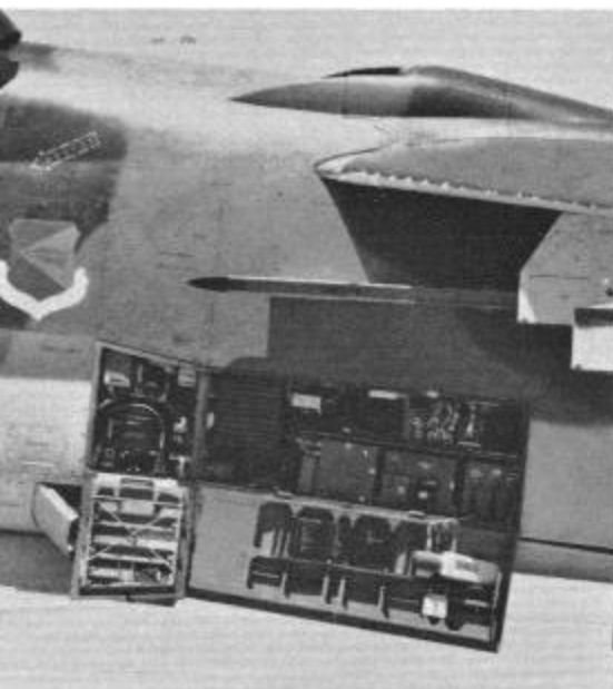
A-7D of the 357th TFS, 355th TFW. (above) (Norman E. Taylor) Avionics bay of A-7D. (left) (Jerry Geer) A-7 has 35 access panels, 90% of which can be reached without use of aircraft stand. Engine change can be accomplished in 30 minutes.
