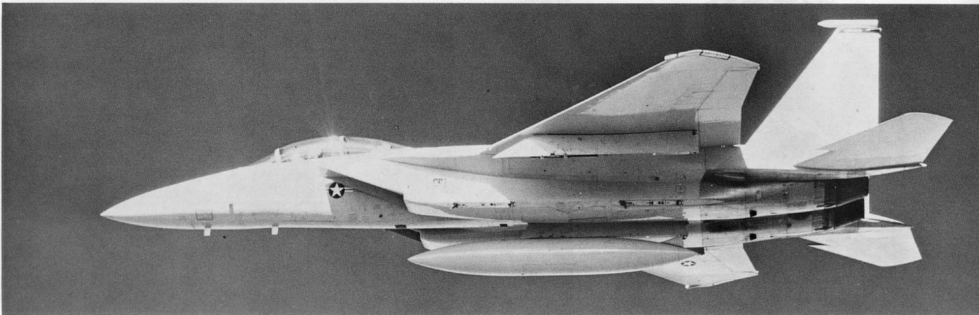
A Production F-15 shows "rounded" wing tips and "notched" leading edge of the horizontal stabalator. The first two F-15s had a straight leading edge on the stabalator. They were re-fitted with the production modification for
