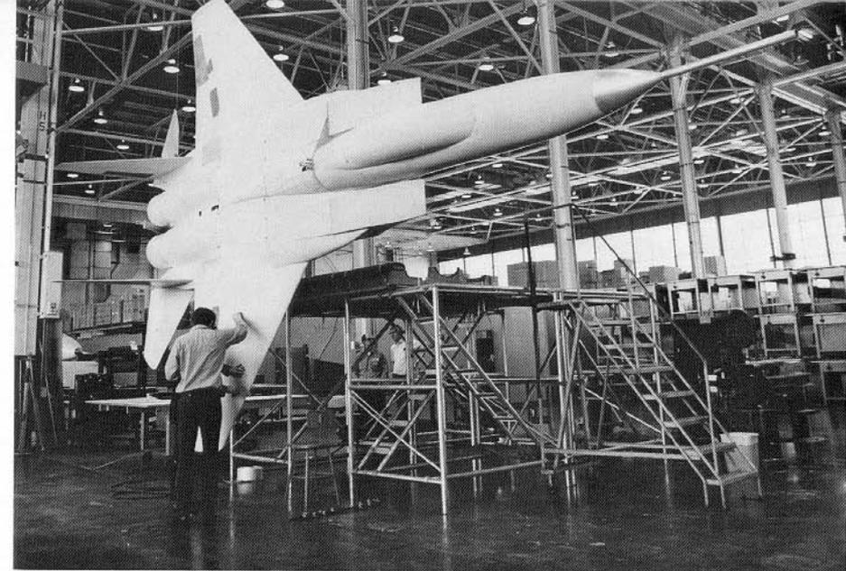
**This 5/8ths scale model of the F-15 was used for test drops from a B-52 launch aircraft. The remotely guided model was used to gather flight data and was then recovered by parachute to be used again. (McDonnell Douglas)**
