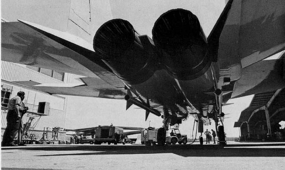
Ground level view shows location of four AIM-7 Sparrow missiles on lower corners of fuselage. The F-15 can also carry four AIM-9 Sidewinder missiles, 940 rounds of 20 MM ammunition, and a variety of ordnance totaling up to 12,000 pounds (McDonnell Douglas)
