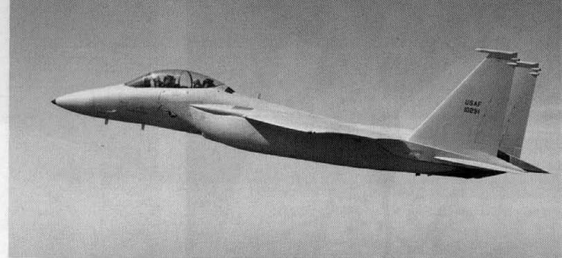
The F-15 Pulse Doppler radar offers "look down" capability, automatic and manual modes, excellent electronic counter measure resistance, long range, and modular design. It weighs about 500 pounds and is designed for ease of operation by a single pilot. Note the "Fast Pack" external fuel pallets outboard of the engines. [McDonnell Douglas]
