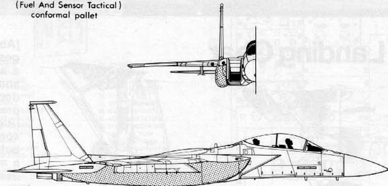
An F-15 with "Fast Pack" external fuel pallets outboard of the engines. "Fast Packs" each hold 4400 pounds of fuel and add a minimum of drag. The pallets can have Sparrow missiles mounted on their outboard corners. Special versions with reduced fuel capacity can hold ECM gear, reconnaissance equipment or weapons. This was not an Air Force Program. One set of pallets were built by the contractor and are not standard USAF equipment. (McDonnell Douglas)
