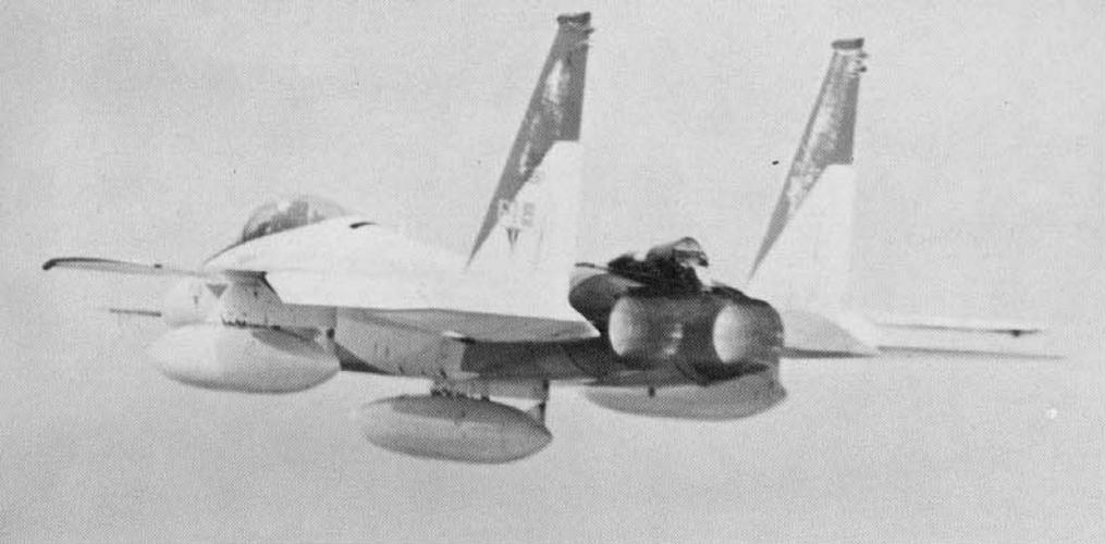
10287 accelerates in full afterburner. The aircraft is configured with three 650 gallon external fuel tanks. This aircraft was flown with many different ordnance and fuel loads to test its spin characteristics. [USAF]
