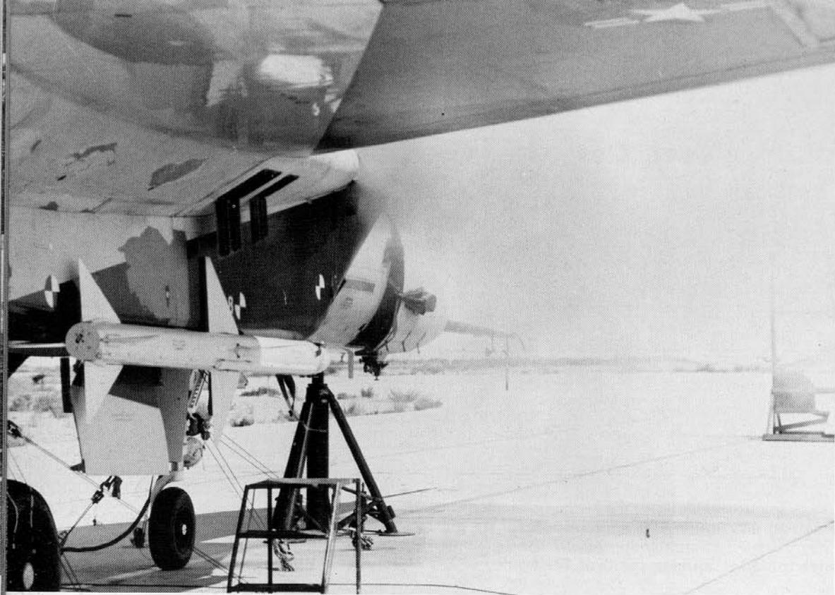
Ground test firing of the M-61 20MM gatling gun. The F-15 will carry 940 rounds of ammunition. An AIM-7 Sparrow missile is mounted on the lower fuselage corner. [McDonnell Douglas]
