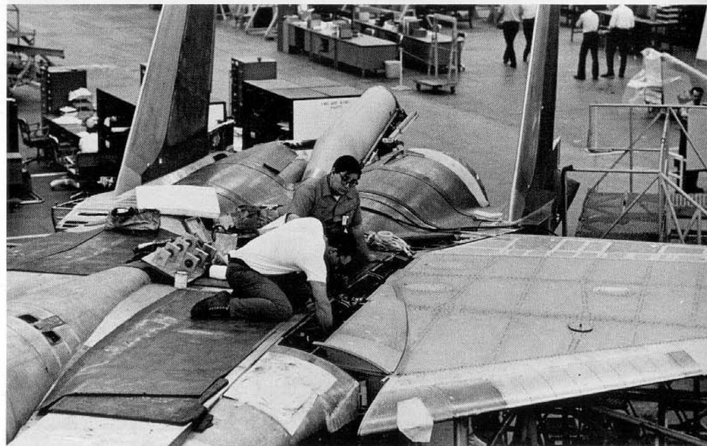
McDonnell Douglas employees attach the left wing to #10287. This was the test aircraft #8 used for spin evaluations. Note the spin recovery chute cannister installed between the tailpipes. (McDonnell Douglas)
