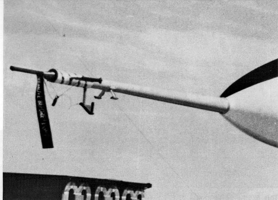
NOSE PROBE TEST BOOM
