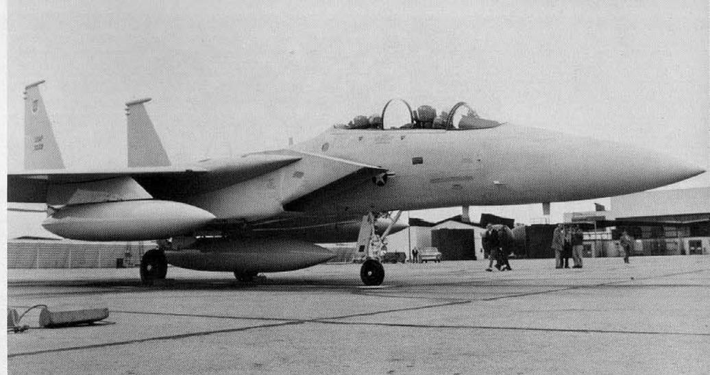
An F-15 prepares for flight from the McDonnell Douglas facility at St. Louis, MO. Note the variable inlet ramp (below rear cockpit) is down. These inlets move with different throttle settings and flight conditions to adjust air flow to engines during all phases of flight. (McDonnell Douglas)
