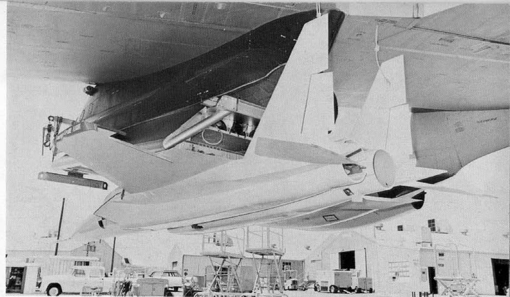
**This is the F-15 scale model mounted under the wing of a B-52 launch aircraft at the USAF Flight Test Center, Edwards AFB, Calif. It was used in a series of tests to gather flight characteristics data for actual flights that followed. (NASA)**
