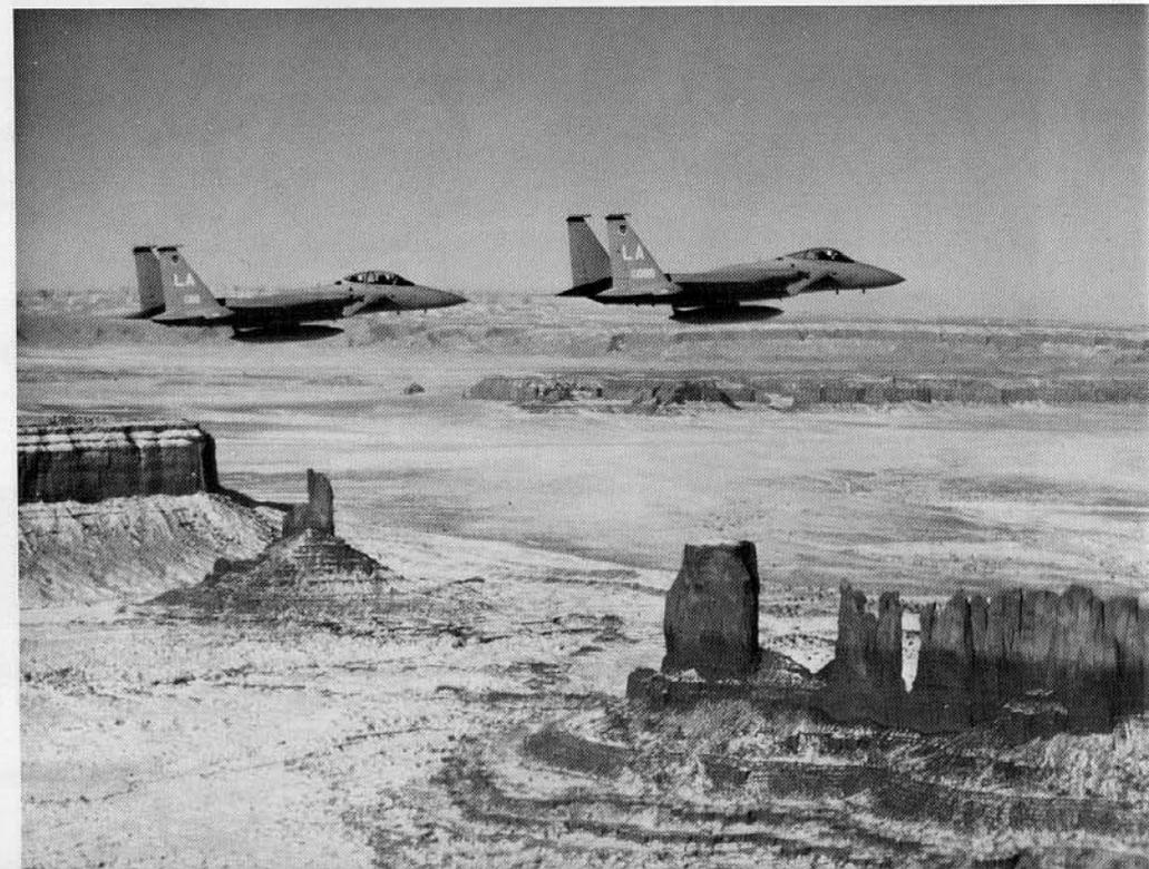
(Above) An F-15 Eagle takes off at Luke AFB, Ariz. The F-15 can take off in less than 1000 ft. in its interceptor configuration of full internal fuel and four AIM-7 missiles. (Right) An F and TF-15 fly formation over Monument Valley, Ariz. The F-15 is extremely stable and responsive in formation flying. (USAF by Kokojan)
