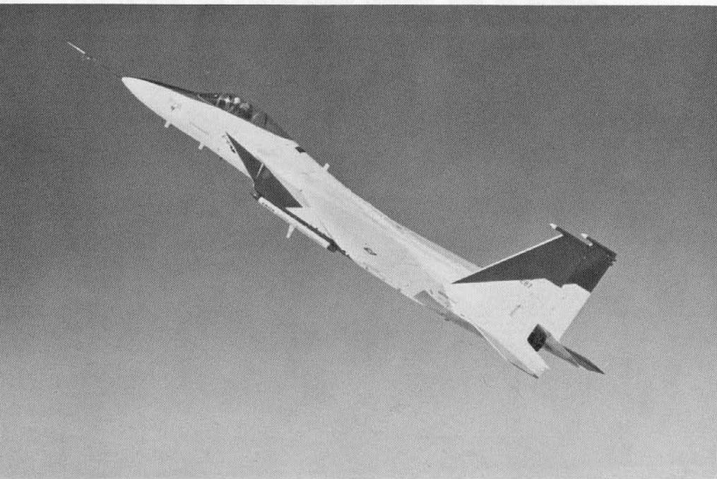
Aircraft #8 (10287) in white and day glow orange paint scheme shows off its impressive rate of climb in military power (non afterburner). Note the absence of exhaust smoke. Smoke is a give away in air combat since it makes it easier for an enemy to visually find an aircraft. (USAF)
