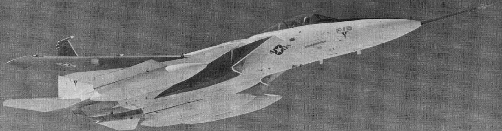
Aircraft #8 was painted white and orange for better visibility and radar reflectivity by chase aircraft. It was used to conduct spin tests and was
