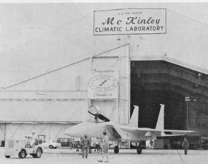
(Above) The seventh production Eagle during pre-acceptance flight trials over the farmlands of Missouri. (McDonnell Douglas) (Left) An F-15 is towed from the McKinley Climatic Laboratory at Eglin AFB, Florida. This hangar can duplicate weather conditions over a wide range of temperatures. Tests done here check the aircraft's operating capabilities in extreme climates. [USAF] (Right) Irv Burrows, McDonnell Douglas Chief Test Pilot, dismounts after the F-15's first flight. [McDonnell Douglas]
