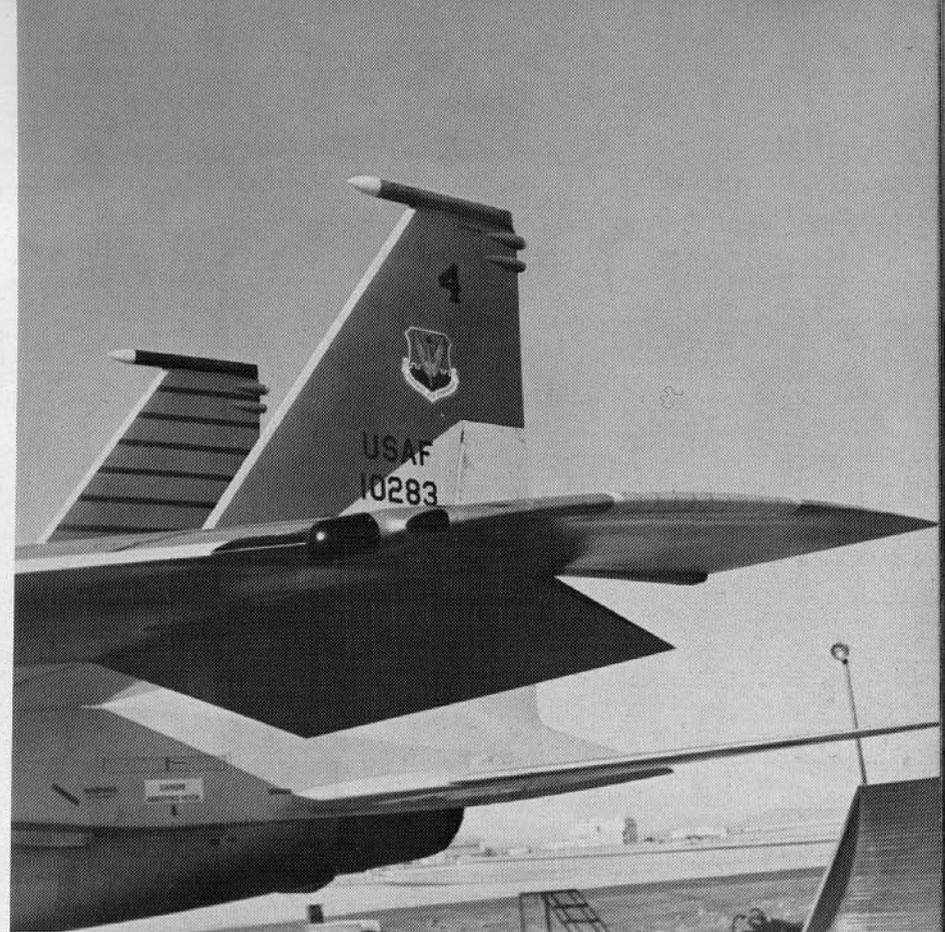
Close up detail of F-15 wing tip. "Day glow" orange paint was used during the flight test period to make the F-15 easier to see from chase aircraft and the ground. Black horizontal stripes on the inside of the tails were to measure flutter during speed brake tests. The white rectangle areas under the wing, just above the "danger" sign, are indirect lighting for formation flying at night. (McDonnell Douglas)
