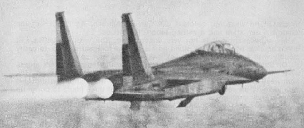
**Maj. "Mac" Macfarland accelerates to 500 knots before climbing straight up to set a new 6,000 meter record. The F-15 accelerated through the speed of sound (Mach 1) 23 seconds after brake release. Maj. Macfarland also set new 9,000 and 12,000 meter climb records in the F-15. (USAF)**
