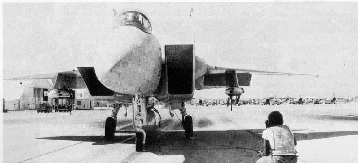
Ground crewmen remove intake duct dust covers and make final checks on a 555th F-15 as the pilot climbs into his bird for a mission at Luke AFB, Ariz. The F-15 is a large aircraft. The height to the top of the tails is 18 ft. 5 in. It is 12 ft. to the top of the closed canopy. (USAF by Kokojan)
