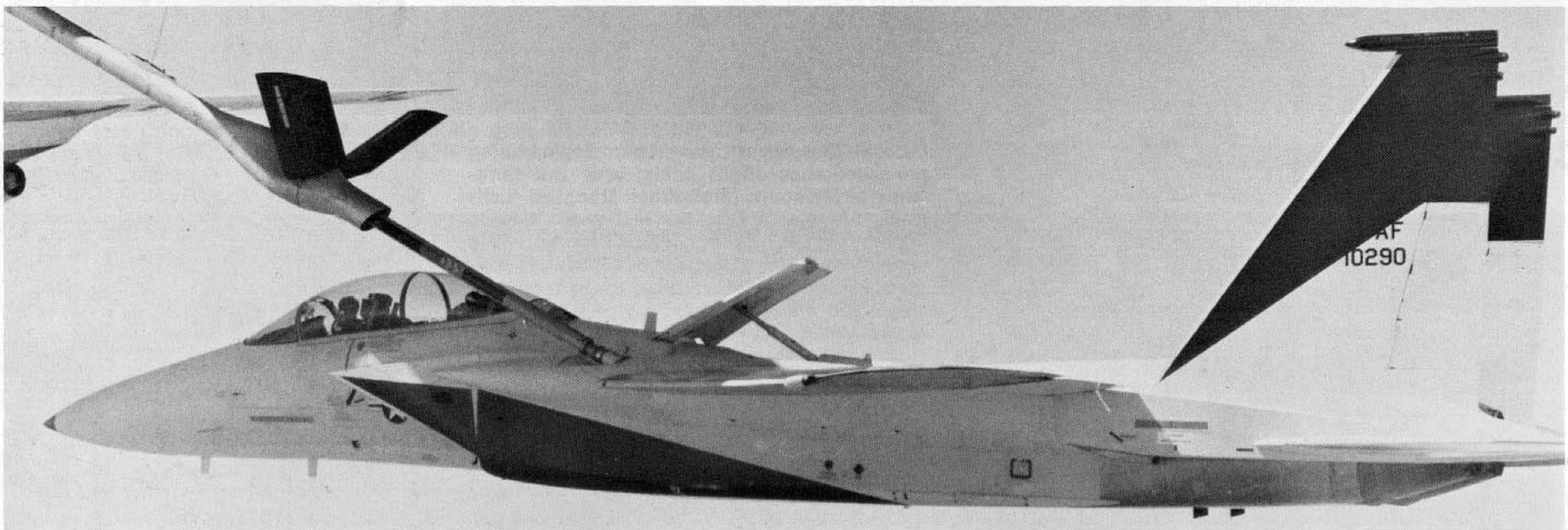
An F-15 (10290) in the test paint scheme takes on fuel from a KC-135 tanker during the tests. Note the hydraulic actuator that extends the speed brake. (USAF)
