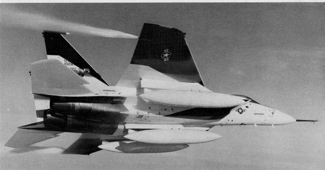
10287 vents fuel from wing ports as it returns from a spin test mission. The F-15 has proven to be a very stable aircraft and fully recoverable from any type of spin that it can be forced into. (McDonnell Douglas)
