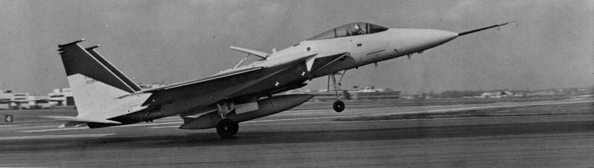
Aircraft #5 (10284) in test colors is shown during a landing with the speed brake extended. The F-15 has excellent brakes and with its low landing
