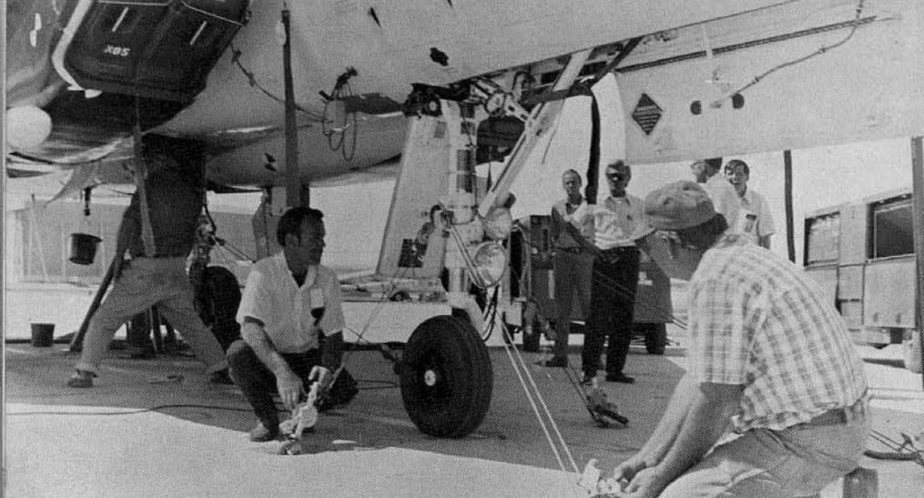
McDonnell Douglas maintenance technicians prepare an F-15 for flight at the Edwards flight test center. Air Force and contractor maintenance men worked side by side during the test program. Note detail of nose gear and door assembly. Also warning stenciled on intake cover — an allusion to engine capability to “pick your pockets” (McDonnell Douglas)
