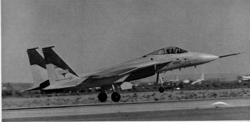
The first F-15 (10280) takes off from Edwards AFB, Calif. The long boom on the nose of the radome was used on some aircraft during the test flight period for special instrumentation. Production F-15s do not have the boom. (McDonnell Douglas)
