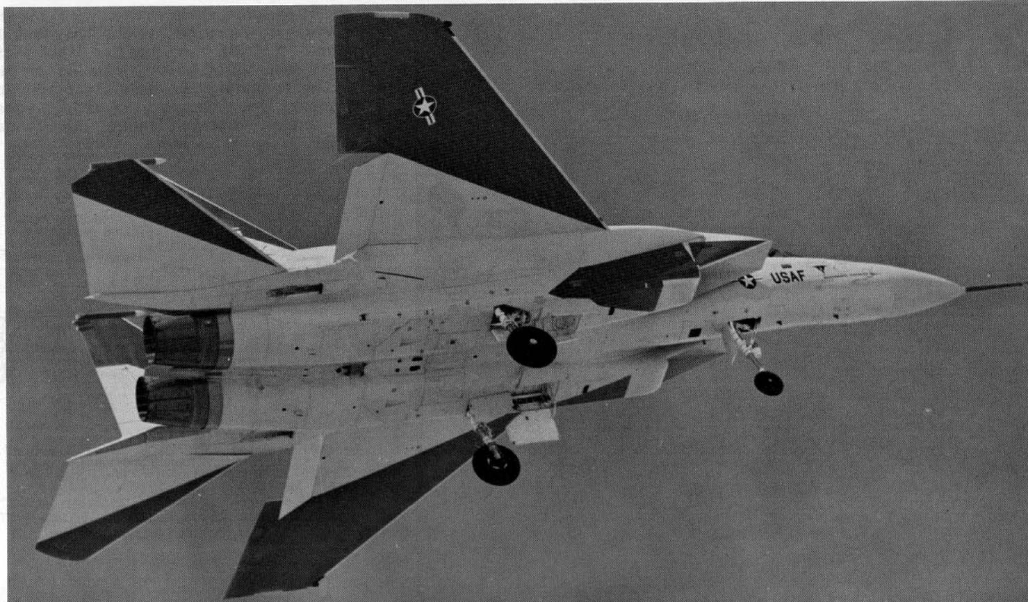
Aircraft #1 (10280) in orange and blue paint scheme takes off from the Edwards AFB runway. The F-15 has so much power that afterburner is normally not used for takeoff. Note the elevons do not have the "notch" in their forward surface. The first two F-15s came from the factory this way but were later modified with the "notched" elevon that is now used on all F-15 models. (McDonnell Douglas)
