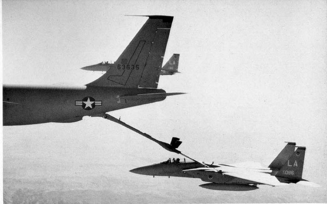
A TF-15 (73110) of the 555 TFTS takes on fuel as an F-15 waits off the right wing of the KC-135 tanker. Every seventh F-15 off the production line is a two seat "TF" model. The only external difference is a slightly raised rear portion of the canopy. Performance of both models is essentially the same. The "TF" weighs about 800 lbs. more than the "F". (USAF by Kokojan)
