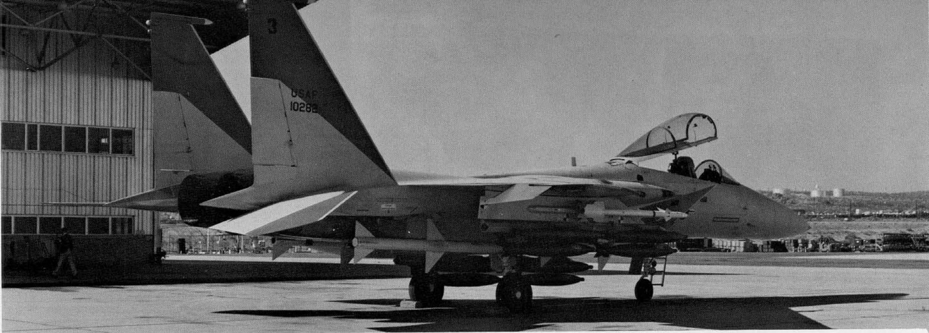
Aircraft #3 (10282) with a mixed load of air-to-air and air-to-ground ordnance. See chart below for Weapons Stations and Loads. (McDonnell Douglas)
