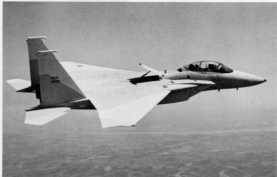
TF-15 (10290) returns to St. Louis plant after a test flight. Note the speed brake extended to help slow the aircraft. The speed brake is very effective and may be opened at any speed up to the aircraft limit. (McDonnell Douglas)
