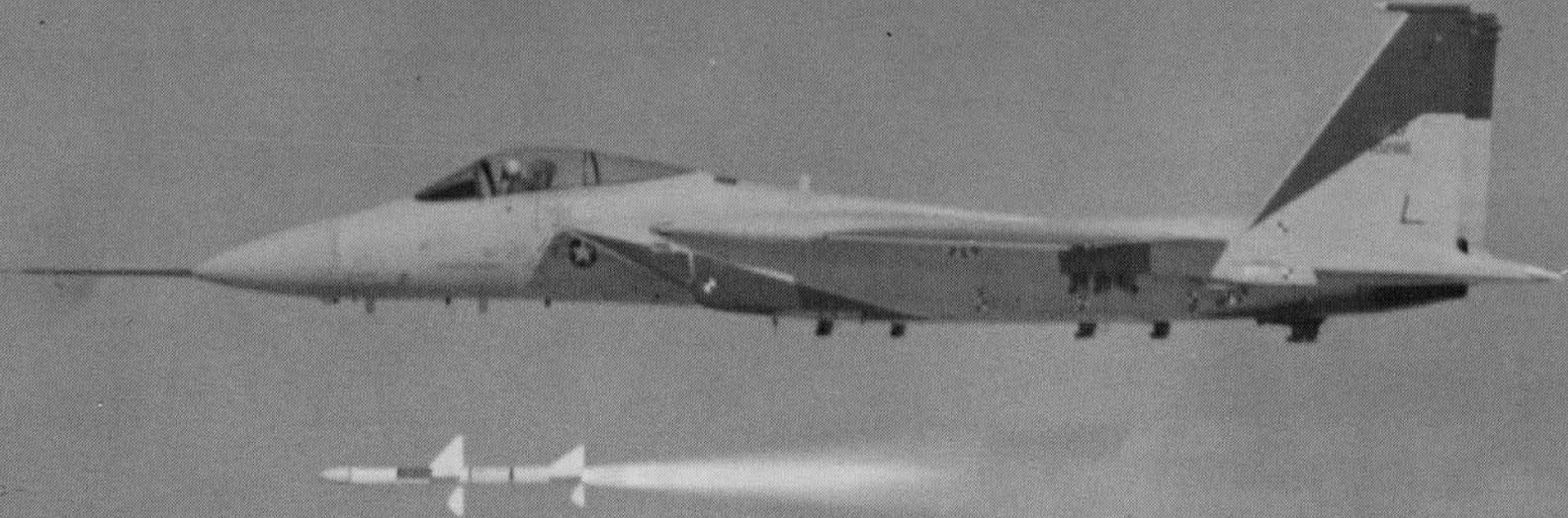
[Above] Aircraft #7 [10286] fires an AIM-7 "Sparrow" medium range air to air missile. The F-15 can carry four AIM-7 radar missiles and four AIM-9 "Sidewinder" infra-red missiles. The aircraft also has 940 rounds of 20
