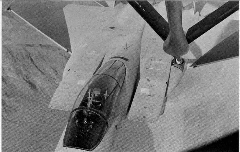
This is what the KC-135 boom operator sees as an F-15 moves into position to take on fuel. Refueling slip away door (not open in this photo) is outlined by the orange rectangle on the left wing root area.
