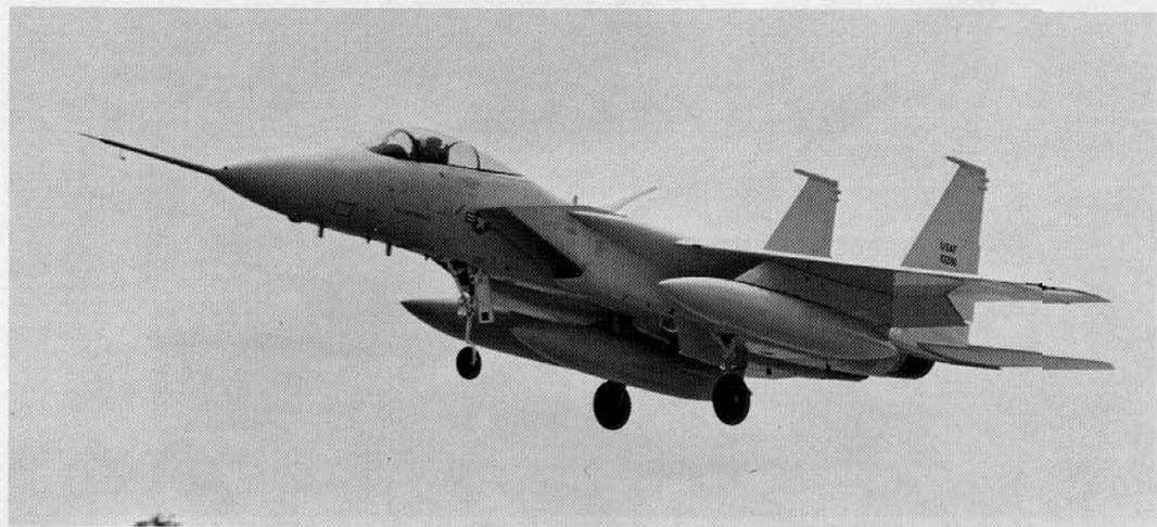
F-15 with three 650 gallon fuel tanks comes in for a landing. The F-15 lands at relatively slow speeds and does not require a drag chute to help stop. The aircraft does have an emergency tail hook to use in case of brake failure. (McDonnell Douglas)
