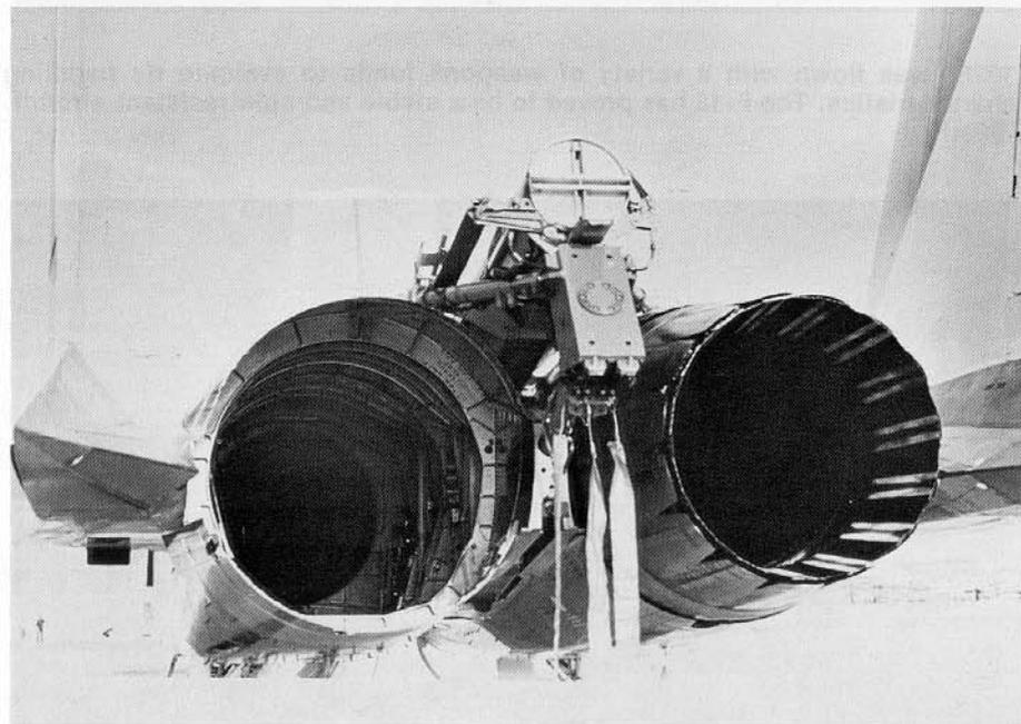
Close up shows details of the spin recovery chute installed on Aircraft #8 (10287). This was the only test aircraft to be fitted with a spin chute. Production F-15s do not have spin chutes. (USAF)
