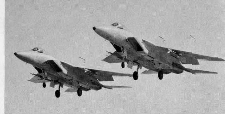
Two Eagles come in for a formation landing. Both aircraft have AIM-9 Sidewinder missiles mounted on wing pylons. The F-15 can carry both AIM-9 and AIM-7 Sparrow missiles, giving it great weapons flexibility during aerial combat. (McDonnell Douglas)
