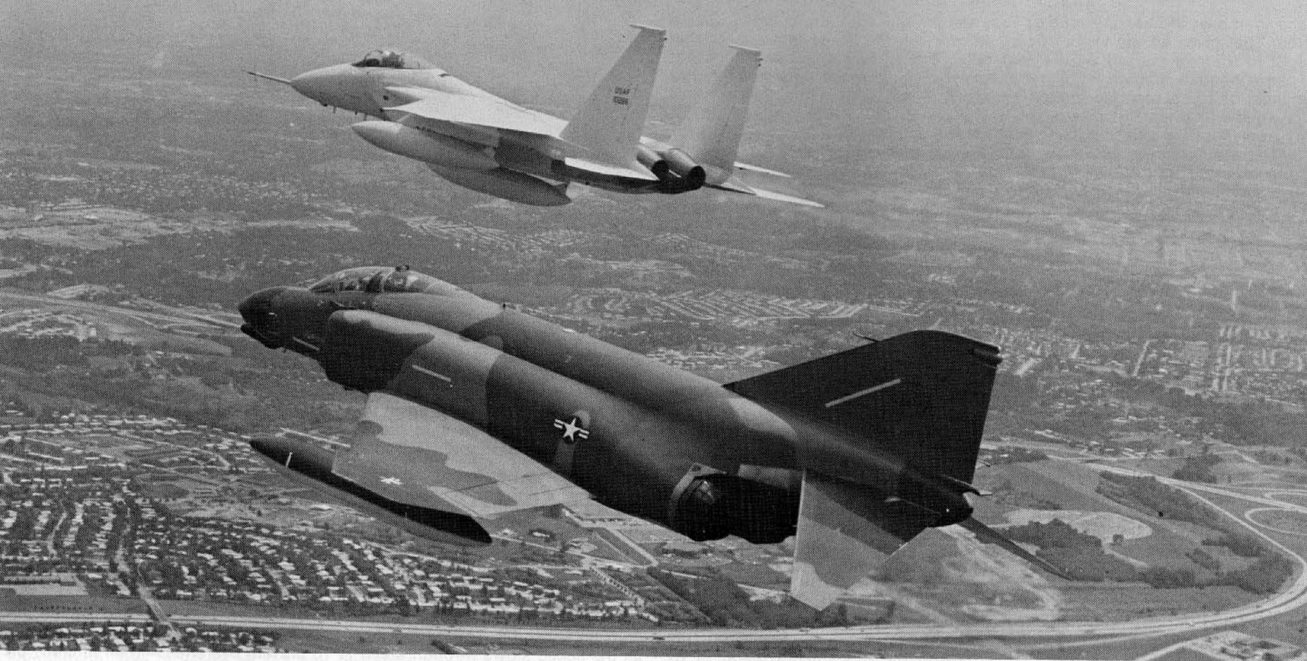
**F-4 chase plane flies formation on an F-15 with three 650 gallon fuel tanks installed. F-15 performance exceeds that of the F-4 by a wide margin.**
