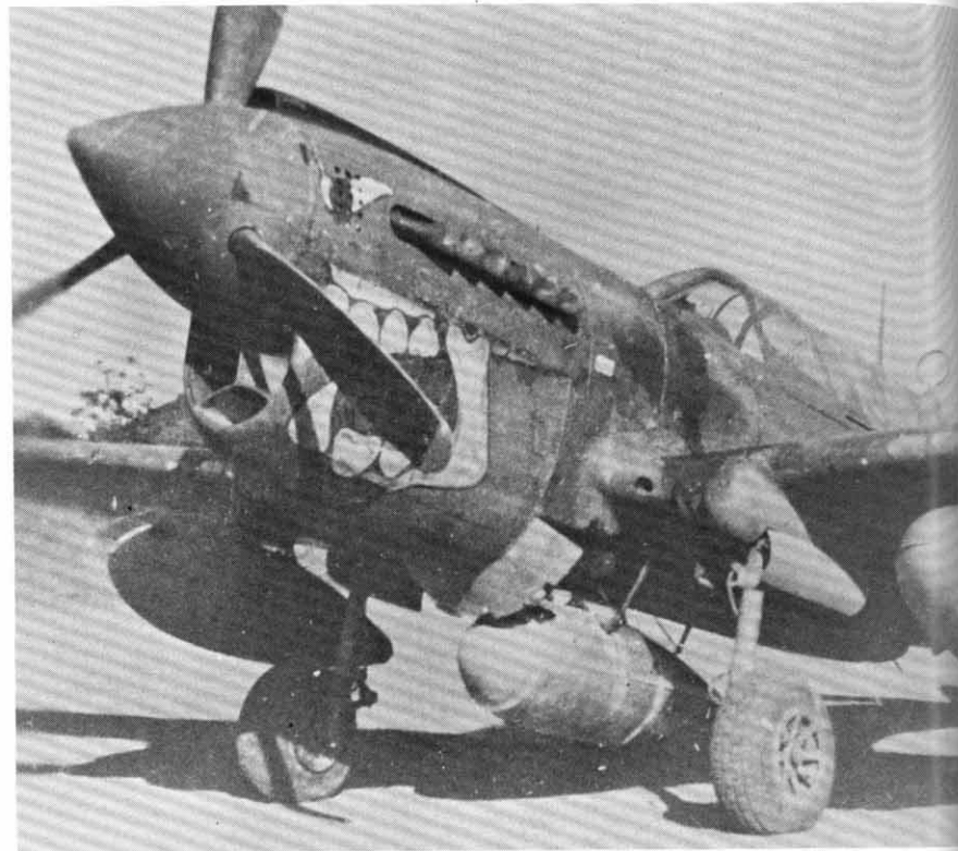
The photo above is unusual in that only the jaw bones and teeth show, possibly the upper cowl was damaged and replaced and an eye hastily painted in or that portion of the cowl could have come from a hanger queen that had the sharkmouth scheme. Note also that this aircraft has three drop tanks mounted possibly for ferrying or photo recon work.
