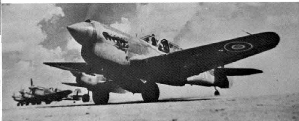
Flight of Kittyhawk Mark Is take off in line abreast formation to reduce amount of dust each had to face. All leading edges of these aircraft were soon scoured down to bare metal and their wind screen and canopies were scored and dulled, hence taking-off with an open canopy was SOP. Sand and grit played havoc with engines and other working parts. [SA War Museum]
