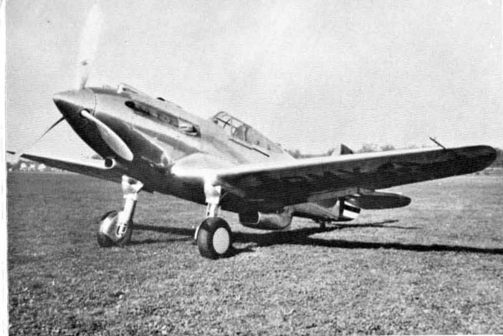
The XP-40 Prototype, Air Corps serial number A.C. 38-10. Designer Donovan R. Berlin elected to locate the scoop for the radiator under the belly, but fear that it might be damaged by debris thrown up by the slipstream on takeoff and landing led to its relocation. Berlin was later proven correct when the North American P-51 flew with the radiator in the same location. [USAAF]
