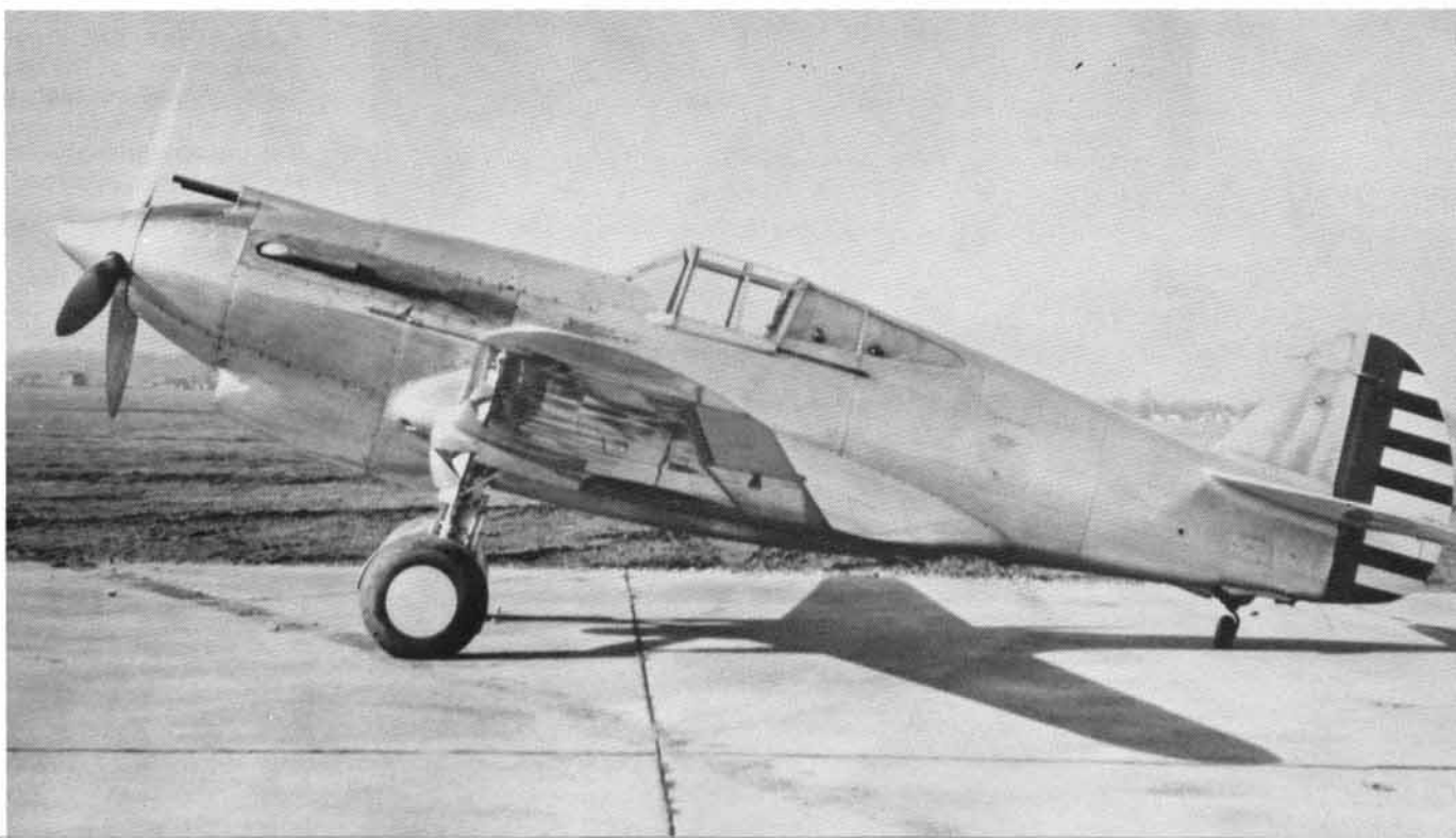
The XP-40 Prototype in final form, now carrying twin .50 cal. machine guns in oversized blast tubes, which doubled as caburetor intakes. The most obvious external alteration is the repositioning of the radiator air scoop.
