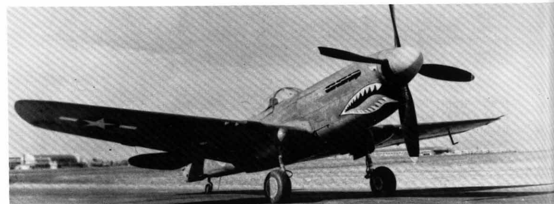
[Bottom] XP-40Q second form with wing guns mounted. Note the underwing pilot tube, a departure from the Curtiss practice. [USAF Museum]
