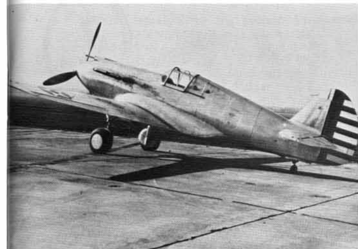
The XP-40 Prototype in final form, now carrying twin .50 cal. machine guns in oversized blast tubes, which doubled as caburetor intakes. The most obvious external alteration is the repositioning of the radiator air scoop.
