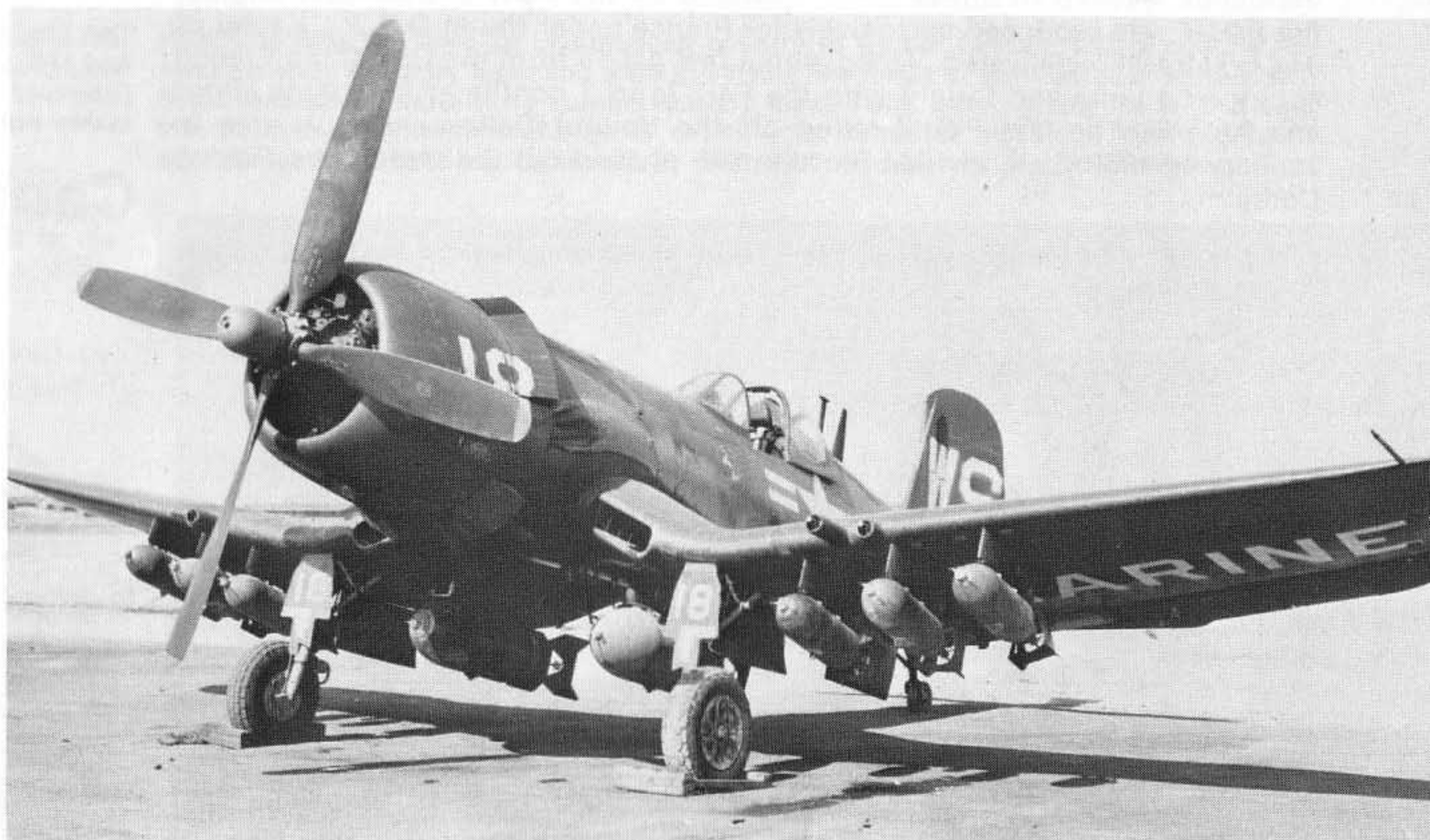
AU-1 of VMA-323 packs 6 250-lb., 1 500-lb. and 1 1,000-lb. bomb for close air support, February 20, 1953. [USMC]
