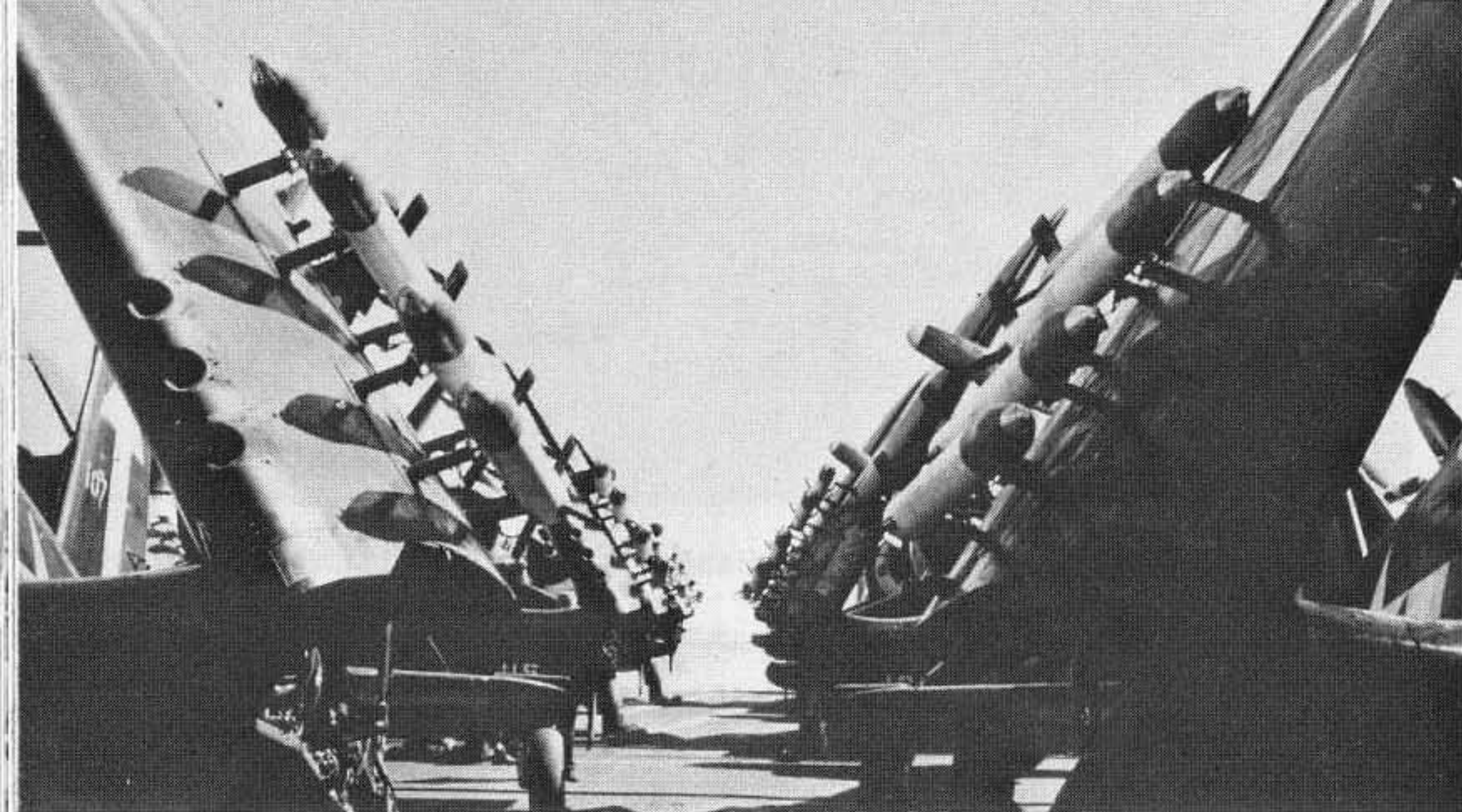
F4U-1Ds of VMF-221, 451 and VF-84 armed with 5-in. High Velocity Air Rockets [HVAR] onboard the USS Bunker Hill just prior to strike that marked the beginning of the invasion of Iwo Jima, February 19, 1945. [National Archives]
