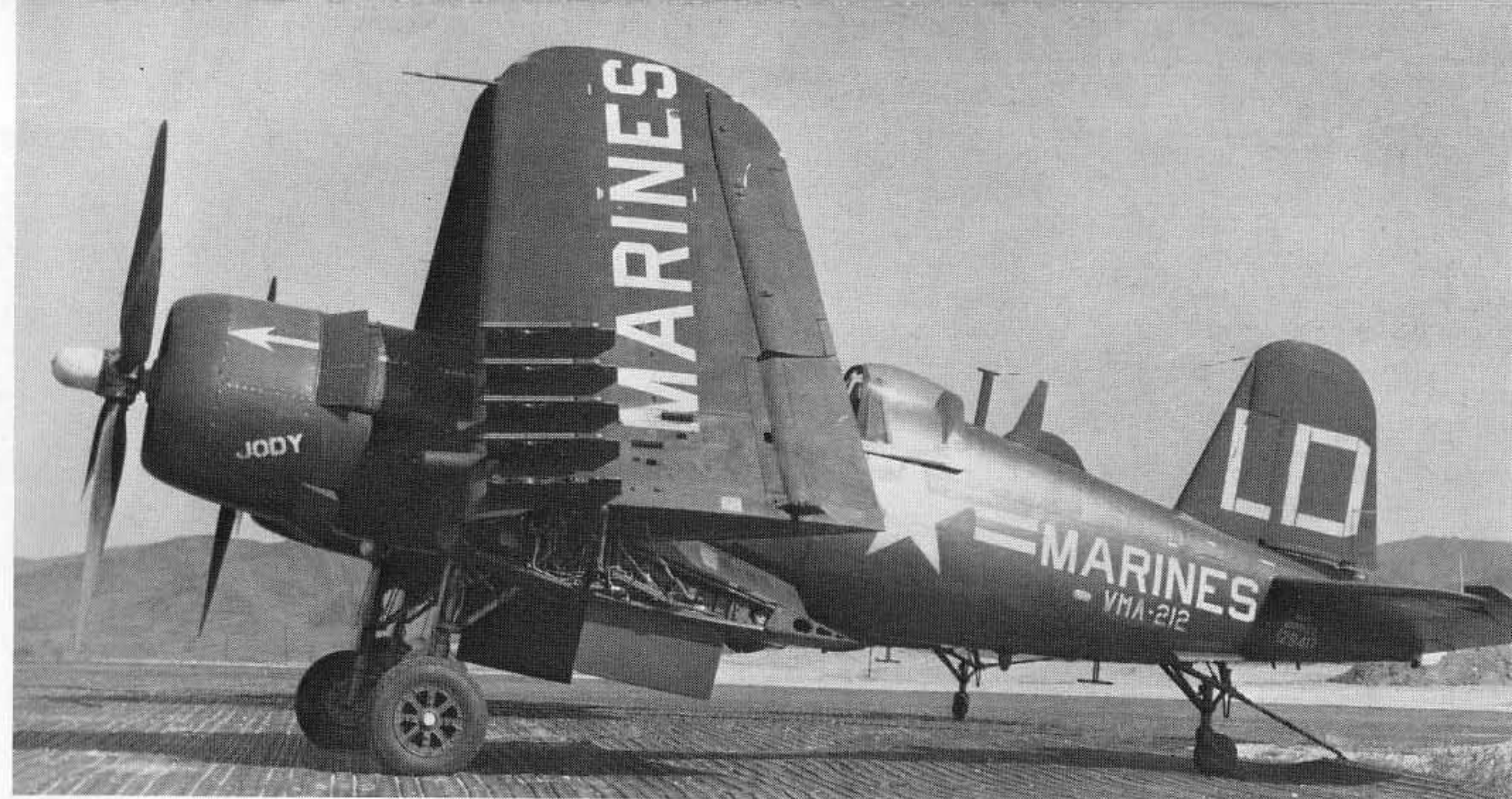
AU-1 [129417] of VMA-212 at K-3, Pohang, Korea in 1953. Note the 5 underwing racks for HVARs or 100-lb. bombs, 1953. [Clay Jansson]
