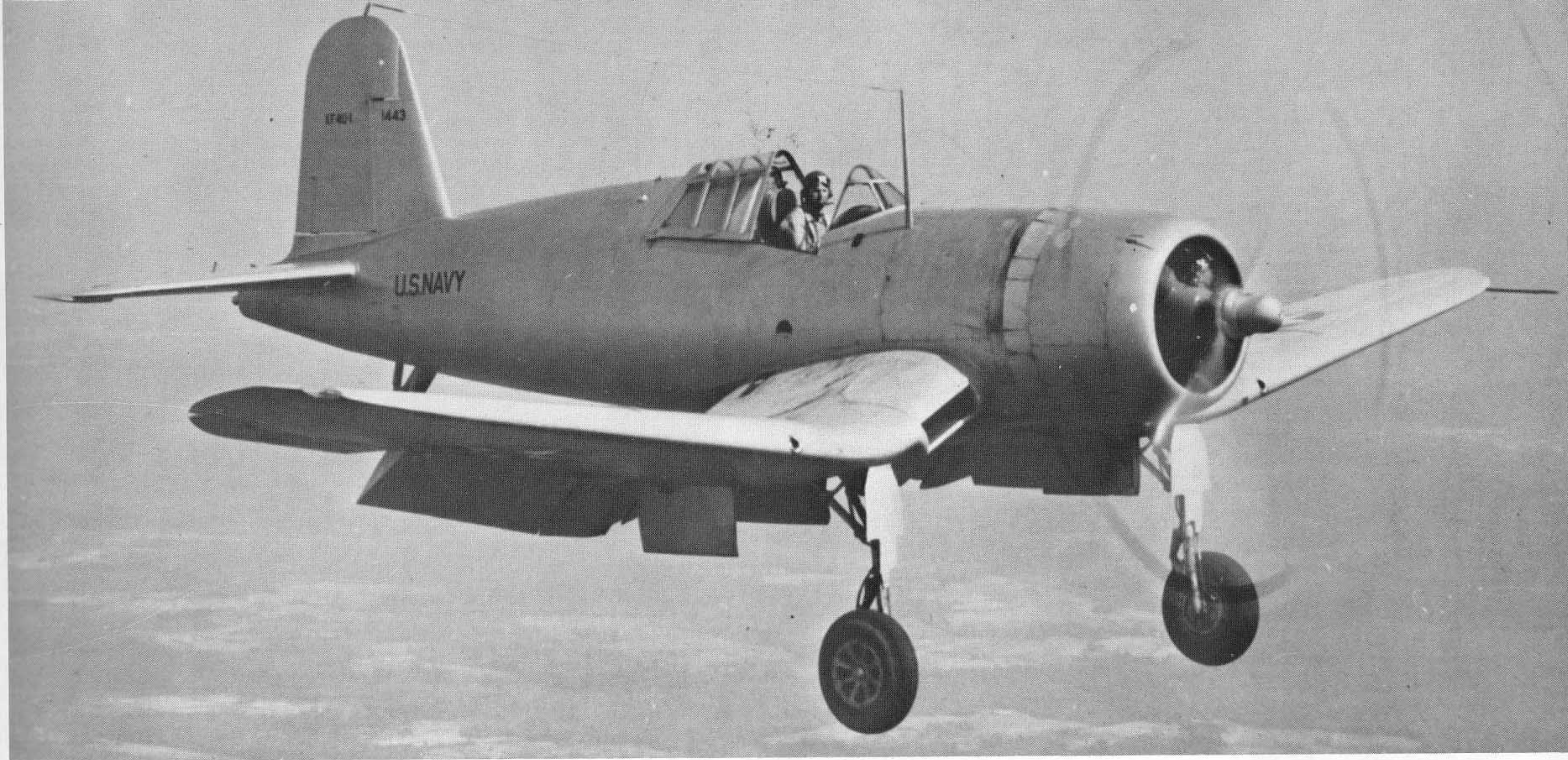
Flight testing for the XF4U-1 by Vought test pilots over the Connecticut countryside. Landing configuration has flaps and gear down, canopy in the open position. [See centerspread for color markings] May 8, 1941. [National Archives]
