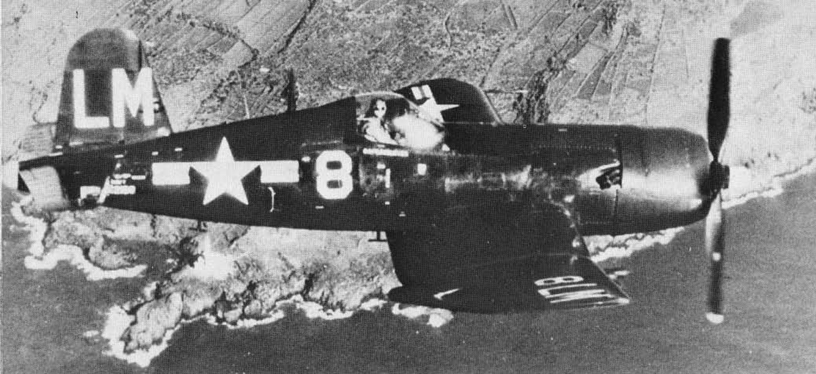
F4U-5P [122168] of VMC-1 flying from the USS Leyte. Note open camera port under the bar in the National insignia, December 1949. [USMC]
