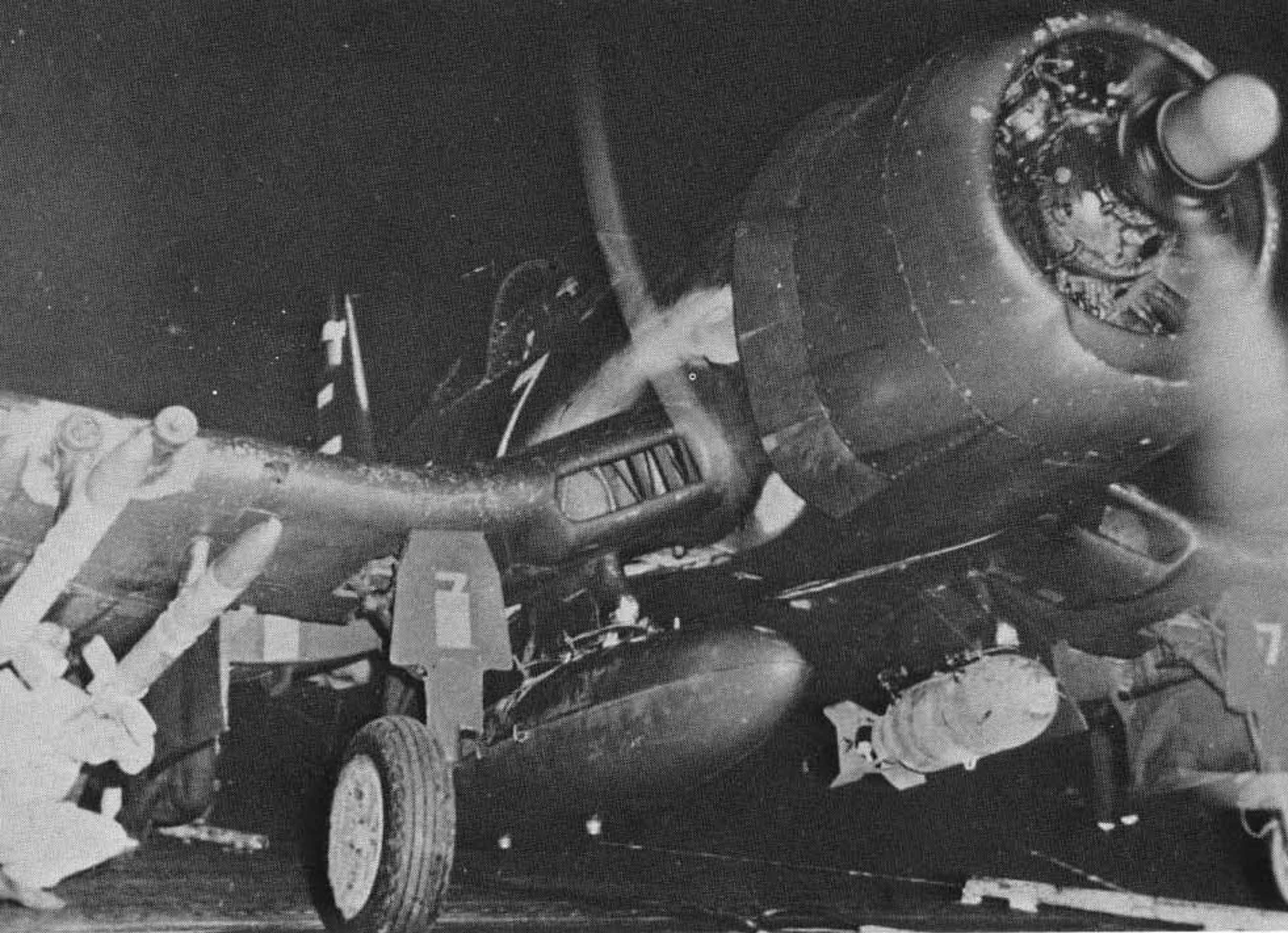
F4U-4B of VMF-214 [Blacksheep] ready for pre-dawn launch for Korean strike. Armament consists of 8-HVARs, 1 500-lb. bomb and a Mk 5 150-gallon drop tank. USS Sicily, December 16, 1950. [USN-Bob Lawson]
