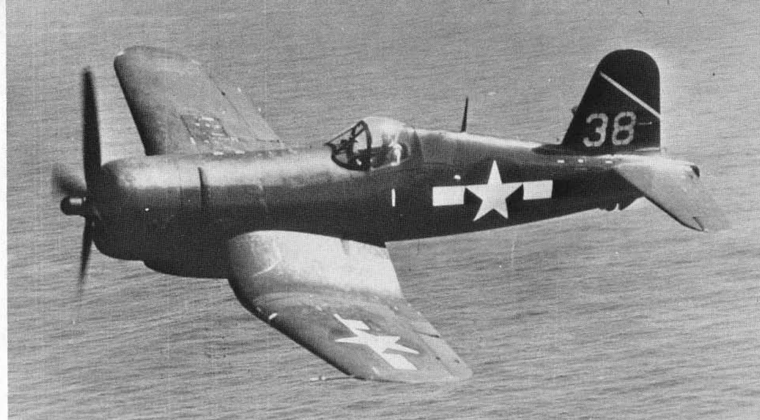
F4U-4 in post-war markings with the new flat bulletproof center-panel windscreen and blown rear canopy for better visibility, March 1, 1945. [National Archives]
