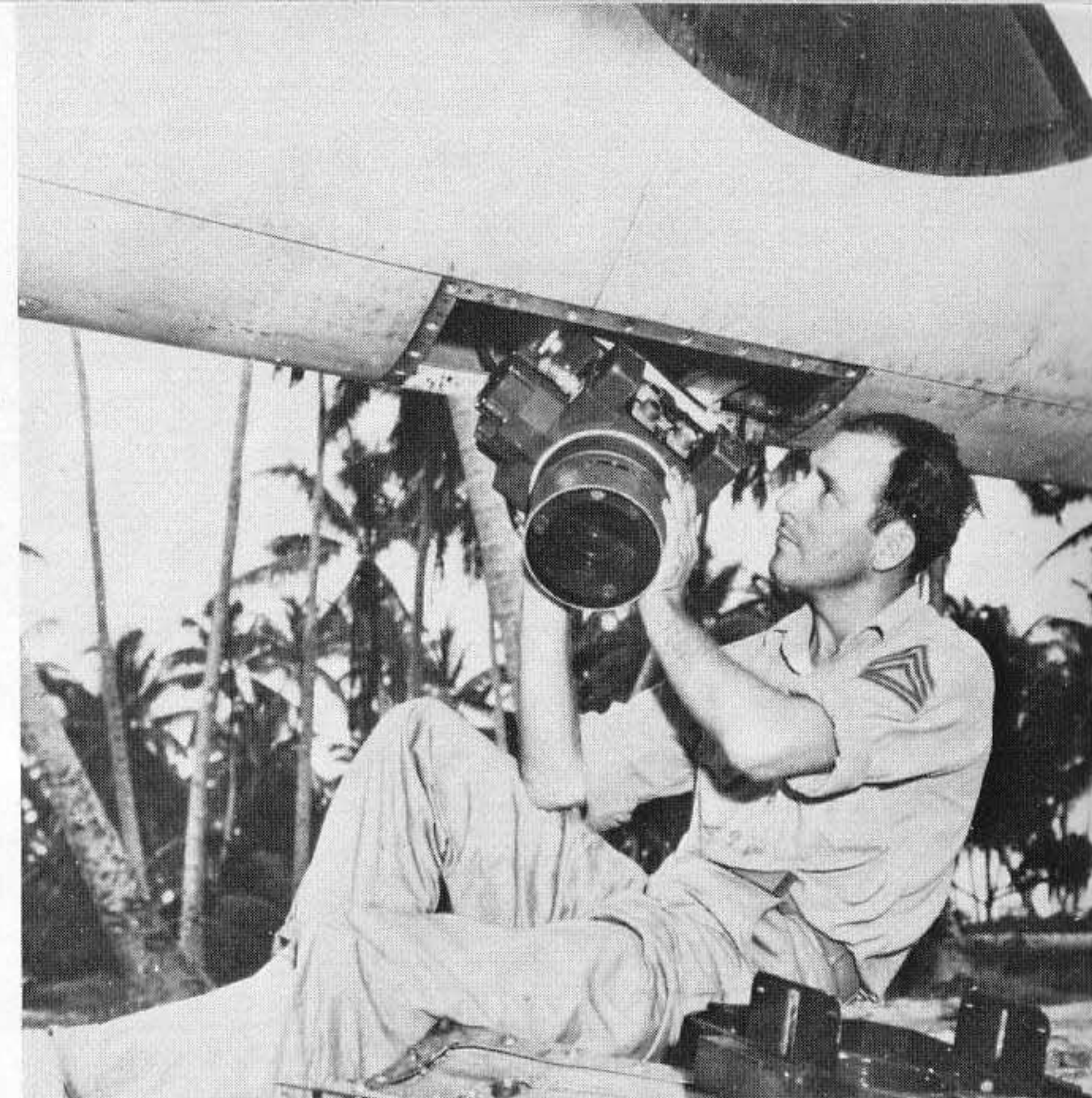
K-21 aerial camera is loaded into F4U-1P photo-fighter of the 4th MAF by T/Sgt. R.F. Melville. The Corsair was used in daily raids on the enemy-held Marshall Island atolls. February 1944. [Vought]
