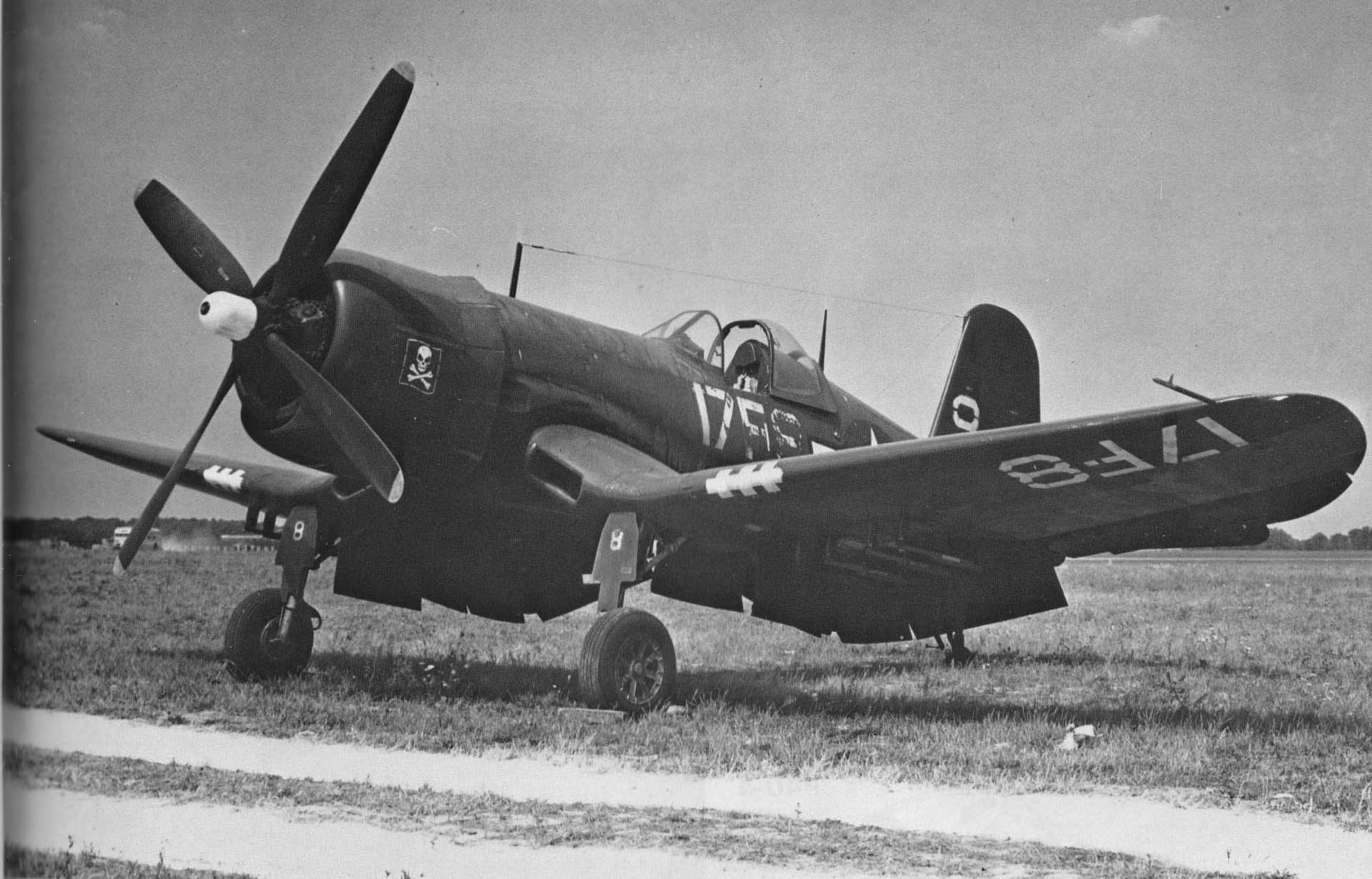
F4U-4 [82125] Stateside still carrying the Skull-and-Crossbones markings of VF-17. Note the gun ports taped over to reduce drag, also the new blown canopy. VF-17 last saw combat in the F4U-1A model. [Robert O'Dell]
