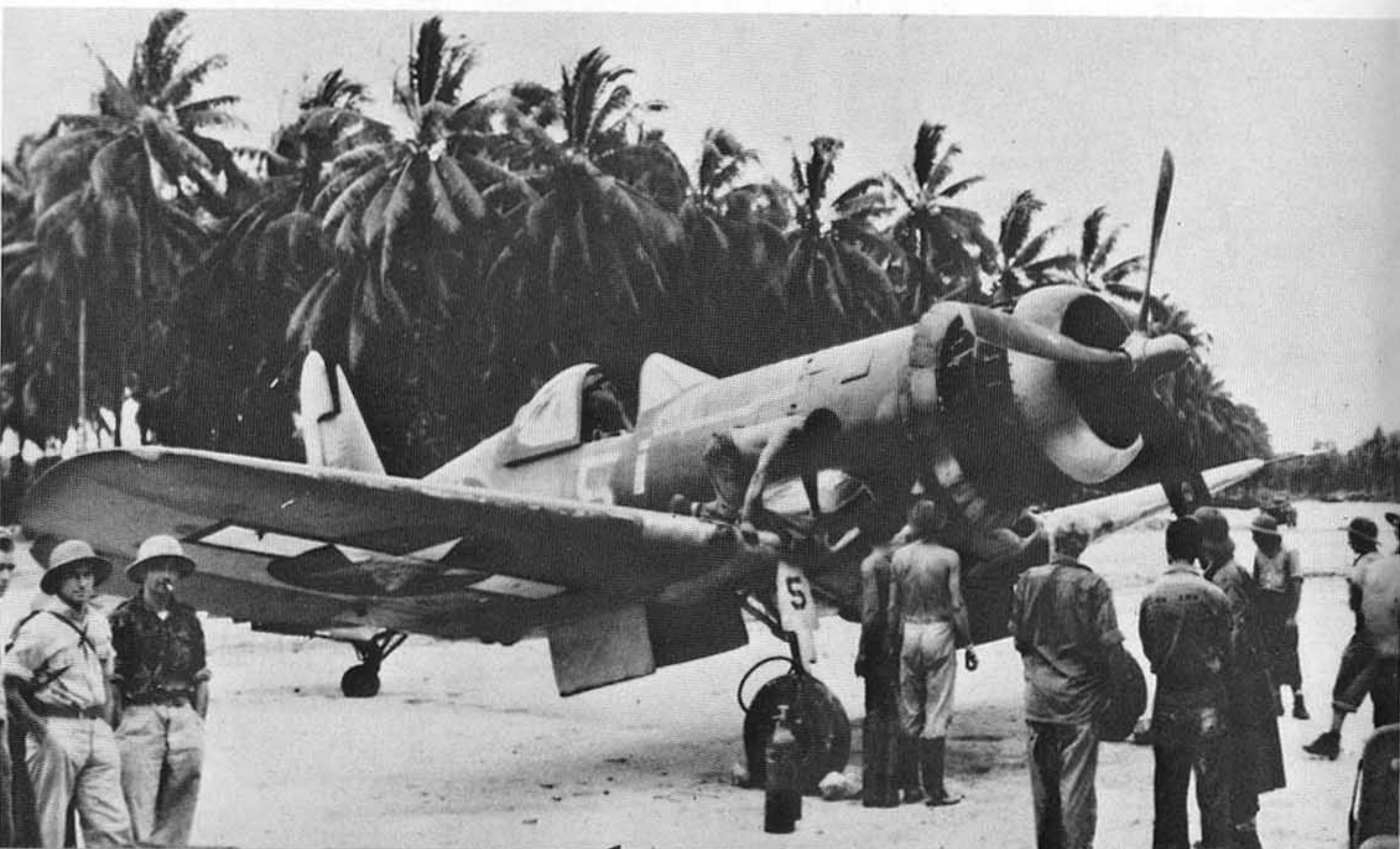
Navy F4U-1A flown by Lt. [JG] Tom Killefer of VF-17 landed dead-stick on Nissan Island in the Green Island group after a complete engine failure. After repairs that night and following day, Killefer flew out. Note 5 kill marks under the cockpit. March 5, 1944. [National Archives]
