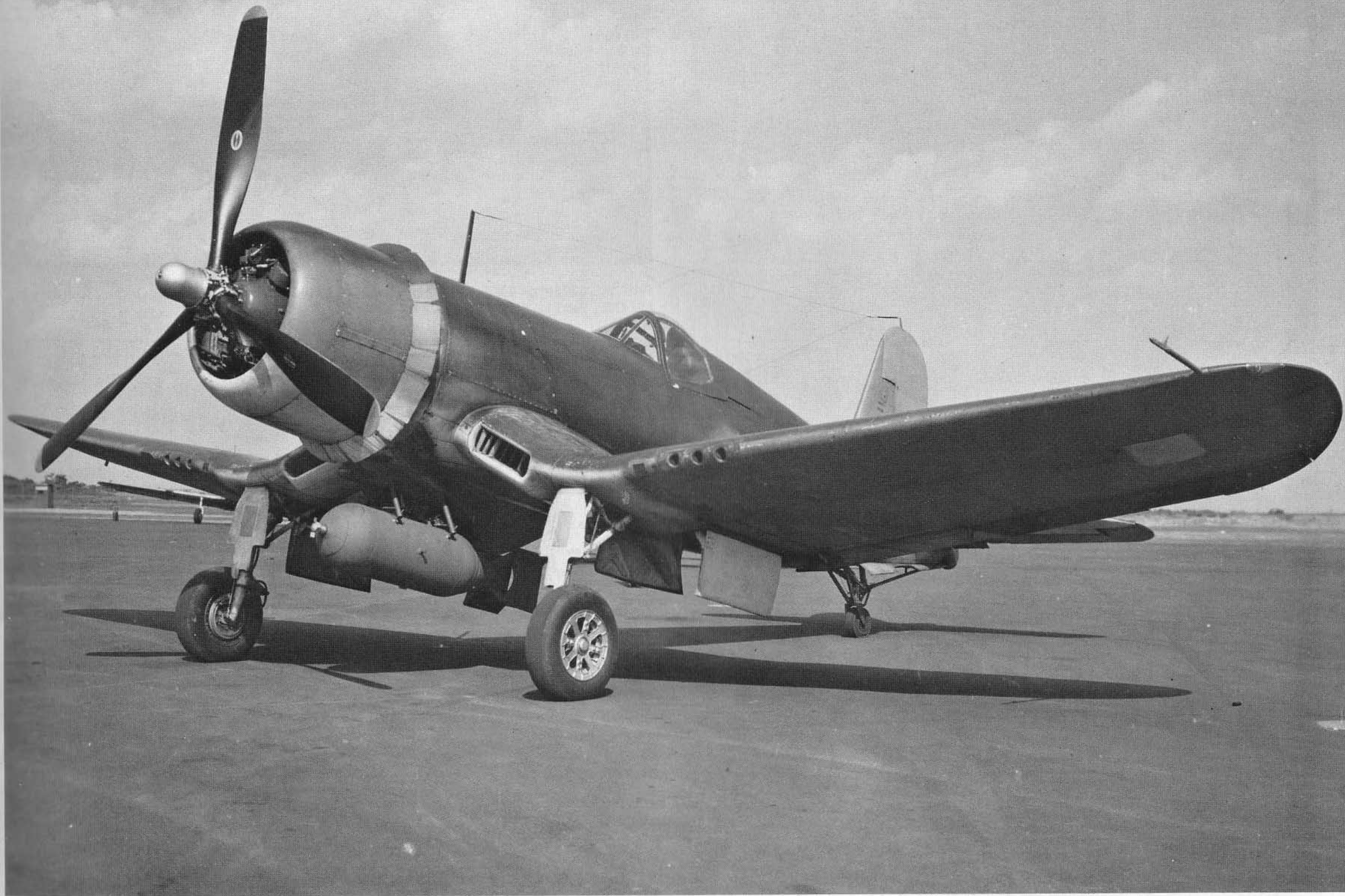
F4U-1A [18026] with a Brewster designed adapter rack securely holds 1000-lb. bomb. Navy and Marine Squadrons used this modification to wreak additional havoc to the already battle-tired Japanese. January 8, 1945. [Vought]
