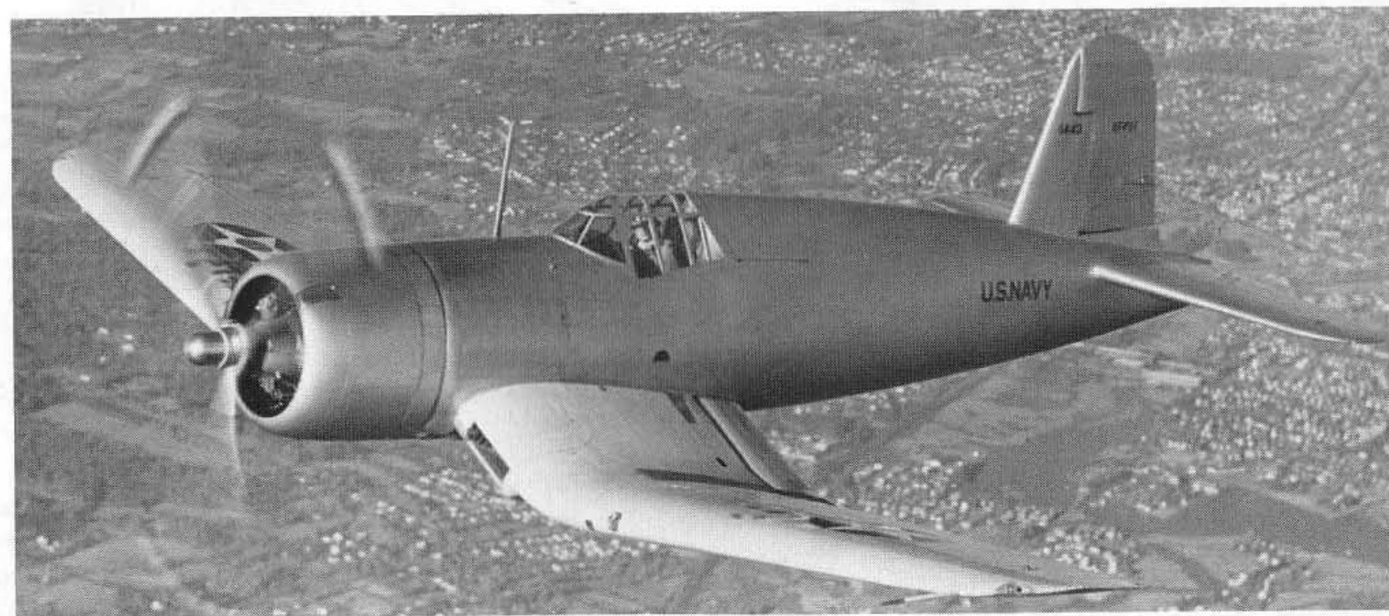
On October 1, 1940 the XF4U-1 set a World's Speed Record of 405 MPH while flying a record attempt between Stratford and Hartford, Conn. At this time, the Corsair was the fastest plane in the world. [Vought]
