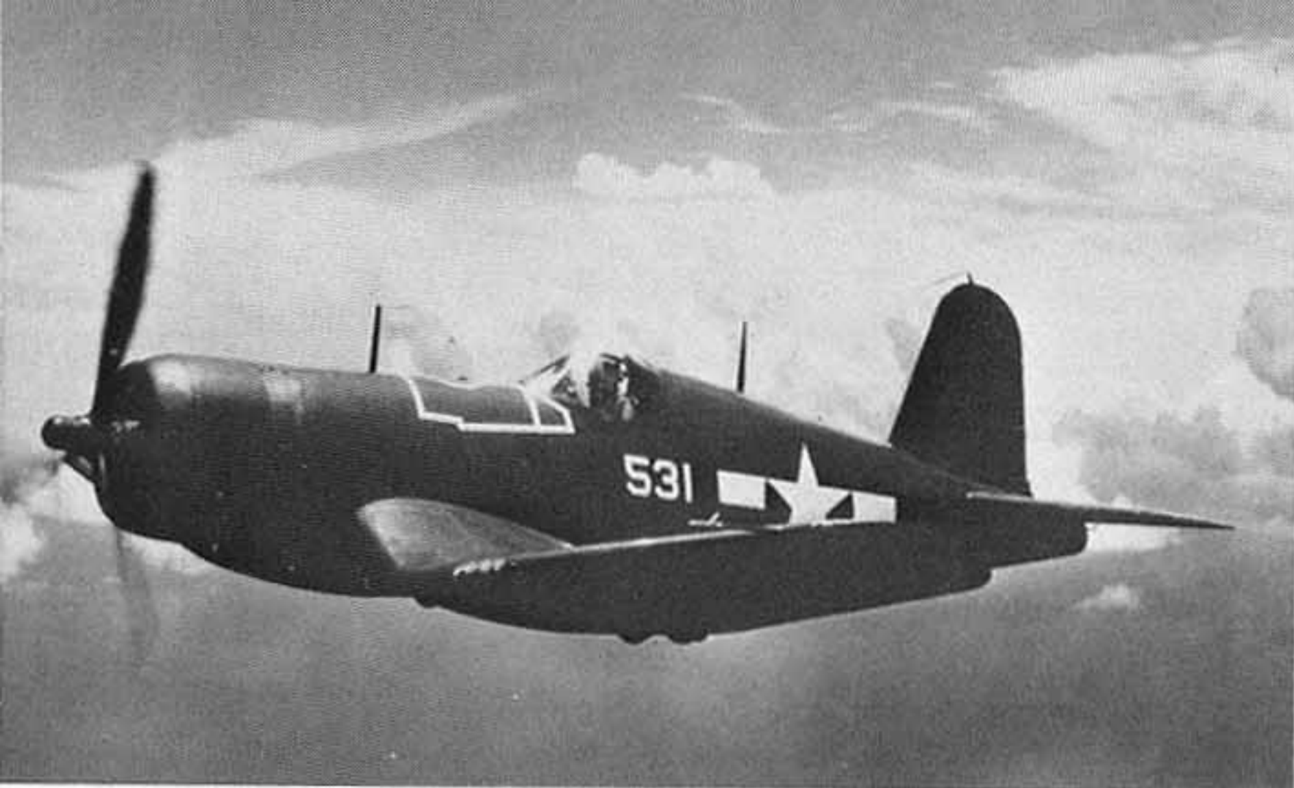
Marine FG-1A #531 displays modified raised cabin section. Problems with fuel cell leaks frequently caused taping of the fuselage skin joint areas just forward of the cockpit. September 1944. [National Archives]
