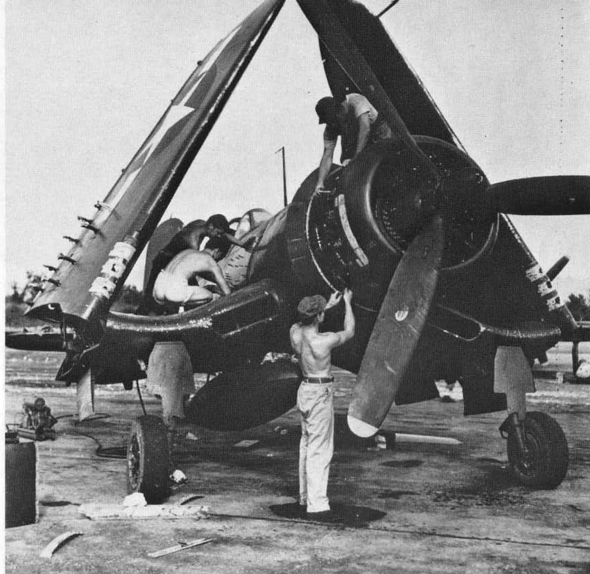
To repair battle damage, a F4U-1D is getting a new plate riveted on by ground crew in a service area in the Gilbert Islands. July 12, 1945. [National Archives]
