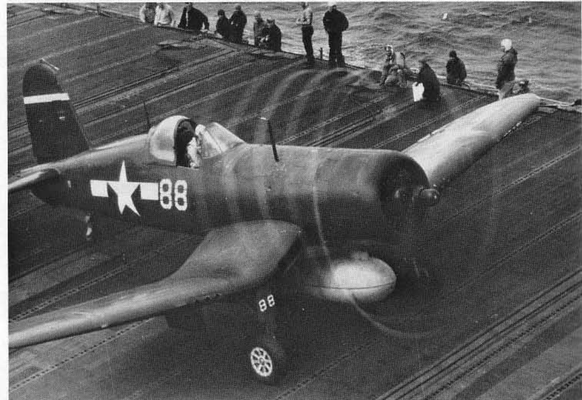
Marine F4U-1D of VMF-124/213 creates vortex on his take off roll. Finally cleared for Carrier operations, Corsairs make up for lost time in their strikes against Japanese targets. USS Essex, January 25, 1945. [National Archives]
