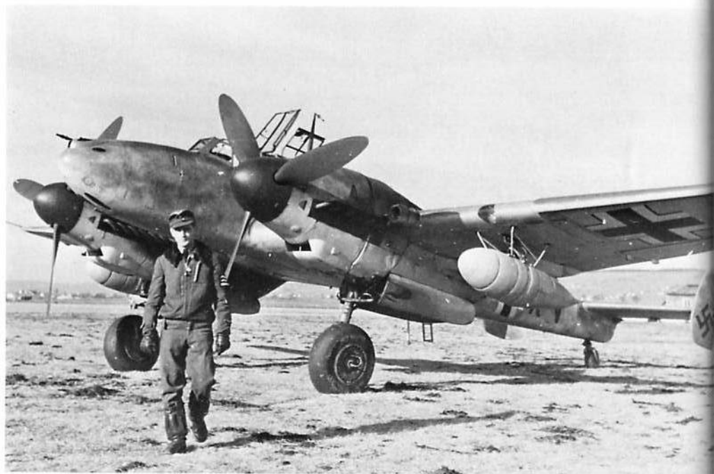
The Bf 110G-2 began leaving assembly lines during May 1942 and could be utilized as either a Zerstörer or heavy fighter bomber through the application of various Rüstsätze. [Bundesarchiv]
