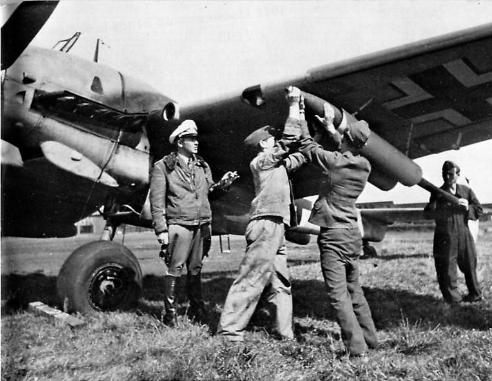
When the Wfr. Gr. 21 rocket launching tubes were carried on the Bf 110G-2/R3, the twin Mk 108 cannon were removed but in order to not lose fire power the interchangeable ETC 500 bomb carriers were replaced by the twin MG 151 cannon tray. [Bundesarchiv]
