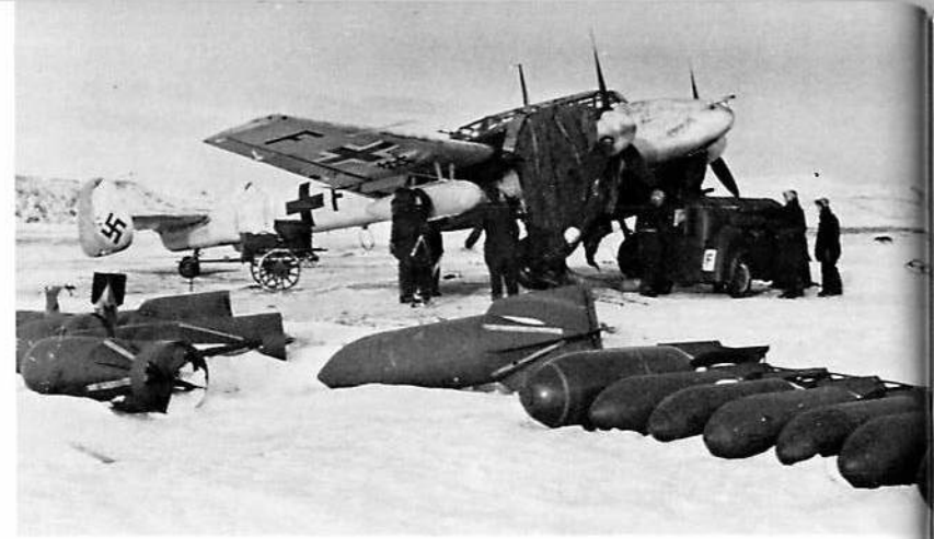
Flying under the most adverse winter conditions 7.[Z]/JG 5 learned to keep their aircraft serviceable despite the bitter cold. Of note are the presence of ETC 50 bomb racks at the same time the machine is carrying 66 Imp. gal. auxiliary fuel tanks. [Bundesarchiv]
