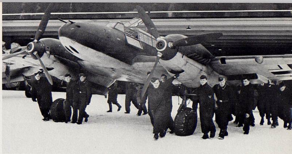
The initial production Bf 110C-1s were delivered to I(Z)/LG 1 at Greifswald during January, 1939. The C-1 series standardized on the new UDM three-bladed, controllable, full-feathering prop. [Bundesarchiv]
