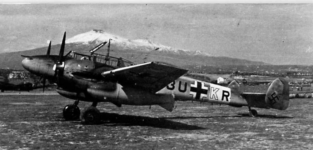
This Bf 110D-3 of 7./ZG 26 carrying the long range 198 Imp. gal. drop tanks sits on a Sicilian airfield after escorting Ju 52s returning from Africa. The very clearly seen "N" on the outboard nacelle denoted that the machine was powered by DB 601N engines and was to be fueled with 96 octane C3 fuel. [Bundesarchiv]
