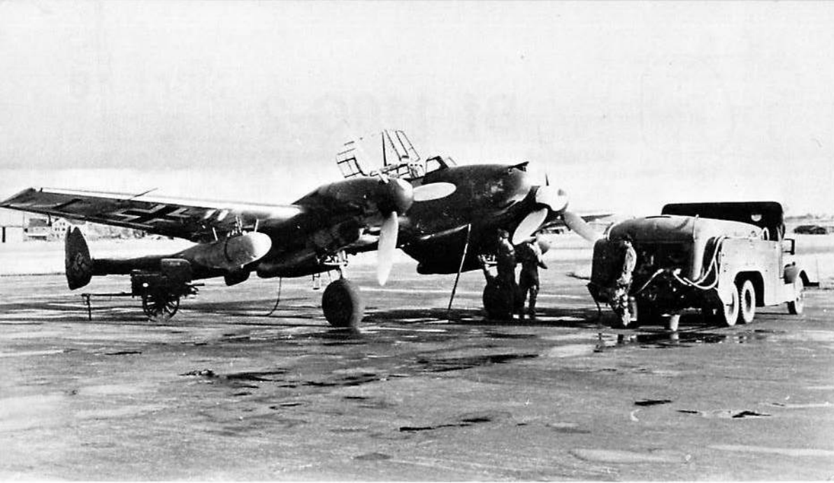
Flying under the most adverse winter conditions 7.[Z]/JG 5 learned to keep their aircraft serviceable despite the bitter cold. Of note are the presence of ETC 50 bomb racks at the same time the machine is carrying 66 Imp. gal. auxiliary fuel tanks. [Bundesarchiv]
