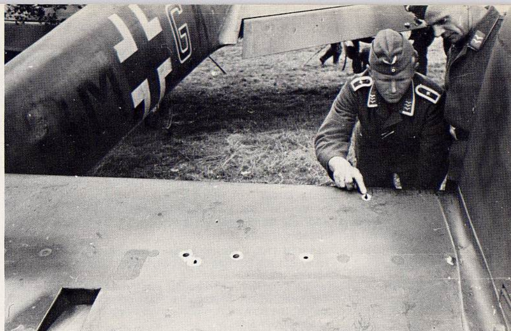
These air frame mechanics are examining the tail assembly after it has taken hits from ground fire. Previously repaired damage can be seen on the rudder. Damage such as this usually caused few problems and could often times be repaired within an hour. [Bundesarchiv]
