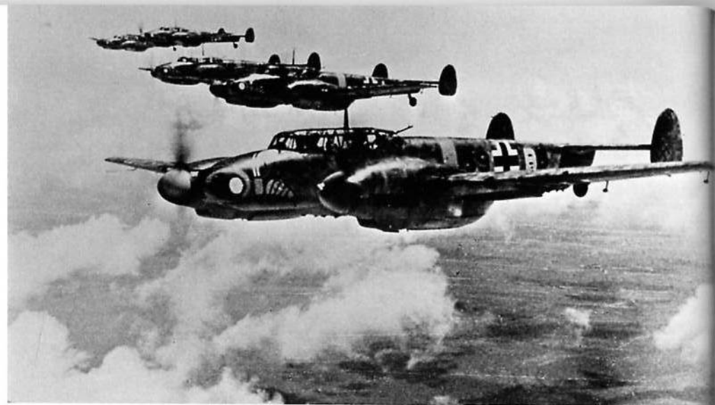
Early Bf 110G-2s of Stab I/SKG 210 over Russia during July 1942. Note the retention of the early vertical tail surfaces and the single rear firing MG 15. It is possible that these are pre-production G-0s. [Bundesarchiv]
