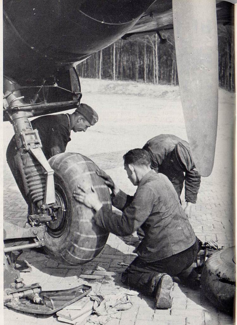
A special hydraulic jack was provided that fit under the landing gear oleo lifting the aircraft free of the ground allowing the "black ones" to easily replace a worn or damaged tire. [Bundesarchiv]
