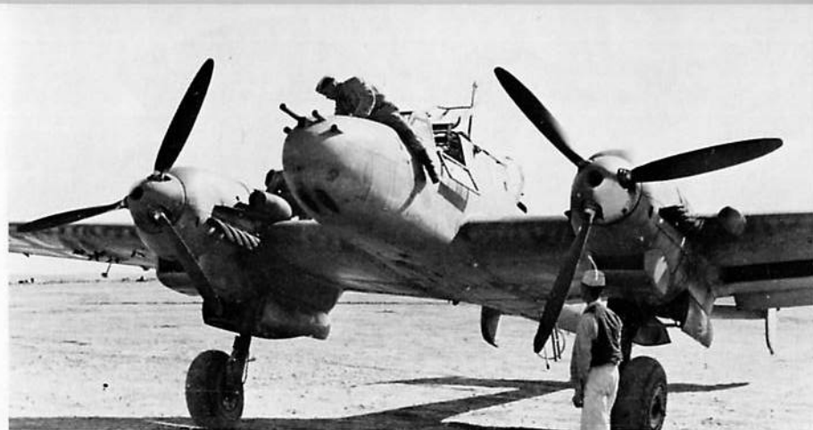
During the spring and summer of 1942, the new Bf 110F-2 Zerstörer began to arrive in the Western Desert. The increased performance of the F series was a welcome addition to the Luftwaffe, who were supporting Rommel's Drive to El Alamein. This Bf 110F-2 Zerstörer belonging to ZG 26 carries the tropical dust filters and two ETC 50 bomb racks under each wing. [Bundesarchiv]
