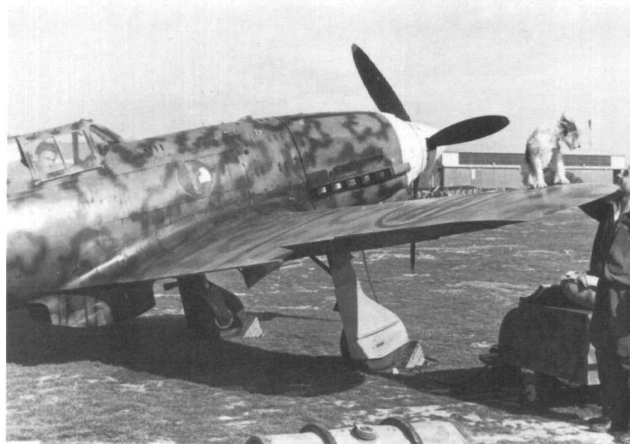
This Folgore of 151° Gruppo in Tunisia retains its desert marking of white nose and spinner. It has the later style windscreen with armor glass and supplementary cockpit air scoop but has the venturi tube beneath the fuselage.
