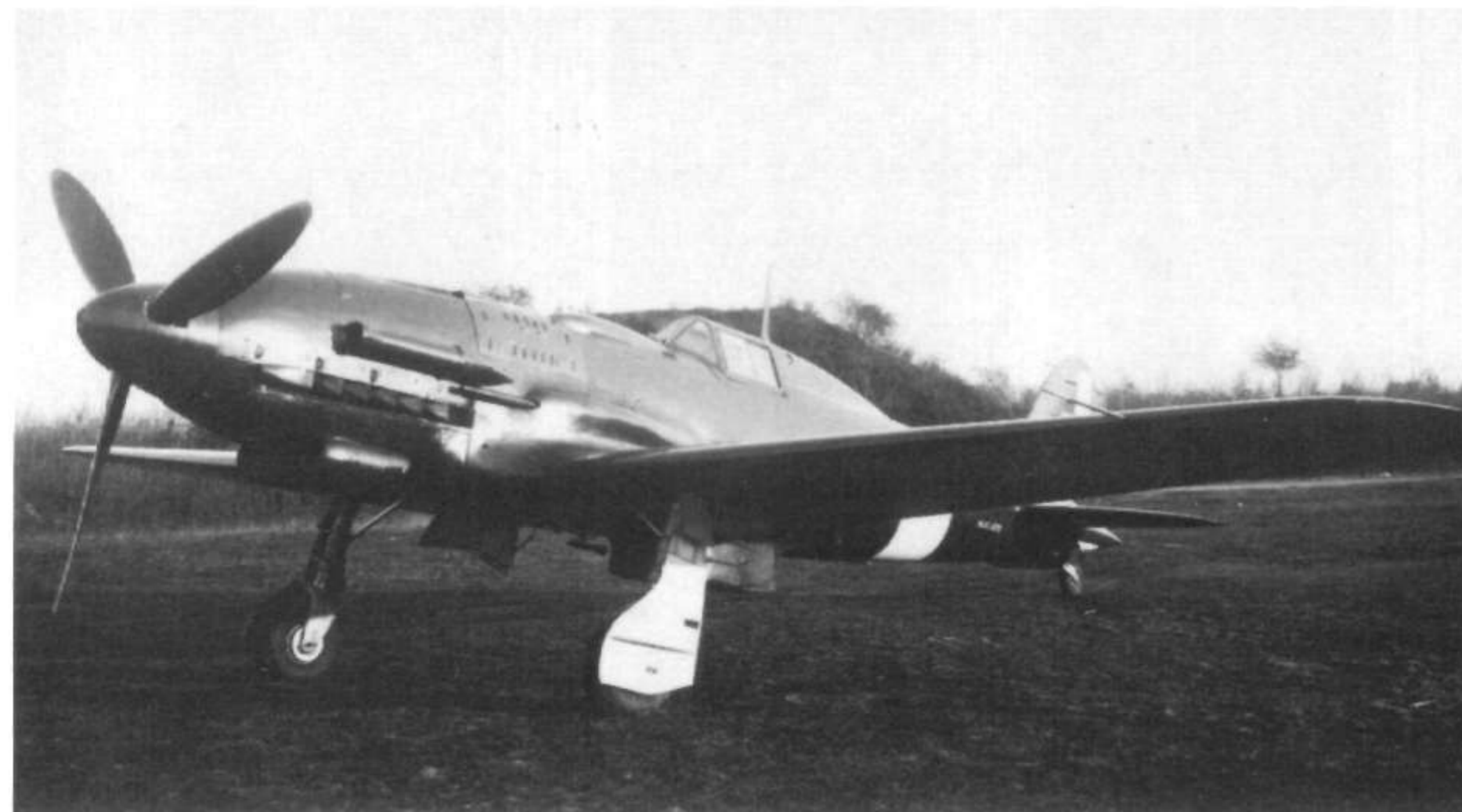
The first C.205N Orione (Orion) prototype, M.M.499. The armament was a single 20mm cannon firing through the propeller hub and four 12.7mm MGs, two in the cowl and two above the wing roots.
