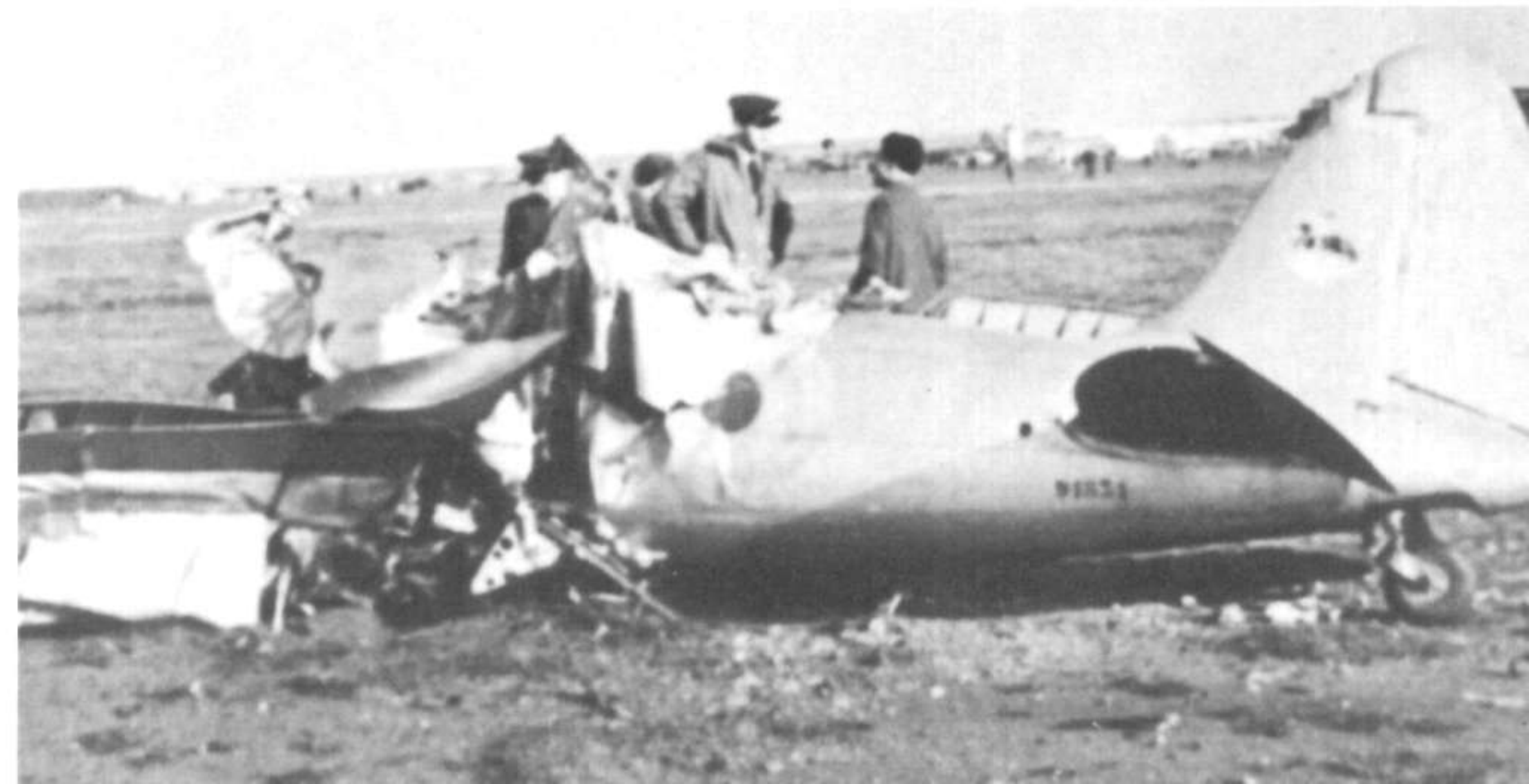
(Below & Below Left) Rebuilt from parts by 8° Gruppo mechanics, with a DB605 engine, but retaining the Folgore oil cooler, this C.205 was left unpainted and was called 'Biancone' (Whitey). It came to its unhappy end when a novice pilot spun it into the ground. That this Veltro is a rebuild can also be ascertained from the non-retracting tailwheel.
