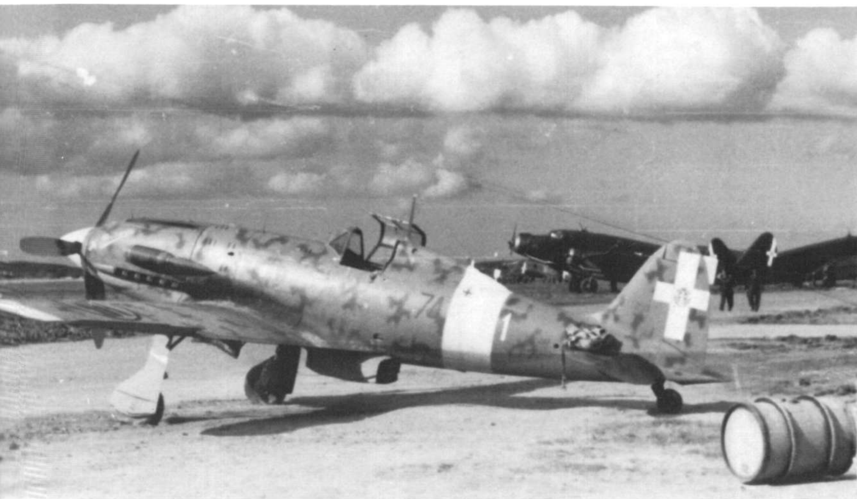
This Folgore of 151° Gruppo in Tunisia retains its desert marking of white nose and spinner. It has the later style windscreen with armor glass and supplementary cockpit air scoop but has the venturi tube beneath the fuselage.
