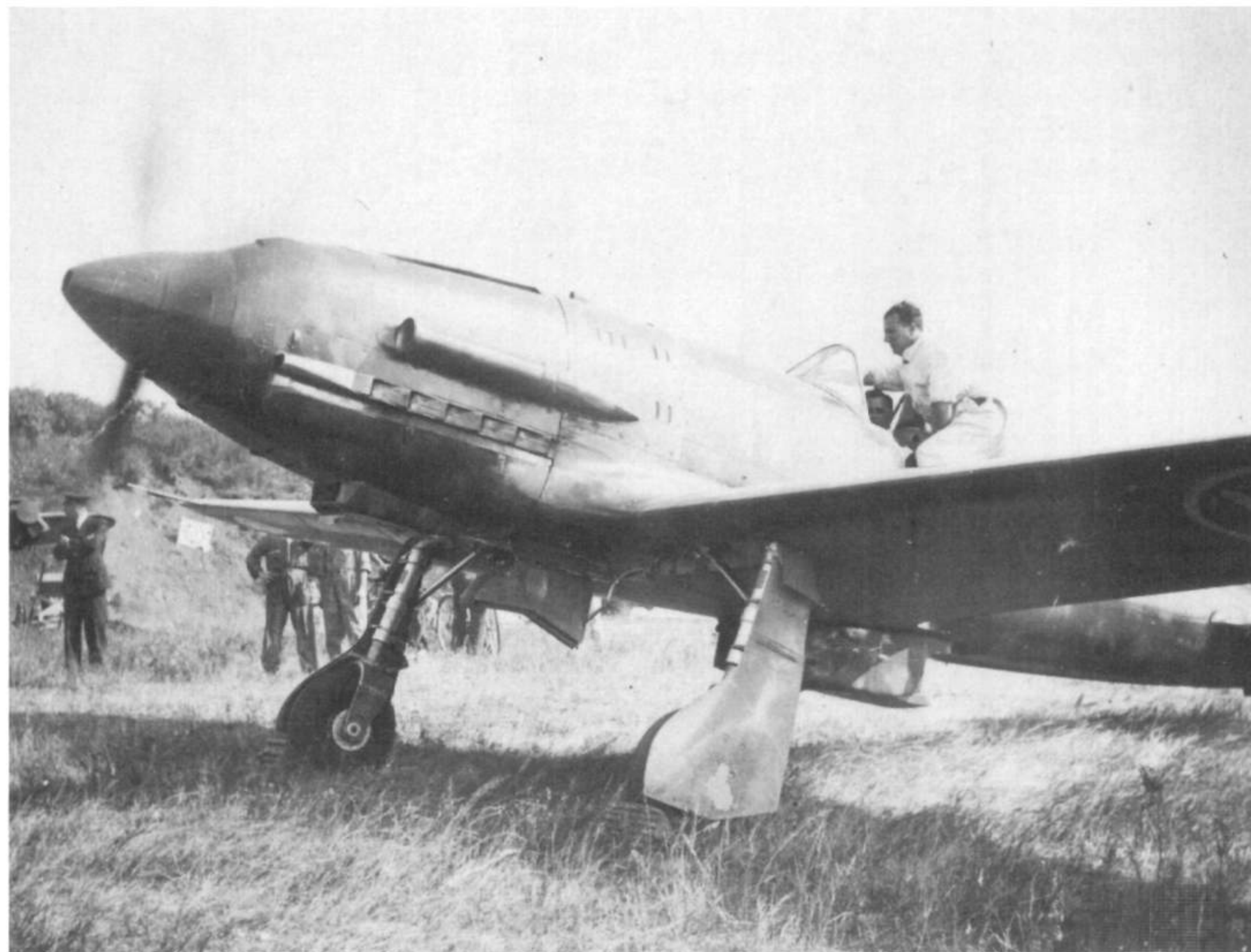
(Above & Below) The prototype in its final form, with long, circular-section supercharger intake and sporting a brown, green and sand dapple camouflage. The fasces insignia on its wings are black and white, the colors reversed on the upper and lower surfaces. In the photo below, the engine is being warmed up. In the cockpit is Comm. Guido Carestiato, Macchi's chief test pilot.
