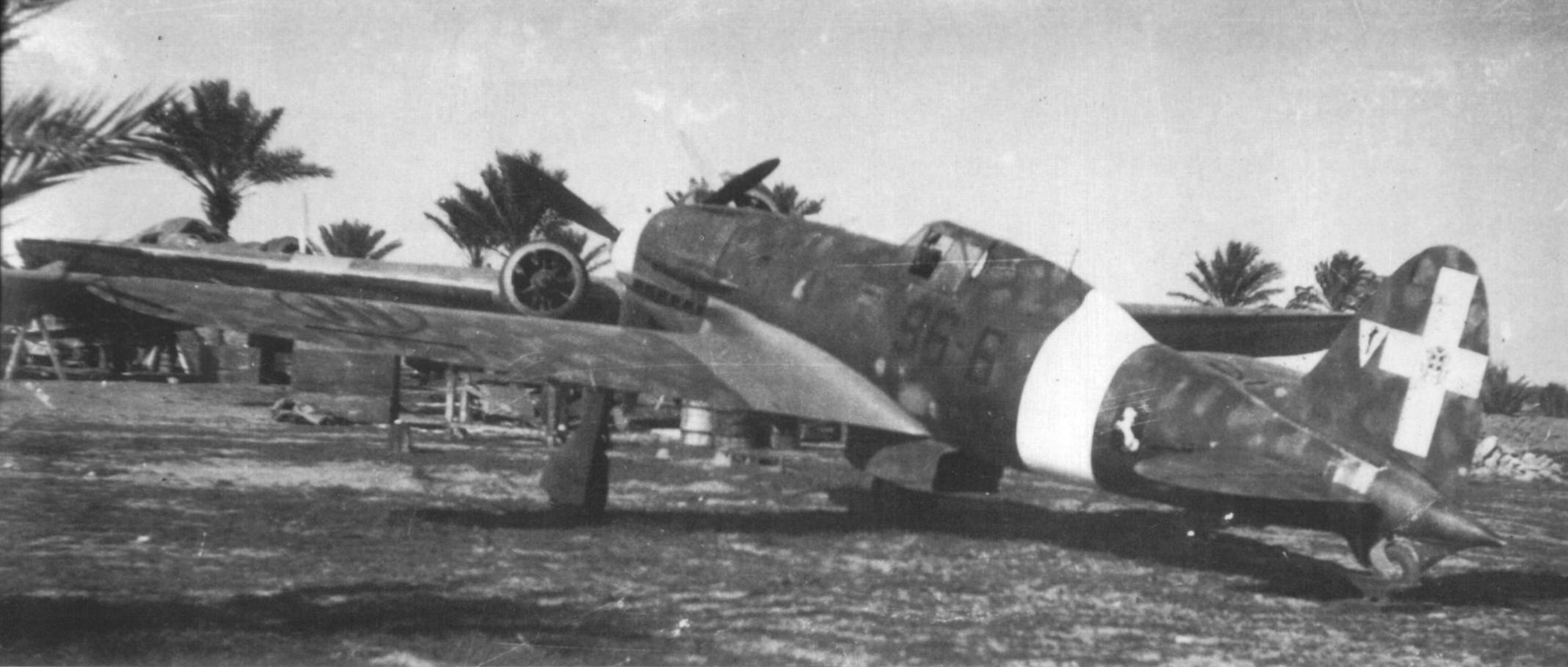
(Above & Left) C.202 96-6, now sporting a white spinner and nose, shows gloss gray paint over repairs at the wingroot and on the fuselage, resulting from damage acquired in the air over Malta. Note the stub radio mast, characteristic of early Folgore s.
