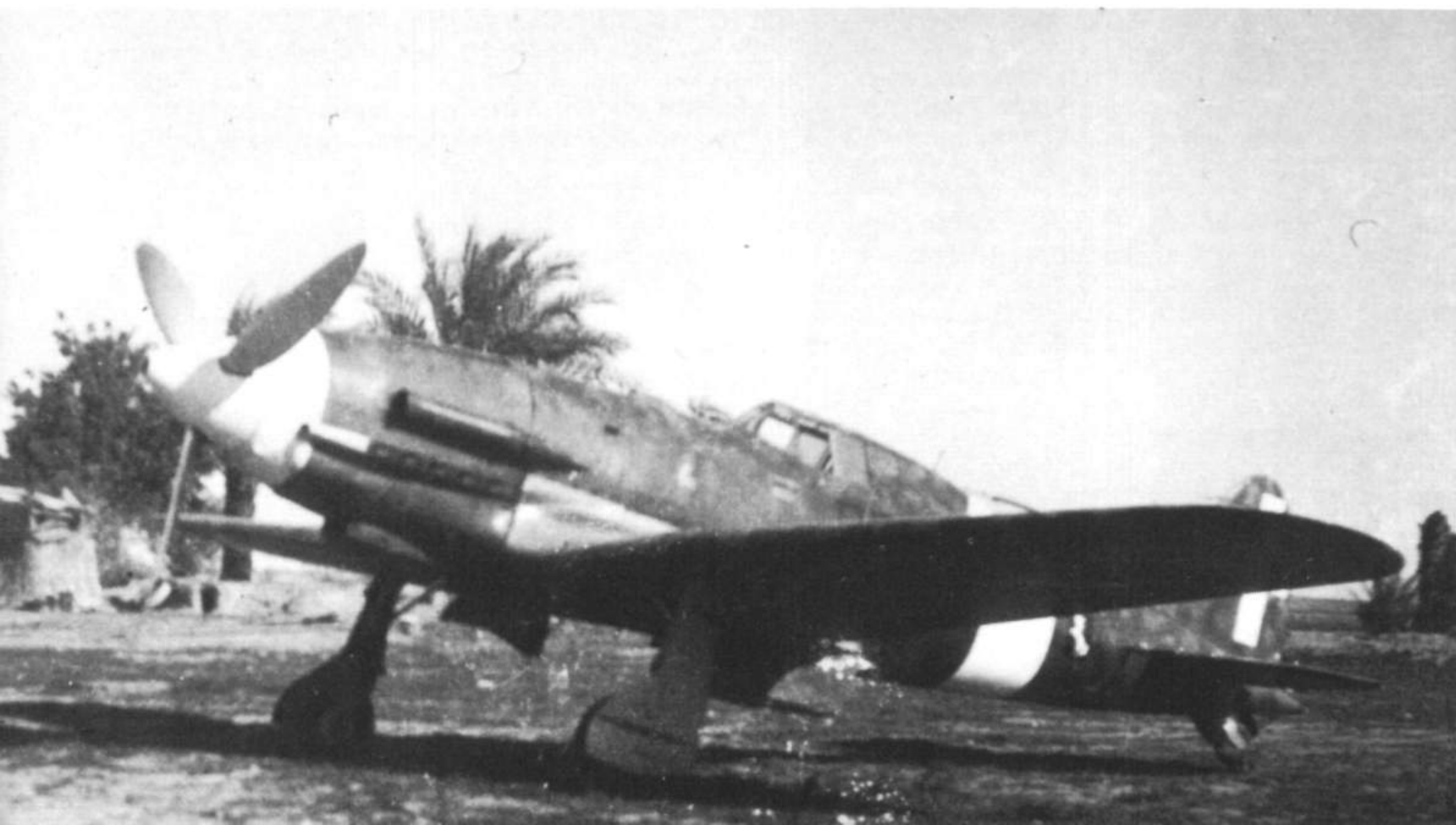
(Above & Left) C.202 96-6, now sporting a white spinner and nose, shows gloss gray paint over repairs at the wingroot and on the fuselage, resulting from damage acquired in the air over Malta. Note the stub radio mast, characteristic of early Folgore s.
