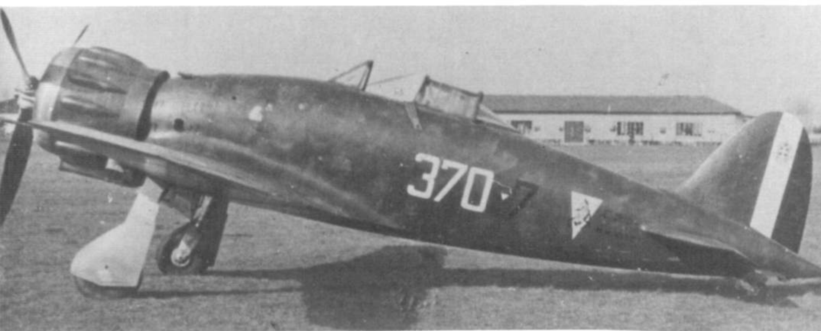
The sole C.202 prototype, M.M.445, as it first appeared, overall natural metal except for the pre-war green, white, red tail stripes. The short supercharger intake was later changed in shape and length. The windows set into the headrest 'hump' and the retracting tailwheel were deleted from production Folgores .
