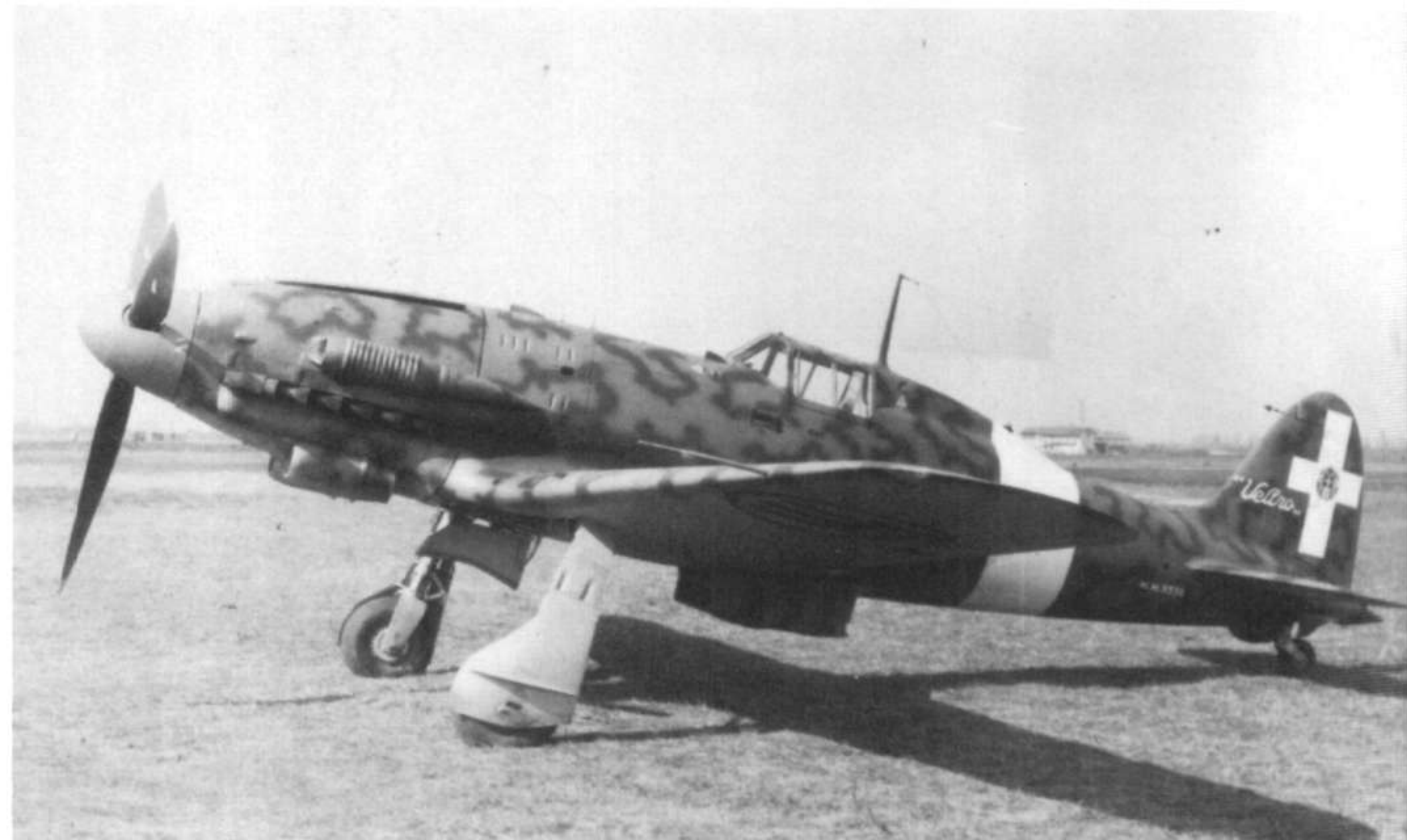
A Serie I Veltro , M.M.9338, with late-style C.202 armament, two cowl-mounted 12.7mms and two wing 7.7s. The name on the tail was to remind the reluctant pilots of the 'official' nickname.
