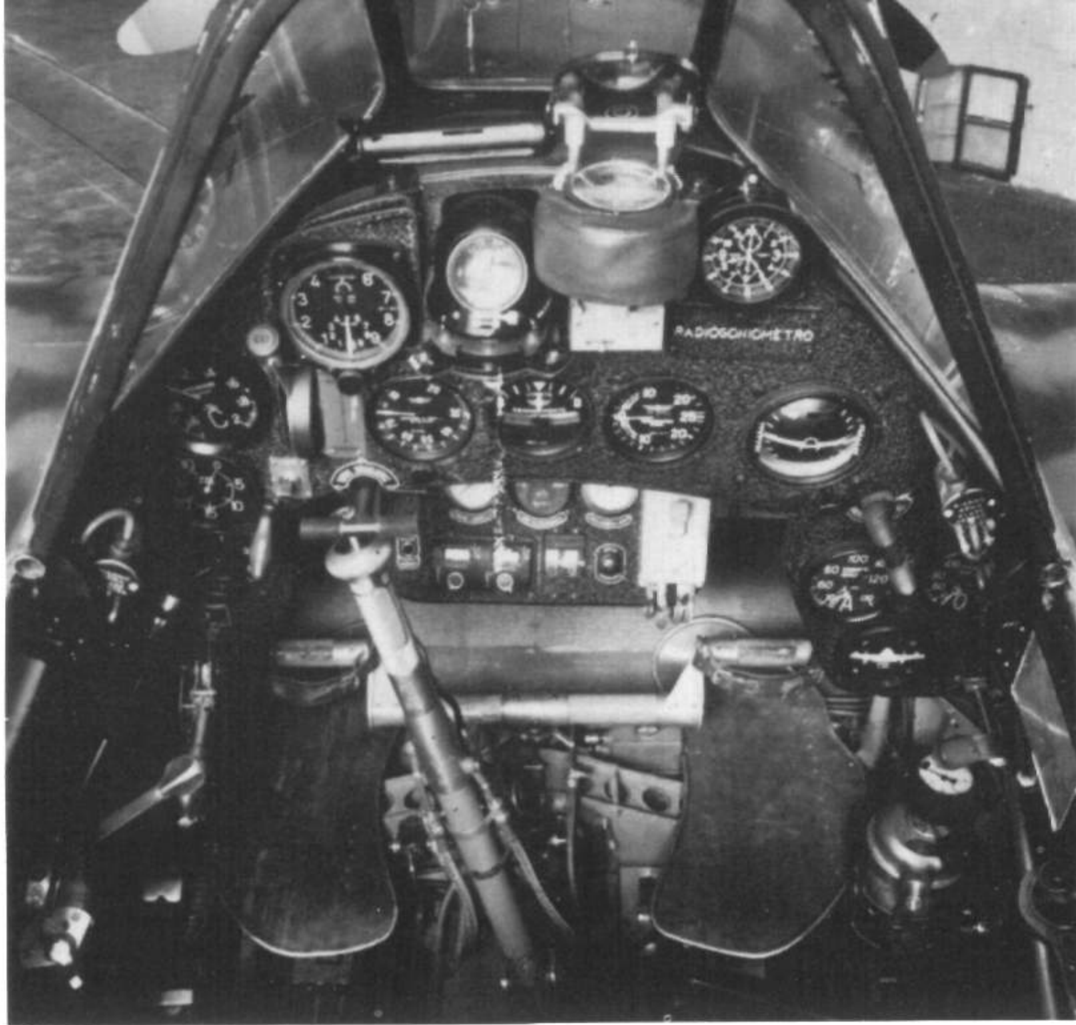
(Left) C.202 instrument panel, with reflector gunsight. This is a later variant as it has recharging handles for the wing guns. (Above) Left side of cockpit, showing oxygen bottle behind the seat position (the seat itself has been removed), tailplane trim wheel, sand filter control, throttle (which on Italian aircraft was pulled to open), flap and landing gear controls. This is an early model without pilot armor. (Below) Right side of cockpit, primarily devoted to fuse boxes. This is a later model with head and 'kidney' armor.
