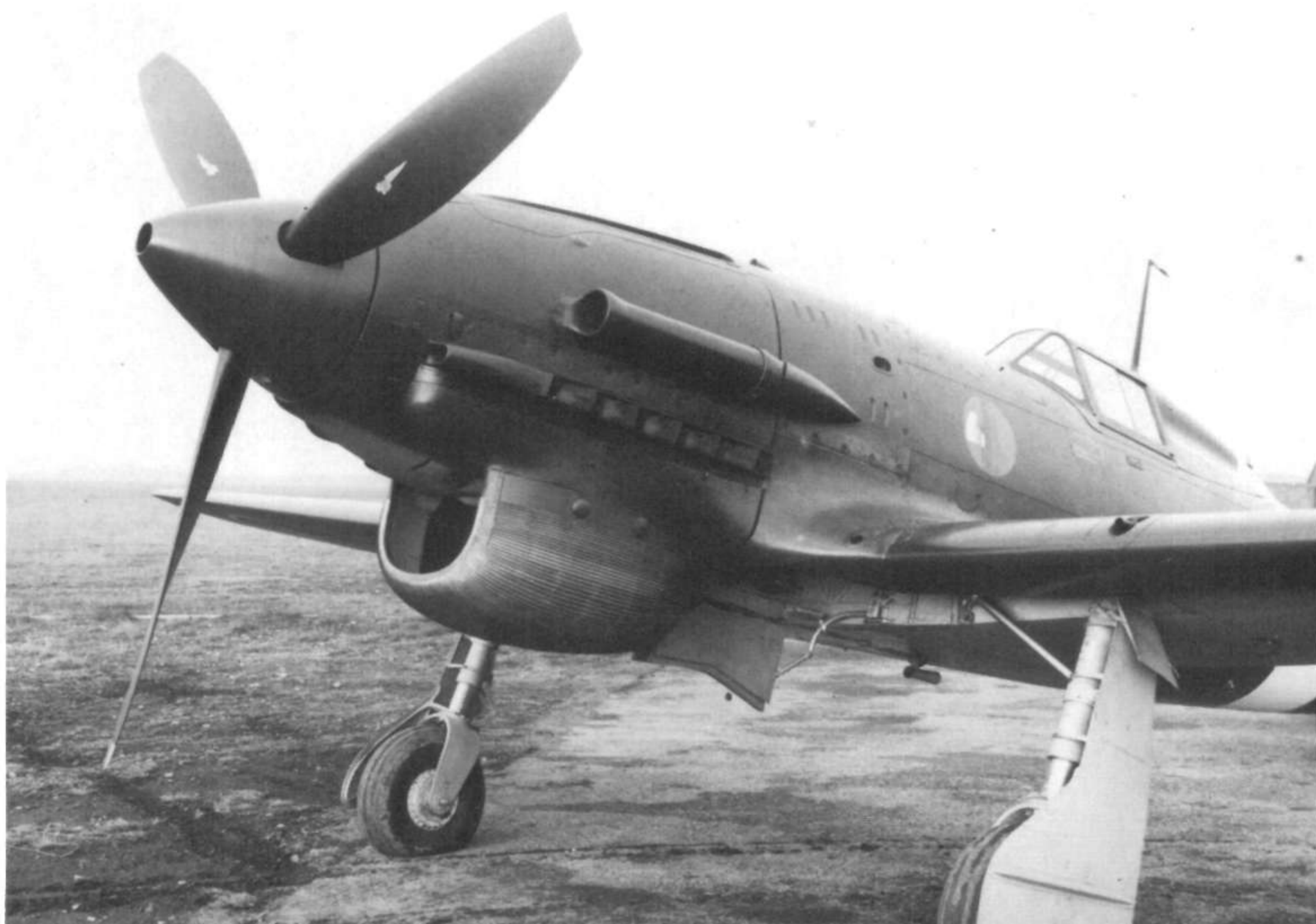
(Above and Left) The sole Macchi C.202D, M.M.7768, as fitted with a chin radiator. The improvement in performance was marginal, not justifying an interruption of the assembly lines.
