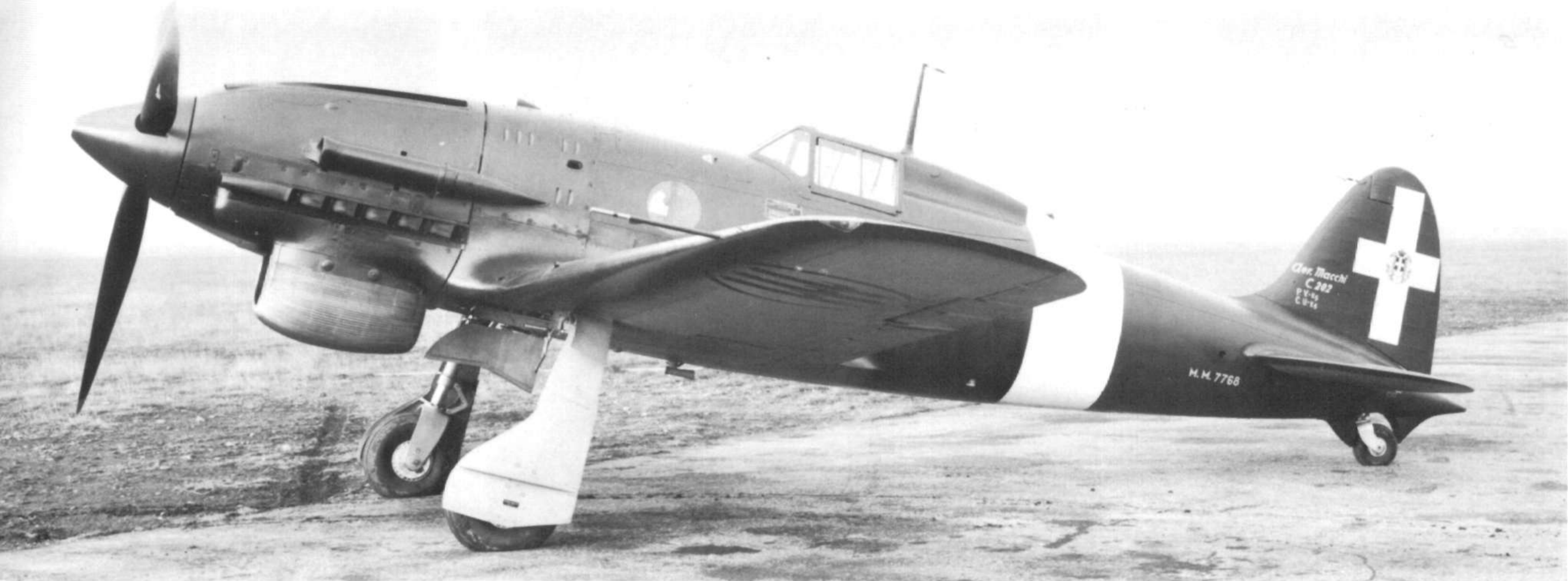
(Above and Left) The sole Macchi C.202D, M.M.7768, as fitted with a chin radiator. The improvement in performance was marginal, not justifying an interruption of the assembly lines.
