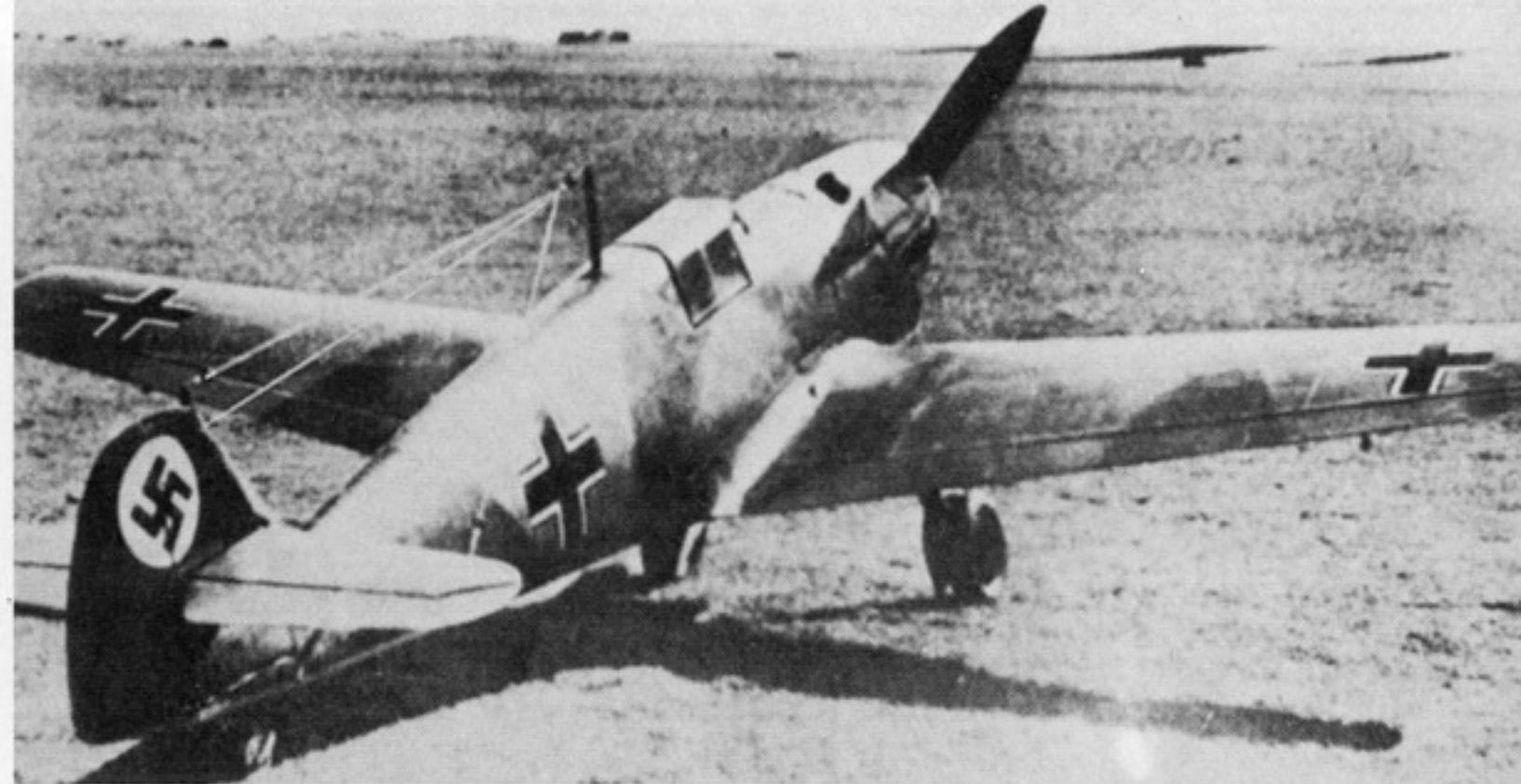
The initial B-1s carried a three wire radio antenna clearly seen on this early B-1, this was quickly changed to a single wire configuration.
