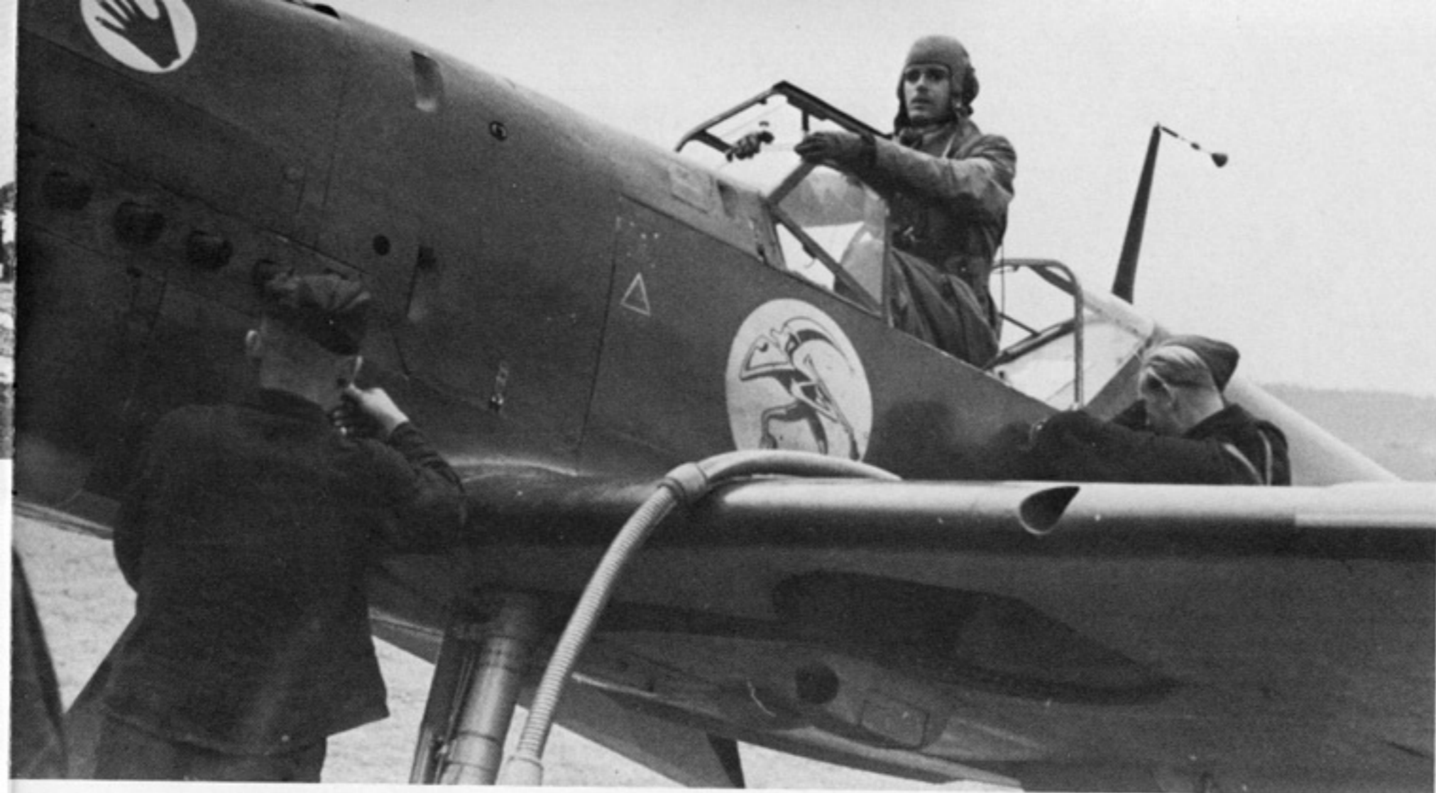
The short barreled MG 17s buried in the wings provided much needed additional firepower since the engine-mounted cannon had proven unsatisfactory. The small oil cooler mounted under the port wing can also be seen to advantage. (Bundesarchiv)
