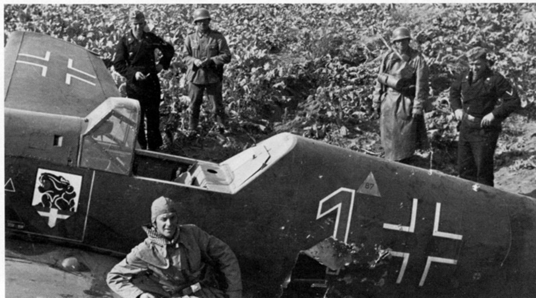
(Above Right) This E-1 of JG 21 that bellied in, seems to have some damage near the oil reserve tank. The prop was turning as the pilot touched down as evidenced by the bent blades. The pilot, being able to bring the machine back to an airfield, meant that the aircraft could usually be made airworthy in a few days. (Obert)
