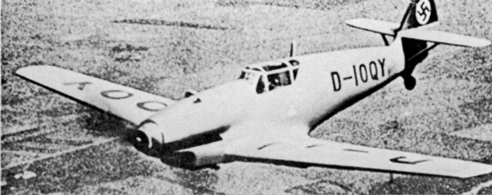
The Bf 109V3 (D-10QY), was the third prototype and mounted three MG 17s, one of which fired through the specially designed cropped spinner. Painted overall RLM Gray, the tail band was red and codes were in black.
