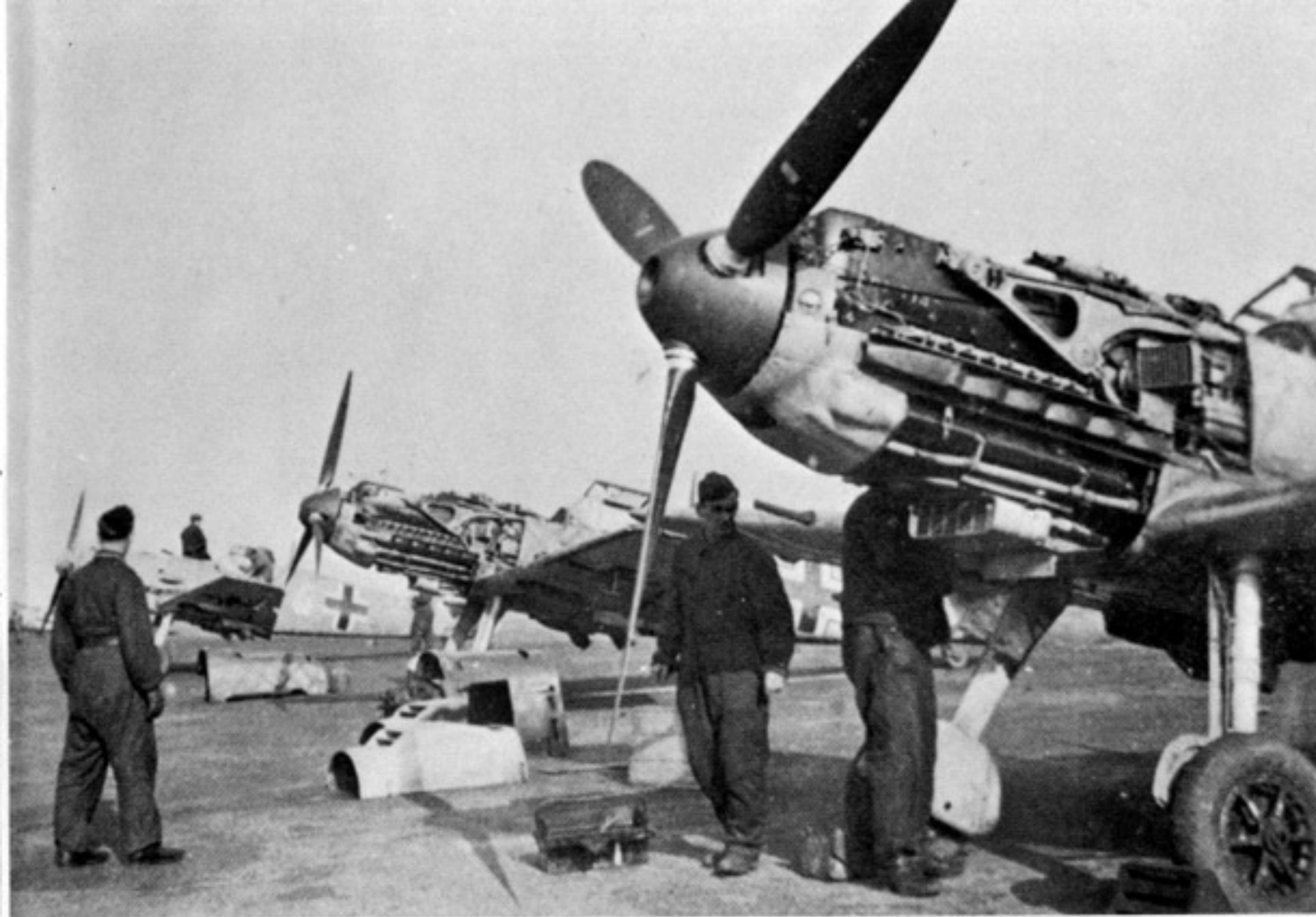
Emils of II(Schlacht)LG 2 at Calais-Marck are being bombed up for a mission across the Channel. The first and third machines are E-4/Bs, while the middle machine is an E-1 which has been retrofitted with a bomb rack, becoming an E-1/B. (Barlow)
