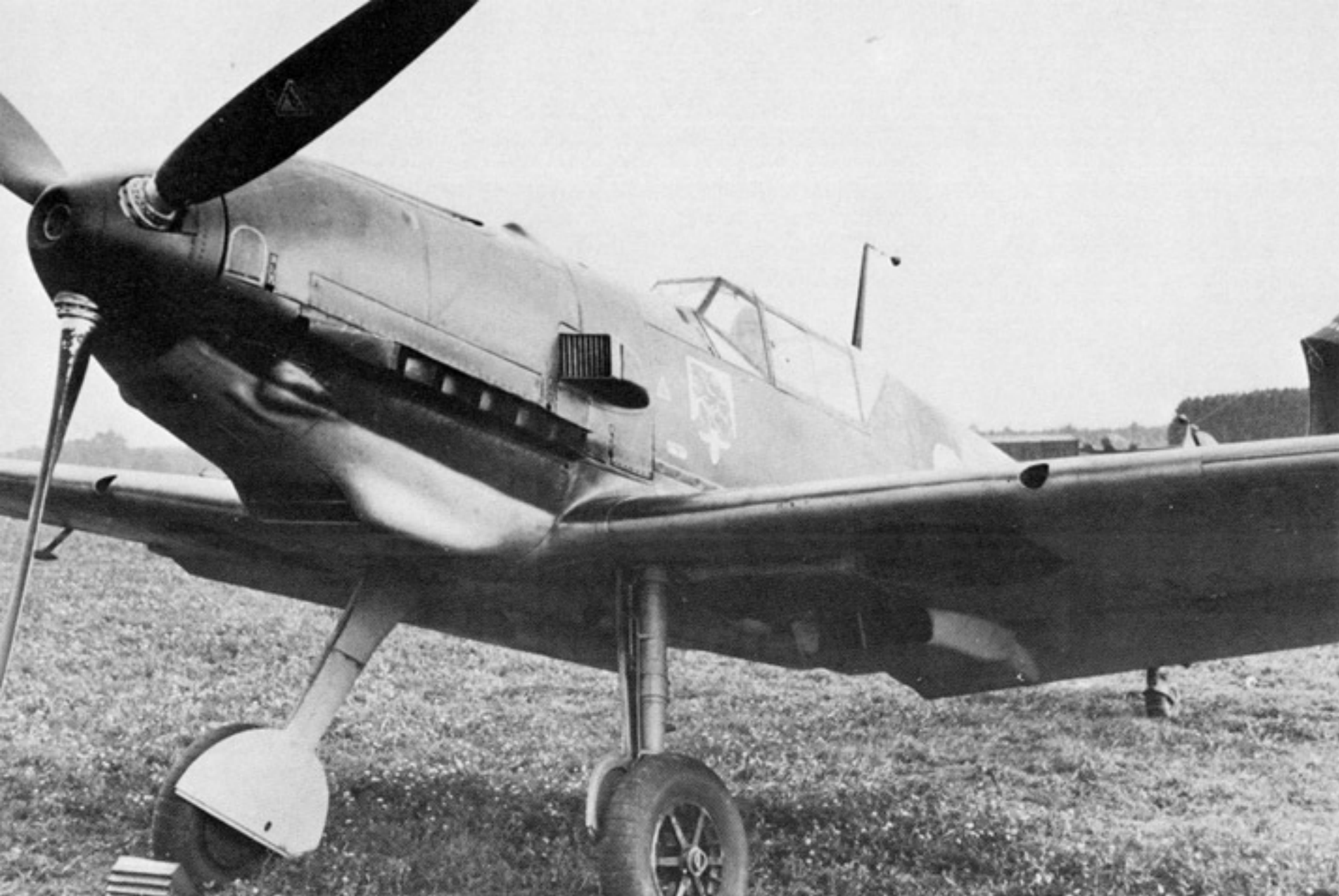
The Bf 109E-1 featured a completely redesigned and much more aerodynamically streamlined lower cowling. The single large radiator bath under the engine was supplanted by two small glycol radiators under the wings and the small underwing oil cooler was moved under the engine. (Bundesarchiv)
