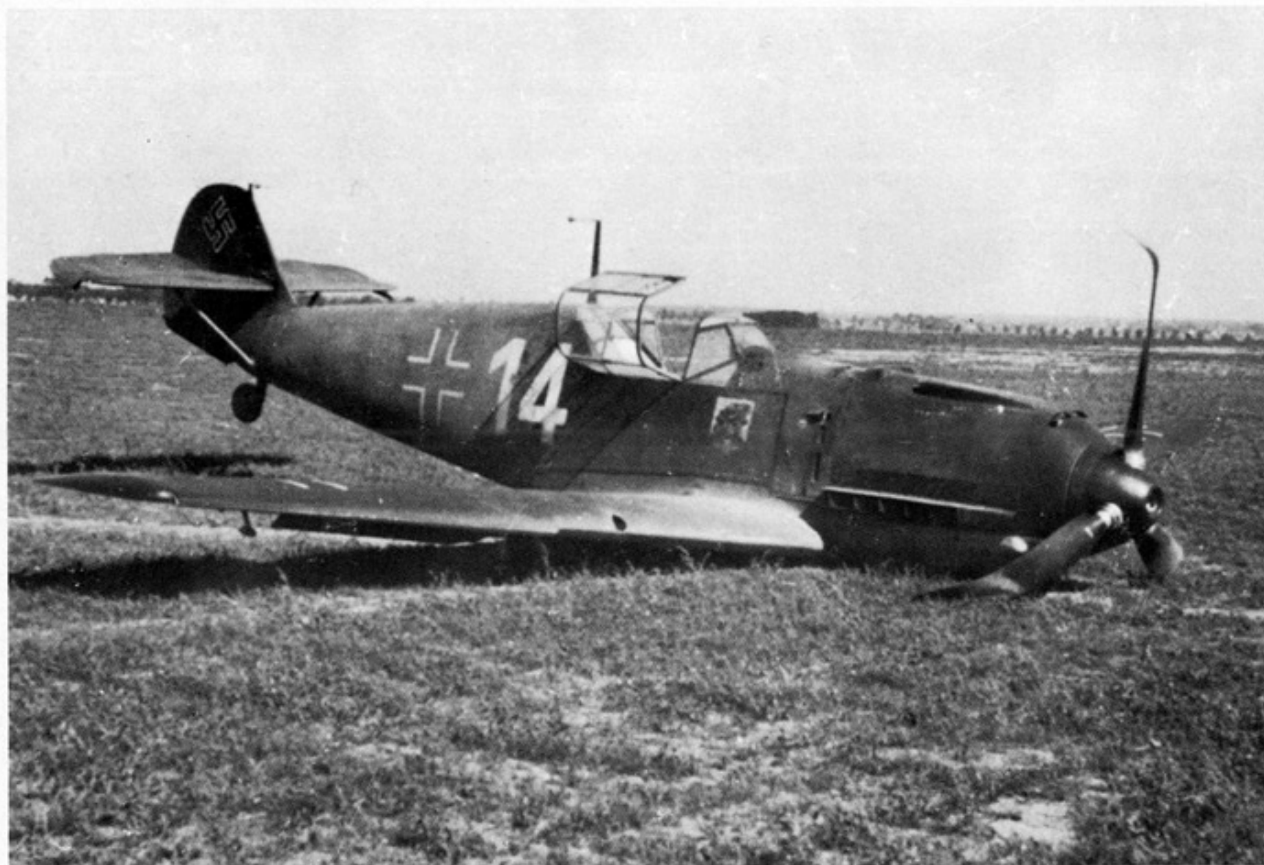
A Bf 109C-1 of 3/JG 21 (later 9/JG 54) at Gutenfeld/East Prussia early in the Polish Campaign. The rings on the spinner are in the 3. Staffel color of yellow. The wheels, which appear to be painted black, are in fact Gray (66), a very dark color. (K. Ries)
