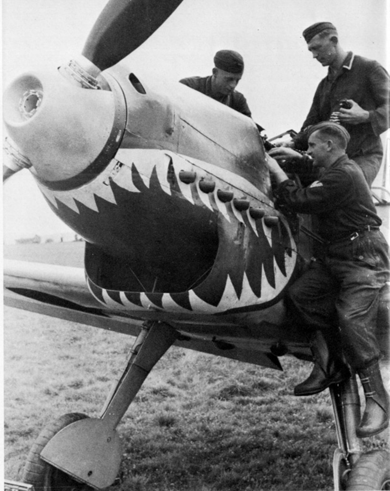
The two armorers are replenishing the MG 17 ammunition while the Obergefreiter in the foreground adjusts the fuel injection unit first introduced on the Bf 109C-1. This sharkmouthed machine is believed to belong to 2/JG 71 which later became II/JG 51 Mölders . (Bundesarchiv)
