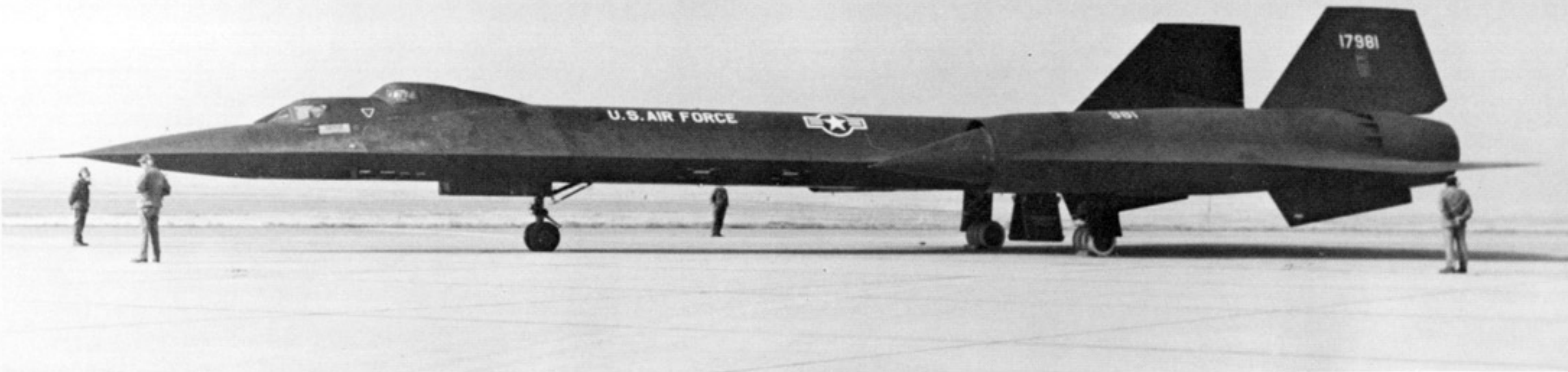
The one and only SR-71C was built from bits and pieces of an engineering mock-up and salvaged parts after half the SR-71B force was lost in the January 1968 crash of 951. Known as The Bastard , it was not extensively used, and has been in storage for several years. (Brian Rogers via Jerry Geer)
