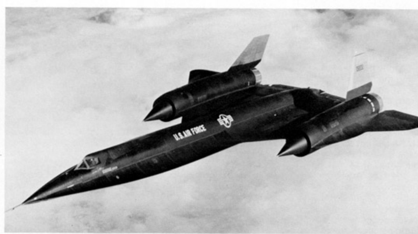
One of the few A-12s which were painted nearly all-black. The sharper nose profile, with more triangular-shaped chines are most evident in this view. Also of interest in an apparent flight test camera housing at the rear of the fuselage. The direction in which it is pointing indicates that it may have been mounted to record the launching of the D-21 Drone. (See page 22) (USAF)
