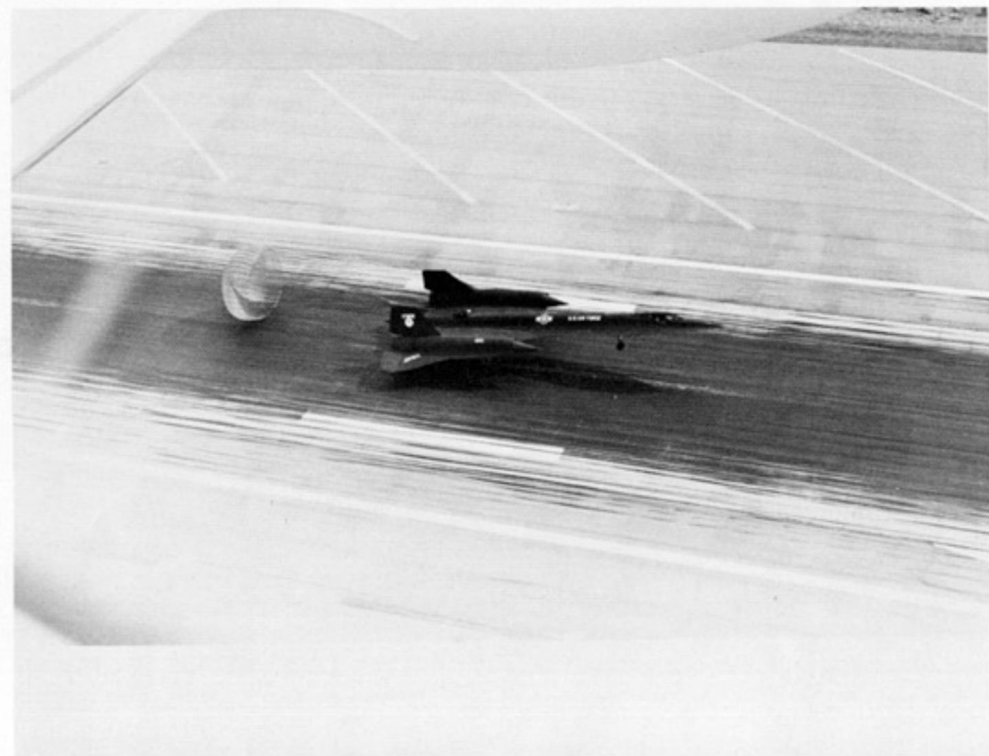
(Below) Large drag chute provides effective braking action on landing. It has been deployed here before the nose wheel is on the runway. Note the deflection of the out-board elevons. Drag chute must be released before the aircraft slows to 60 knots to avoid entanglement with rudders. (USAF)
