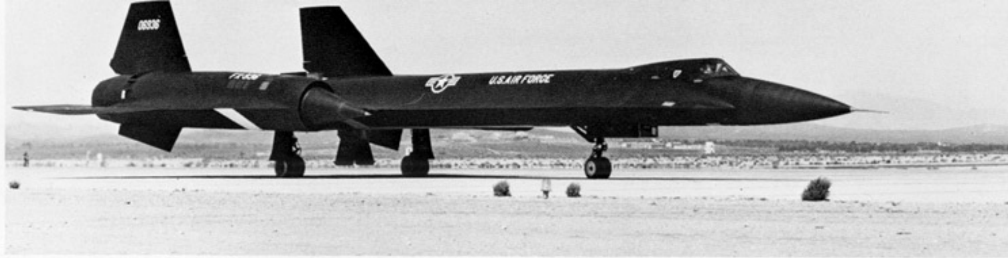
Yf-12A #06936 taxis in after a test flight. Note that the drag chute compartment doors are still open. White markings on undersides were to aid in calibration of record-run instrumentation during the record-setting flights of May 1, 1965. (Lockheed)
