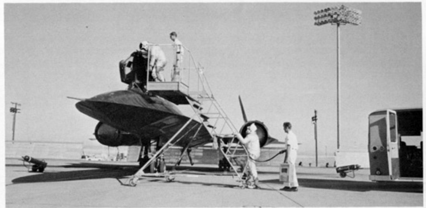
Once the crew is fitted with their pressure suits, they need portable air conditioning units to maintain comfortable body temperatures until they are plugged into the aircraft. (USAF)
