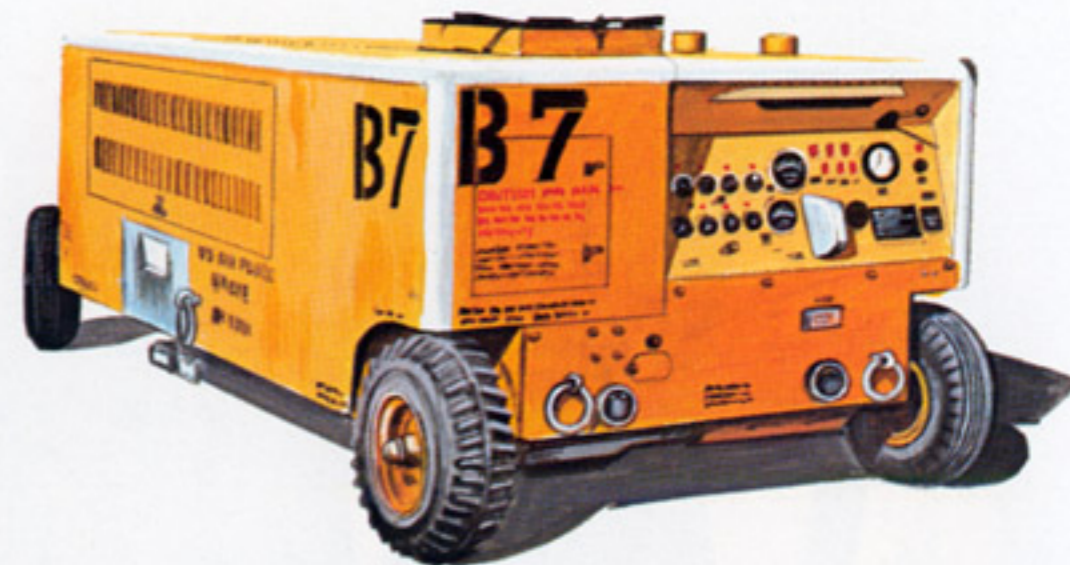
(Above) Provisional engine starter cart used twin Buick V-8's (unmuffled) to provide starting power to the SR-71's J-58's prior to installation of a permanent starting system in the hangers at Beale.
