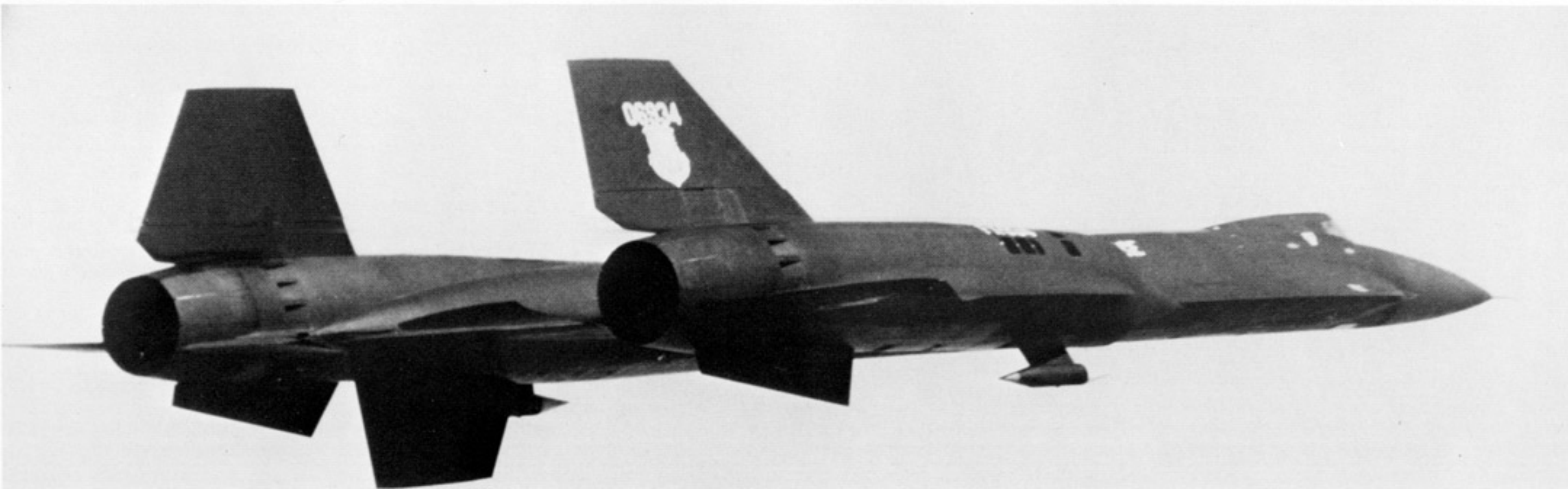
The redesign of the nose shape to accomodate the YF-12A Fire Control System is obvious in this bottom view of the Fighter version of the Blackbird. (John Mallozzi)
