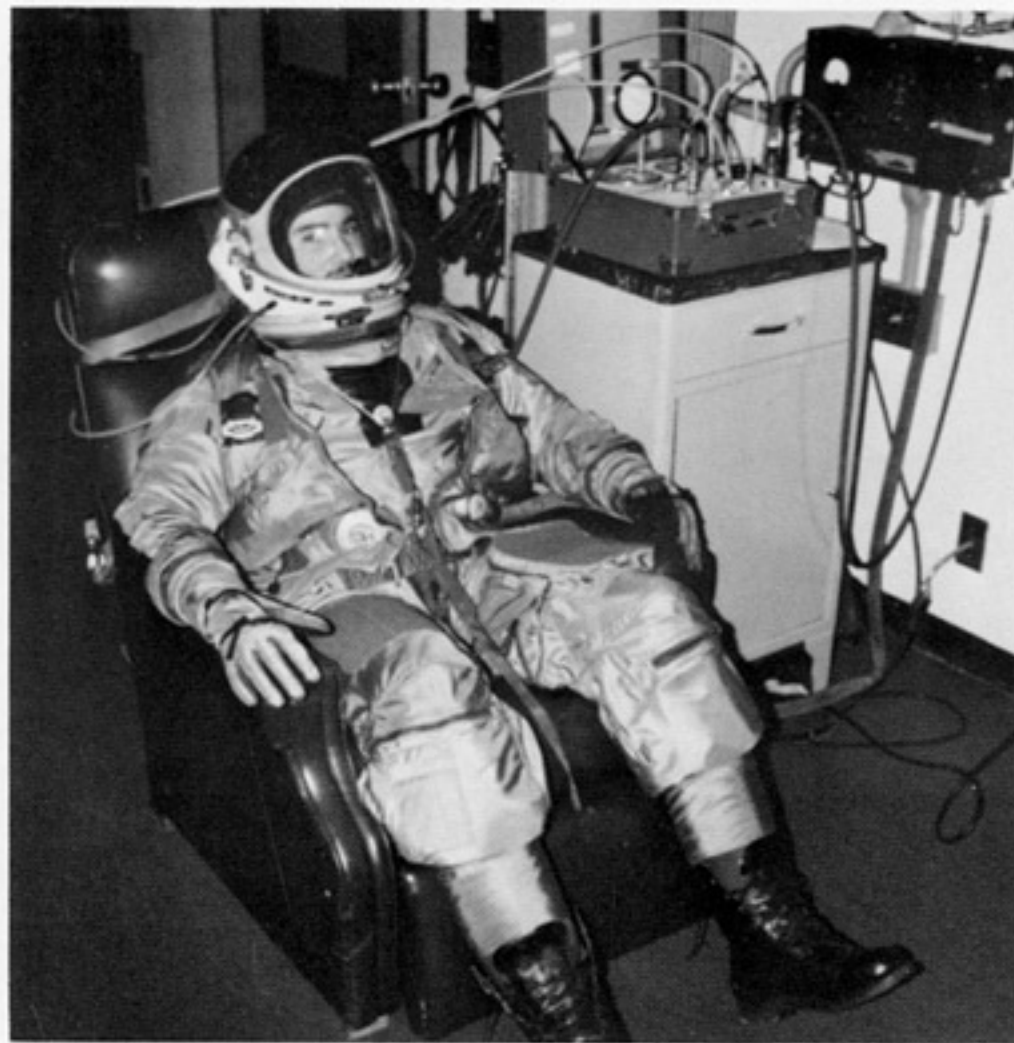
The suit worn by SR-71 crewmen is identical to that now used in the Space Shuttle. It is the principle protection in the event of an ejection at high Mach and altitude, and has been proven in several cases to be effective. (Author)
