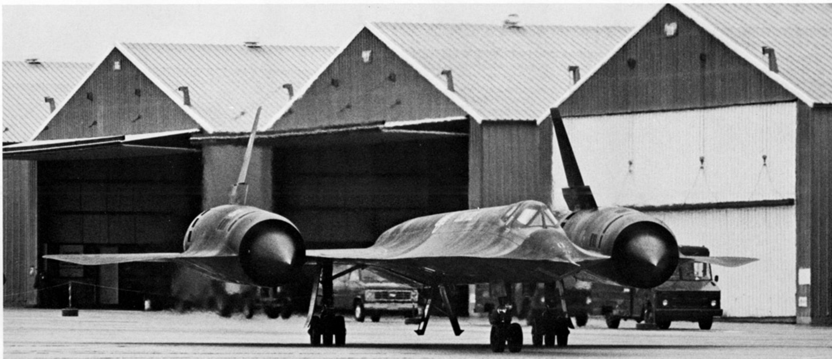
SR-71A serial number 64-17964 taxis away from the special hangars (built for exclusive use of the Blackbirds) at Beale AFB for a training mission during March of 1980. The camera nose is fitted, with cameras installed. (C.B. Mayer)
