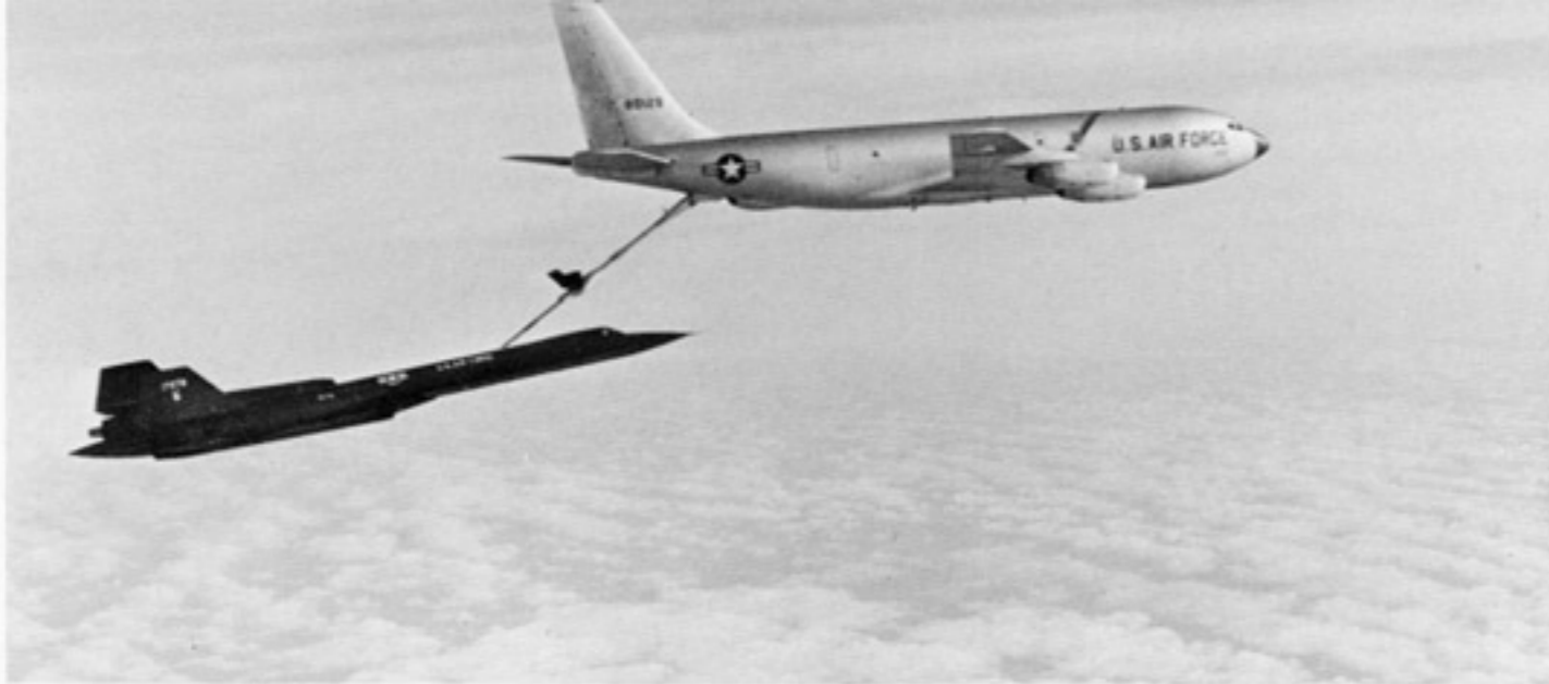
The Rapid Rabbit refuelling from a KC-135Q. Though the JP-7 is kept in separate tanks in the tanker, crew members report that they are able to burn it if necessary in the tanker engines. (USAF)
