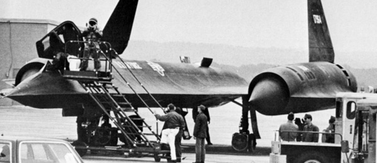
Blackbird crew de-planing at Offutt AFB, July, 1979. Note that ground crew have placed fans in front of the main gear in order to cool wheels and brakes. (Charles B. Mayer)
