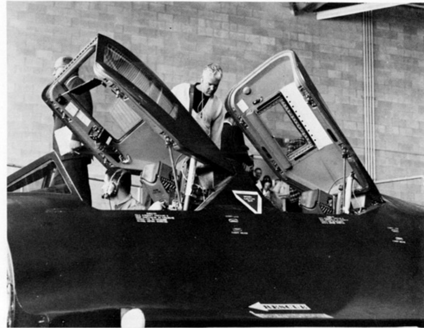
YF-12A undergoing ground checks during the initial flight test. Note that the YF-12s apparently were equipped with a different ejection seat than the SR-71. (Lockheed)
