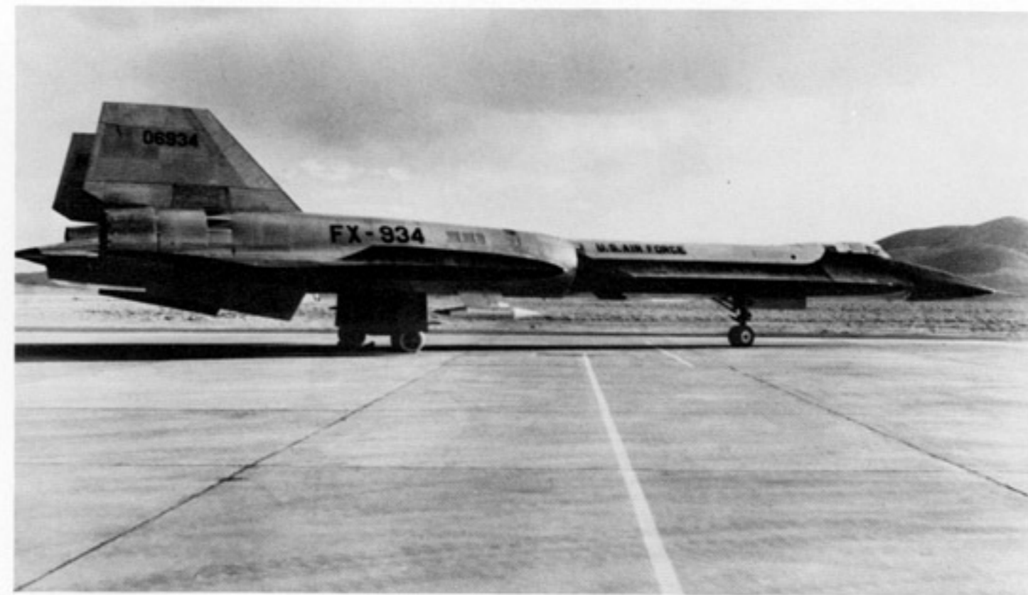
The "A-11" announced by LBJ, which was in reality the AMI, later designated YF-12A. First publicity photos showed the YF-12s in their CIA (mostly natural metal, ala A-12) finishes. (USAF)
