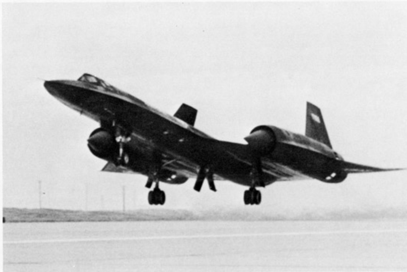
With a light fuel load, the SR-71's 30,000lb plus thrust J-58 engines allow it to accelerate quickly to a liftoff speed of approximately 200 knots. (USAF)
