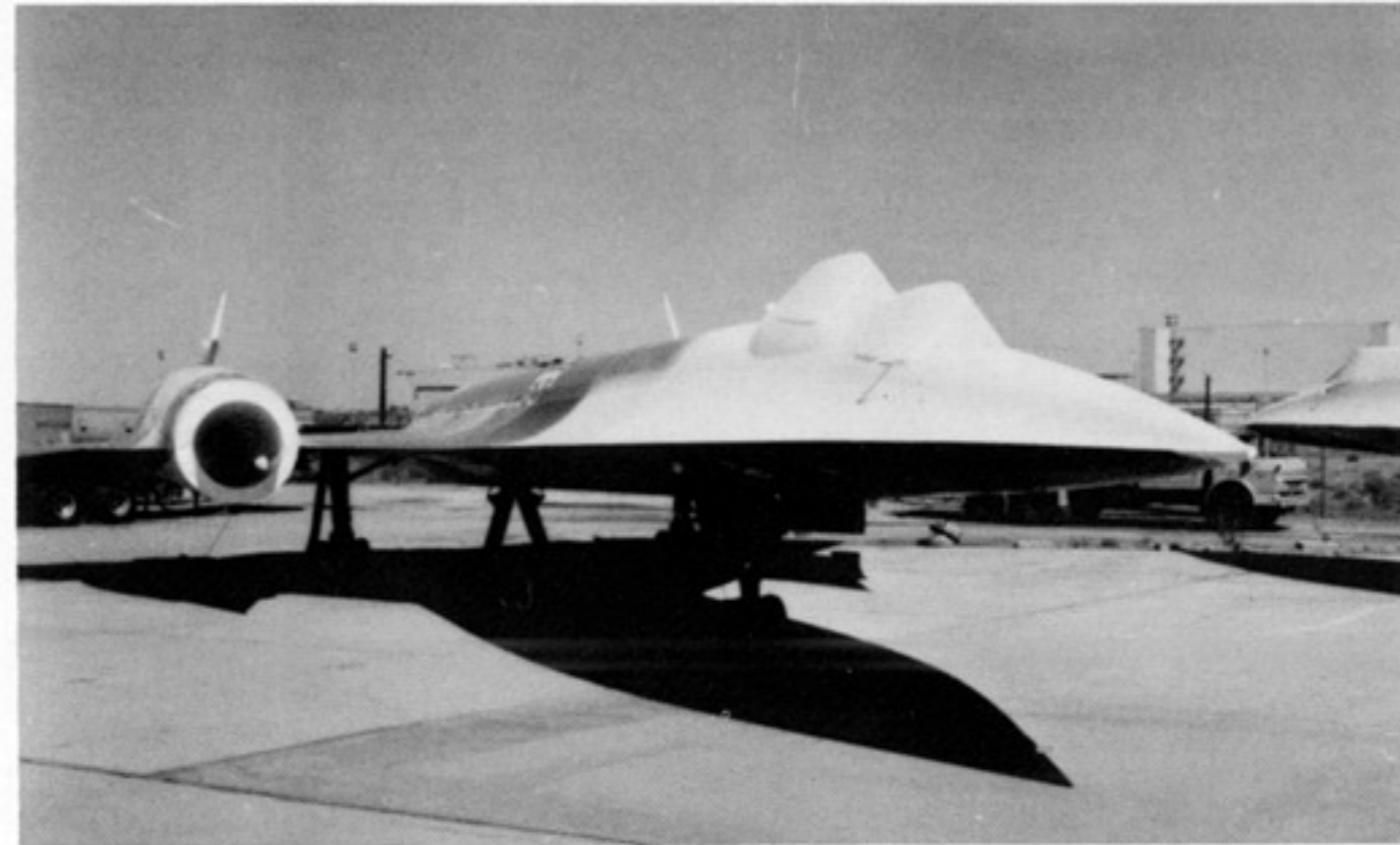
There was a two seat version of the A-12, used for pilot training. This one is in storage at Palmdale. (John Andrews)
