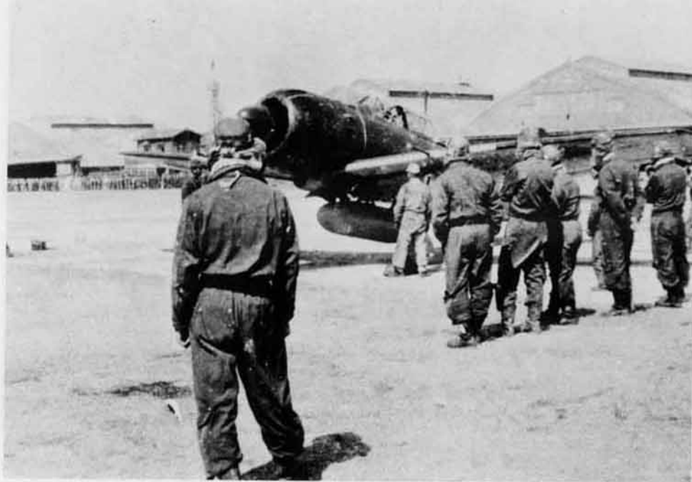
A Zero 52c, of the Yatabe Kokutai, carrying the late style drop tank with four attachment points.
