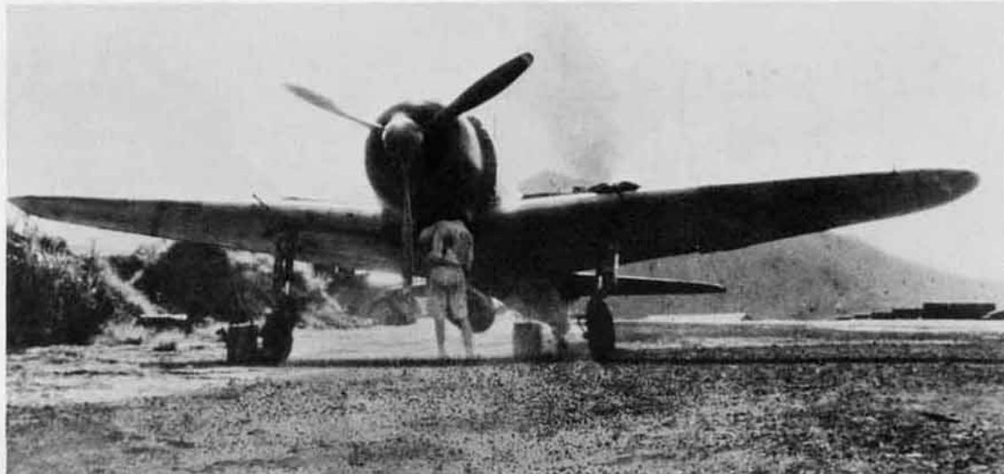
A6M3a Model 22a equipped with the long barrelled 20mm cannon at Rabaul. The smoke in the background is from an active volcano near the airstrip.
