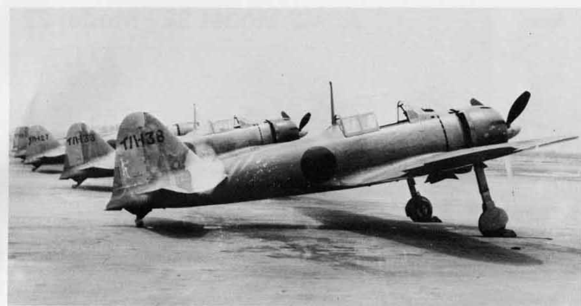
These Zero 22s of the Iwakuni (Training) Kokutai carry the overall Light Gray scheme. The new recessed rudder trim tab is the large dark area at the rear bottom of the rudder.
