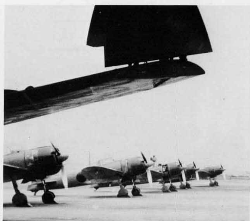
A line up of Zero 22s of the Iwakuni (Training) Kokutai, framed below the folded wing tip of another Model 22.
