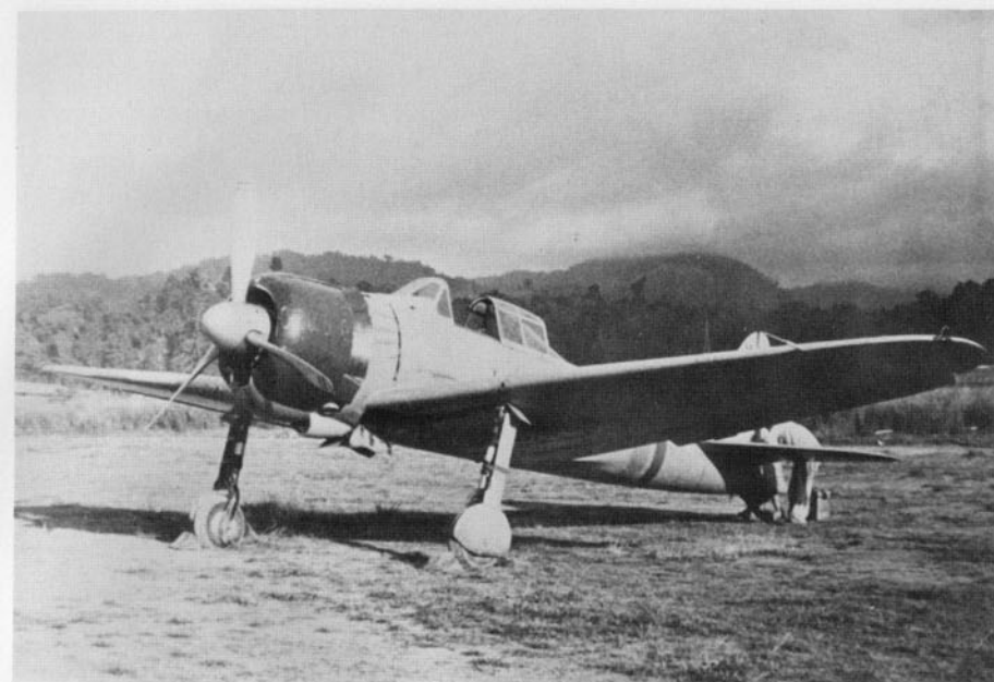
X-183, of the 23rd Hikotai at Ambon Island, has had the radio equipment removed. Since the radios experienced a very low degree of reliability and replacement parts were very difficult to obtain, pilots often had the radio equipment removed to save additional weight.
