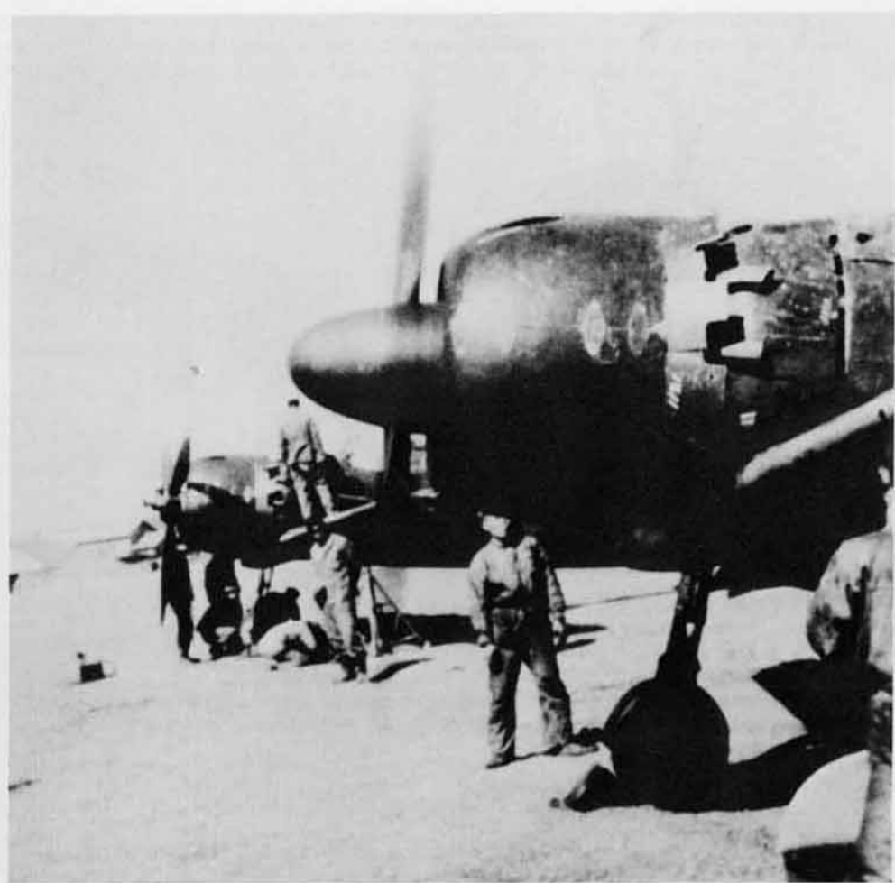
The new individual exhaust pipes replacing the exhaust collector ring helped to increase the Zero 52's maximum speed to 351 mph in level flight. The new exhaust pipes exited between the cowling flaps which were notched.
