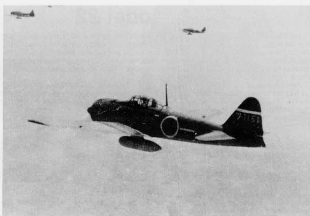
A formation of Zero 32s of the Tsukuba (Training) Kokutai. The White line on the fuselage and tail were aids for flight training.
