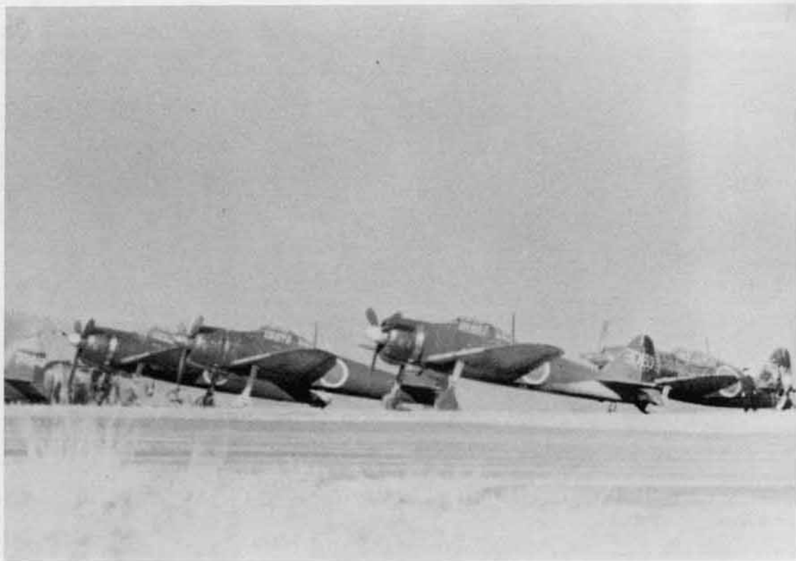
(Left) These aircraft belonging to the 302nd Kokutai at Atsugi during 1945 are part of the Home Defense. Each of the three Zero 21s carry a somewhat different camouflage scheme. The last aircraft is a J2M1 Raiden interceptor.
