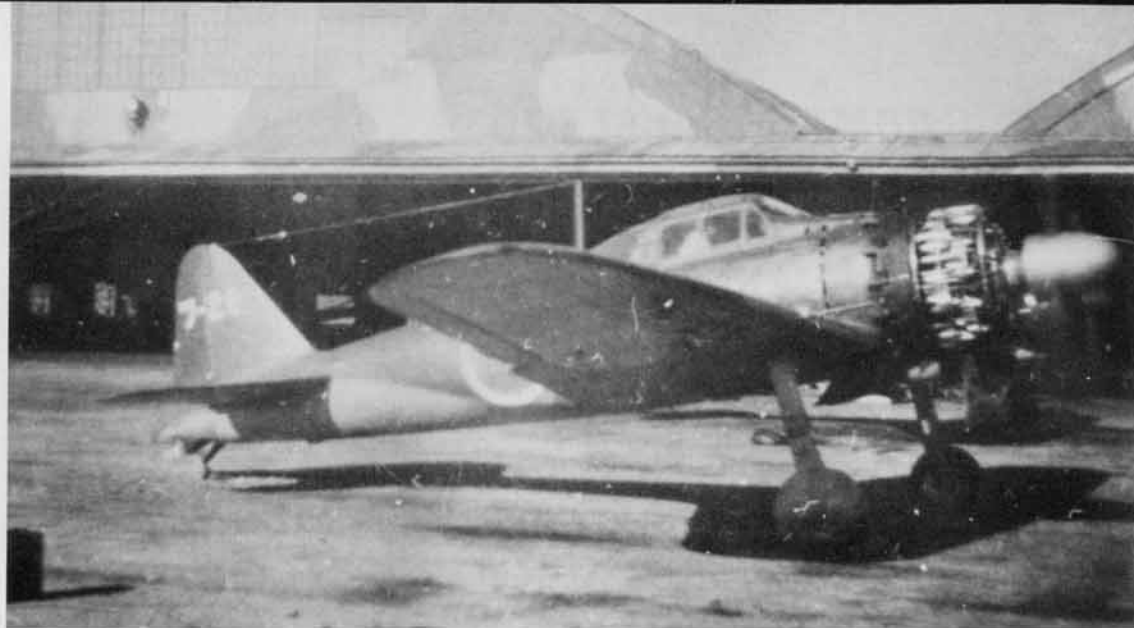
This Model 52 Otsu (Model 52b), TSU-29, belongs to the Tsukuba Kokutai, which was a training group until the B-29 raids forced the pilot instructors to begin carrying out interception missions. The 45mm armored glass added to the windscreen of the b-series is barely visible.
