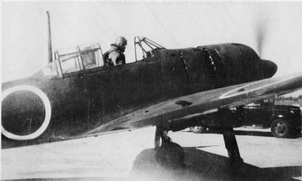
The Sakae 21 engine of the A6M3 Model 32 is being run up prior to takeoff. The lack of a gunsight indicates that this is probably a training aircraft. The camouflage is the standard late scheme of Dark Green upper surfaces over Light Gray lower surfaces. The White outline on the national insignia is the specified 75mm in width.
