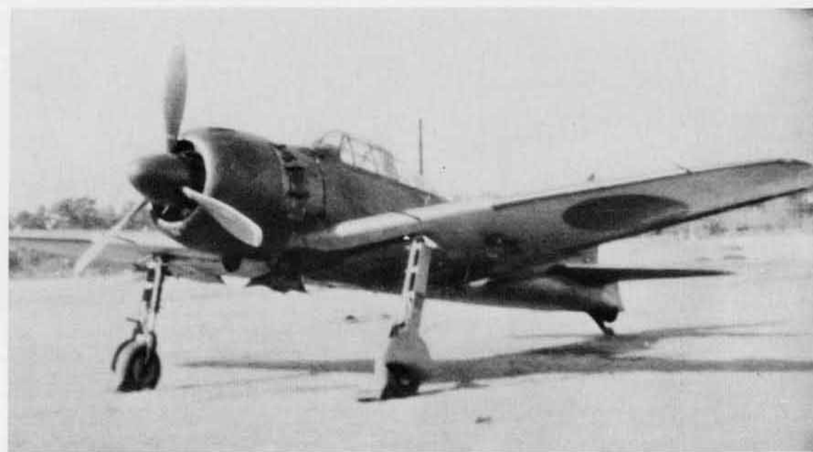
This A6M5 Model 52 is equipped with a 30/60 kg bomb rack under each wing mounted just outside the landing gear. Note how the Dark Green paint overlaps the wing leading edge.
