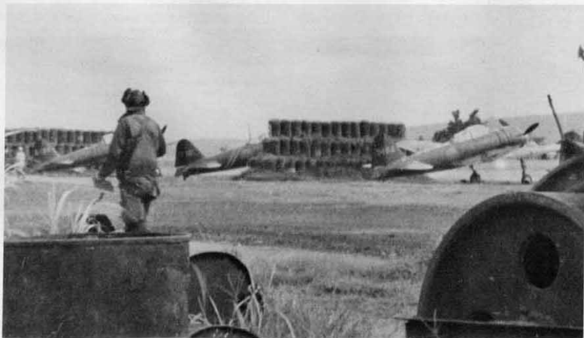
A6M3 Model 22s of an unknown unit at Rabaul in late 1943. The center aircraft, coded 7-101, carries two Yellow/Orange diagonal fuselage bands and is believed to belong to the unit commander. Each aircraft has had its landing gear covers removed. The revetment is made of earth filled fuel drums.
