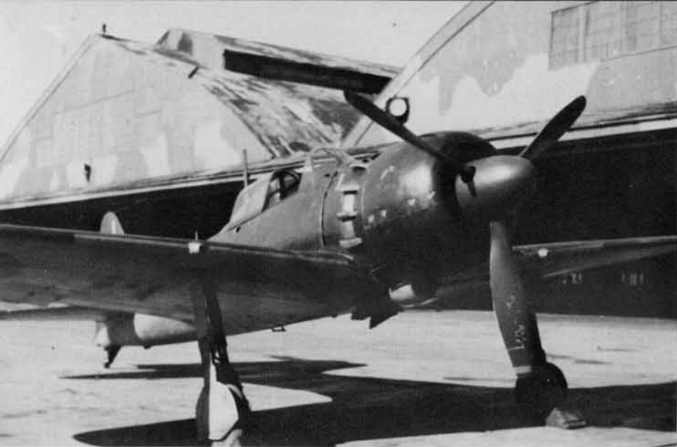
The removal of the 20mm wing cannon allows an excellent view of the new fairing.
