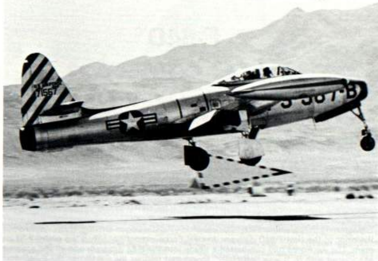
33rd FG F-84C landing at Las Vegas AFB (now called Nellis) after a gunnery mission. Notice how far all three landing gear struts have extended. (Col. W. Thomas, via Taylor)
