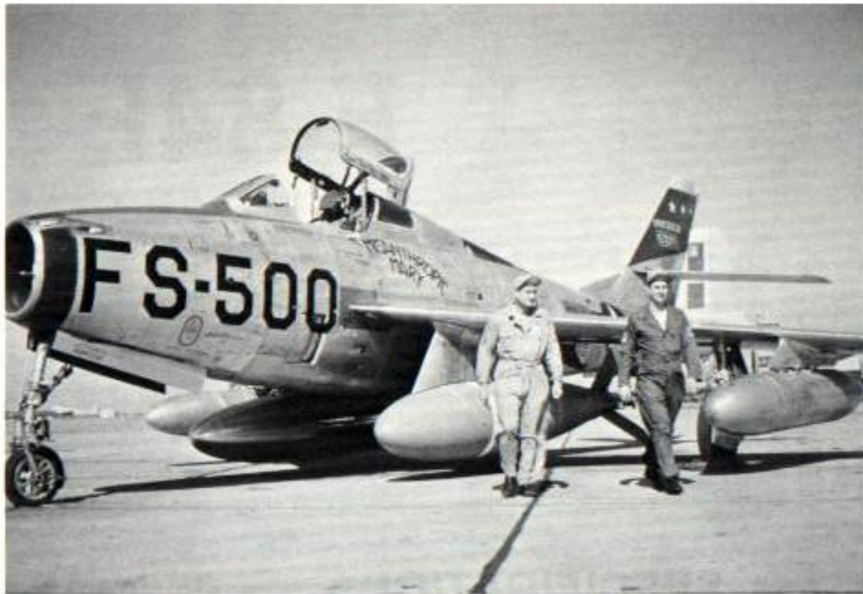
"Misanthropic Mary", from the 405th FBWg, carries a practice Mark 7 nuclear bomb on the port special store pylon. The F-84F used the Low Altitude Bombing System (LABS), to deliver nuclear weapons. This was commonly called 'toss bombing'. (USAF)
