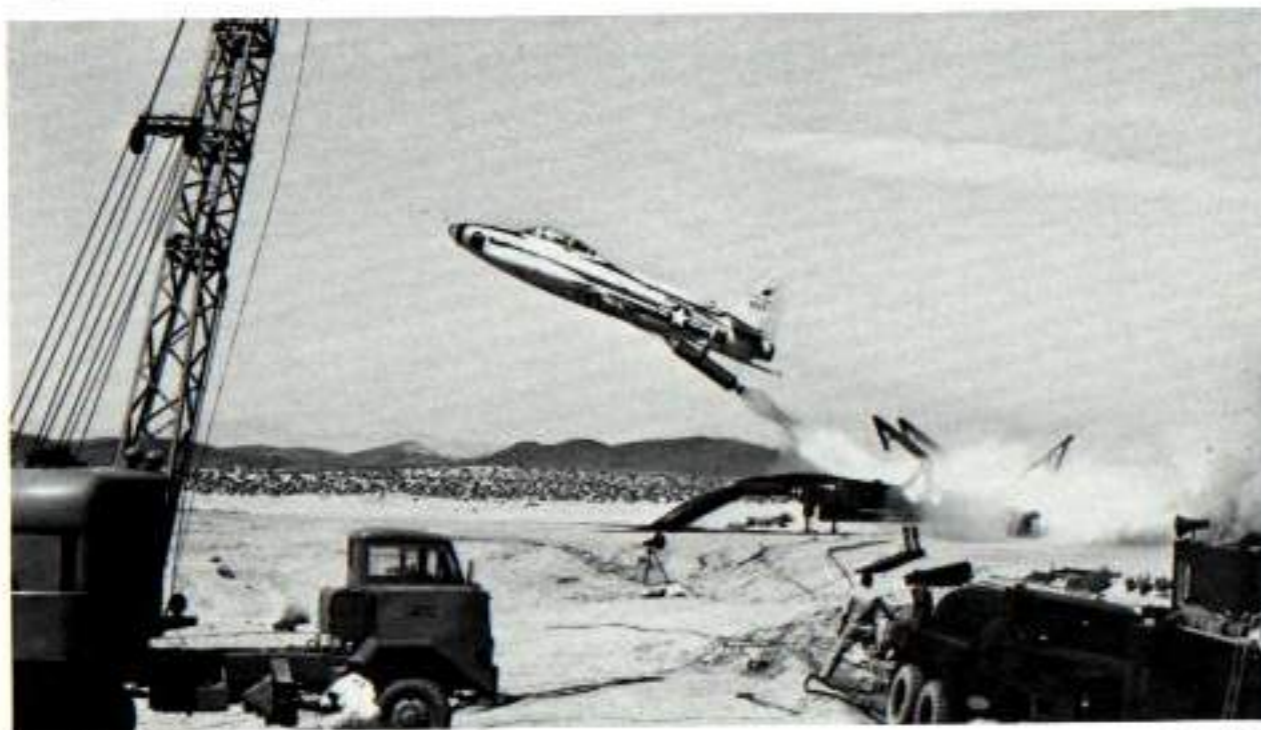
EF-84G serial 51-1225, was converted to test the Zero Length Launch concept. The bird was launched from a Matador Missile launcher by a solid fuel booster rocket, which was then jettisoned and the aircraft would proceed to its target using its normal J35 powerplant. The idea was to place these aircraft in camouflaged wooded areas around the Soviet Union, armed with nuclear weapons, and await a possible attack. Without a runway, the ZELL F-84Gs could be hidden in hundreds of places, making them virtually impossible to knock out. The concept is quite similar to that of today's Cruise Missile, only these were manned aircraft. (Menard)
