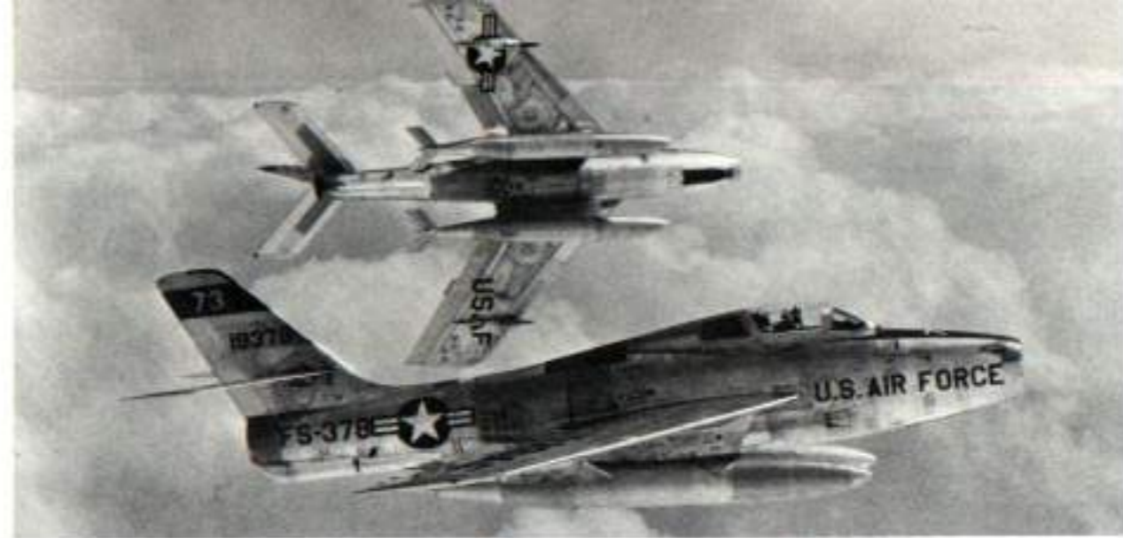
A pair of 31st SFWg F-84Fs inflight near Turner AFB, Georgia in April 1957. Of note are the great variety of metal shades which indicates the many different alloys used. The tail band and nose gear doors are Insignia Blue with a Yellow number, which is repeated on the angle panel. (USAF via Menard)
