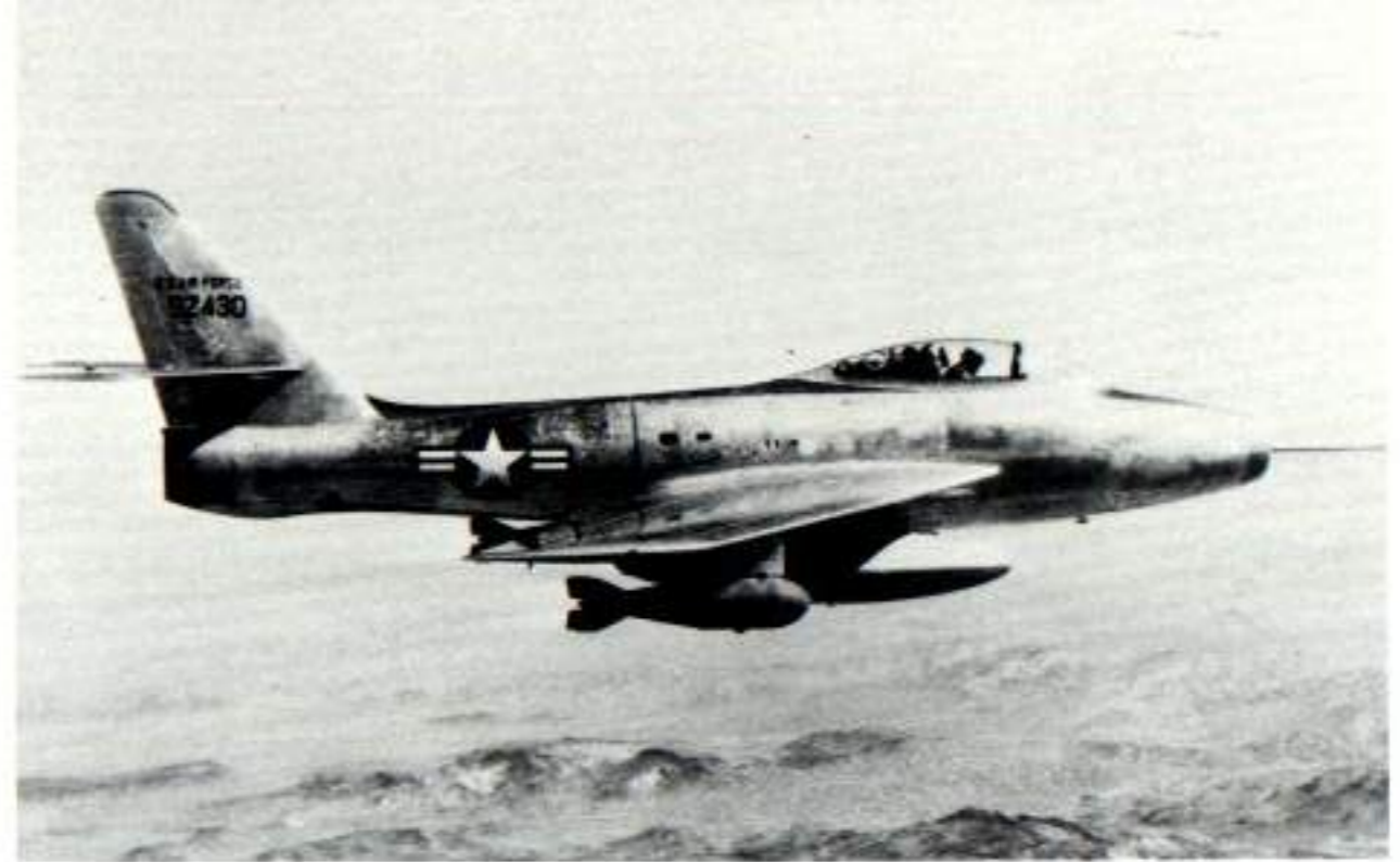
The YF-96A inflight over Edwards AFB during the summer of 1950. The YF-96A had a standard F-84E fuselage but had swept wing and tail surfaces. Note the v-shaped windscreen similar to that found on the F-86A Sabre. (AFM)
