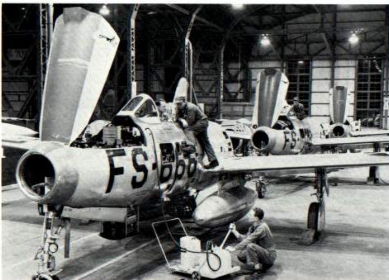
All major maintenance on the F-84s in Korea was performed at the REMCO (Rear Echelon Maintenance Combined Operations) facility at Itazuke AB, Japan. The aft fuselage sections have been removed and the engines taken to another area for testing and rebuilding. The armament bay is in the upper nose, while the battery hangs down behind the nose gear well. (USAF)
