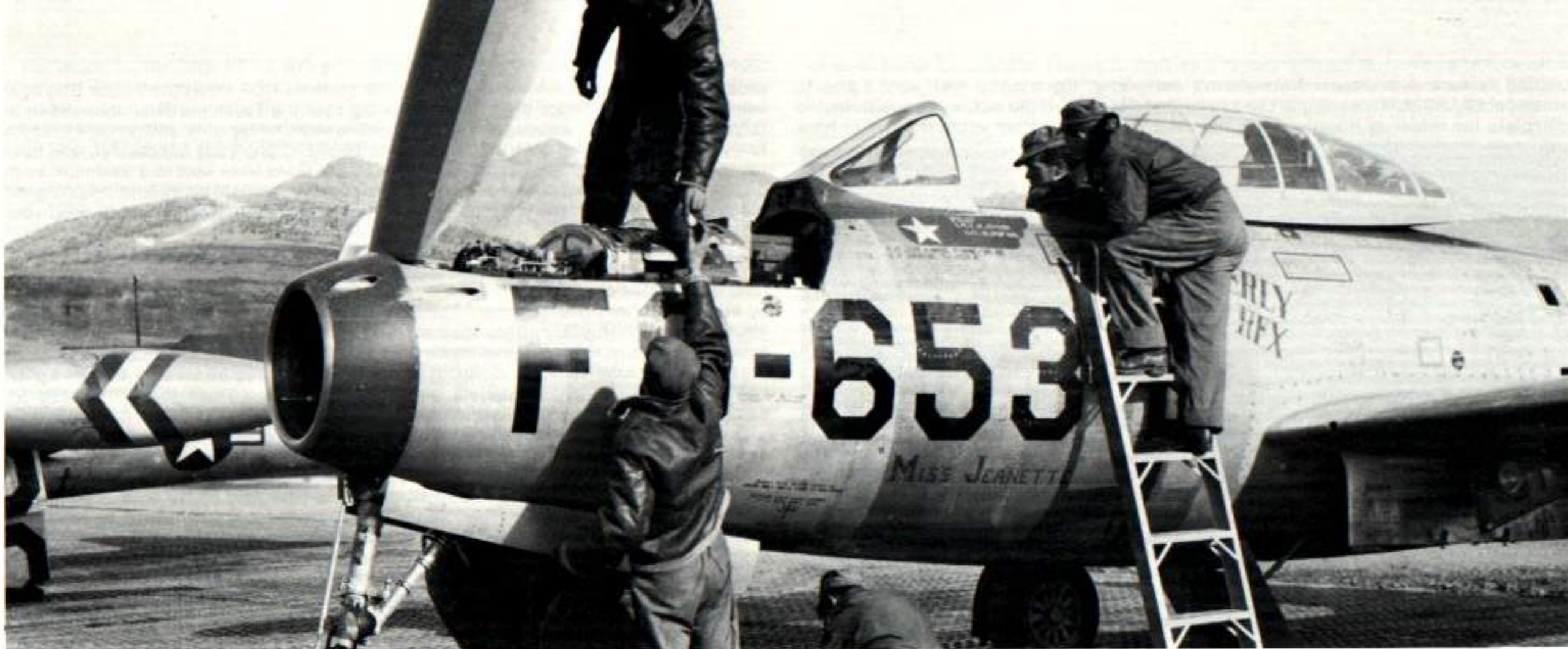
An obvious change has taken place here. But what radio call sign is used — "Air Force 651" or "Air Force 545"? Although having a mismatched fore and aft fuselage, the aircraft is fully combat operational, an indication of how badly the F-84s were needed in Korea. (Galbraith via Menard)
