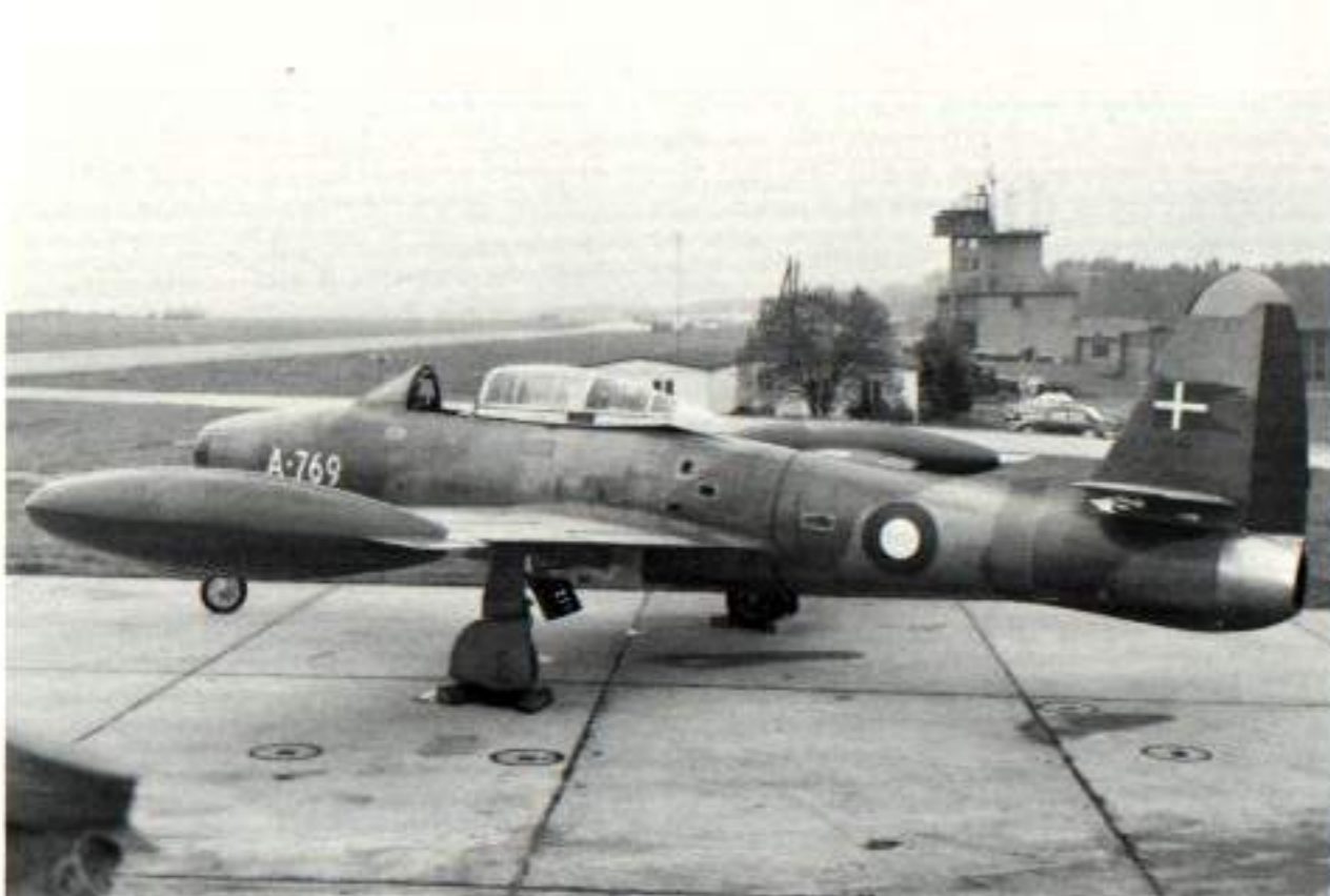
(Above) Late in the service life of the Danish Air Force F-84Gs, they were camouflaged in the standard NATO colors of Dark Green and Ocean Grey, over Medium Sea Grey under-surfaces — all RAF colors. See the color illustration for details of this No. 730 Eskadrillen aircraft. (Menard)
