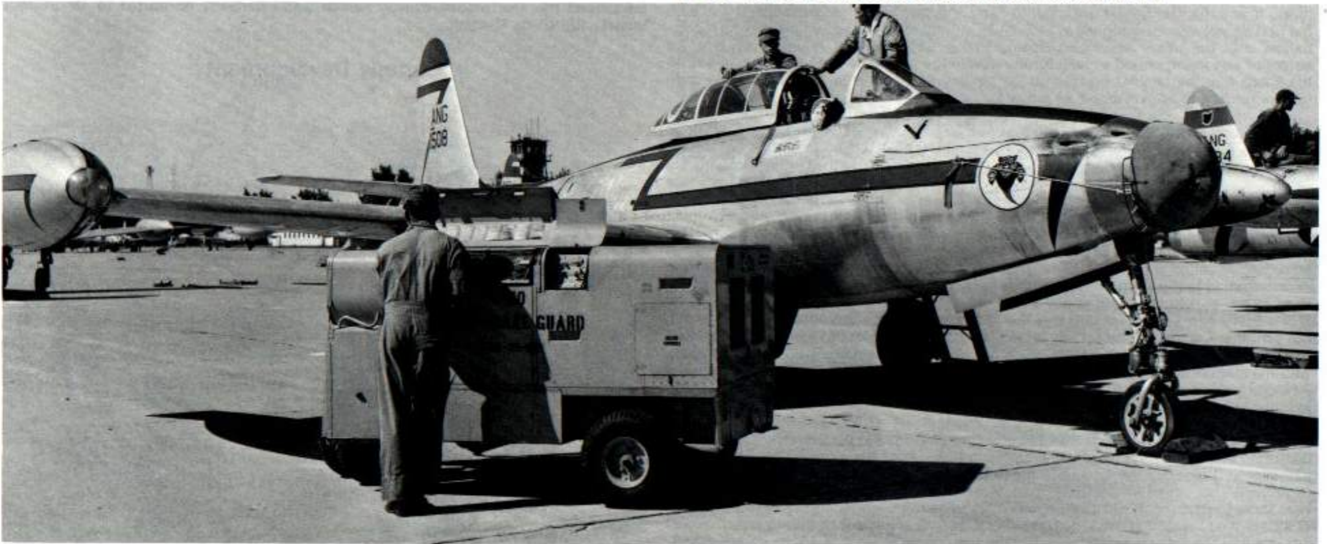
The F-84E was the backbone of the Air National Guard fighter-bomber force well into the late 1950s. This Ohio Air Guard aircraft was recently transferred from the Iowa ANG as it still carries the color flash from its former unit. Note the fine mesh screen over the intake to keep foreign matter out of the jet intake during ground runups. The smallest amount of dirt was hazardous to the health of the temperamental J35. (AFM)
