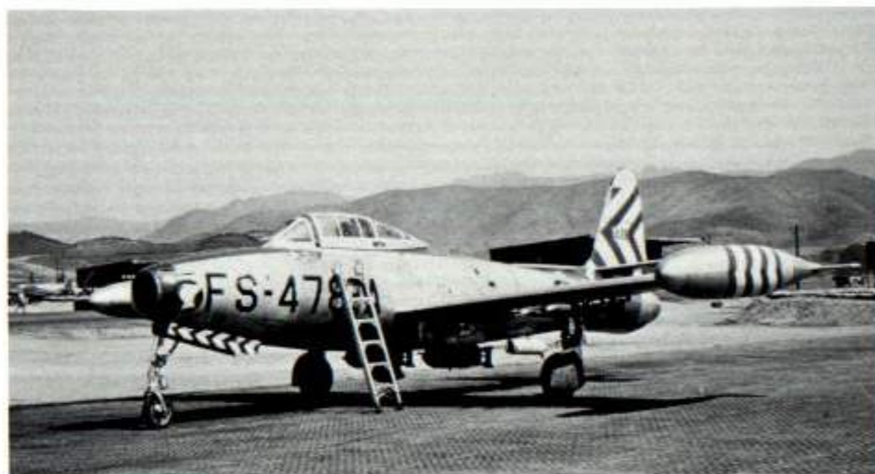
"Lil' Butch" from the 9th FBSq, 49th FBGp, with a full combat load of two 500 lb GP bombs, four 5 inch HVAR rockets, and two JATO bottles. "Butch" is the squadron CO's aircraft as denoted by the multiple Red and White wingtip tank stripes. (Galbraith via Menard)
