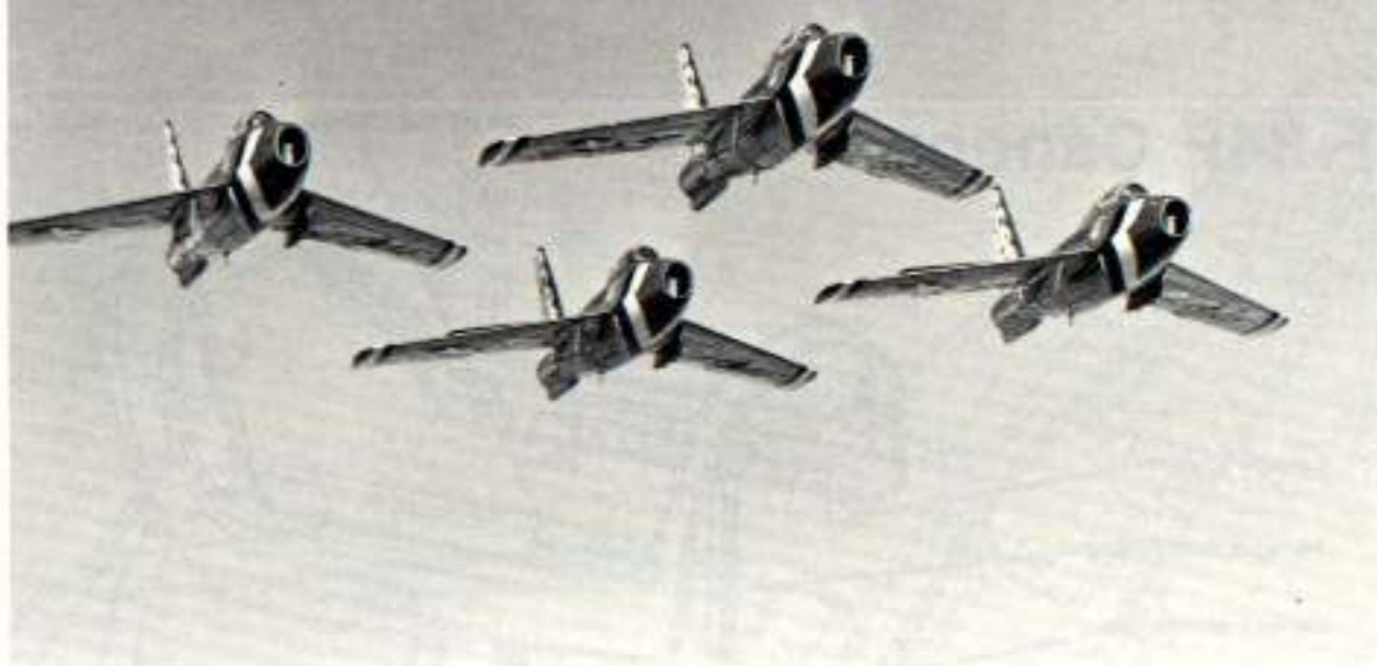
The US Air Force Thunderbirds switched from F-84G straight-wing Thunderjets into new swept-wing F-84F Thunderstreaks during the 1955 season, flying these aircraft until May 1956 at which time they went supersonic in North American F-100C Super Sabres. Note the added TACAN radio antenna under the fuselage. (USAF)
