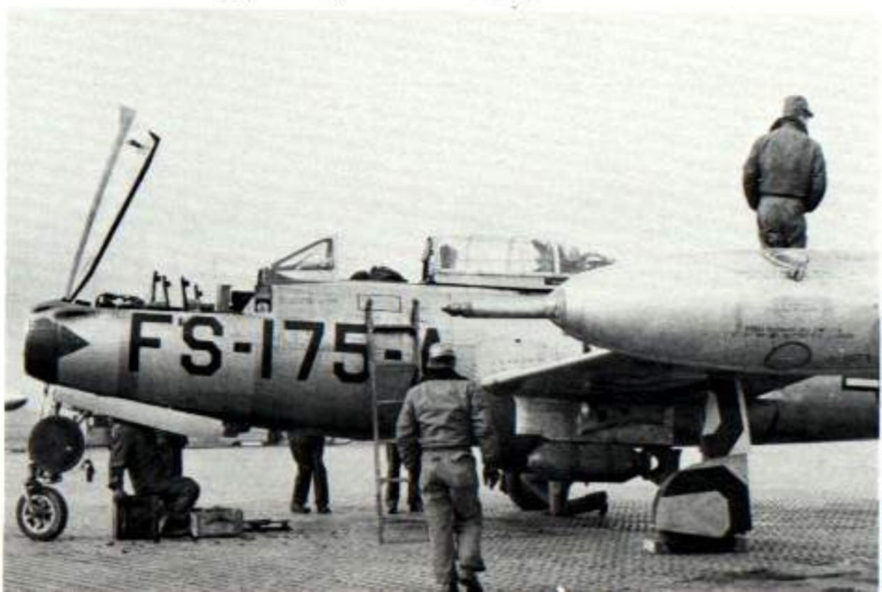
A HI-TIDE aircraft from the 159th FBSq with refueling probes mounted in the wingtip tank. Only the wingtip tanks could be refueled by this method and only Far East Air Force F-84s had the modified wingtip tanks. (Mason via Menard)
