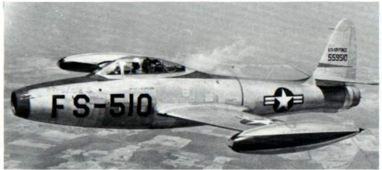
"Virginia S", a 20th Fighter Bomber Group F-84B over Langley, Virginia in 1948. Note the lack of stabilizing fins on the wingtip tanks. (USAF via Menard)
