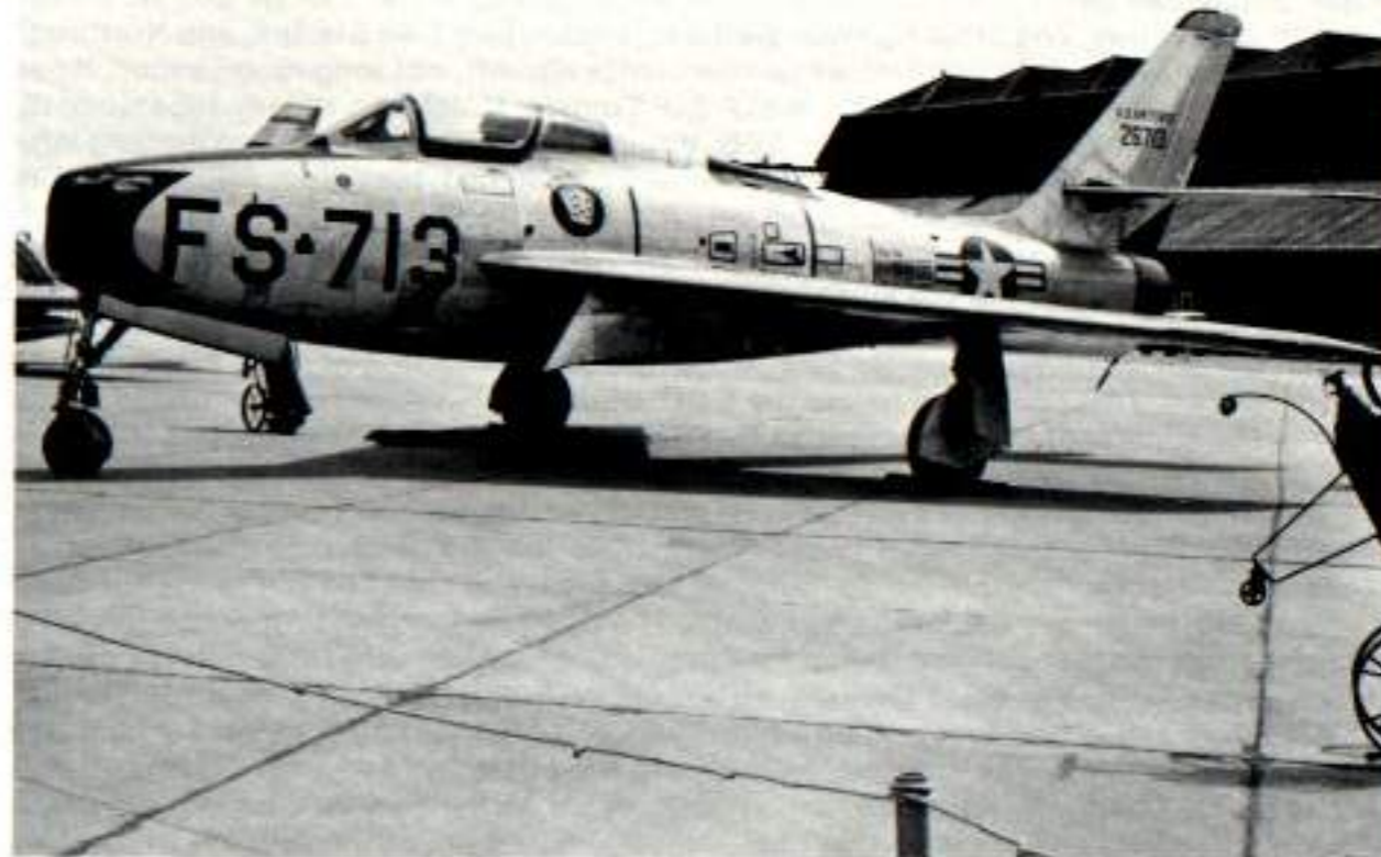
An operational F-84F from the 77th FBSq, 20th FBGp, at Wethersfield RAF Base in the United Kingdom. Note the radical change in the canopy design over that found on the YF-84F prototypes. Of special note is the special weapons pylon needed for delivery of nuclear weapons. 77th FBSq aircraft were trimmed in Red. (R.L.Ward via Menard)
