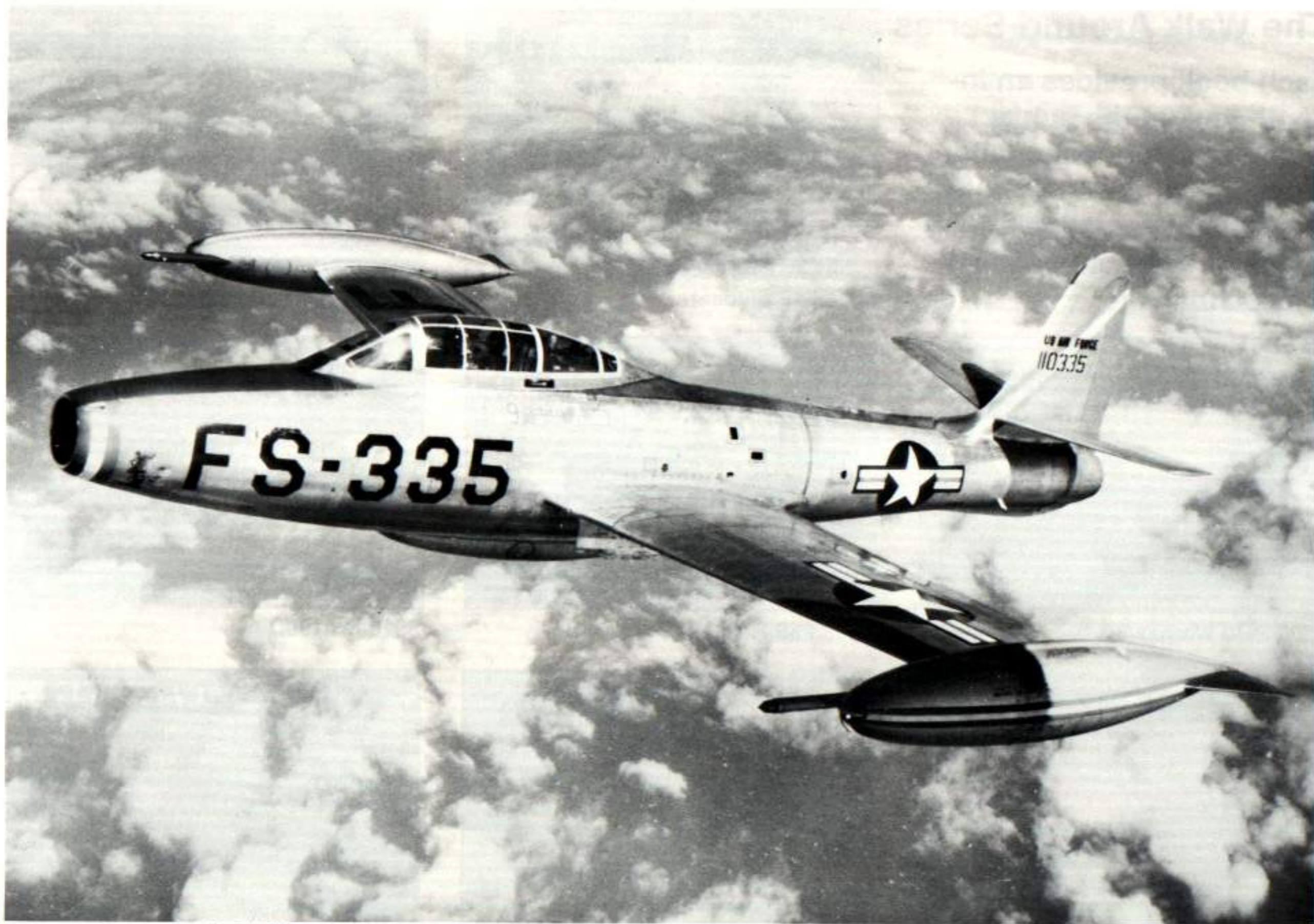
An F-84G from the 9th FBSq over Japan in December 1953. Even though the G model was built to accept the Boeing flying boom refueling method, FEAF F-84Gs still used the modified wingtip tanks with probes as all the tankers in the Far East used the probe and drogue system. (USAF)
