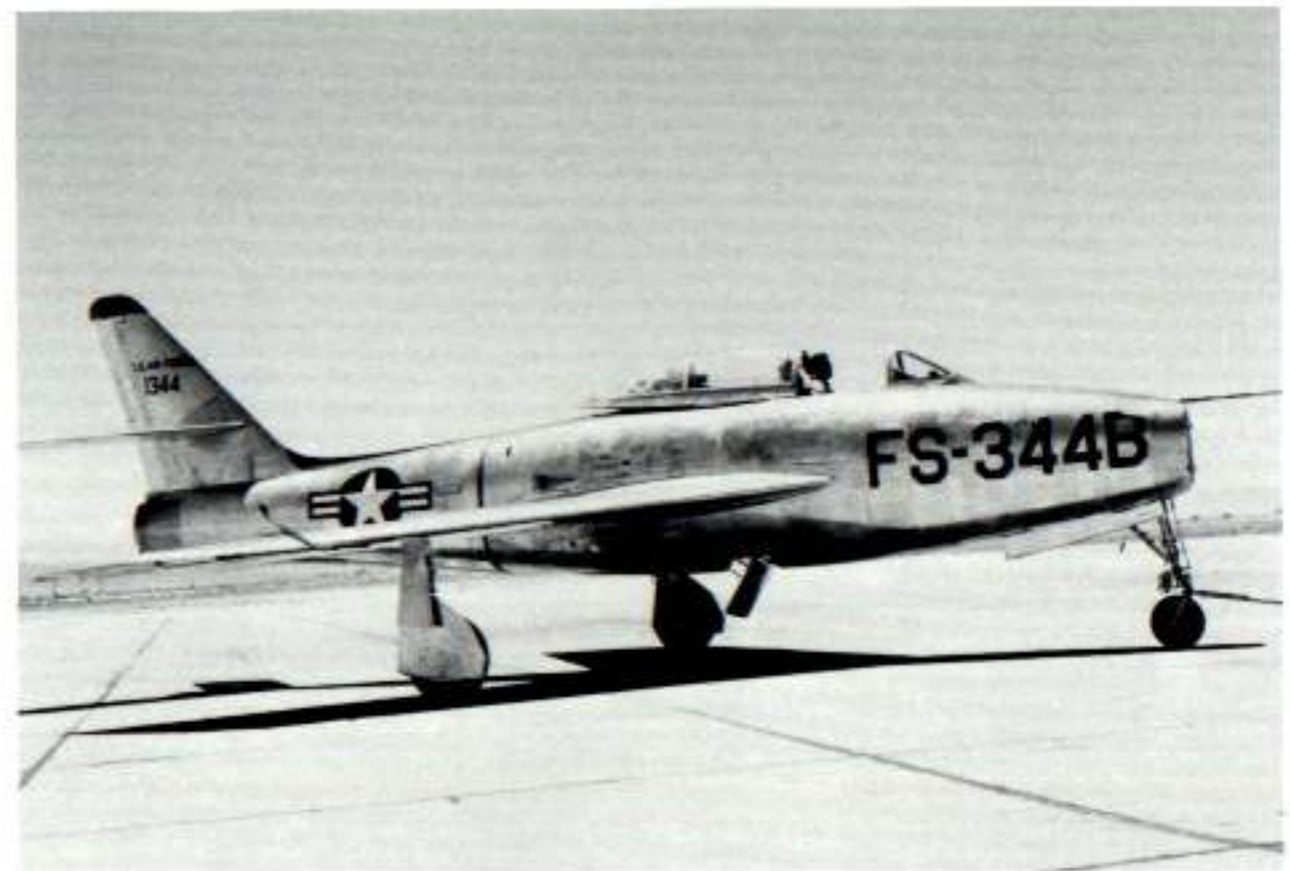
The first YF-84F on the Edwards AFB ramp in 1952. Note the 6 inch vertical spread throughout the length of the fuselage needed to both accommodate and supply air to the new XJ-65-B-3 engine. The v-shaped windscreen was removed from the YF-84F prototypes in favor of a new flat armored glass windscreen. (Wm. J. Balogh)
