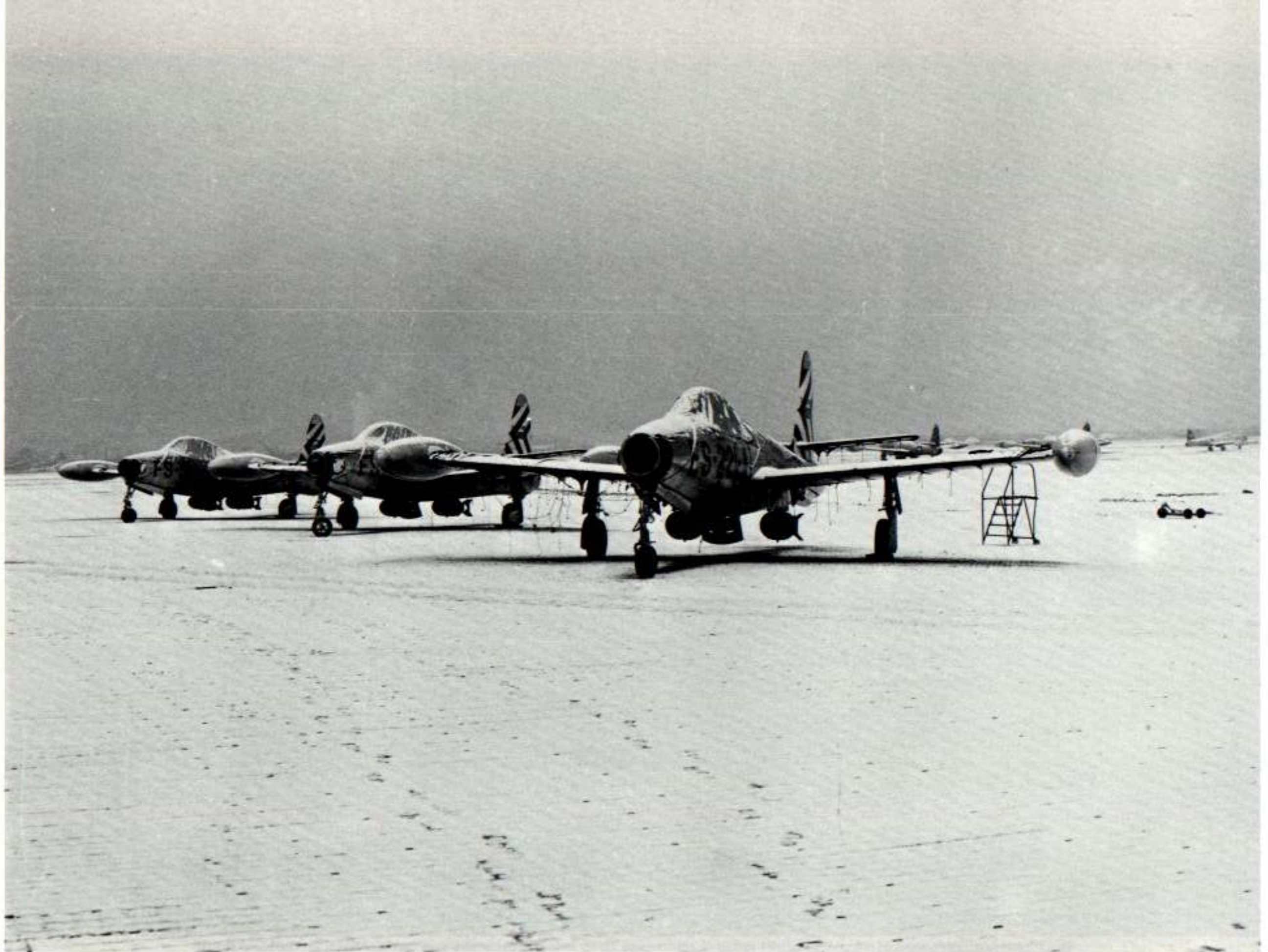
A trio of 9th FBSq F-84Gs sit combat ready in the snow at Taegu. The canopy and all flying surfaces are covered with canvas tarps to prevent ice build-up on moving parts and flying surfaces. (AFM)
