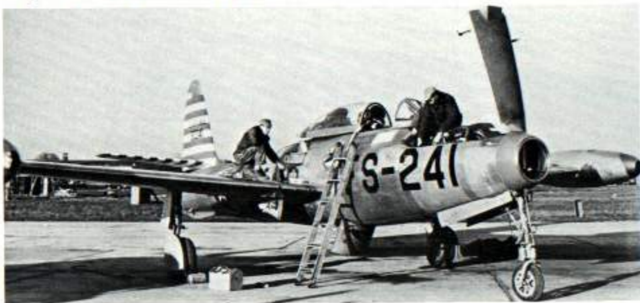
A Red and White striped F-84E from the 86th FGp. Compare these markings with those above. The armorer on the wing is loading the ammo cans that feed the starboard wingroot .50 calibre machine gun. (Jourdan)
