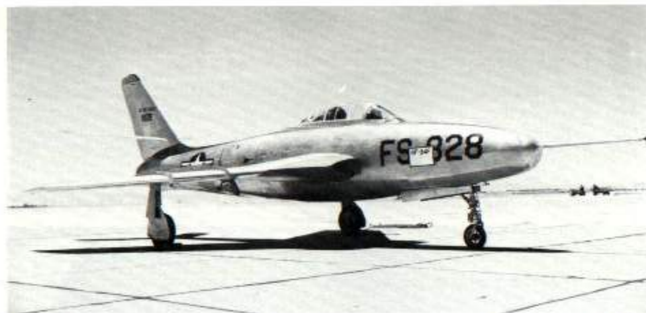
The YRF-84F prototype on the Edwards AFB ramp in July 1952. Note the reinforced F-84G-style canopy (deleted on production aircraft), the all-flying tail surfaces, and lack of camera windows. (Balogh)
