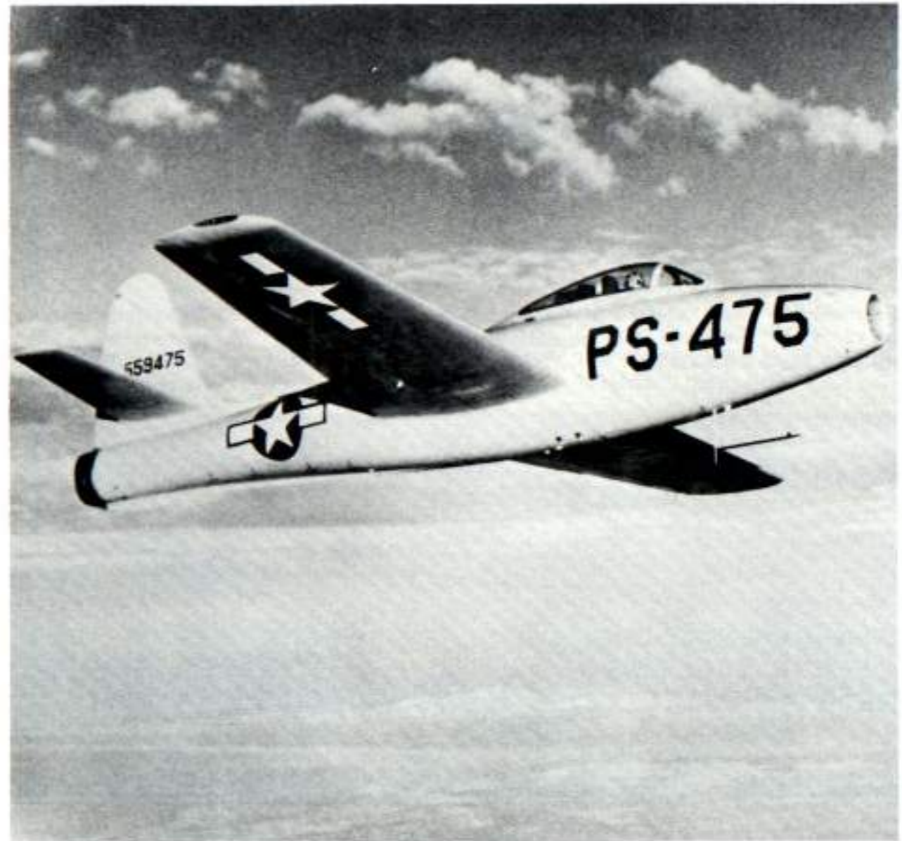
The No. 1 prototype XP-84 inflight over Muroc Field, in 1946. It is painted in the light Pearl Grey that was scheduled to be the standard paint scheme for Army Air Force jet fighter aircraft. The painted surface was supposed to cut through the air better than an unpainted, or natural metal surface. But the paint peeled badly at high speeds, causing an even greater loss in airspeed and the Air Force switched back to natural metal. Note the pitot boom on the port wing and the radio antennae under the forward fuselage. The buzz number was repeated on the underside of the left wing. (Republic via Menard)
