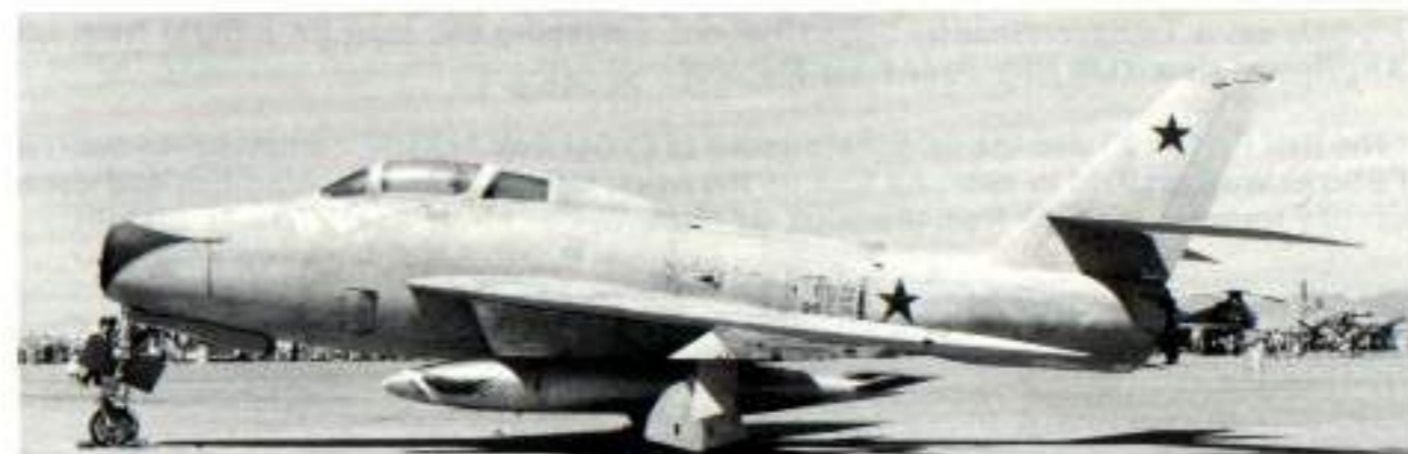
F-84Fs fought many battles in the 'reel war' as Hollywood used them to simulate MiG-15s in the movies "The Hunters" and "The McConnell Story". The aircraft were painted Light Grey (FS 36440) overall with Red stars. What appears to be a painted nose scallop is actually an air intake cover. (Baker)
