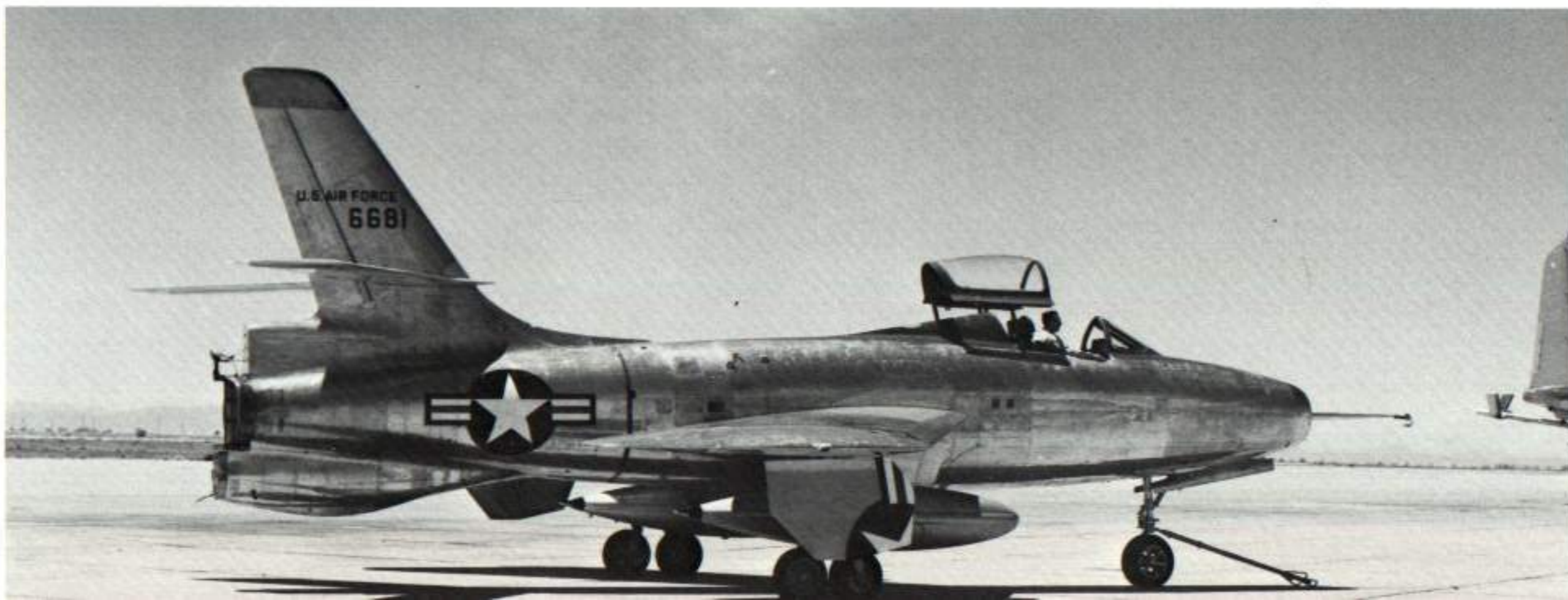
The XF-91 was a direct outgrowth of the F-84F program. The aircraft was strictly experimental having many innovations such as an internally mounted KLR 11-RM-9 rocket engine with 6000 lbs of thrust in addition to the J47 turbojet engine normally used. Another radical change was the inverse-taper wing which was wider at the wingtip than at the wingroot. The aircraft was later modified by the addition of an F-86D-style nose and now rests at the Air Force Museum in Dayton, Ohio. (Balogh)
