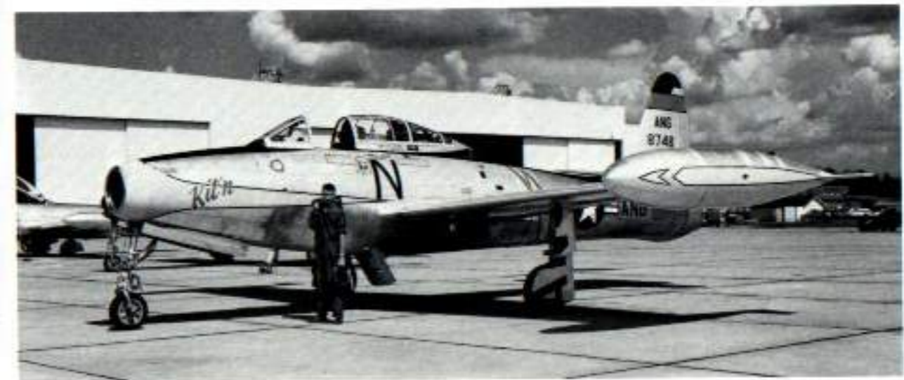
"Kit'N", an F-84D from the 128th FBSq, Georgia Air National Guard, seen at Dobbins AFB, Georgia in 1955. Note that "Kit'N" has had the braced canopy retrofitted. Air National Guard aircraft did not carry 'USAF' on the upper right and lower left wings, substituting the letters 'ANG' and the last three digits of the serial number in their place. (116th FBWg via Taylor)
