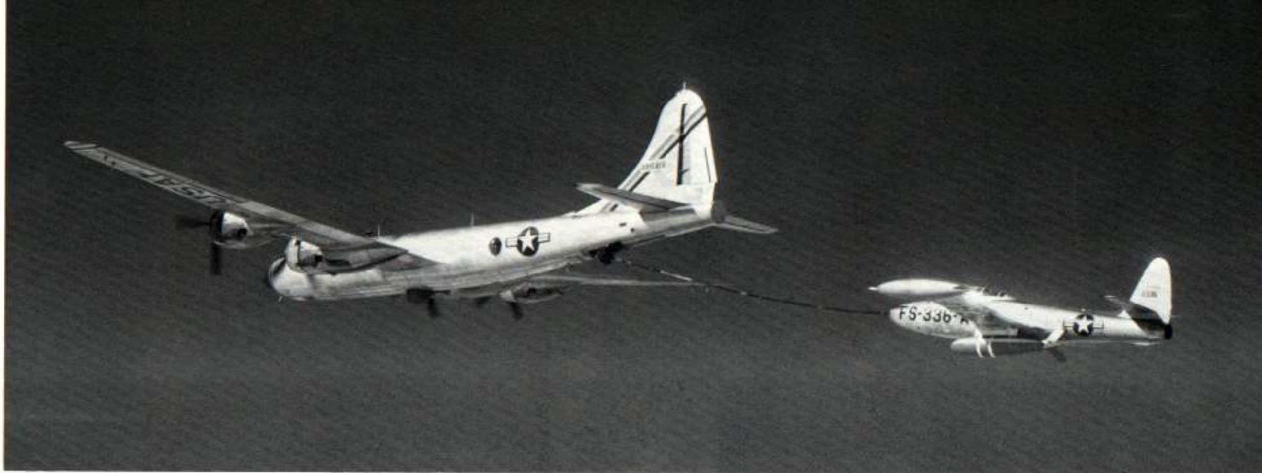
A 421st Air Refueling Squadron KC-97 tanker refuels a 49th FBGp F-84G carrying a practice Mark 7 nuclear bomb. Even though the F-84G was designed to accept the Boeing 'flying boom' method of inflight refueling, the aircraft of the Far East Air Force continued to use the 'probe and drogue' method due to the fact that no flying boom tanker aircraft were available in the Far East. The F-84G was the first fighter aircraft designed to carry nuclear weapons. (USAF via Menard)
