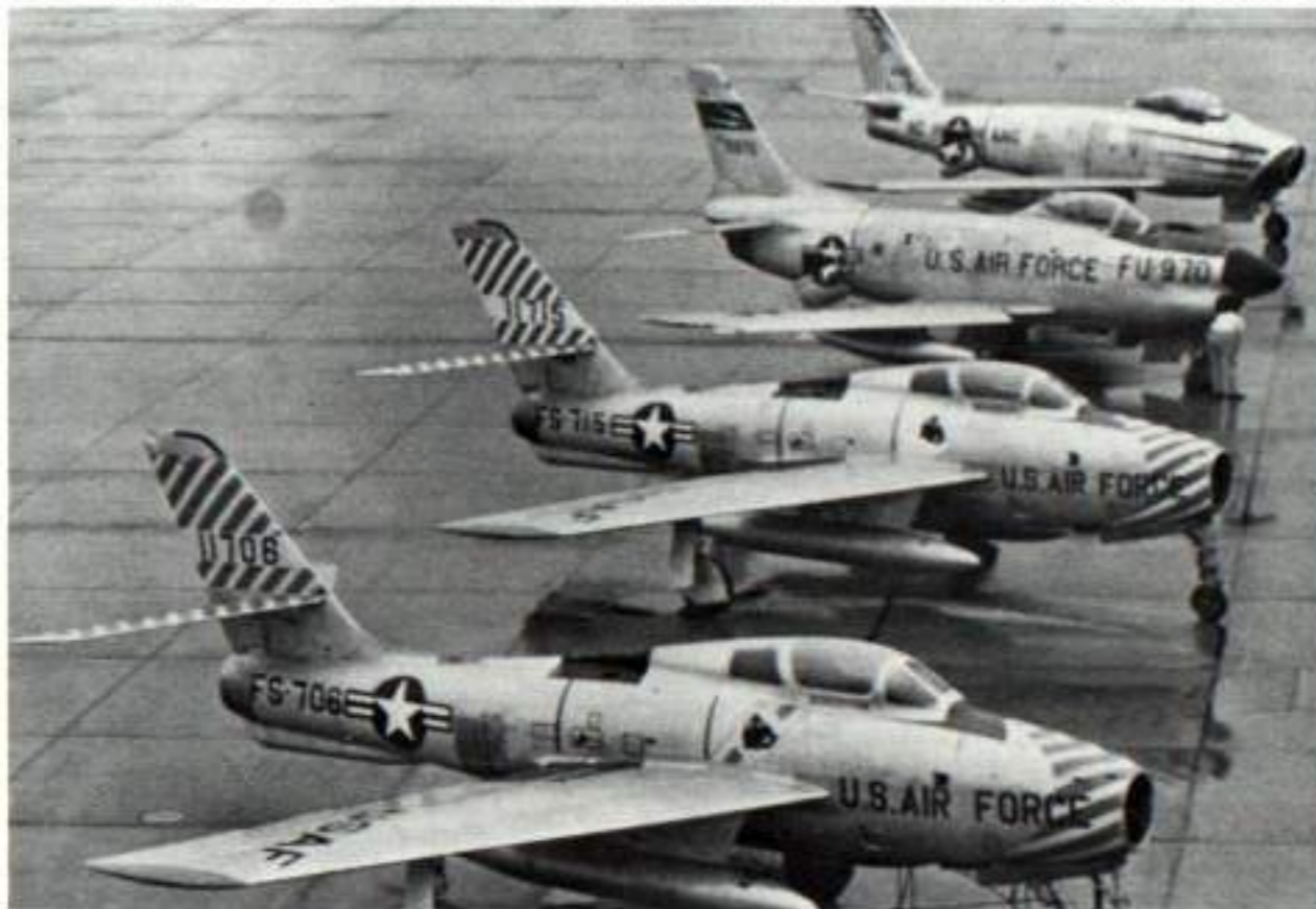
A pair of blue and white striped 390th FBSq, 366th FBWg F-84F-45s on the ramp at Alexandria AFB, Louisiana. The -45 model introduced the enlarged parachute housing under the tail. The 390th FBSq emblem under the canopy is a wild boar's head. (USAF via Menard)
