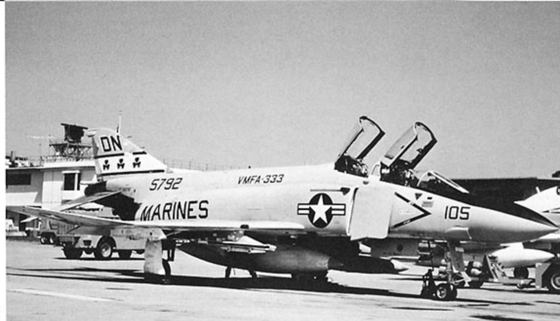
Later F-4Js had the addition of AN/APS-127 DECM antennas on the intake shoulders. These antennas are much shorter than those found on the F-4N. (Roth)
