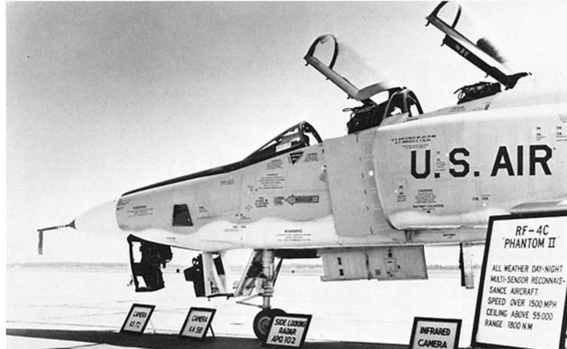
The Air Force developed the RF-4C Phantom II as a replacement for their RF-101 Voodoo fleet which suffered from a lack of speed. One of the most interesting new features found on the RF-4 was a side-looking terrain-mapping radar. (AFM)
