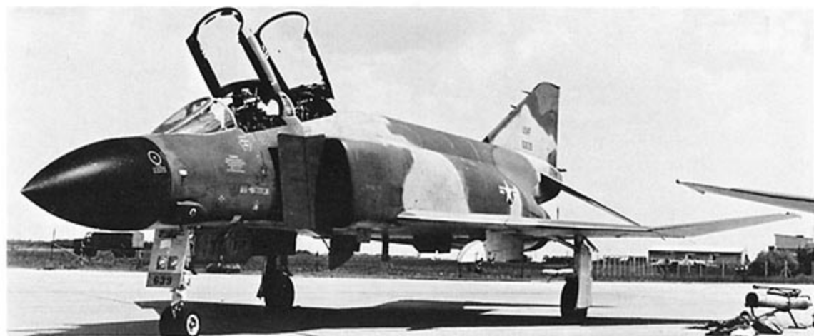
An early F-4D without the infra-red seeker housing beneath the nose. Later aircraft had the housing added but instead of the IR seeker, the housing contained RHAW antennas. This aircraft is from the 53rd TFSq, 36th TFWg based at Bitburg AB, Germany. (Hughes via Taylor)
