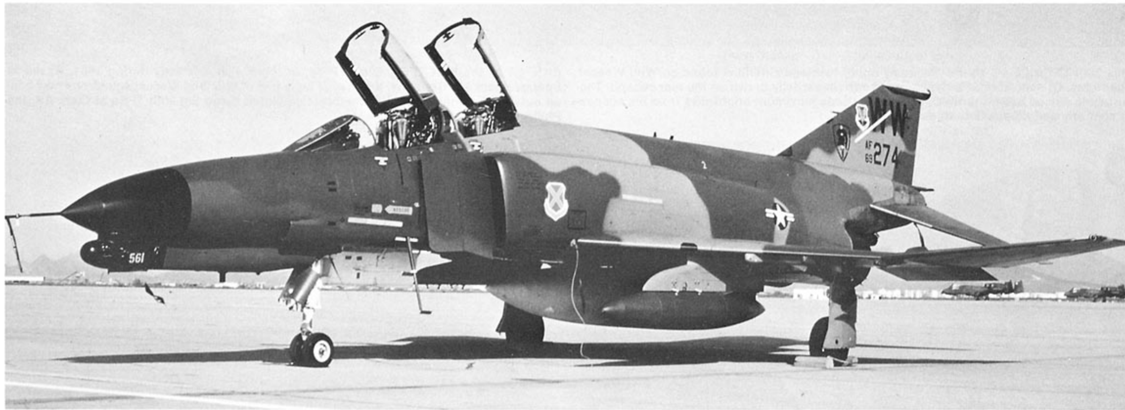
The APR-38 radome and antennas on an F-4G Wild Weasel 4 aircraft. (Knowles)
