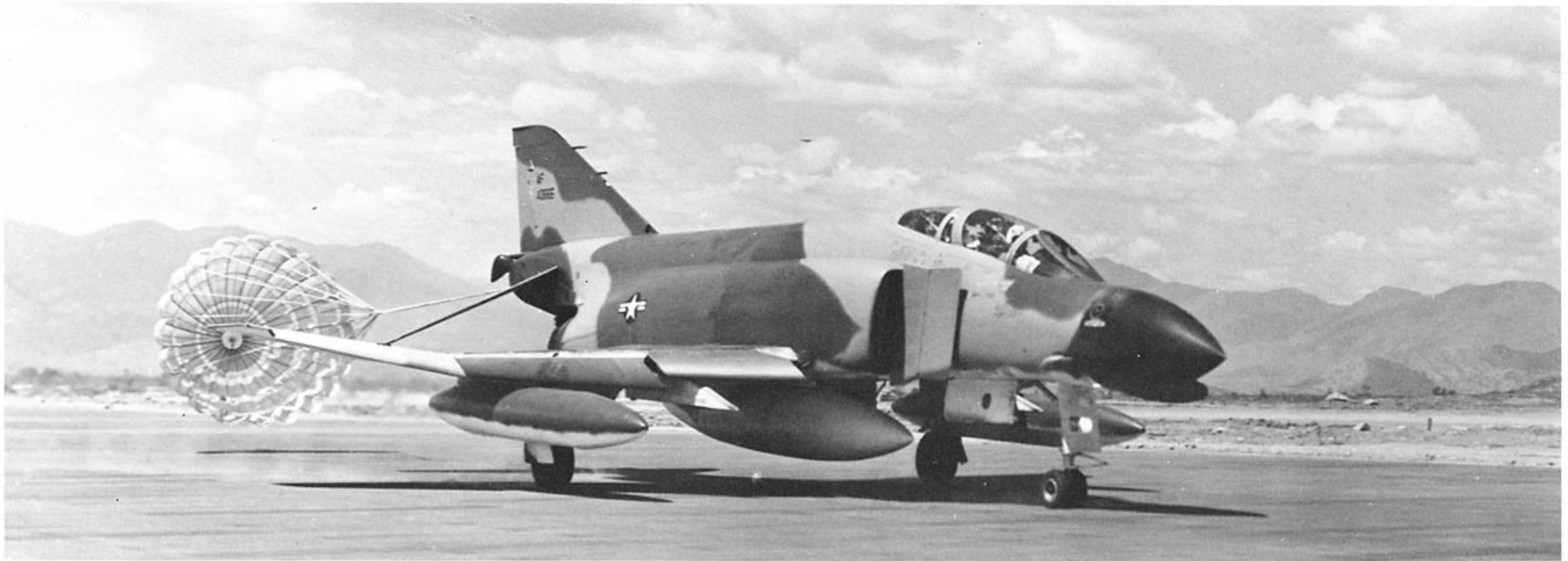
This F-4C of the 366th TFWg, landing at DaNang, carries the new Southeast Asia scheme. The three-section leading edge flaps are in the full down position. (USAF)
