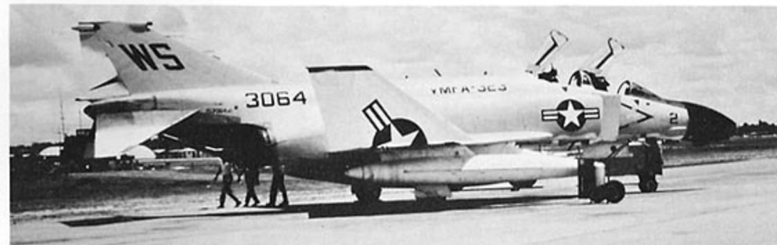
A Marine F-4B from VMFA-323 at Ubon RTAB in July, 1968. Marine F-4s were based in South Vietnam and flew mainly close support missions for "Mud Marines". Note the Fletcher-style wing tanks. (Piccirillo via Brewer)
