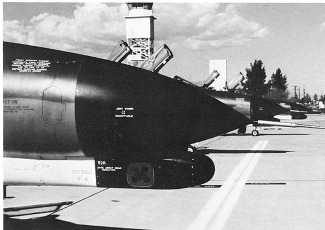
The APR-38 radome and antennas on an F-4G Wild Weasel 4 aircraft. (Knowles)
