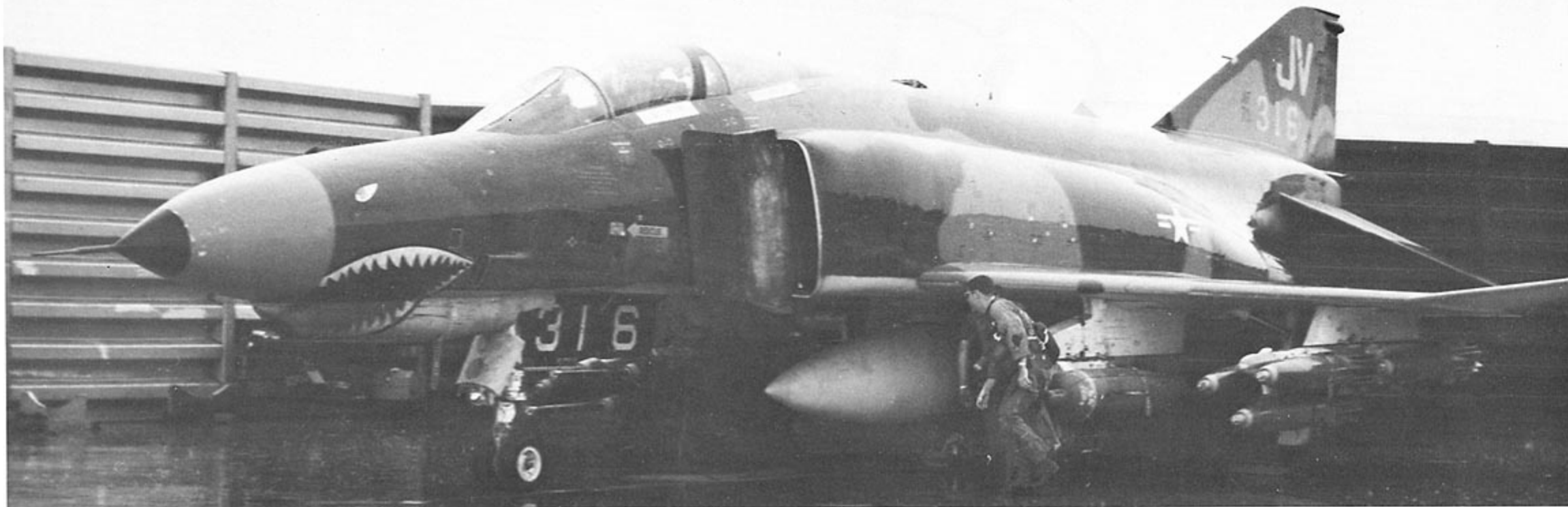
An F-4E from the 469th TFSq, 388th TFWg, at Korat RTAB. Each pylon carries a different store, which was not unusual for a mission in Vietnam. From the left to the right: Mk 84 2000-lb. bomb, three Mk 82 500-lb. bombs with 36-inch fuze extenders, 600-gallon centerline fuel tank, CBU-24B/B cluster bombs, and six Mk 82 500-lb. bombs fitted with Snakeye fins. (USAF)
