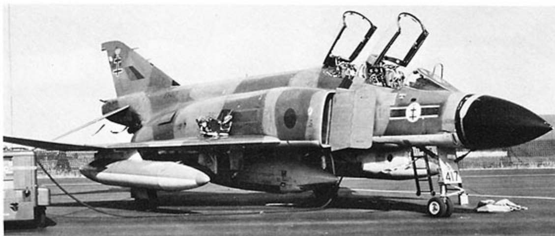
An RAF FGR-2 from No. 41 Squadron painted in the usual Northern Europe camouflage of Medium Green (34079), and Medium Sea Grey (36270) upper surfaces over Light Aircraft Grey (36357) undersurfaces. An EMI reconnaissance pod is being carried on the centerline station. Most NATO air forces, except for West Germany's RF-4Es, use some type of reconnaissance pod for intelligence-gathering missions. (Thomson via Brewer)
