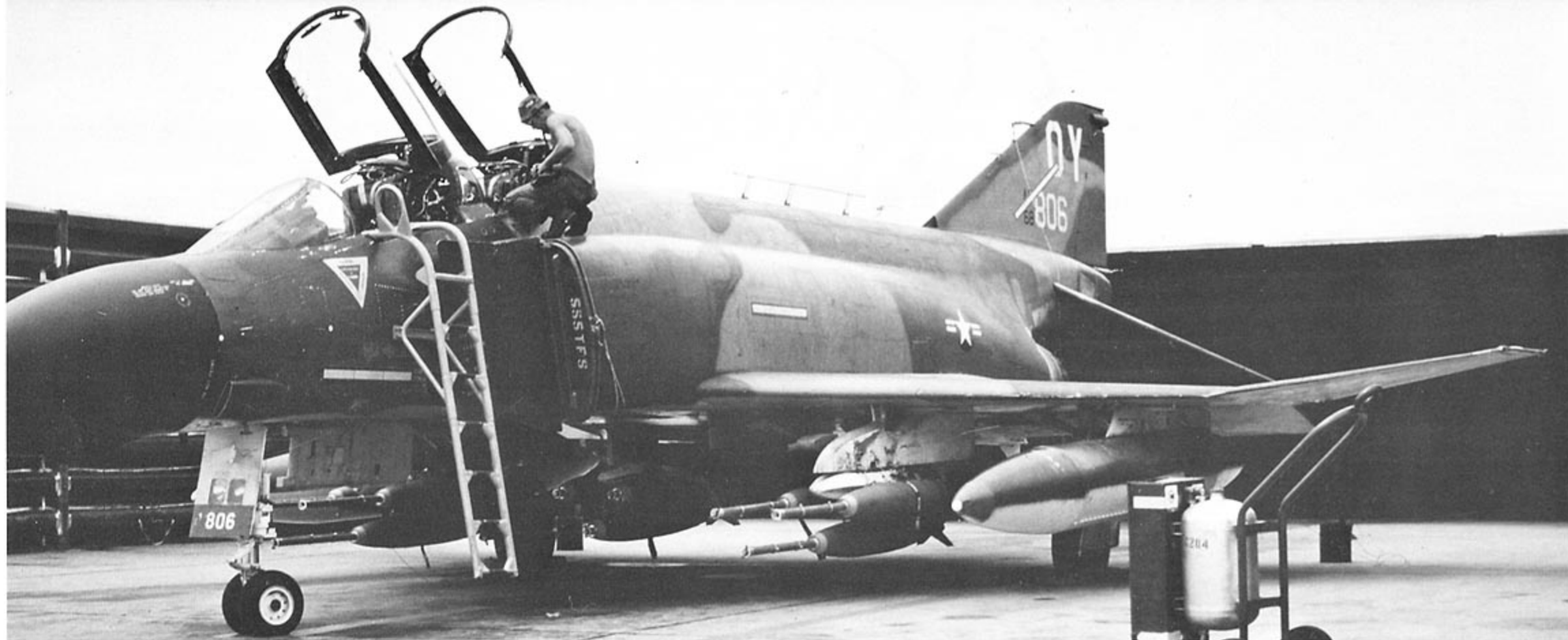
“Sex Machine”, F-4D serial 66-8806, from the 555th TFSq, 432nd TFRWg. The aircraft has had both the LORAN (LONG RANGE Navigational) radar antenna and formation tape lights added. These formation lights were screwed on and gave off an eerie, soft Yellow Green glow for night formation flying. It is carrying Mk 82 500-lb. bombs, both with and without 36-inch fuze extenders. (Larsen/Remington)
