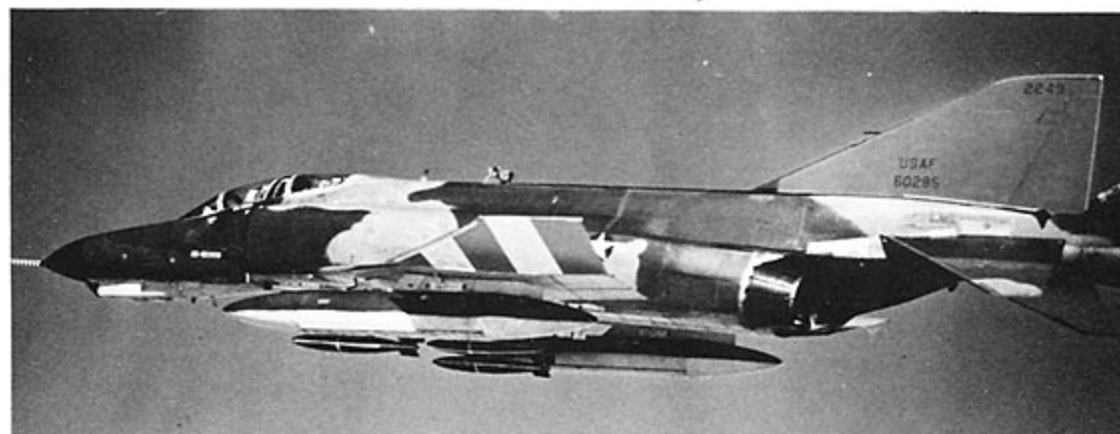
One of the first production F-4Es was used for spin tests. The large housing added to the aft fuselage area contains parachutes which are used to both create and control various spins to see how the aircraft will recover. (Brewer)
