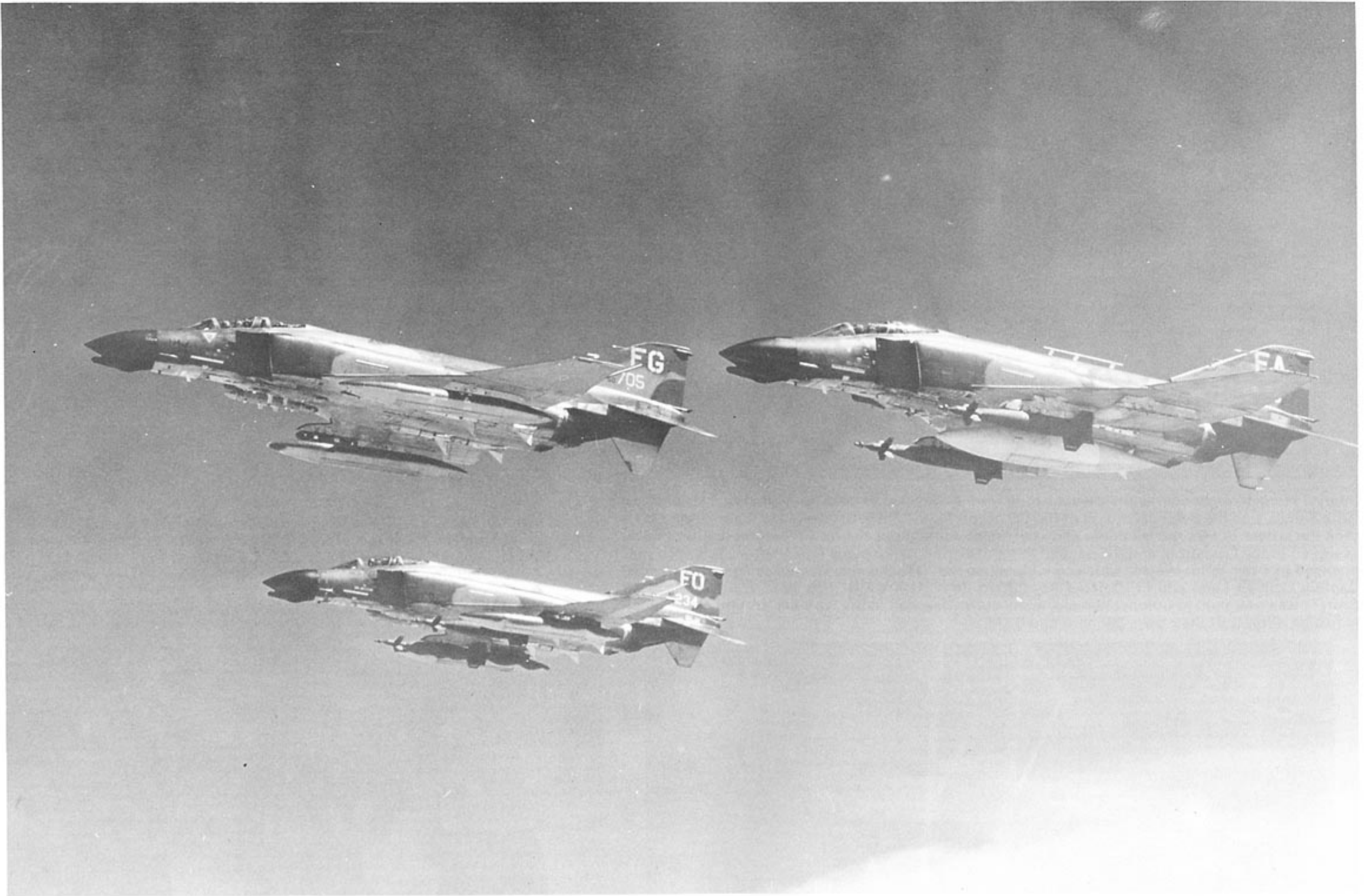
A trio of 8th TFWg F-4Ds on their way to hit an industrial target near Hanoi. All three are configured differently — FG-705 carries a guidance pod for smart weapons and a pair of ECM pods; FO-234 carries a pair of 2,000-lb. Mk 84 Pave Knife laser-guided bombs, ECM pods, and wing tanks, while the third aircraft again carries Mk 84 LGBs, but with a 600-gallon centerline fuel tank, and has the LORAN antenna fitted. (USAF)
