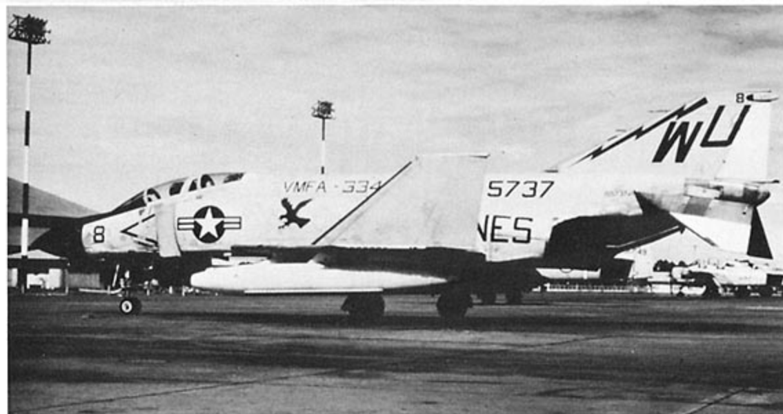
An F-4J from VMFA-334 "Falcons", based at DaNang, but seen on the Ubon ramp in 1969. The F-4J incorporated the Air Force bulged wing and updated J79-GE-10 engines, while retaining other standard Navy features such as the Probe and Drogue inflight refueling system. (Brewer)
