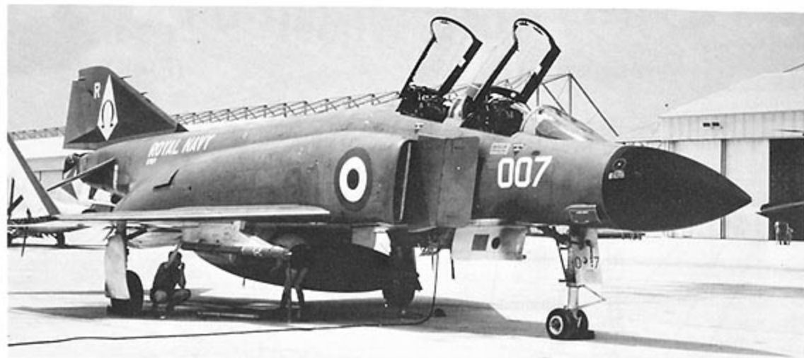
A Royal Navy FG-1 (F-4K) on the ramp at Cecil Field NAS, Florida, in July, 1971. The FG-1 differed from their RAF cousins, the FGR-2 (F-4M), in having a slotted stabilator and a greatly extendable nose gear leg to gain a better angle of attack during carrier take-offs. (Morris via Brewer)
