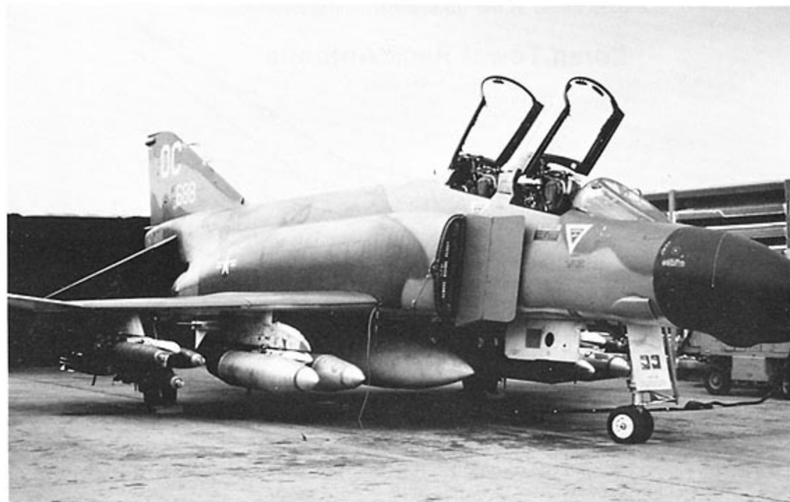
This 13th TFSq, 432 TFRWg F-4D is armed for a strike against a VC position in South Vietnam. On the outer pylons are Mk 82 Snakeeye bombs, while each of the inboard pylons carry dual napalm canisters. On strikes in South Vietnam, the forward missile bays carried neither ECM pods nor Sparrow missiles since the threat was very low. (Larsen)
