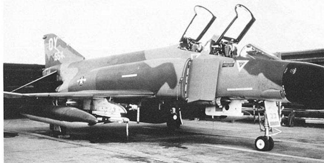
“Trapper John”, F-4D serial 66-7554, from the Triple Nickel Squadron. “Trapper” is armed with AIM-4 Falcon missiles — a rarity in Southeast Asia. (Foote)
