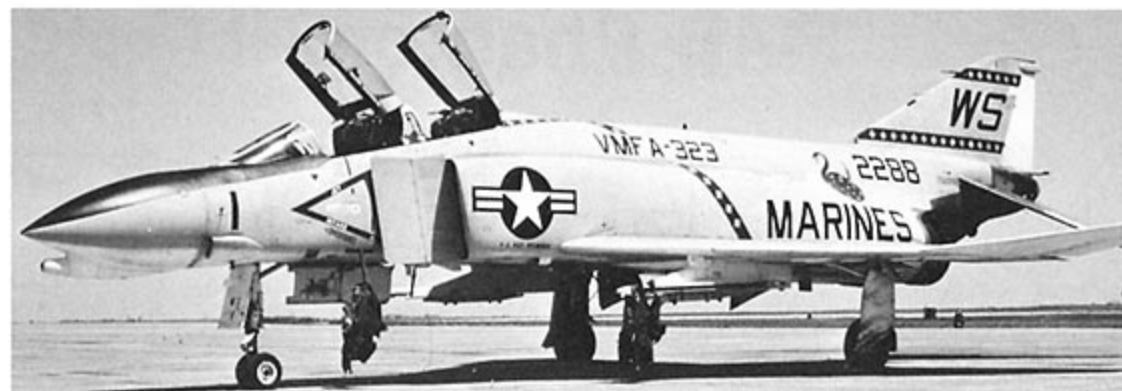
The F-4N was the result of Project BEE-LINE, a Navy program to update and rebuild the ageing F-4B fleet. Early F-4Ns, such as this example from VMFA-323 "Death Rattlers", did not have the AN/APS-127 DECM antennas on the intake shoulders. (Mills via Brewer)
