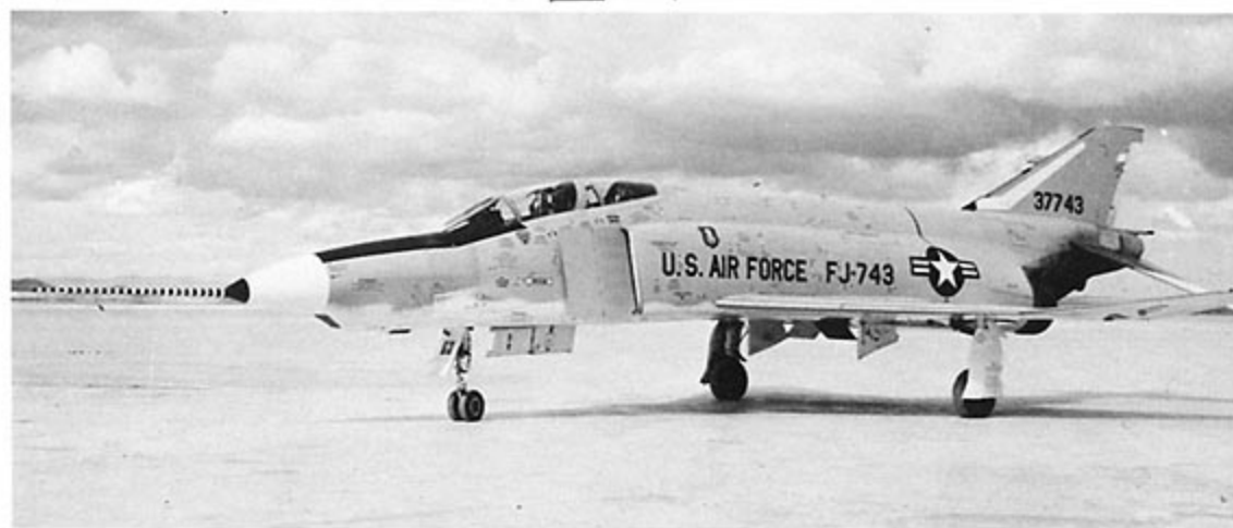
An early RF-4C from the Flight Test Center at Edwards AFB carries a long instrumentation test boom in the nose. The light-colored panel on the forward edge of the vertical fin is a shunt antenna panel. (USAF)
