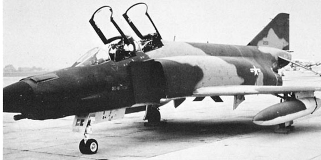
"Father of all Phantoms", 62-12200, after being modified to YF-4E prototype specifications and equipped with a 20mm M61-A1 Gatling cannon that fired through the forward camera bay opening. The air scoops atop the nose dissipated gun gases in the breech area. (Brewer)
