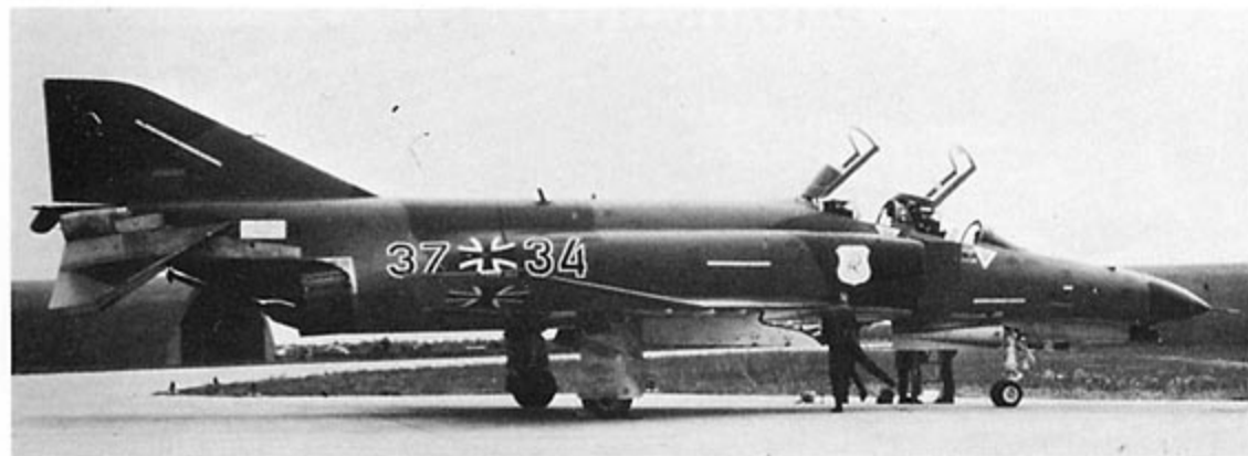
The lack of a slotted stabilator can be plainly seen on 37 + 34, the F-4F prototype. The aircraft belongs to JG 71 "Richtofen" which was the first operational F-4F unit in the West German Air Force. (Centurian Enterprise)
