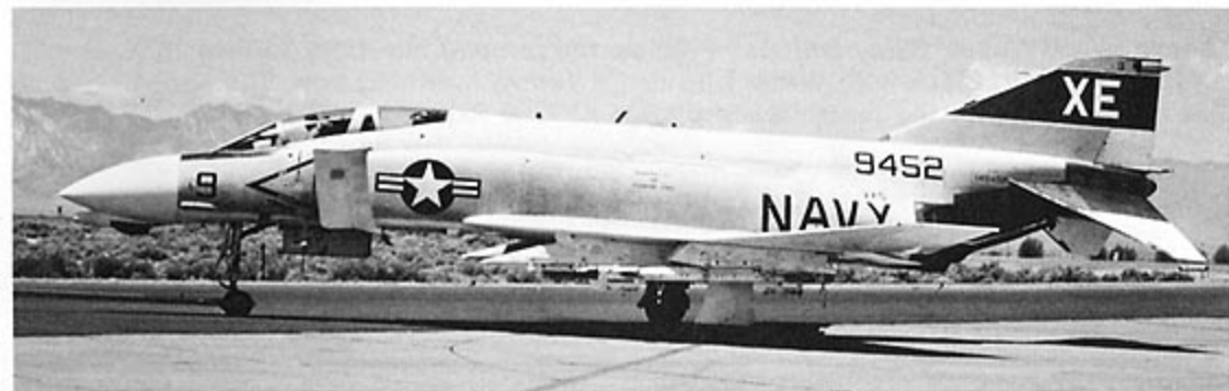
This F-4B from VX-5 at the China Lake Naval Weapons Center carries the revised infra-red seeker housing under the nose and the ECM fairing on the fincap, both of which housed APR-30 RHAWS antennas. The tail band is Kelly Green with White trim. (Lock via Brewer)
