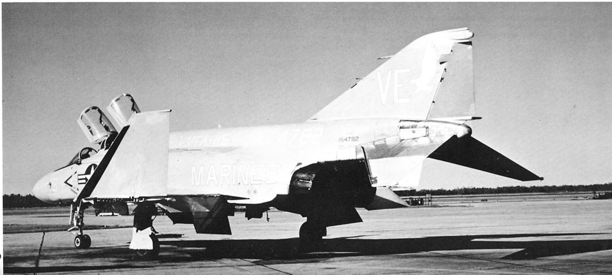
An early Marine attempt at subdued markings was seen on VMFA-115 "Silver Eagles" F-4Js. The aircraft were painted overall Gull Gray (36440) with all major lettering in White with a thin Black trim. This didn't work well since in the air the White letters became almost as distinct as the old Black letters. (JEM Slides)
