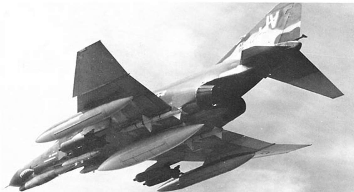
CBU-armed F-4E from the 469th TFSq at Korat. Northbound F-4E strike aircraft always carried two different ECM pods in the forward Sparrow bays. MiGCAP F-4s also carried ECM pods but were armed with a full load of AIM-9 Sidewinders. (USAF)
