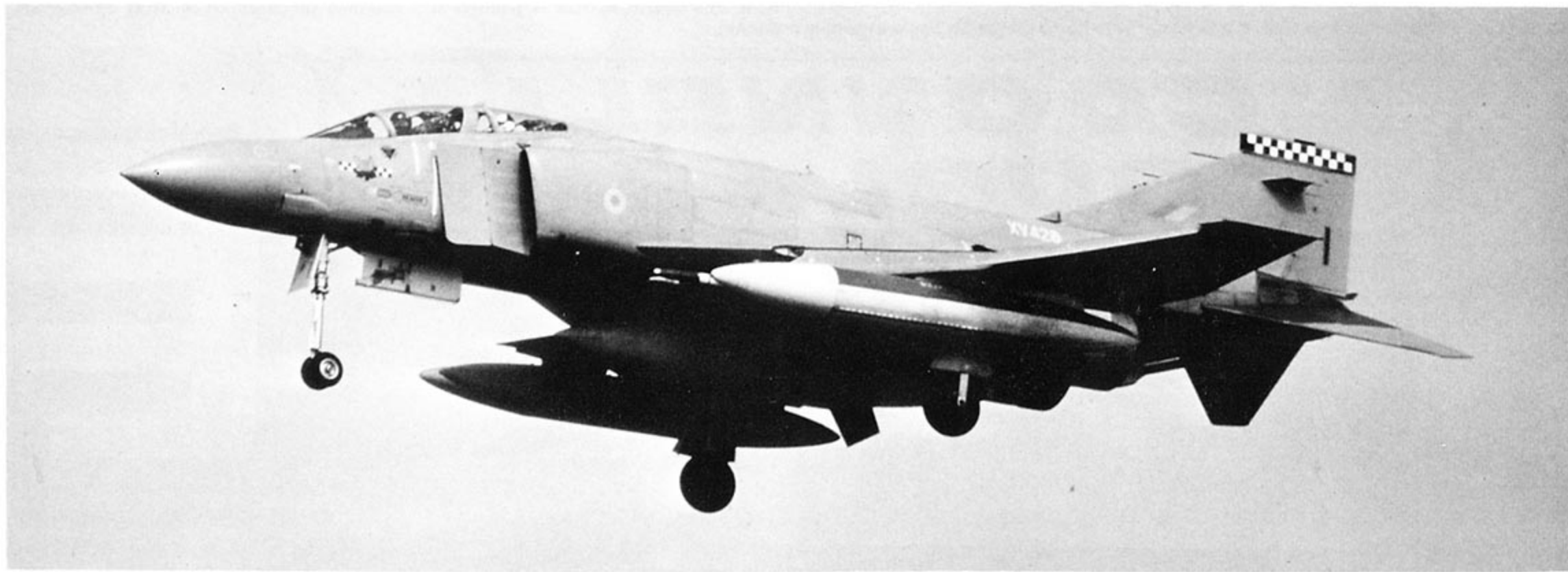
An RAF Phantom from No. 56 Squadron painted in the new Barley Grey camouflage scheme. All RAF Phantoms and other air superiority aircraft will be painted in this scheme. The Passive Warning Receiver (PWR) fairing can be seen at the top of the fin; the ILS blade antenna is on the side of the vertical fin. (JEM Slides)
