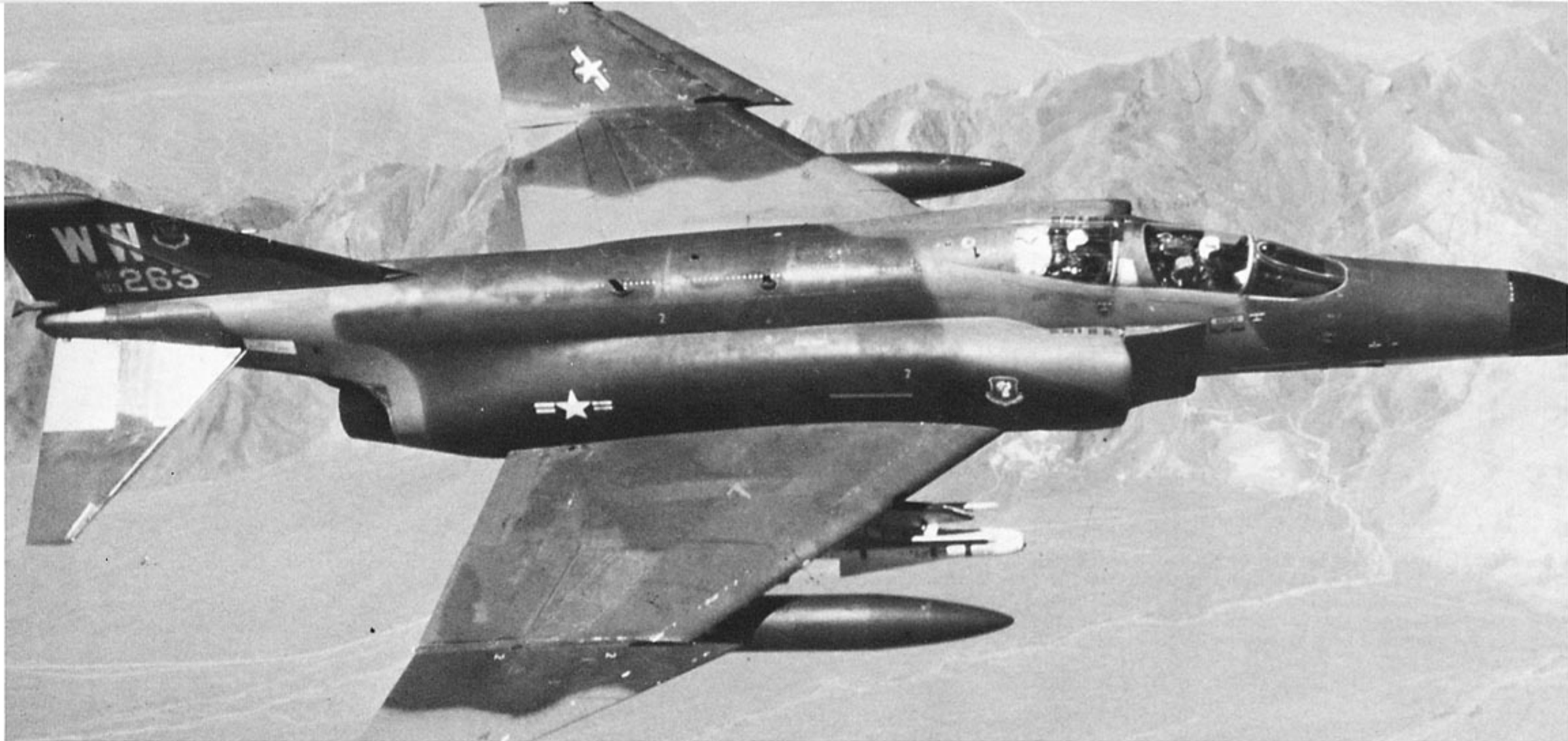
This 35th TFTWg F-4G shows the many upper fuselage antennas found on Wild Weasel Phantoms. Of special note is the blackout curtain partially drawn on the rear cockpit. The curtain is closed when the WSO, or "Bear", needs maximum brightness from his scopes to spot any and all possible threats. (USAF)
