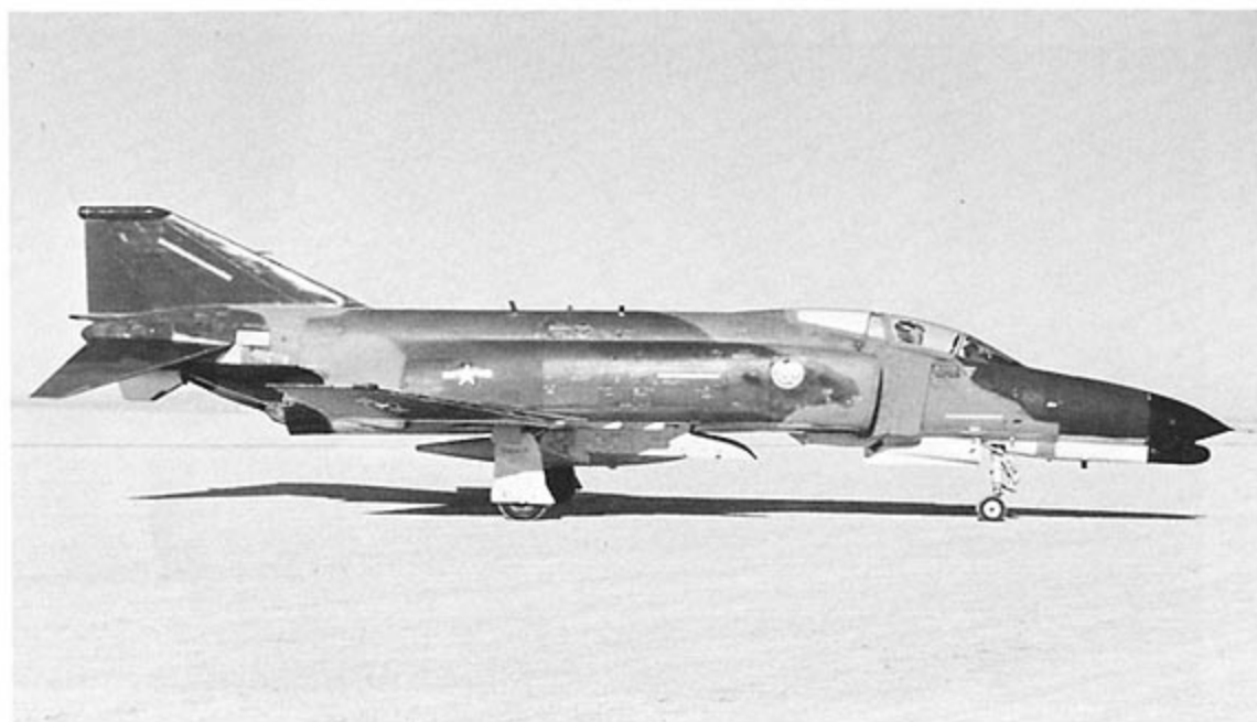
The F-4G Wild Weasel 4 prototype aircraft on the ramp at Edwards AFB. The F-4G was a development of the F-4E for use in the defense suppression role. The M61-A1 Gatling cannon was removed and various ECM systems, all part of APR-38, were installed in a redesigned nose bay and tail tip fairing. (Isham)
