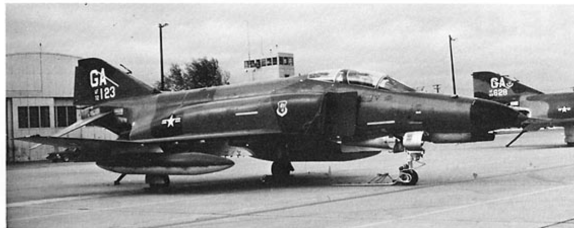
Another F-4F from the 20th TFTSg at George AFB. Note the open Gatling gun access door just in front of the nose gear. (Roth)
