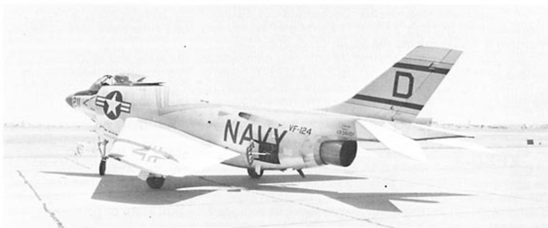
A McDonnell F3H-2N Demon of VF-124. There is a strong family resemblance to the eventual F4H-1 Phantom II design. (Krieger via Menard)
