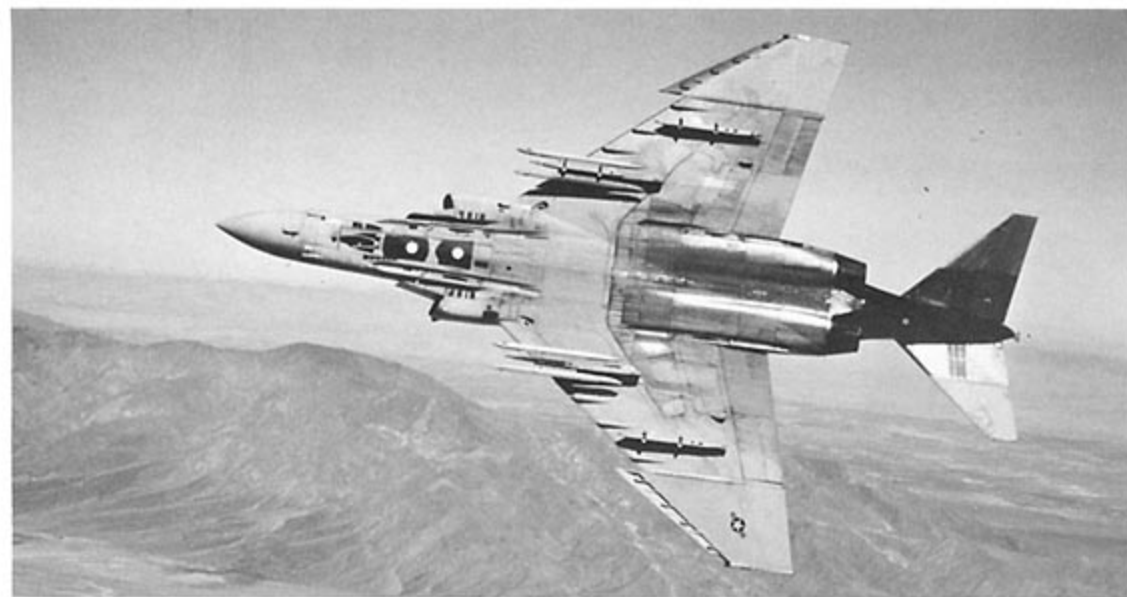
(Below) The Heater-Ferris camouflage colors are Dark Gray (35164), Medium Blue-Gray (35237), Light Aircraft Gray (36307), and Light Ghost Gray (36375) on both the upper and lower fuselages. Arrow on the tail is finely outlined in Red; all other markings are in Black. Gray schemes weather very rapidly, especially in desert climates, as evidenced by the fuselage sides. (Jacobs)
