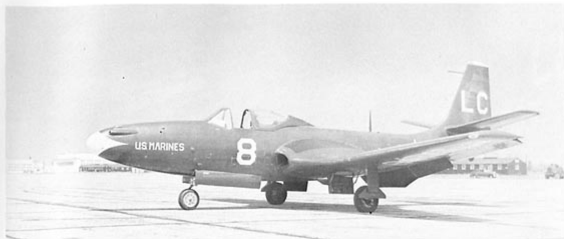
The McDonnell FH-1 Phantom was the Navy's first jet-powered carrier-based fighter. (W.J.Balogh)
