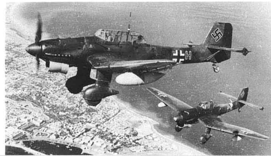
(Below) A pair of Ju 87R-2s of 2./St.G 3 returning from a patrol out into the Mediterranean in early 1941. The Med was a region in which the 'R' was repeatedly used against British convoys. Note the physical likeness between the R-2 and B-2. (Bundesarchiv)
