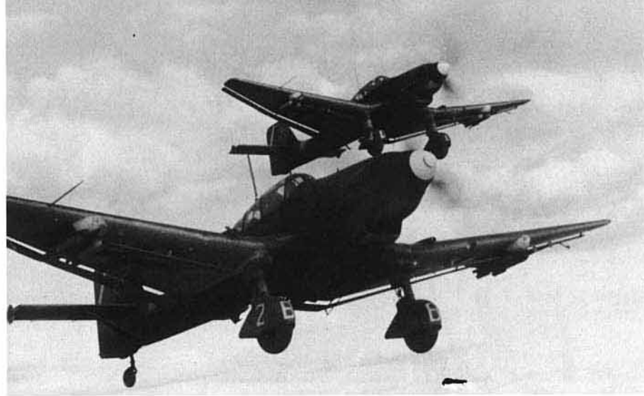
(Above) 'Dora-3s' enroute to the fateful Battle of the Kursk salient, where the Stuka reached its eclipse as an effective dive-bomber and the Third Reich reached its eclipse in its last great armored offensive. With its days as a 'terror weapon' passed, the Ju 87 gradually dispensed with the propellor sirens, the mounting pods being totally eliminated on late production Ju 87D-3s as seen on the second aircraft. (Bundesarchiv)
