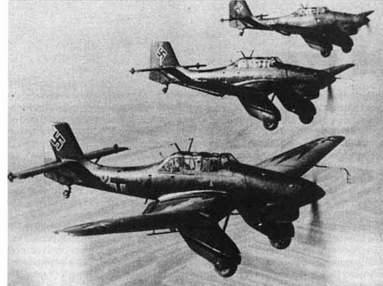
(Above) A trio of Ju 87A-2s serving with St.G 165 in 1938, displaying a not-uncommon variety of camouflage finishes — usually obtained by switching the basic colors and splinter pattern. The Red tail banner and White circle behind the swastika were soon eliminated on operational aircraft. The fuselage code on the nearest aircraft is 52+C24. (Zdenek Titz)
