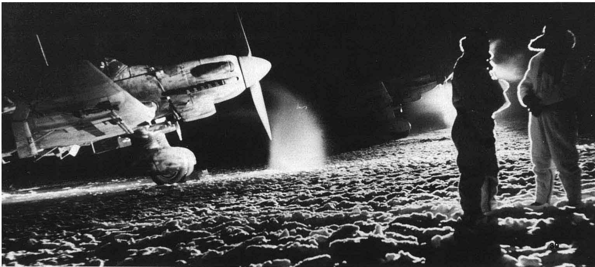
(Below) This atmospheric pre-dawn scene may look attractive, but the harsh Russian winters were incredibly brutal to both men and machines. Day after day sub-zero temperatures froze oil and fuel lines and cracked propeller blades — problems which were only partially solved with heating tents over the Stukas' cowlings. Another hazard was the deep hatred that Soviet troops had for both the Stuka and its air crews, making the prospect of bailout behind enemy lines almost unthinkable. (Bundesarchiv)
