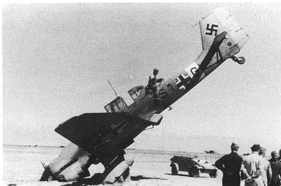
(Below) While taxiing out for a mission, S1+GK of 2./St.G 3 suffered a Kopfstand (headstand), which was one of the less fortunate traits of the somewhat nose-heavy Ju 87. When landing, Stuka pilots were advised to make a three-point touch down whenever possible. Overall Sand-Yellow uppersurfaces were not unusual on early desert aircraft of St.G 3. (Bundesarchiv)
