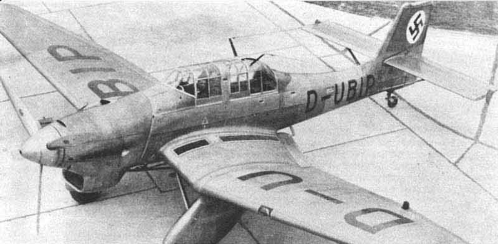
(Above) The Ju 87V-4 in its original form, with smooth cowling side panels and before the rearmost canopy windows have been installed. (Zdenek Titz)
