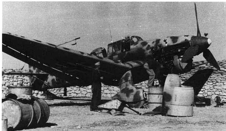
(Below) By the spring of 1942 St.G 3 had absorbed I/St.G 1 as its second gruppe and II/St.G 2 as its third gruppe. The revised 'S7' Geschwader code of St.G 3 replaced the 'A5' Geschwader code on the fuselage of St.G 1 aircraft, but the gruppe continued using its diving crow emblem throughout the remainder of the desert war. The pilot's belly viewing-window structure has been removed and can be seen in the foreground with the upper adjustment handle projecting to the right. (Bundesarchiv)
