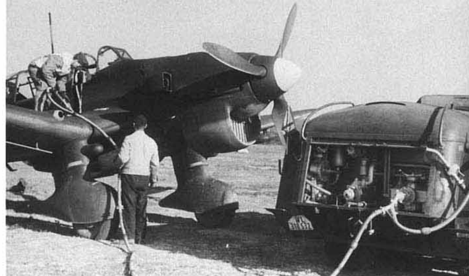
(Above) L1+DW takes on fuel in its starboard wing root tank, the rubber bumpers on the hose helps to prevent paint from being scraped off the wings. Again, small Sand Yellow patches are visible, as well as a tropical supercharger air intake dust filter on the cowling. Undersurfaces are probably desert Light Blue (78). (ECP Armees)
