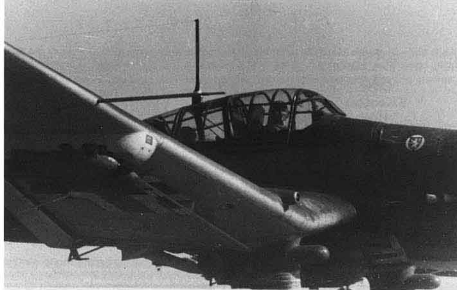
(Above) The greenhouse of the 'D' series was more rounded in both profile and cross section than the 'B' series. The 'Dora's' redesigned canopy also afforded the pilot substantially more armor protection with his seat-mounted headrest and the overturn plating (just visible at the front of the center canopy section). On all variants of the Stuka from the Ju 87B onward nearly half the canopy framework was on the inside of the plexiglass. (Bundesarchiv)
