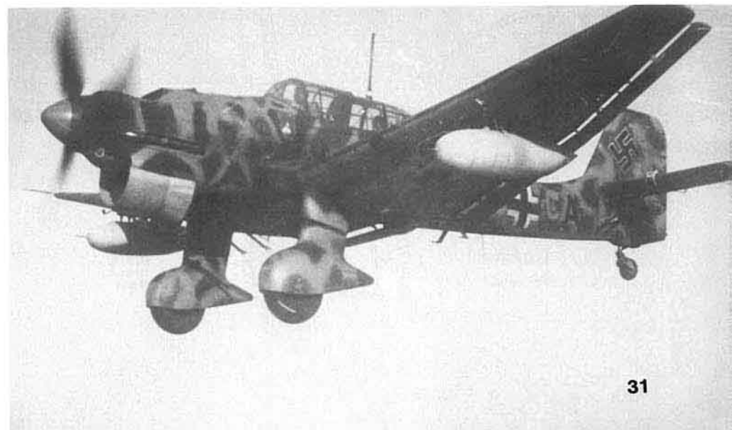
(Below) 2F+CA, a Ju 87 R-2/Trop with Sand Yellow sprayed over the splinter Green upper surface. With desert 'R's flying increasingly short-range missions against British forces, the 300 liter tanks became less frequently used. Beneath the aft fuselage is the antenna for the FuG 25 IFF radio, and the plexiglass bubble of the Peil G.IV D/F aerial is just visible between the inboard flaps. (Smithsonian Institution)
