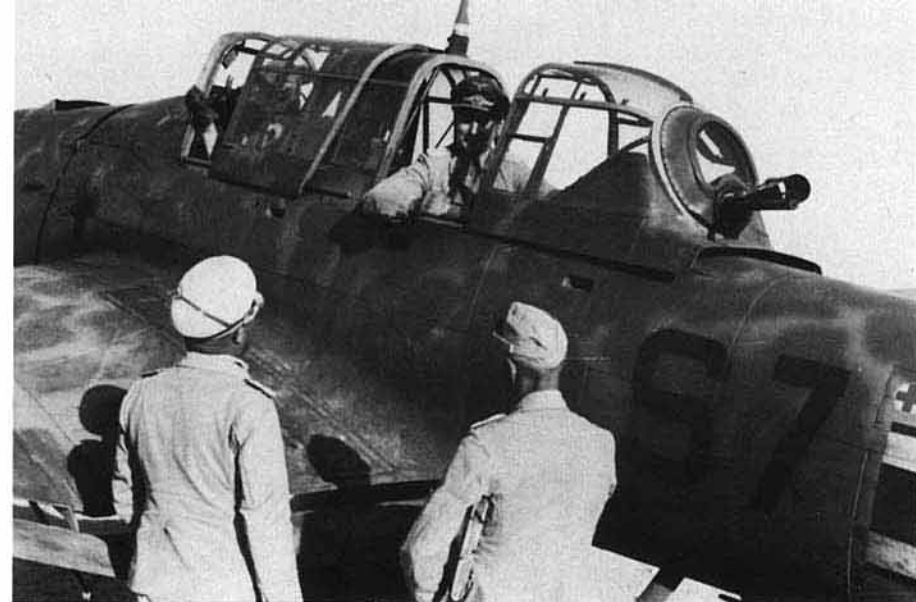
(Above) Luftwaffe officers chat beside a Ju 87B-2/Trop of St.G 3 after a meeting with Field Marshal Albert Kesselring at El Adem on 19 June 1942. The gunner's position is equipped with an armored gun mount of the type more commonly associated with the upper rear defensive positions of the Ju 88. This same rear gun installation was found on Ju 87Bs and Rs serving on other fronts, and may have been a late factory fitting. The gun is complete with a sun shade over the gunsight. (Bundesarchiv)
