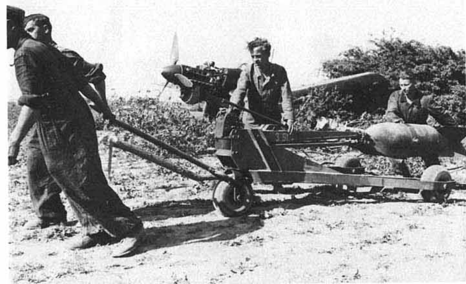
(Above) France 1940. Armorers manhandle one of the ubiquitous three-wheeled loading carts which were used to lift bombs into position beneath aircraft. The small inscription '3. St.' on the arm of the cradle indicates that it is the property of 3./Stukageschwader 2. (Bundesarchiv)
