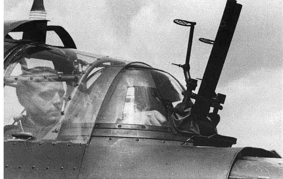
(Above) The half-bowl shaped GSL-K 81Z turret rotated beneath the open end of the sloping rear gunner's canopy, its armor plating being integrally mounted in the turret. To avoid damage to the twin MG 81Z and its ammunition links, the guns could be held in position when the rear canopy was slid open — unlike the arrangement of the Ju 87B/R where the MG 15 travelled with the gun mount. The MG 81Z also featured VE 22 and later VE 42 twin sights. (Bundesarchiv)
