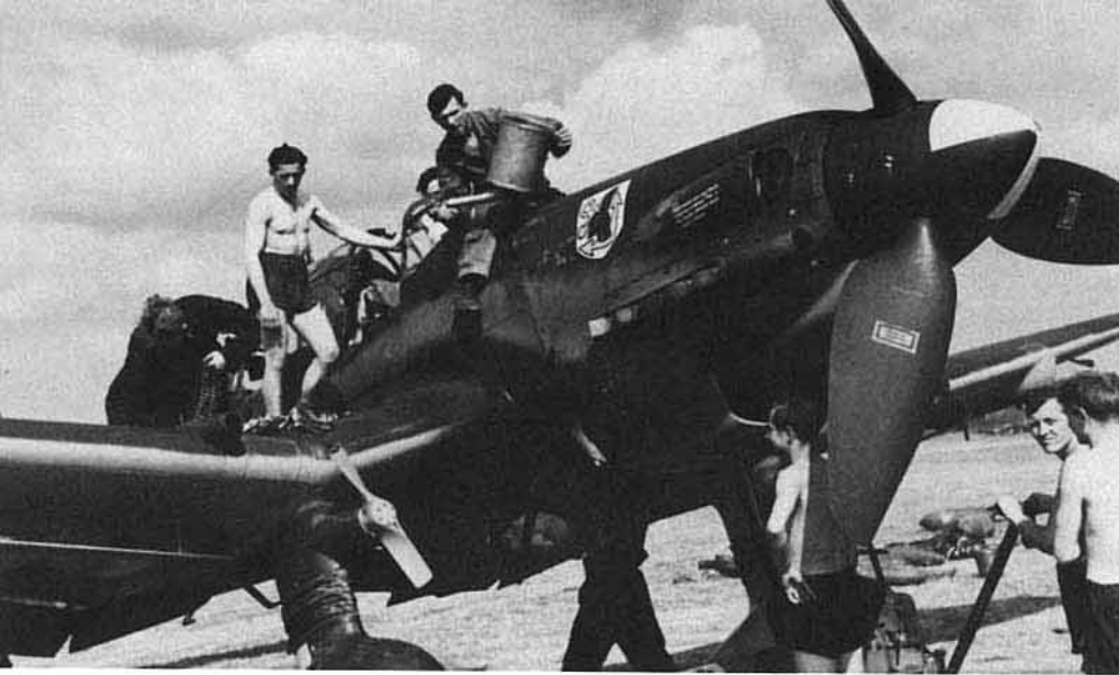
(Above) Even with its aerodynamic redesign, the 'Dora' was still an ominous-looking beast. The starboard supercharger intake now included a closable flap at its mouth. The new undercarriage legs were rather fragile looking in comparison to those of the earlier 'Berta', especially when considering the loads that the 'Dora' handled! (Bundesarchiv)
