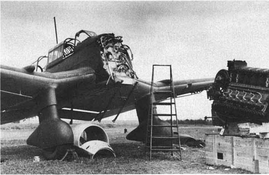
(Above) While having its engine changed this Ju 87B-1 exposes its firewall plumbing and the sturdy support box of the swinging bomb rack. The engine side of the firewall has been left unpainted natural metal, (rather than being painted RLM Gray (02), which was the usual practice with German aircraft. Total Ju 87 motor replacement could be quickly accomplished with simple hoisting gear, making the Ju 87 extremely popular with front line mechanics. (Bundesarchiv)
