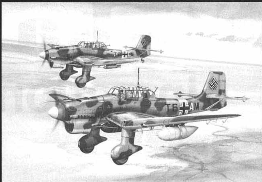
Ju 87R-2/Trops of 4./Stukageschwader 2 on patrol against British positions in North Africa during autumn of 1941. Like many early desert campaign Stukas, these aircraft have had Sand Yellow applied over their upper surface European splinter camouflage. Stukas would later be delivered to North Africa in official factory applied desert colors.
