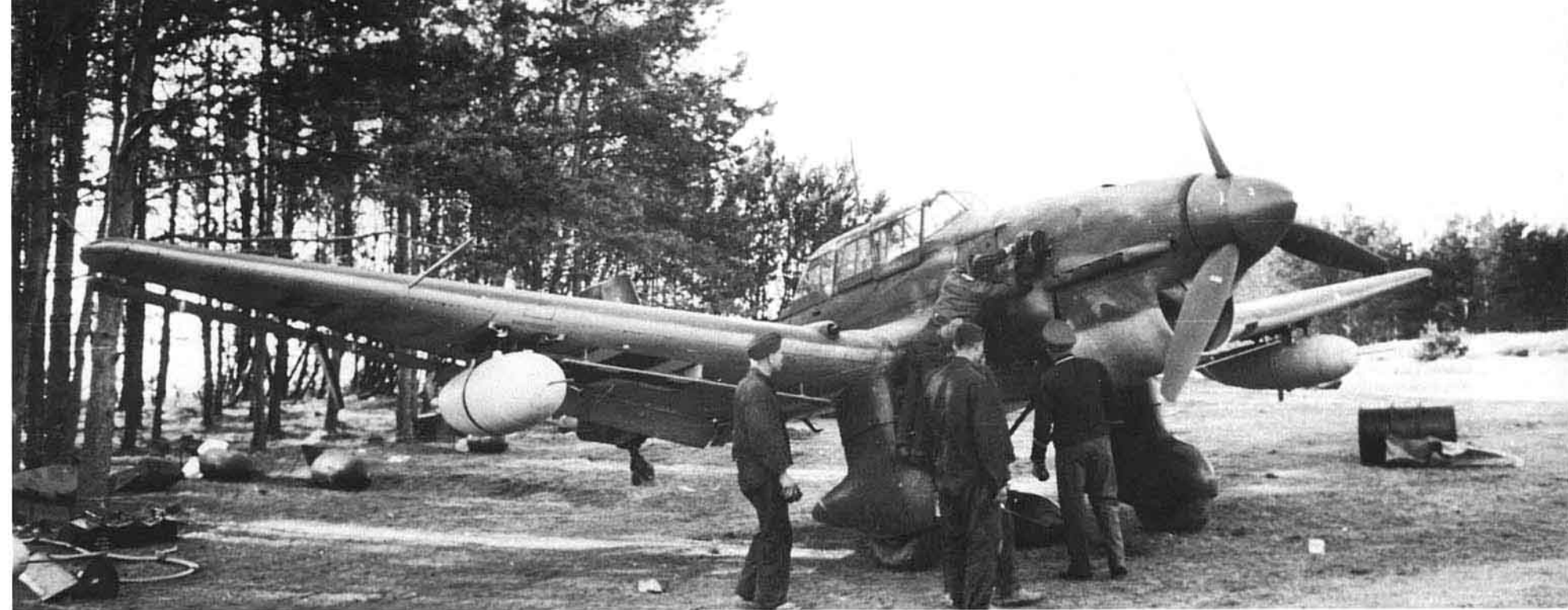
(Above) Without its underwing tanks the Ju 87R was essentially a Ju 87B, and with its tanks the Ju 87R was essentially a long-range Ju 87B. When not carrying its tanks, a full bombload could be carried by the Ju 87R with only minor revision to the ETC 50 wing racks. This red-spinnered Ju 87R-1 (A5+HK) of St.G 1 carries the White, Yellow and Black 'diving crow' emblem of I gruppe on the upper cowling. (Bundesarchiv)
