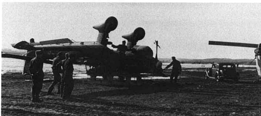
(Below) This damaged Norwegian based Ju 87B-2 is loaded onto a wooden sled to be towed back to base for repairs. Perhaps with an eye toward trying to prevent this type of mishap, the forward coverings had been removed from the undercarriages, however, soft earth, sand or mud could still cause the nose heavy Stuka to flip over. The compressed wood VS-11 propeller blades have sheared off. (Bundesarchiv)
