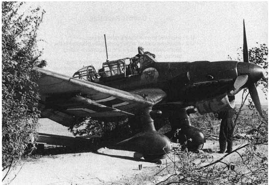
(Right) Partially concealed with foliage, a B-1 of 3./St.G 2 is prepared for crank-up during the Battle of Britain. Having seen its fair share of combat, T6+HL has become typically grubby and has had areas of repair hastily spot painted. The Junkers Jumo 211 A, not the cleanest of powerplants, has deposited heavy exhaust stains along the entire length of the fuselage. (Bundesarchiv)
