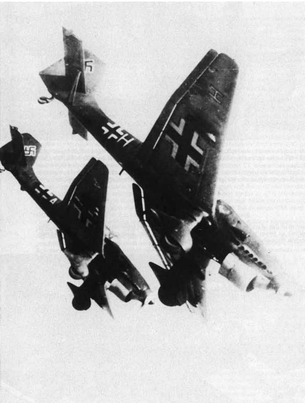
(Above) The low contrast between Black Green (70) and Dark Green (71) led to the misconception that the uppersurfaces of Stukas were routinely painted overall Black Green, the two-tone splinter scheme of 70/71 was the standard factory finish. Staffel colors were the most frequently used additional 'in service markings'; T6+GM of 7./St.G 2 is trimmed in White, while the spinner tip of the 8. Staffel aircraft in the background is Red. Occasionally, however, Gruppe colors were employed instead. (Bundesarchiv)
