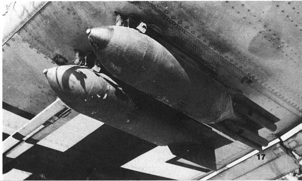
(Below) A pair of underwing SC 50 (110 pound) bombs, with whistles attached to their fins also served as terror weapons. The addition of whistles was a modification made to German bombs throughout the war. (Bundesarchiv)
