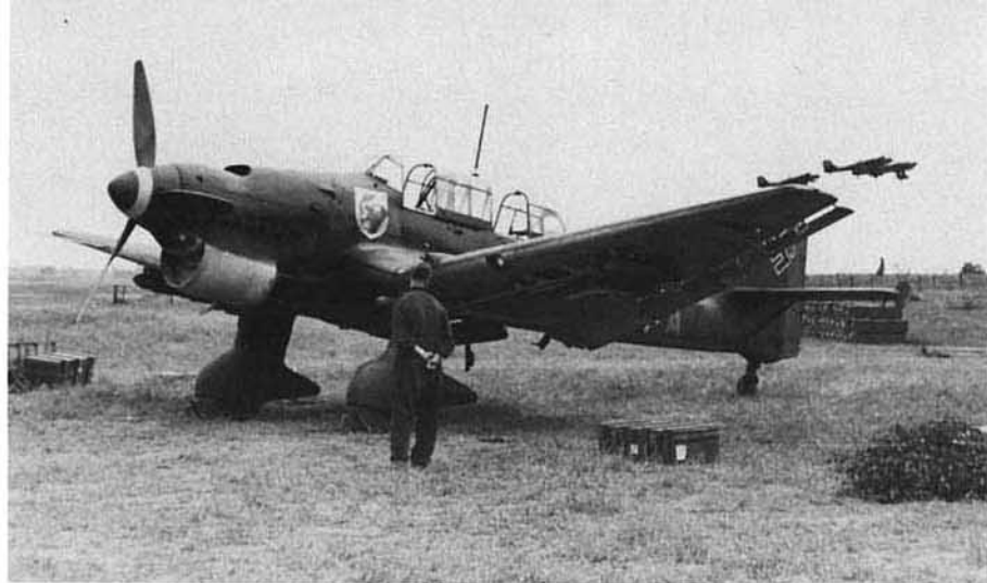
(Above) 6G+AT of III/Stukageschwader 51 (later redesignated II/St.G 1) sits fully loaded and ready on a French field during the Blitzkrieg in the west during 1940. During these campaigns Ju 87 units made increasing use of the wind-driven undercarriage mounted sirens to terrorize their adversaries. This machine carries a siren-propeller mounted on the starboard undercarriage only, the port mounting is faired over. Such combinations were not unusual. (Bundesarchiv)
