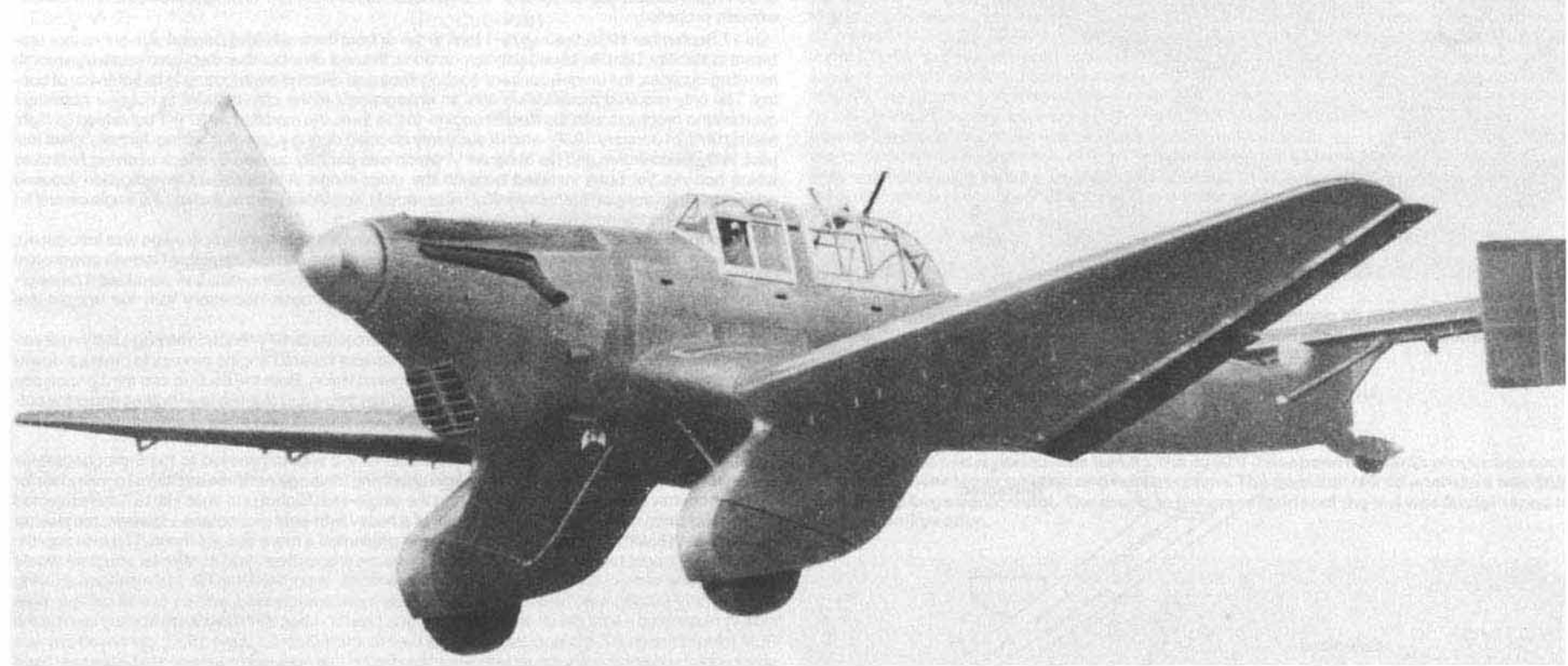
(Above) The first prototype Ju 87V-1 with the early shallow radiator bath and original twin tail assembly inherited from the Junkers K-47. (Zdenek Titz)
