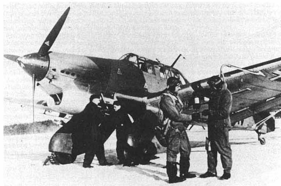
(Below) A pair of Stukafliieger (Stuka pilots) pose in front of their aircraft as the 'blackmen' prepare to crank up the inertia-starter of the Jumo 210 engine. The drooping pitot boom and radiator intake braces were unique to the 'A' series. Also unique to the 'A' series were the greenhouse mounted 'devil's horns' radio masts, antenna wires ran from their tips to the tips of the horizontal tailplanes.
