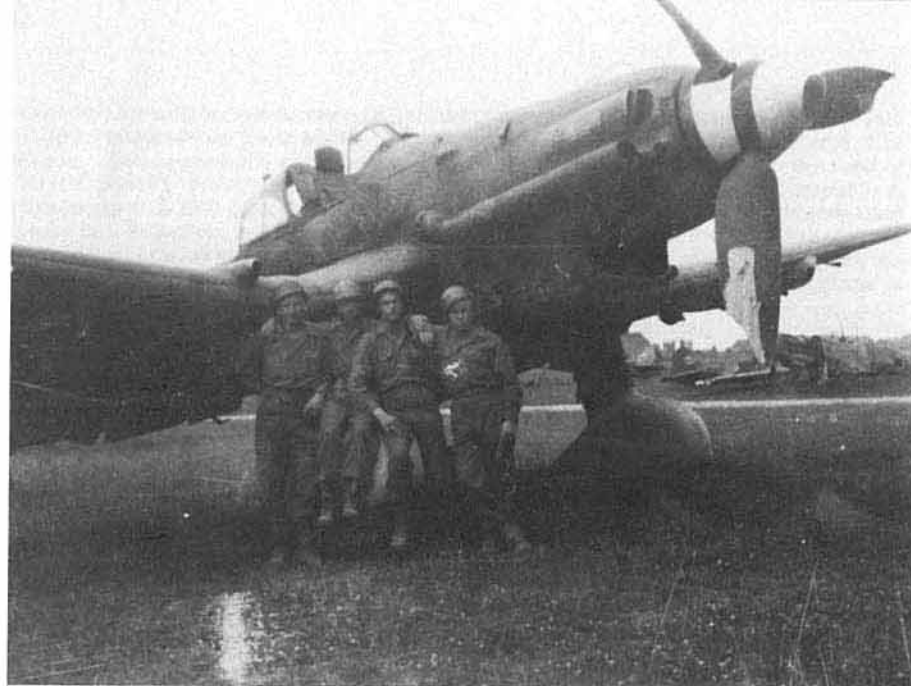
(Above) Germany, 1945. Victorious G I's pose with a short-span Ju 87D-7 (converted D-3) which has had its wooden propeller blades blown off to prevent unauthorized use. The late-war modified windshield is detectable by its flat forward panels and extra braces. The 'spiral-schnauze' spinner was commonplace with aerial-assault units during the last year of the war.
