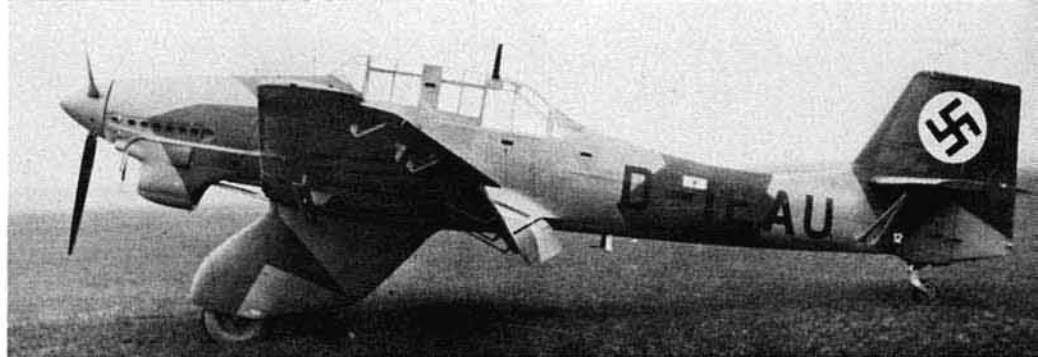
(Above) The twelfth production Ju 87A-1, D-IEAU, typifies the bulky but rakish profile of the 'Anton' series. The four-color camouflage of Dark Brown (61), Green (62), and Green Gray (63) splinter, over Light Blue (65) undersurfaces was the standard scheme of the period. Once the aircraft was in service, the 'civil registry' factory code was replaced by Luftwaffe unit codes and national insignia. The White rectangle on the mid-fuselage is actually light reflecting off the plexiglass first aid panel — a feature found on all Ju 87s, but which was often painted over. (US Air Force)
