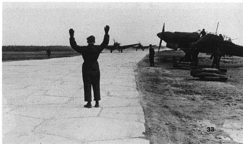
(Below) Open fields or roadways were all the same to the Stuka as it leapfrogged behind the ever-moving Wehrmacht. The stacked SC 50 bombs have been staggered in their piles to prevent damage to the percussion detonators while they await loading. The extended fuses were used to detonate the bombs above ground, scattering shrapnel amongst Soviet troops. (Bundesarchiv)
