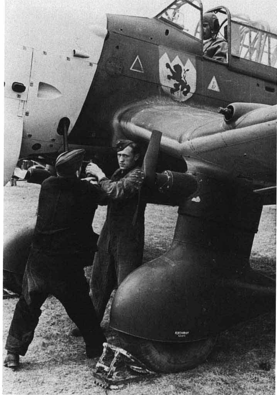
(Above) The undercarriage siren, cowl, and stencil markings can be appreciated here, including the small manufacturer's data plate just forward of the wing root. The Yellow, Red and Black shield of Stab/II/St.G 77, which saw action in the Balkans and Mediterranean during the early months of 1941, is carried below the windscreen. (Bundesarchiv)
