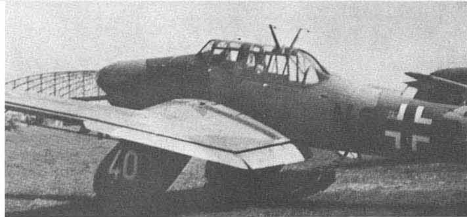
(Above) Like many training 'Antons', NG+RH has been stripped of its rear armament and has been assigned an additional number in White on its undercarriage trousers. Perhaps the greatest service performed by the underpowered Ju 87A was the preparation of young pilots for the rigors of combat, many Ju 87As survived in this capacity until well into the war.
