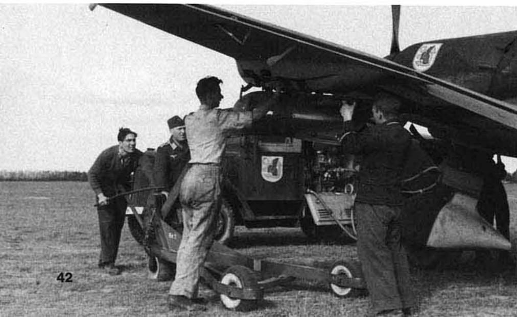
(Below) The groundcrew of 7./St.G 1 use a three wheeled bomb loader to attach an SC 250 bomb into position on the faired underwing bomb rack; the side-mounted ETC 50/VIII racks accommodated lighter loads. Light Blue (65) on the rear spat coverings was an effort to better 'sky camouflage' the Ju 87 when viewed from below — a practice which became more common on later nocturnal-assault Stukas. The placement of unit emblems on Luftwaffe vehicles was a common practice; in this instance on an Opel fuel truck. (Bundesarchiv)
