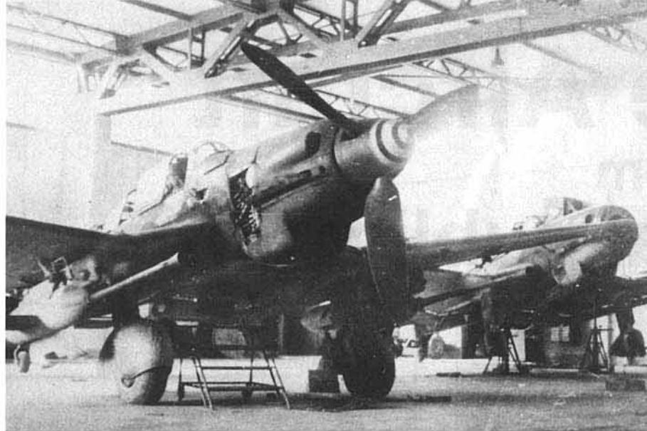
(Above) An abandoned Ju 87G-2 shares a hangar with a cannibalized Ju 87D-5, the 'Gustav' apparently having suffered light damage below the pilot's windscreen. Scattered groups of ground-attack and tankbuster Stukas vainly harassed the advancing Allies in the East and West during the last days of the war. On the 'Dora' at right can be seen the remnants of a Yellow undercowling, which was a wide spread variation of late war tactical markings, and was also to be found on some 'Gustavs'. (Richard F. Grant)
