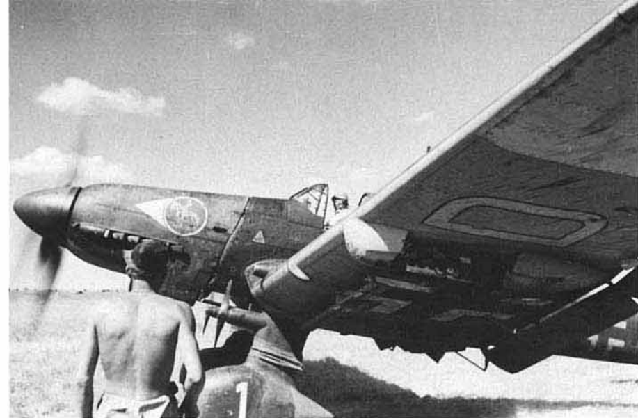
(Above) Oberst Ernst Kupfer of the re-formed II/St.G 2 fires up the engine of his Ju 87D-1 on the Eastern Front in 1942. The Gruppe's 'Knight of Bamberg' emblem carries a Kommandeur's chevron which was occasionally seen within Stuka units. The center section of the underwing bomb rack covers have been removed for easy access to the bomb rack mechanism — a common occurrence. (Bundesarchiv)
