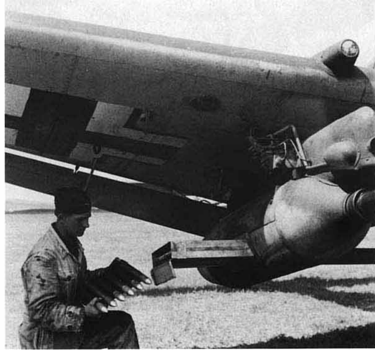
(Above) Six-shot clips of armor-penetrating Wolfram-core 37mm ammunition were loaded into trays through a hinged panel; the rounds were either armor-piercing or blunt-tipped for soft-skinned targets. The structure of the underwing cannons and pods were identical and interchangeable, with the loading aperture and external connections being offset to starboard on each. (Bundesarchiv)
