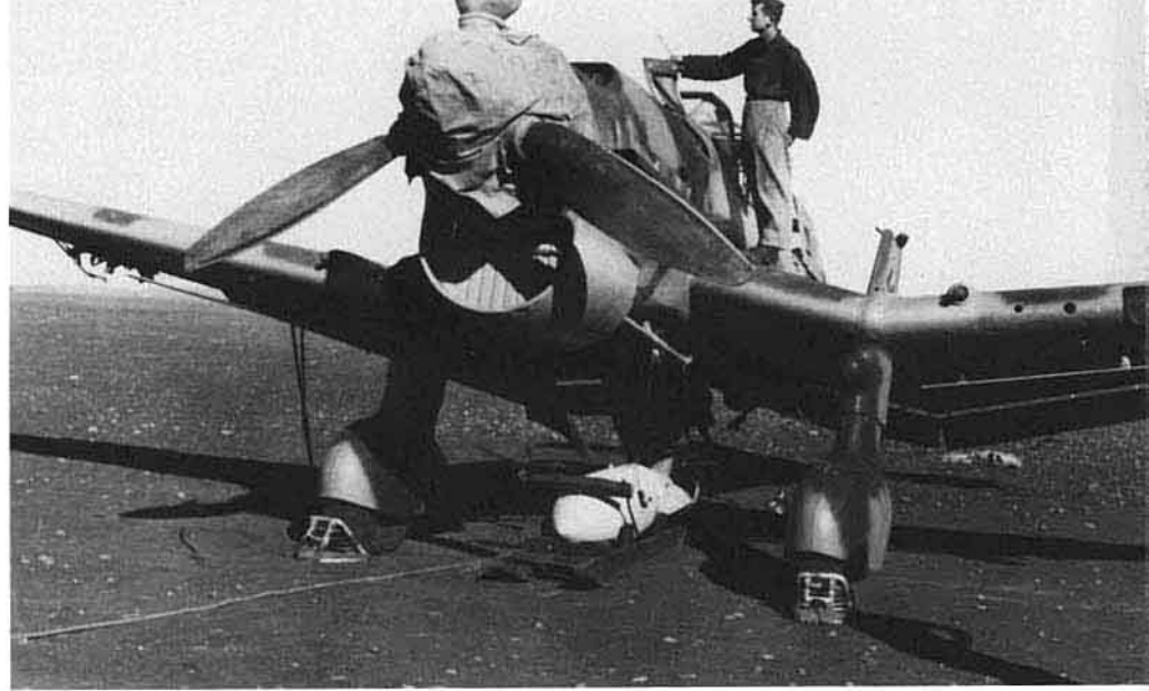
(Above) In the absence of the three wheel hydraulic loading cart, bombloads could be hoisted into place by using block and tackle gear and old fashioned 'elbow grease'. The hinged panel being opened by the ground crewman provided access to the upper fuselage oil tank for servicing. The smaller of the two holes in the port wing leading edge indicates that this Ju 87B-2/Trop has been fitted with an auto-camera. (Bundesarchiv)
