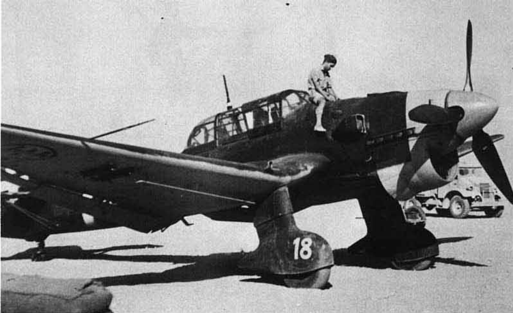
(Above) Italy received over 100 Ju 87s and used them effectively in the Mediterranean and North Africa. This Regia Aeronautica Ju 87B-2/Trop (Werke N. 5763) fell into British hands in September of 1941 and was the subject of an Air Ministry report concerning its Peil G.IV direction-finding device. Uppersurfaces have been resprayed overall Dark Green, with Yellow nose and White Italian national insignia. (Imperial War Museum)
