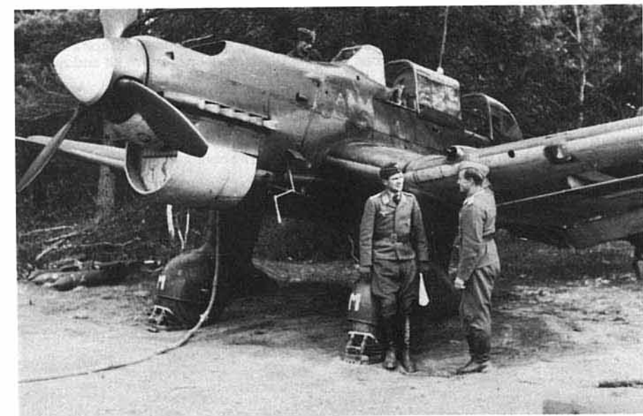
(Below) The small duct in the leading edge of the wing between the landing light and the machine gun was unique to the Ju 87B-2 as were the hinged crank aperture cover, large compressed wood propeller blades, and the new radiator cooling flaps, seen here in the fully retracted position. This machine is S2+MM of 4./St.G 77. (Bundesarchiv)
