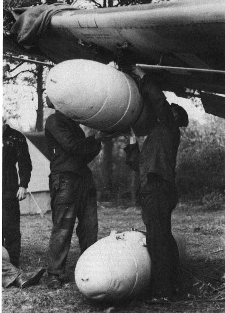
(Above) The waistline securing strap of a 300 liter (66 Imperial gallon) tank is shackled into place below the wing rack of a Ju 87R. Two long detachable steadying pins on each wing rack nestled into corresponding sockets on the tank uppersurface. Stenciling below the wing leading edge reads "Spannband nach dem Tanken nachziehen" (Tighten strap after filling tank). (Bundesarchiv)
