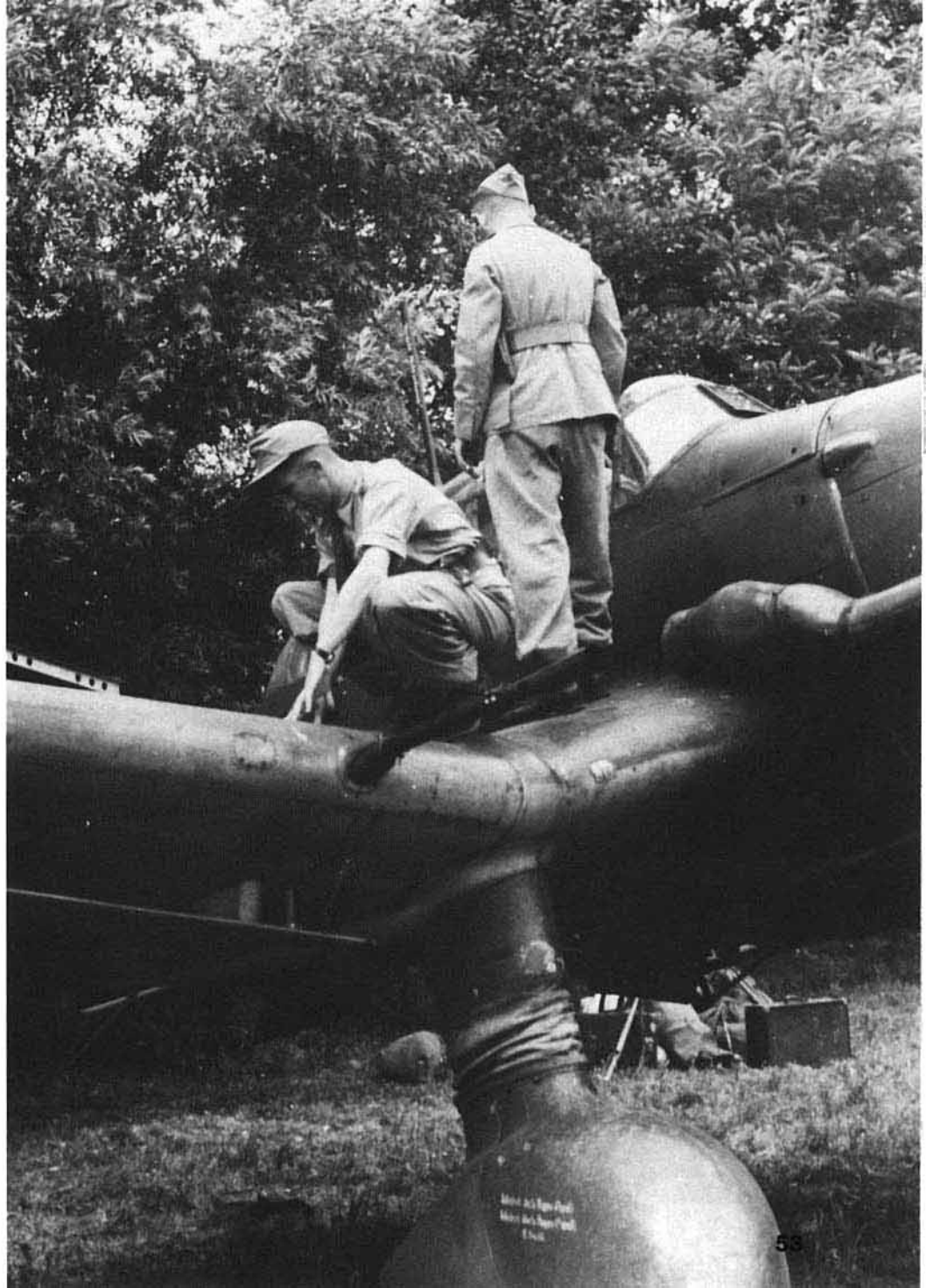
(Right) A groundcrewman inspects the MG 151 cannon bay of a Ju 87D-8 (converted D-5) in southern Italy. The optional flash-hinders have been fitted to the 20mm cannons and a bulbous extension has been added to the flame-dampening exhaust tubes to further reduce exhaust glare. The retention of dive-brakes on nocturnal-assault Stukas was not unheard of, but was somewhat unusual. (Bundesarchiv)
