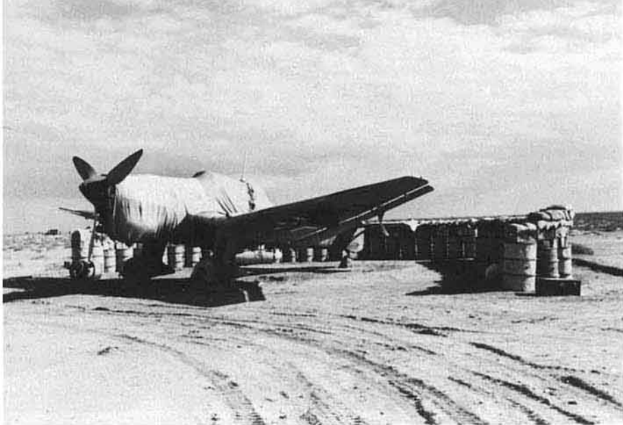
(Above) Conditions in North Africa were often bleak and primitive. This Ju 87R-2/Trop (underwing tanks can be seen on the ground next to the revetment of drums and sand bags) wears a foul-weather tarp. These tarps were standard issue with each Ju 87, and were often labeled with corresponding aircraft serial numbers. (Bundesarchiv)
