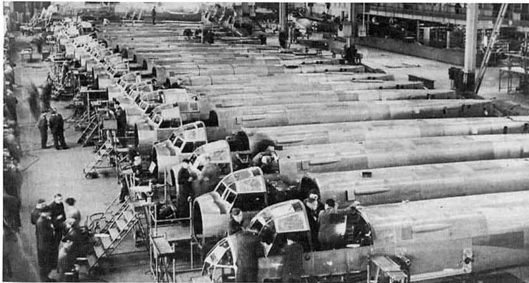
Ju 88A-1 fuselages nearing completion on the Junkers' assembly line during 1939 would be finished in camouflage colors and factory codes before the wings were attached. The ball and socket wing attachments are visible on the fuselage sides.
