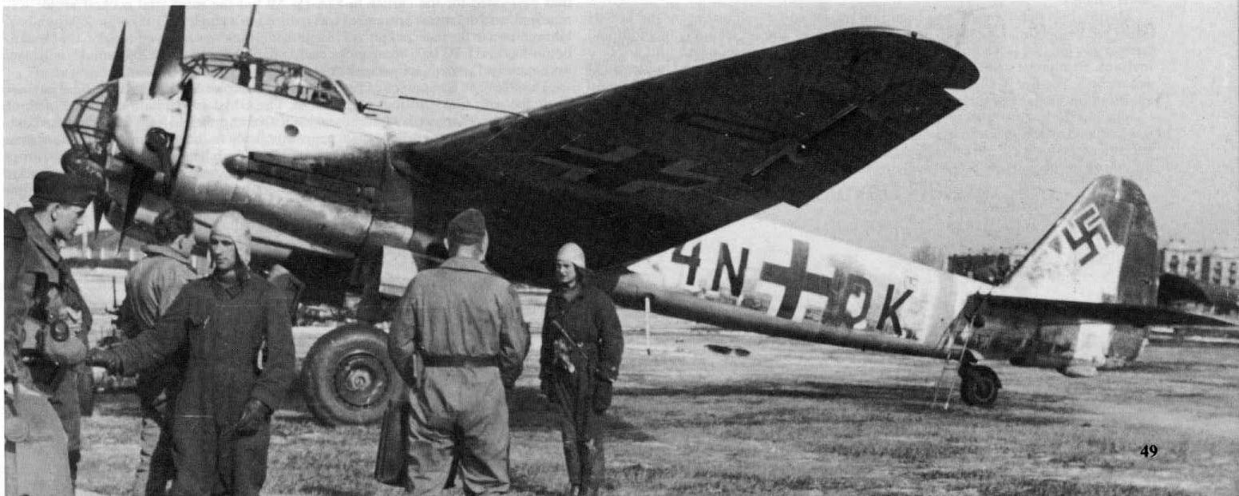
The crew of a Ju 88D-5 of 1.(F)/120 are congratulated after another successful sortie from their Norwegian base. A 20mm MG/FF cannon installation has been fitted to the nose allowing the bomber to attack high priority targets as well as photographing them.
