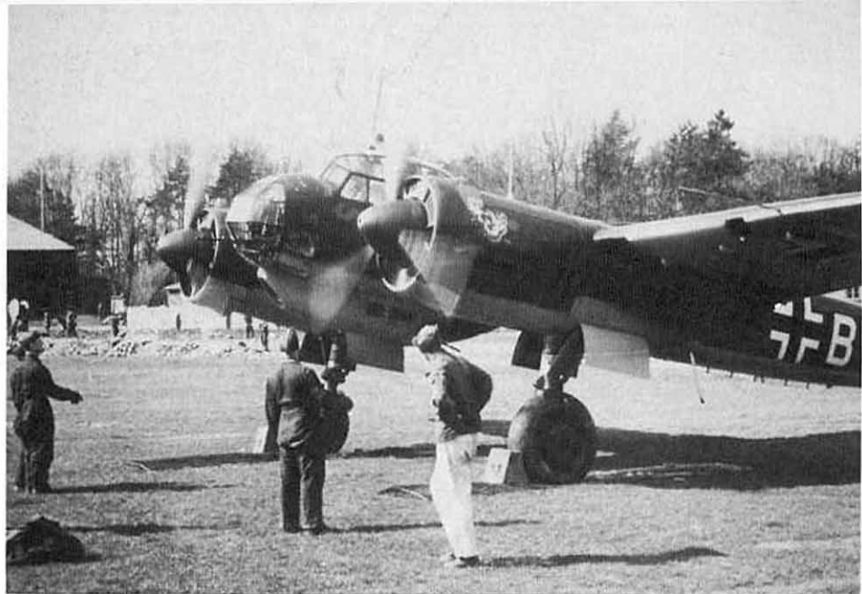
With its wheels chocked, an early photo reconnaissance Ju 88A-1(F) or A-5(F) of 1.(F)/123 runs up its engines during a routine engine test. The dive brakes have been removed, however the mounting brackets near the wing leading edge have been retained. The unit insignia, a Knollenkopf (round headed man holding a spyglass), is carried on the engine cowling. (Smithsonian)
