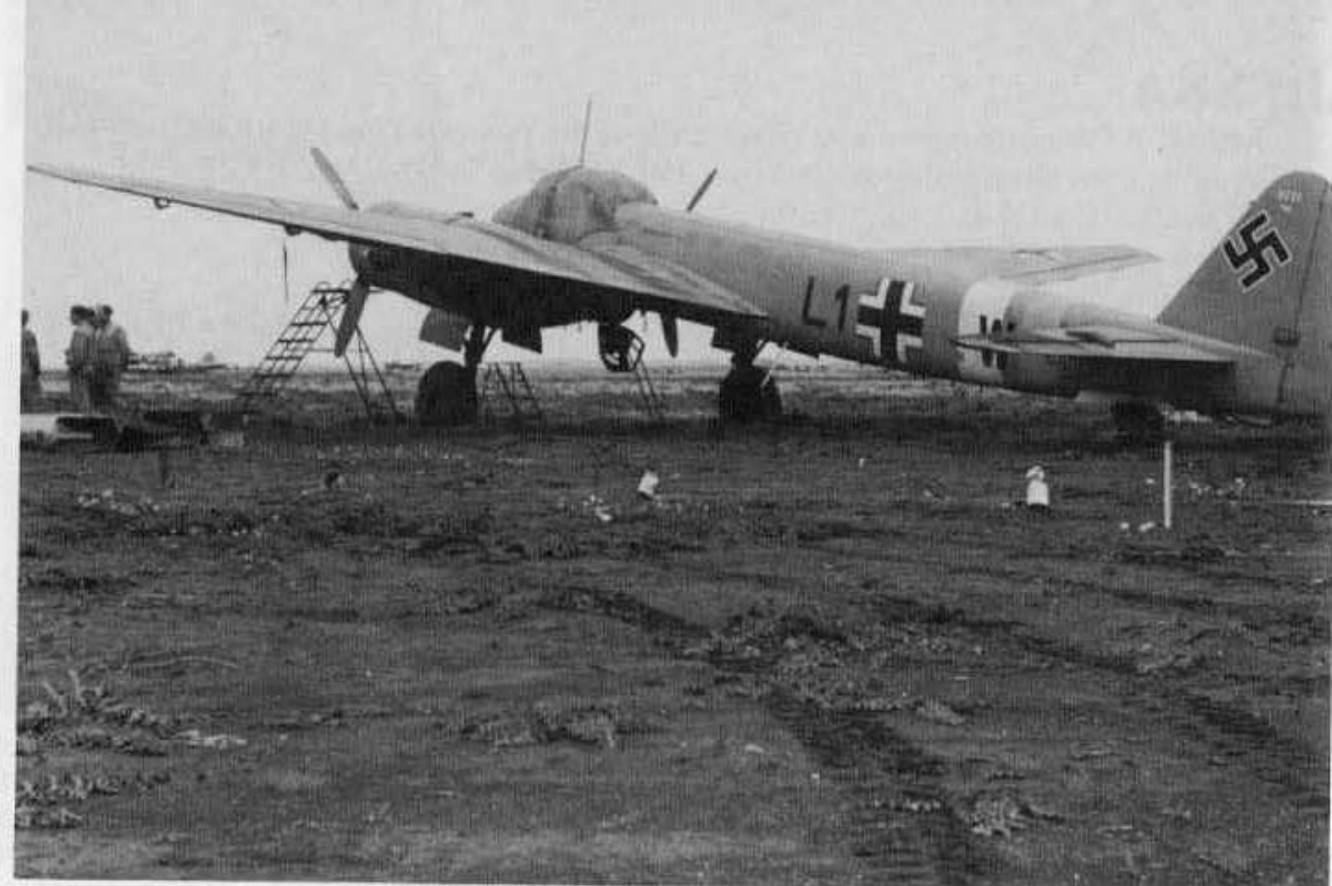
A Ju 88A-10 (L1+LW) of 12./LG 1 parked on a North African airfield has the canopy shielded by a tarp. The bomber carries both a White and Yellow fuselage band. The fuselage code letter 'L' is in Yellow, the identification color of 12.Staffel. Ju 88A-10s were factory tropicalized variants of the Ju 88A-5. The designation 'Trop' is applied under the Werk-Nummer on the fin tip in White.
