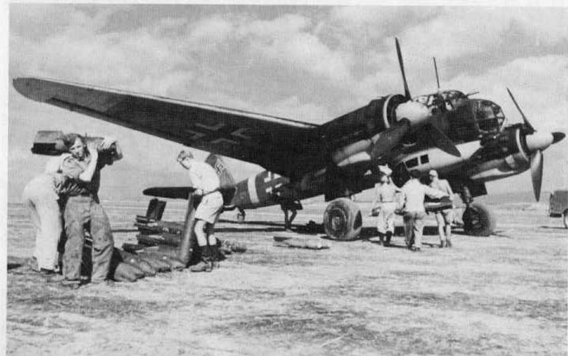
Armorerers load SC 50 (110 pound) bombs into the rear bomb bay of a Junkers Ju 88A-4, armed with an MG-81 machine gun in the starboard windscreen position. The gun is belt fed from an angled ammunition bin installed in the upper portion of the nose. Other Ju 88A-4s replaced the belt fed MG 81 with an optional drum fed MG 15 allowing the ammunition bin to be removed improving the pilot's forward view.
