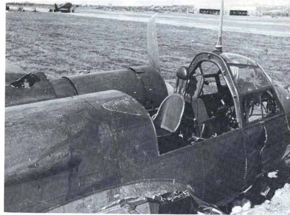
A Ju 88A awaits recovery after a crash landing. The rear canopy was jettisoned in three parts, first the top, then the two side panels. The pilot's seat has a slanted armored head rest while the tubular head rest frame on the radio operator's seat folded downward to allow access to a map case located on the back of the pilot's seat.
