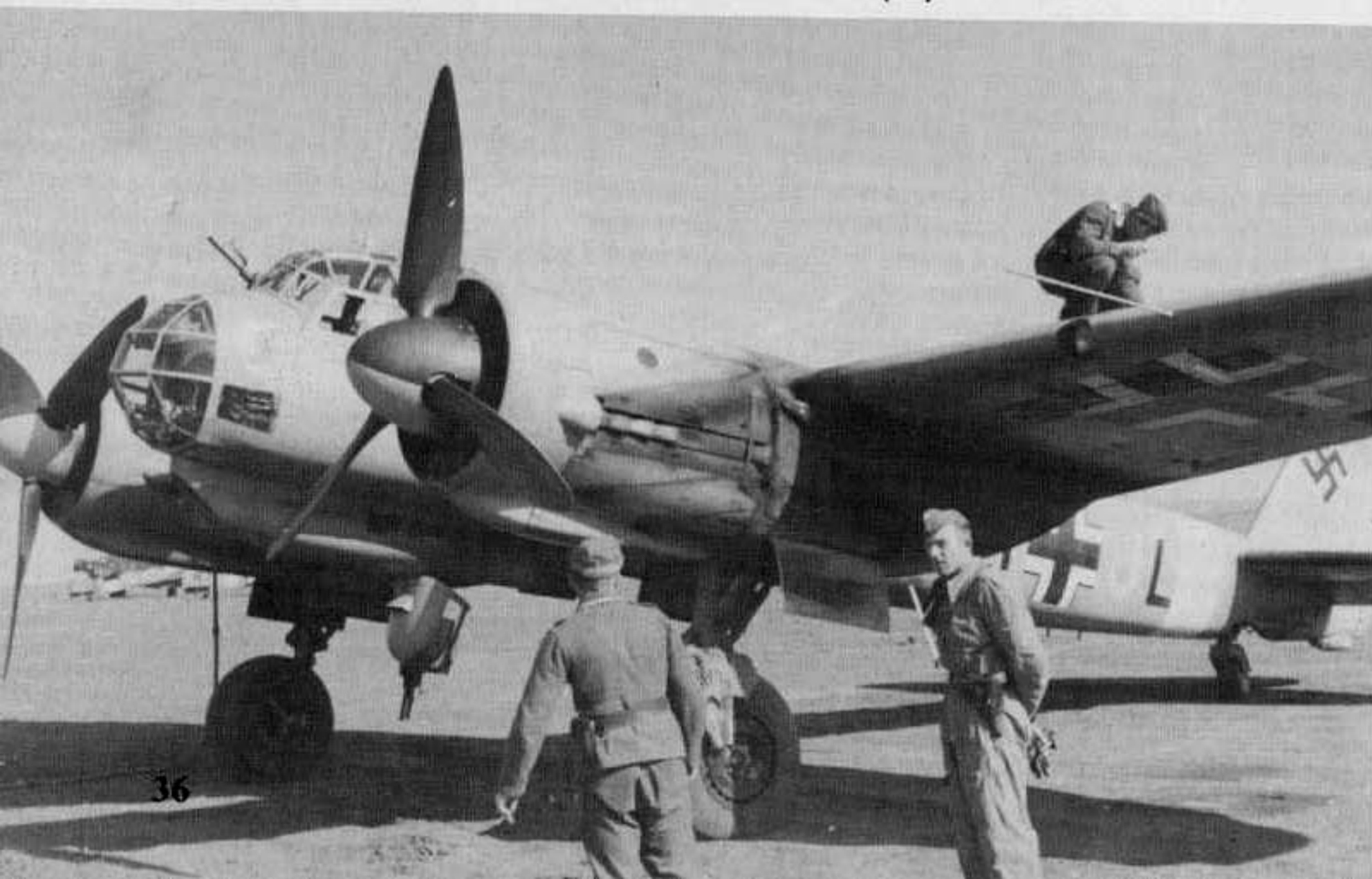
The Ju 88A-11 was externally identical to the Ju 88A-4 and Ju 88A-4/Trop and were usually delivered in a factory applied camouflage of Sand Brown (79) upper surfaces over Blue (78) undersurfaces. This Ju 88A-11/Trop of 3./LG 1 has the fuselage code letter 'J' in Yellow while the spinners are segmented Yellow and Black Green (70).
