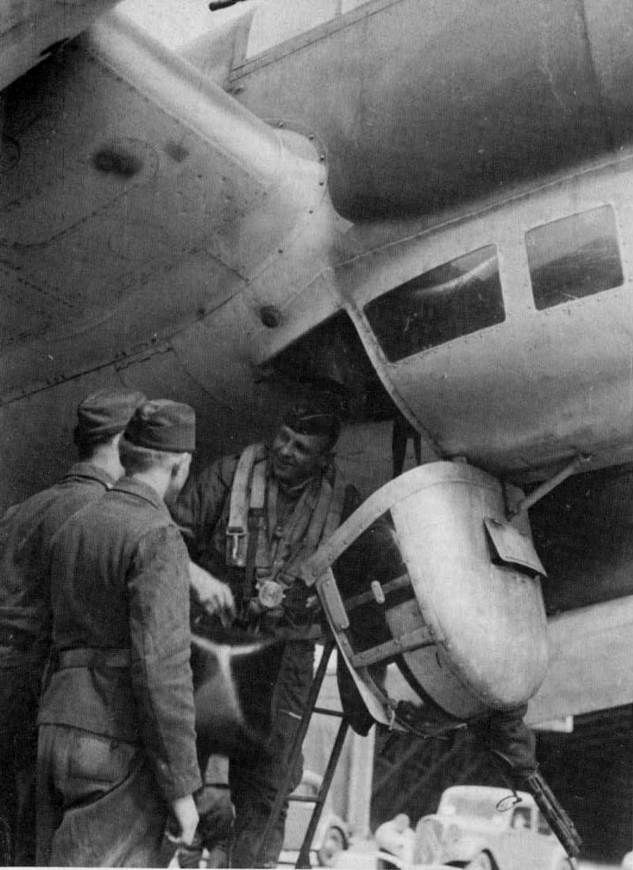
A crewman prepares to enter his aircraft through the open Bola 81Z ventral gun position. The Bola 81Z gun mount was of the same configuration as the Bola 39 but carried MG 81Z twin machine guns instead of a single MG 15 or MG 81J. The Bola gun position had 'horseshoe' shaped armor plate added inside the window framing and a cartridge ejection chute on the underside. The small pneumatic cylinder at the rear of the gun position prevented the hatch from opening too quickly.
