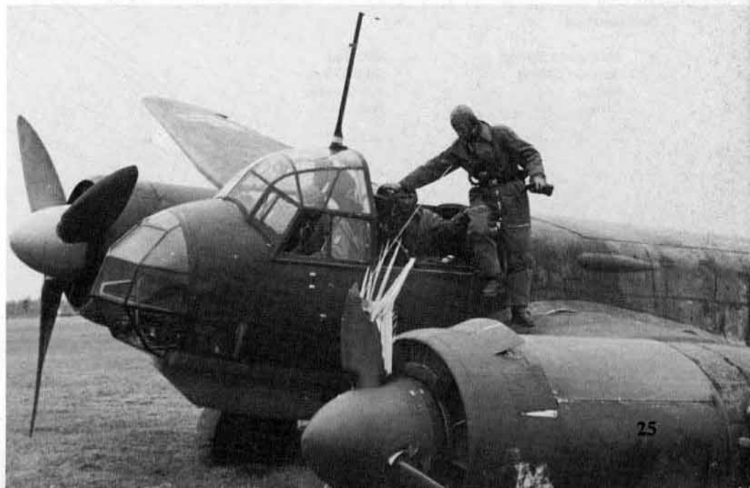
(Below) The radio operator leaves the cockpit of a Ju 88A-4 following a crash landing which splintered the laminated wood of the port VS 11 propeller. The line running down the top of the fuselage is the tow line attached to the life raft which prevented the raft from drifting away after it was deployed. The pilot's fully armored seat is visible.
