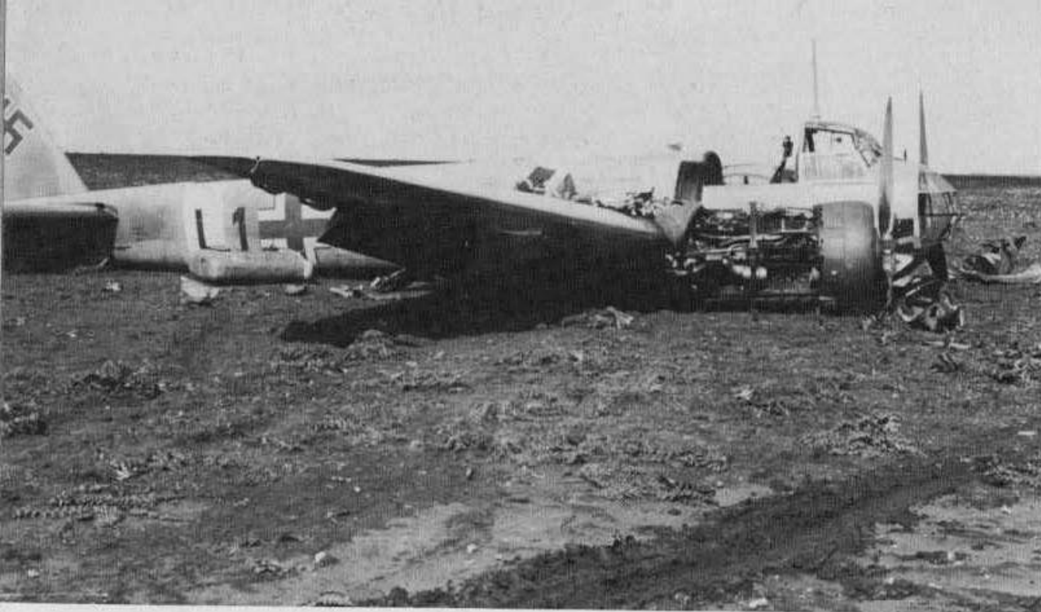
This desert camouflaged Ju 88A-5/Trop of LG 1 has been cannibalized for parts after a crash landing in North Africa. The guns, life raft, engine components, and wing tip navigation lights have been removed for use on other Ju 88s. The Ju 88A-5/Trop designation indicated an aircraft converted for desert operations at a conversion center. Some components of this aircraft retain their original Dark Green European camouflage.
