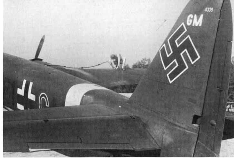
A ground crewman refuels a late Ju 88A-5 (F1+GM, Werk-Nr. 4339) of KG 76 on a Russian airfield. The rubber bumpers on the fuel hose prevented surface damage to the wing during servicing. The last two letters of the fuselage code have been repeated on the fin in White as an identification aid.
