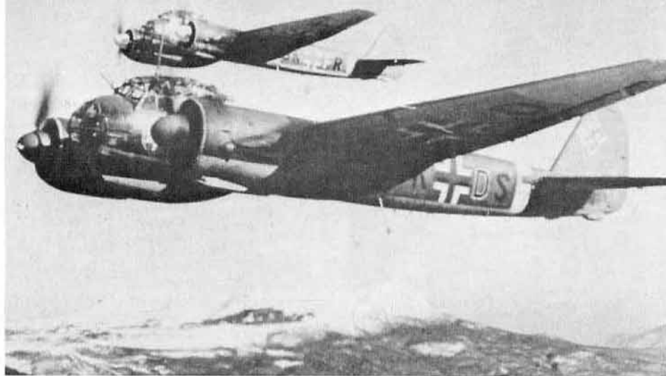
A pair of Ju 88A-4s of III/KG 51 Edelweiss , one of the first units to receive the A-4. The armament improvements which had been progressively introduced on the Ju 88A-5 became standard on the Ju 88A-4, which would become the most numerous variant of the Schnellbomber produced.
