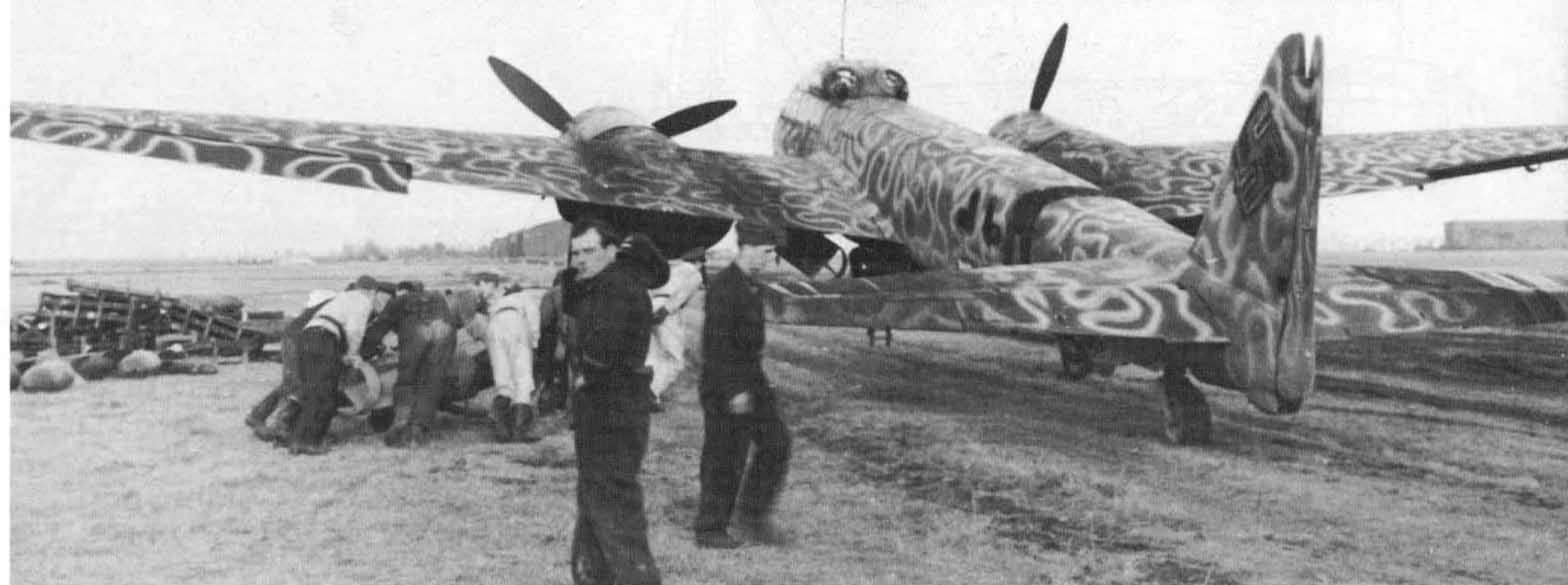
(Above) Ground crews push a bomb dolly toward a Wellenmuster (wave pattern) camouflaged Ju 88A-4 on an Italian airfield during late 1943. The Wellenmuster camouflage was used primarily for operations over water from mid-war onward.
