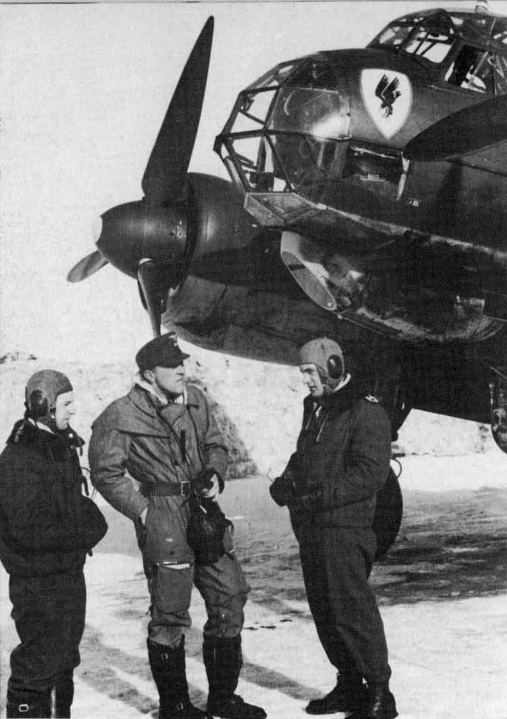
A Ju 88A-4 of KG 3 carries colorful markings, the fuselage code (5K+FN) and propeller spinners are Red, the identification color of 5.Staffel, and the fuselage band is in Yellow. The windscreen machine gun is a belt fed MG 81. The gun's ammunition bin is visible through the upper nose glazing. KG3 was heavily committed to the Eastern Front.
