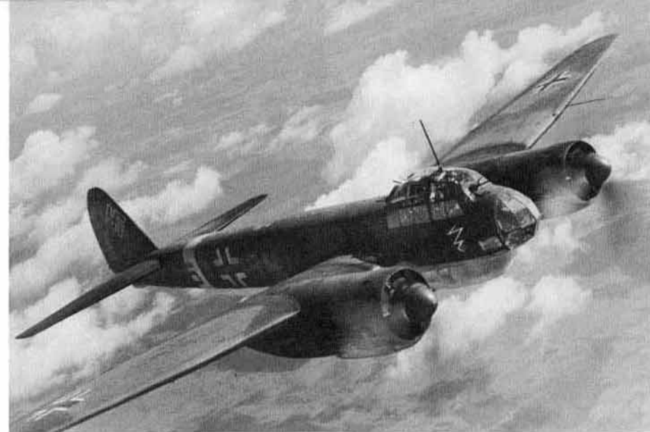
A Ju 88A-4 of KG 3 carries colorful markings, the fuselage code (5K+FN) and propeller spinners are Red, the identification color of 5.Staffel, and the fuselage band is in Yellow. The windscreen machine gun is a belt fed MG 81. The gun's ammunition bin is visible through the upper nose glazing. KG3 was heavily committed to the Eastern Front.
