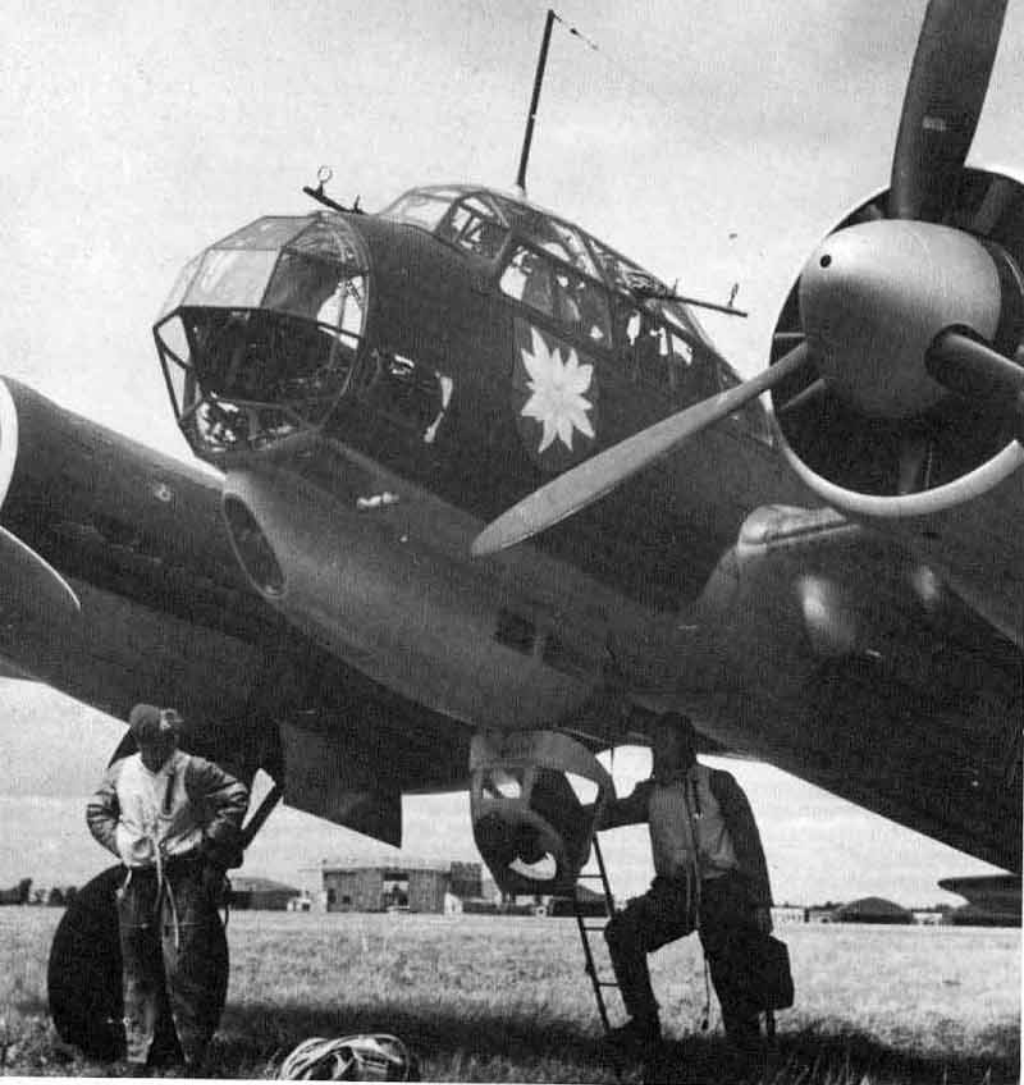
Two crewmen board a Ju 88A-1 of 3./KG 51 Edelweiss on an airfield in France. The oval window at the front of the ventral gondola is the aiming window for the Lotfe bombsight, while the window next to the gondola provided a degree of downward vision for the pilot. The optional side canopy MG 15 machine guns proved difficult to use in the cramped cockpit of the Ju 88.
