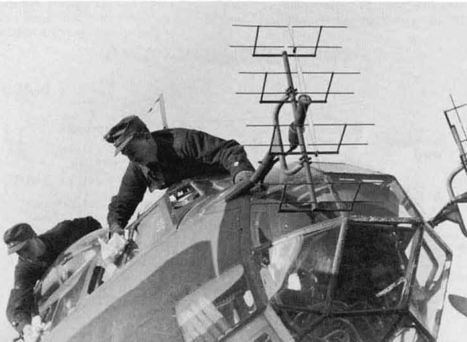
A number of Ju 88A-6 airframes were rebuilt and modified for the anti-shipping role under the designation Ju 88A-6/U. This Ju 88A-6/U has had FuG 200 radar antennas installed on the nose, and the windscreen machine gun position covered with a metal plug. These FuG 200 masts are fixed non-pivoting types.
