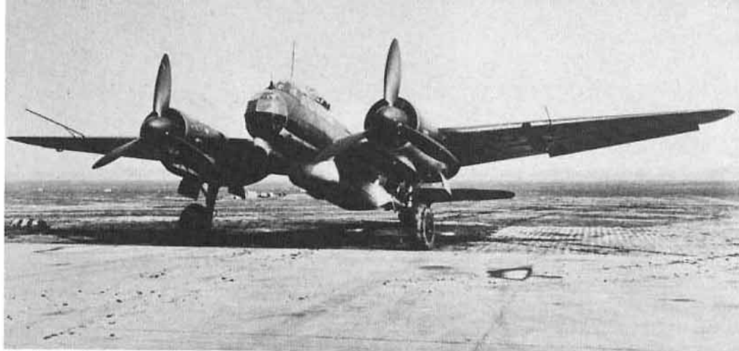
Equipped with a research boom on its starboard wing, this Ju 88A-15 (Werk-Nr. 140561) was retained by Junkers for test trials. The huge wooden under fuselage bomb-bay carried the bomb load internally, eliminating the ETC under wing bomb racks. A streamlined fairing under the nose housed the bomb sight. (Gene Stafford)
