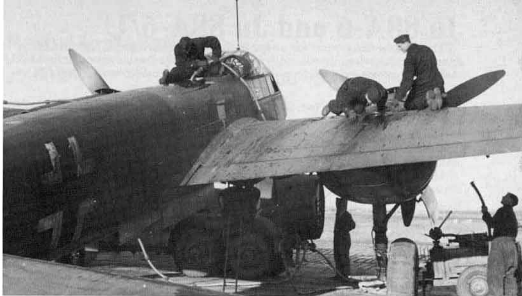
As one ground crewman checks the wing tanks of a Ju 88A-4, another tops off the auxiliary fuselage bomb-bay tank from the upper fuselage refueling point. Both bomb-bays could be equipped with fuel tanks, although the front bay was most commonly used for fuel. The rear bomb-bay four paneled doors are open ready to receive a bomb load once refueling is completed.
