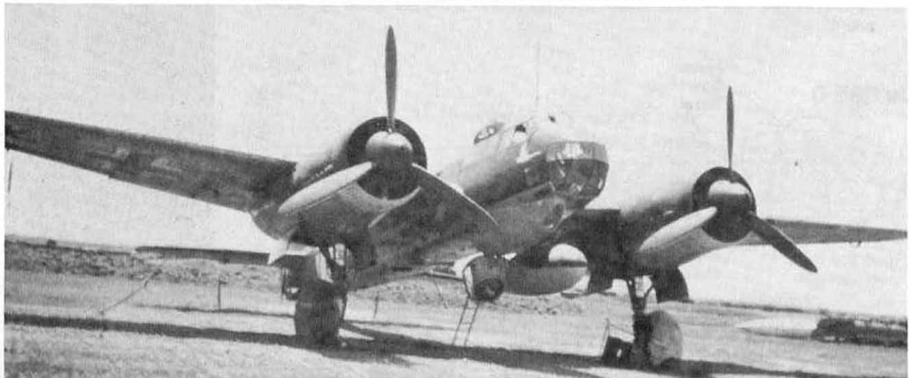
A Ju 88D-2 carries the 'flying goose' insignia of 1.(F)/121 under the cockpit. Three optically flat camera windows are visible in the rear bomb bay. 1.(F)/121 operated a mix of Ju 88 reconnaissance aircraft including the Ju 88D-2, tropicalized Ju 88D-4, Ju 88D-1 and Ju 88D-3 for missions in the Mediterranean and North African theaters.
