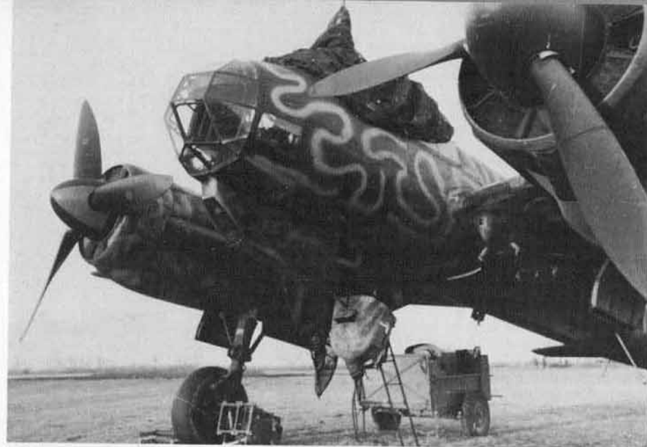
The factory installed flat faced gondola cannon mounting enabled late production Ju 88A-4s and Ju 88A-14s to be easily converted to the cannon armed configuration. This Italian based (either a late Ju 88A-4 or Ju 88A-14) carries the flat faced gondola and cropped bomb sight window with the bomb sight in place.
