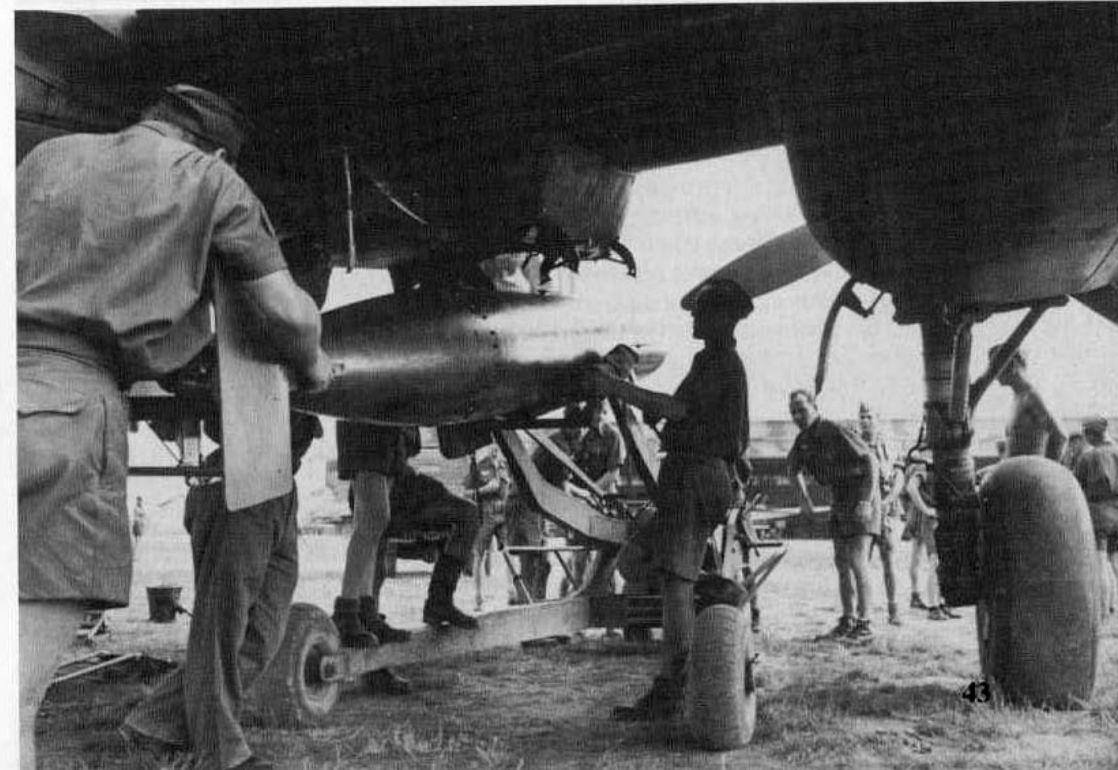
(Above and Below) Groundcrewmembers raise a 1,686 pound LT F5b torpedo into position under the PVC torpedo rack on a Ju 88A-4/Torp. PVC racks were larger and deeper than the ETC bomb rack, and featured a different shackle arrangement. The oversized wooden fins on the torpedo stabilized it after release and broke off upon impact with the water. The Ju 88A-4/Torp and Ju 88A-17 could carry two such weapons.
