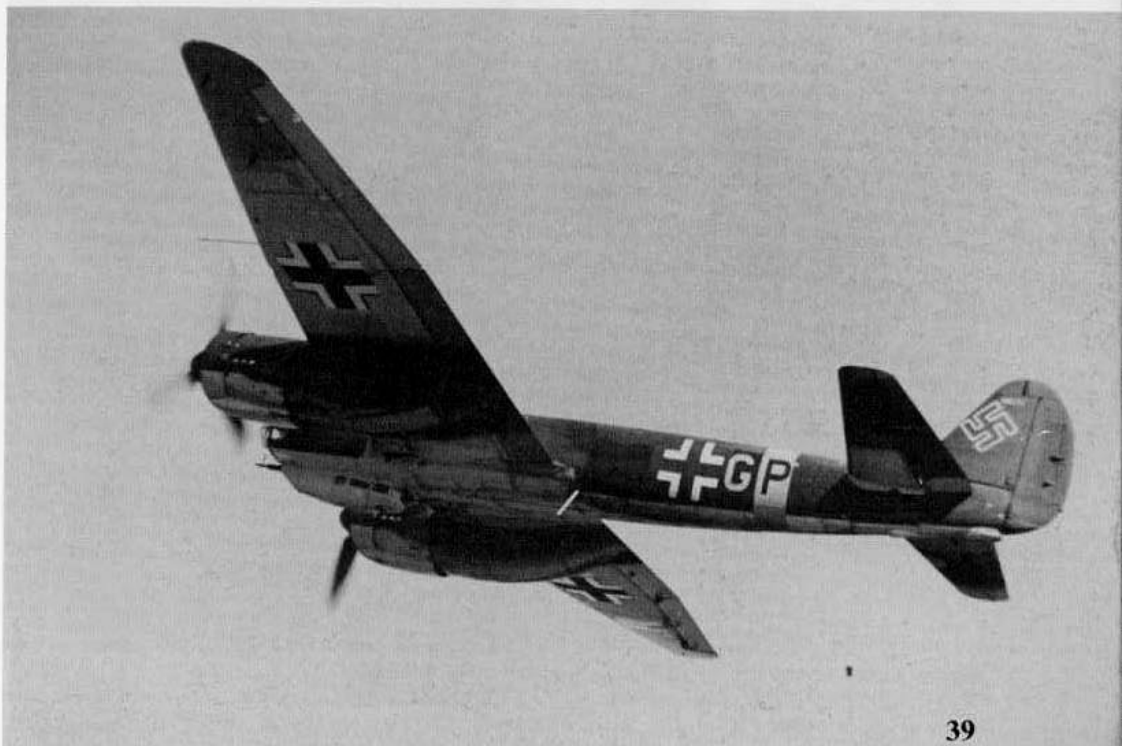
(Above) A late production Ju 88A-5 of II/KG 30 has the windscreen MG 15 removed, an anti-balloon nose fender installed, and an MG/FF 20mm cannon mounted in the nose. The white circular shape inside the nose is the 120 round ammunition drum for the MG/FF cannon.
