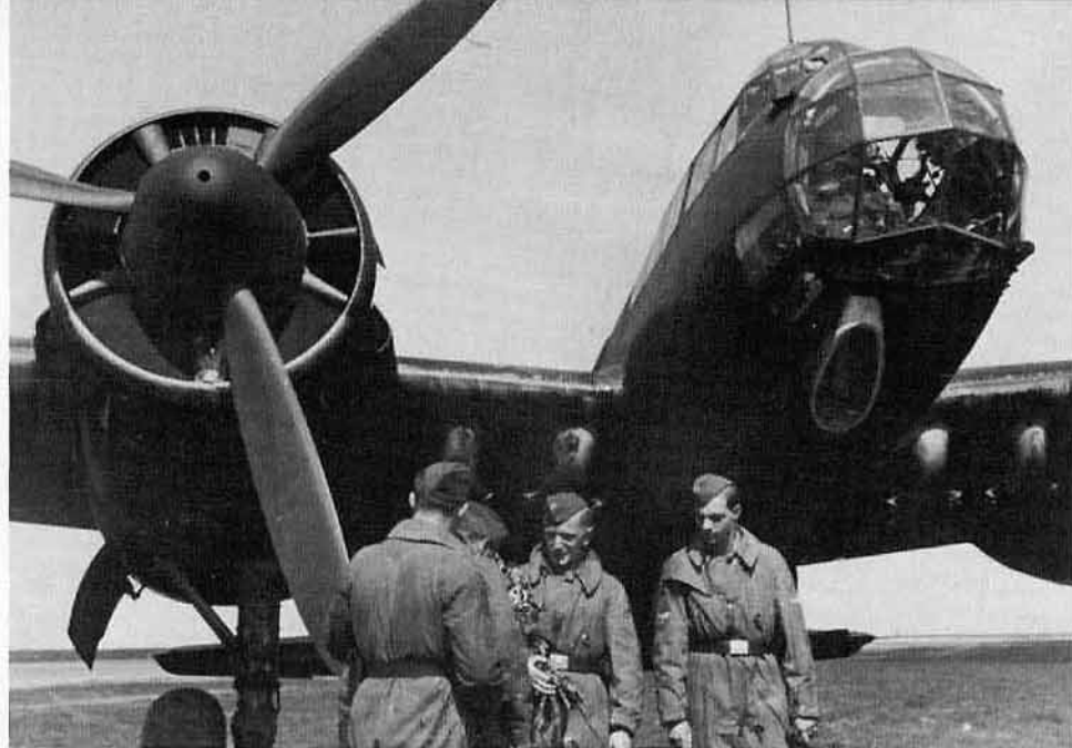
The Ju 88A-6 was identical to the Ju 88A-5 with the exception of the brackets for mounting the anti-barrage balloon cable fender/cutter on the nose and wings. When the fender was not in place the brackets were sometimes covered with streamlined 'teardrop' fairings.
