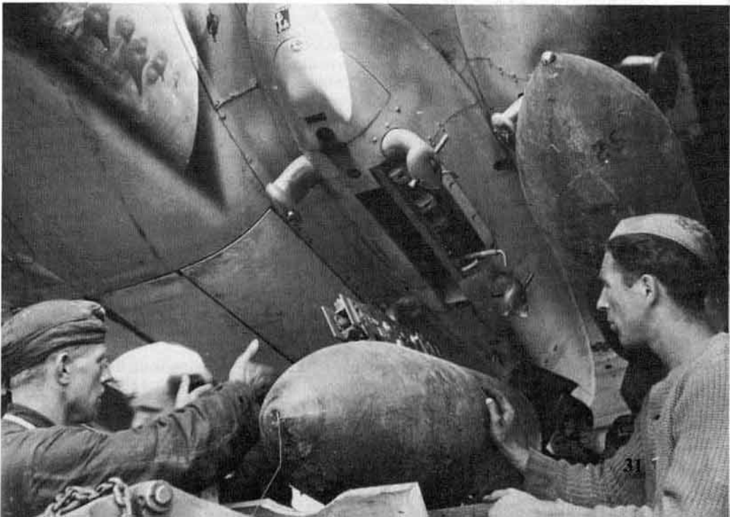
When a bomb was positioned the suspension block was locked into the rack opening, and the sway braces were tightened down against the bomb. When either fuselage bomb-bay was fitted with a four paneled door, the middle sections opened straight down from the fuselage centerline, while the outer doors opened down from the fuselage sides.
