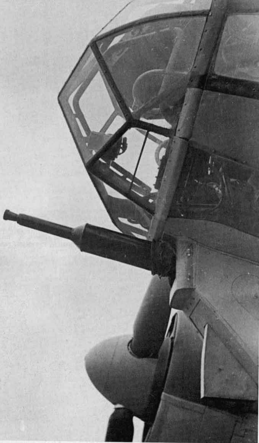
The factory installed flat faced gondola cannon mounting enabled late production Ju 88A-4s and Ju 88A-14s to be easily converted to the cannon armed configuration. This Italian based (either a late Ju 88A-4 or Ju 88A-14) carries the flat faced gondola and cropped bomb sight window with the bomb sight in place.
