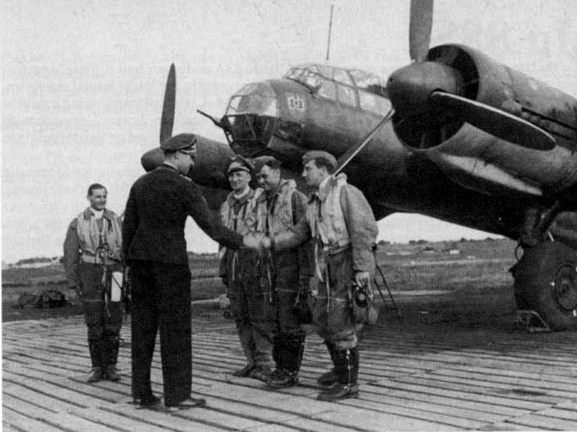
The crew of a Ju 88D-5 of 1.(F)/120 are congratulated after another successful sortie from their Norwegian base. A 20mm MG/FF cannon installation has been fitted to the nose allowing the bomber to attack high priority targets as well as photographing them.
