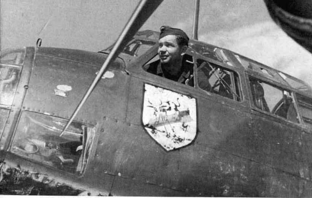
This early Ju 88A-5 carries the cow astride a bomb insignia of 4./KG 1. The opening in the upper canopy center section is a gun mount for an optional side mounted MG 15 machine gun. A number of Ju 88A-5s also featured an exterior 'stop bar' on the canopy framing below the gun mount to prevent the gunner from firing into the engine nacelle.
