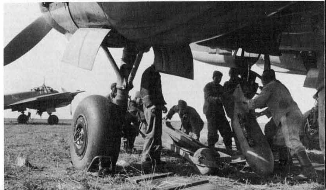
(Below) A bomb fitted with a suspension block is maneuvered from a three wheeled bomb cart in preparation for loading on the inboard ETC rack of a Ju 88A-4. The tires used on the Ju 88A-4 were slightly larger than those used on earlier variants to handle the increased gross weight of the A-4, with the size increased from 1,100 x 375mm to 1,140 x 410mm.
