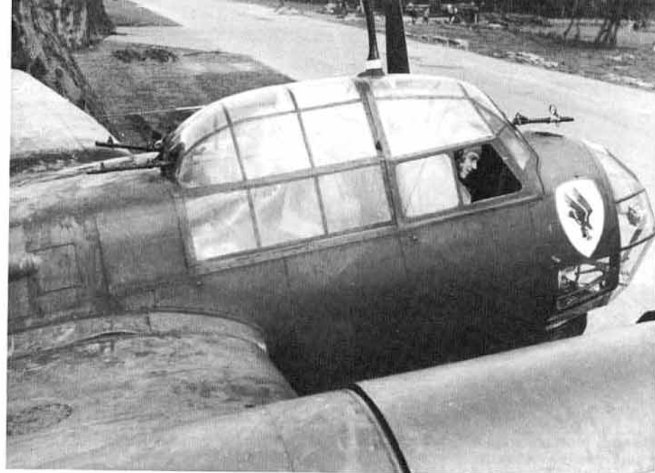
Late production Ju 88A-1s replaced the single rotating rear cockpit gun mount with two MG 15 machine guns in simple flexible gun mounts. The lack of cockpit armor plate and gun-sights indicates that work on the rear canopy conversion has not been completed. The white background of the unit insignia indicates this bomber is assigned to I/KG 30.
