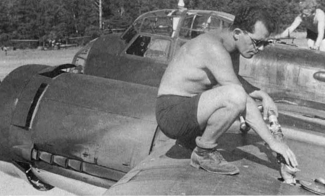
Although various defensive machine guns could be carried on the Ju 88A-5, the 7.9mm MG 15 machine gun was the most commonly used weapon. The triangular marking of the fuel tank filler caps are fuel octane markings which specified the type of fuel to be used when servicing the bomber.
