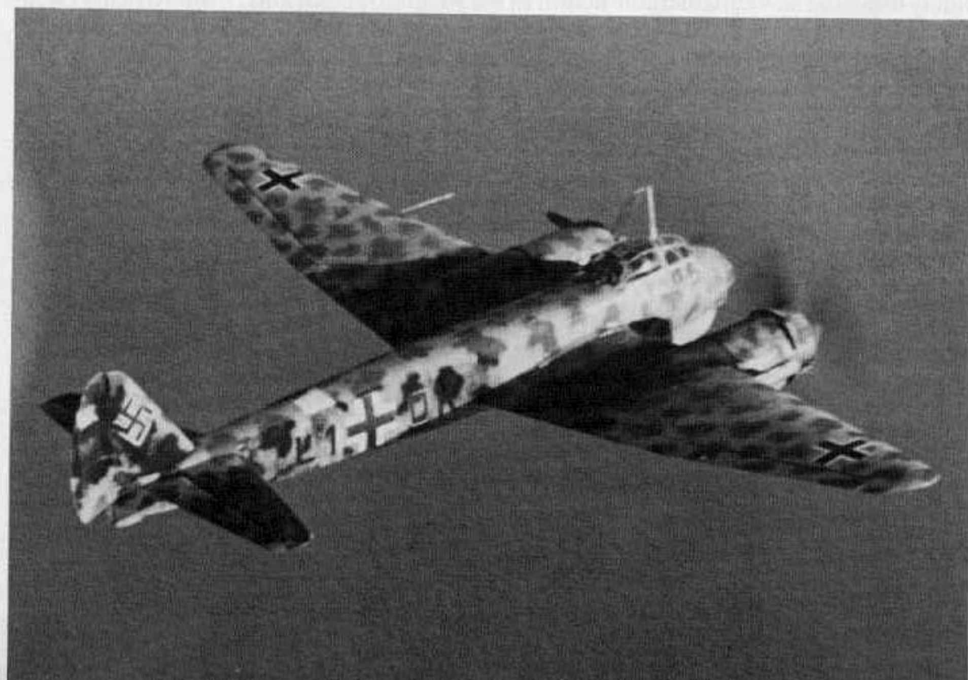
A Ju 88A-11 (L1+OK) returns from a mission with the port propeller feathered. The bomber carries a field applied mottle of Green (80) over the factory applied Sand Brown (79) upper surface camouflage.
