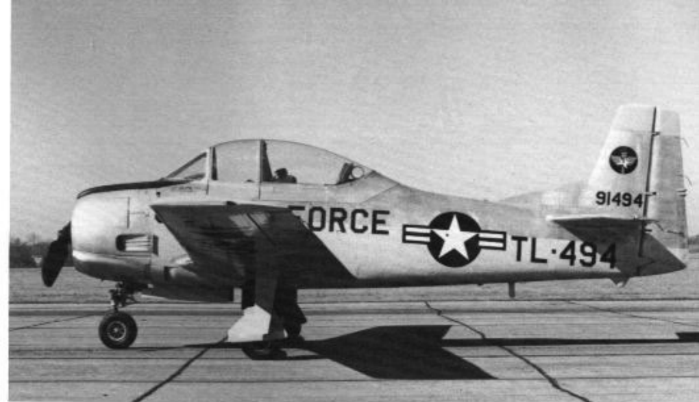
The fourth production T-28A (49-1494) on the ramp at North American's Inglewood, California assembly plant. This Trojan is painted with a corrosion resistant Light Gray paint on the lower half of the fuselage with the upper half left in Natural Metal. The insignia on the tail is the badge of the Air Training Command. (Hugh Morgan)
