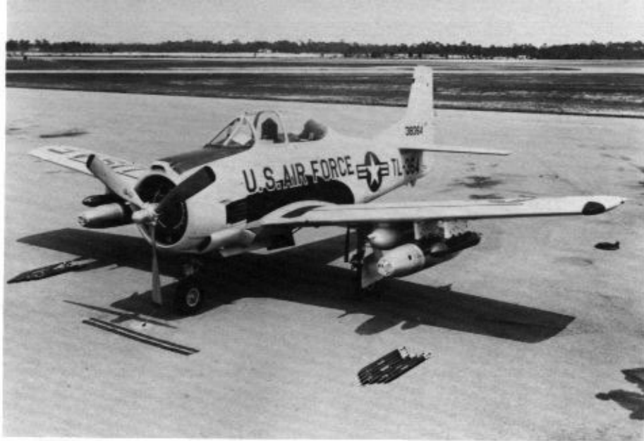
This T-28D-5 (38364) of the 4400th Combat Crew Training Squadron (CCTS) was put on display at Eglin AFB, Florida, during 1961. The armament includes .50 caliber machine gun pods, ammunition, napalm bombs and 2.75 inch rocket pods. Within a short period this same aircraft deployed to Vietnam with the Farm Gate detachment. (USAF Via Rod Bankston)
