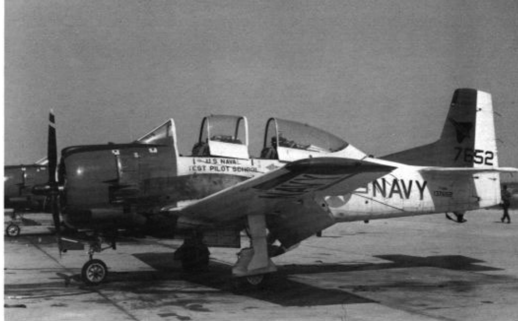
A T-28B (BuNo 137652) of the Naval Test Pilots School parked on the ramp at NAS Patuxent River, Maryland. The insignia on the tail is a silhouette of a Douglas F4D Skyray. The aircraft is configured for towing streamers and the wire running from the front cockpit to the tail bumper controls the cable release. (Norman Taylor)
