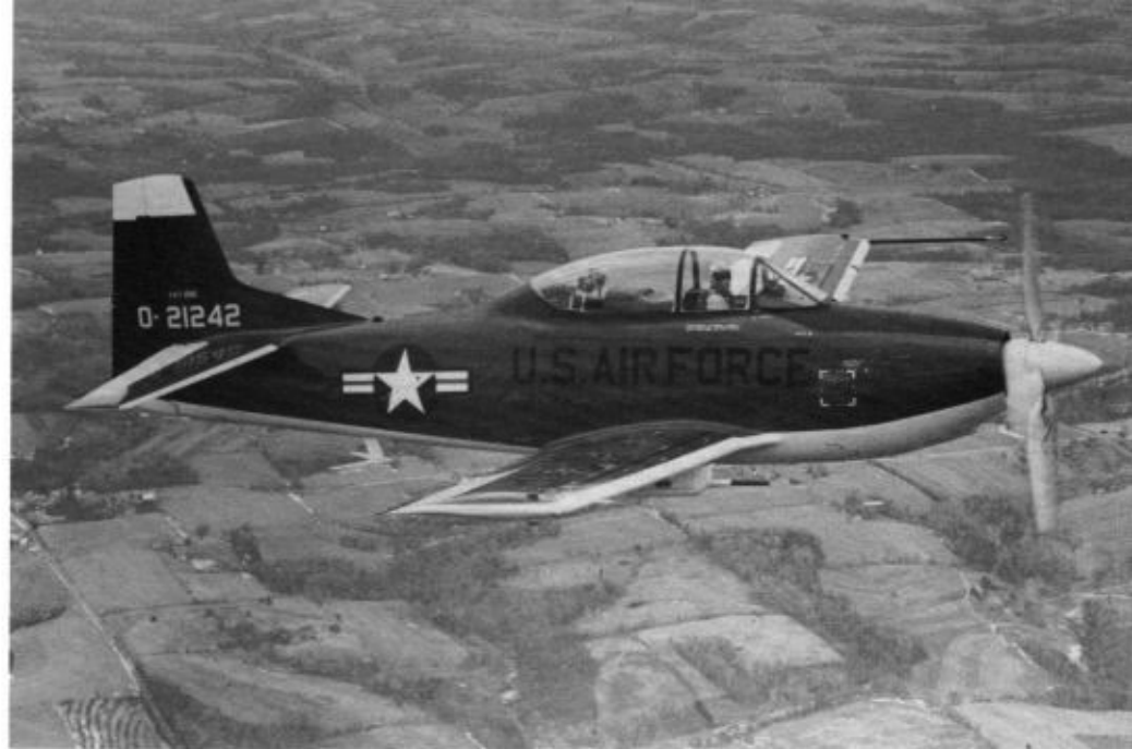
The YAT-28E prototype was developed to replace the T-28D in the COIN role and made its first flight on 15 February 1963 with North American test pilot George Hoskins at the controls. The YAT-28E was powered by a 2,445 shp turboprop engine and had a projected top speed of almost 400 mph. (Norman Taylor)
