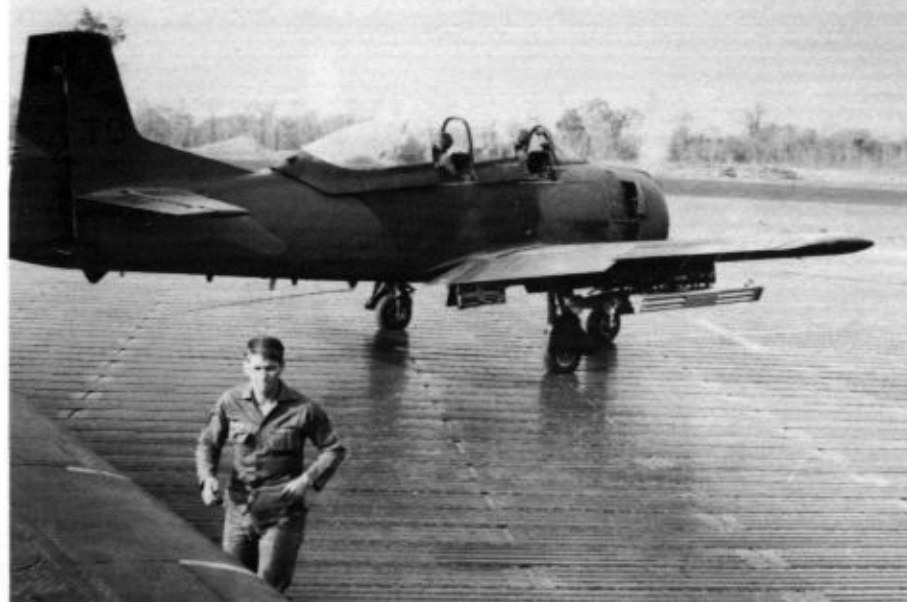
The armorer has just removed the armament safety pins from the weapons on this T-28D-5 (49-1583) of the 606th SOS as the aircraft warms up prior to taxiing out for another mission over Laos during 1968. The long whip antenna under the fuselage is for an FM radio used for communications with ground troops. (N. Crocker via N. Taylor)
