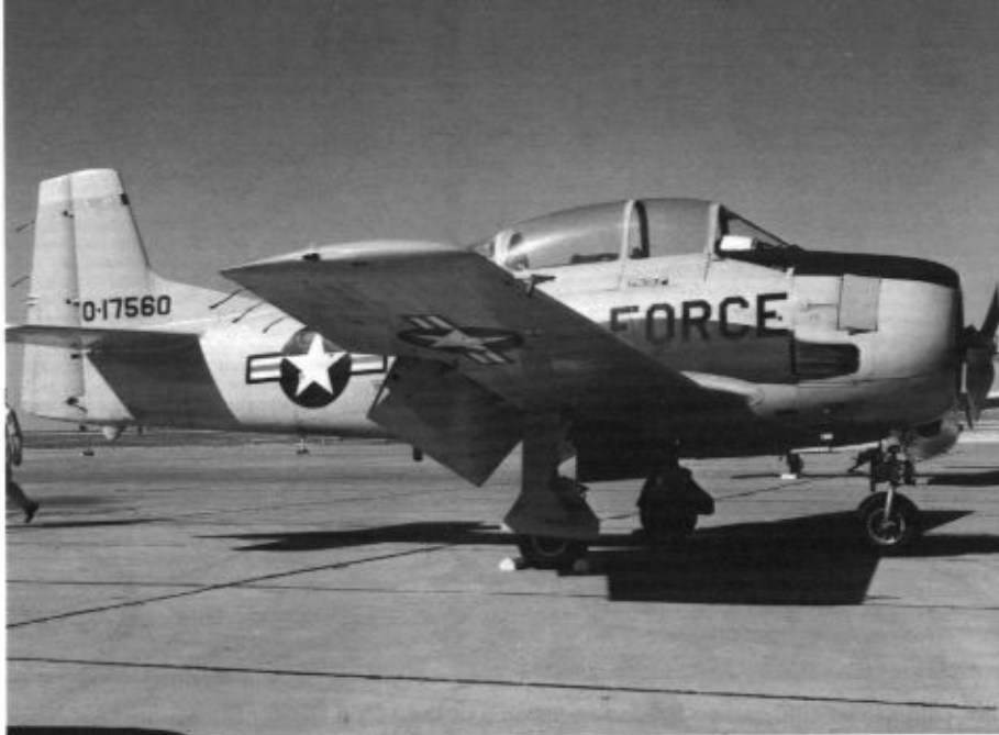
An overall Light Gray T-28A (51-7560) of the 3512th PTS parked on the ramp at Webb AFB, Texas during May of 1965. The gloss acrylic paint was found to be highly radar reflective and easier to keep clean than the earlier lacquer paints. (Norman Taylor)
