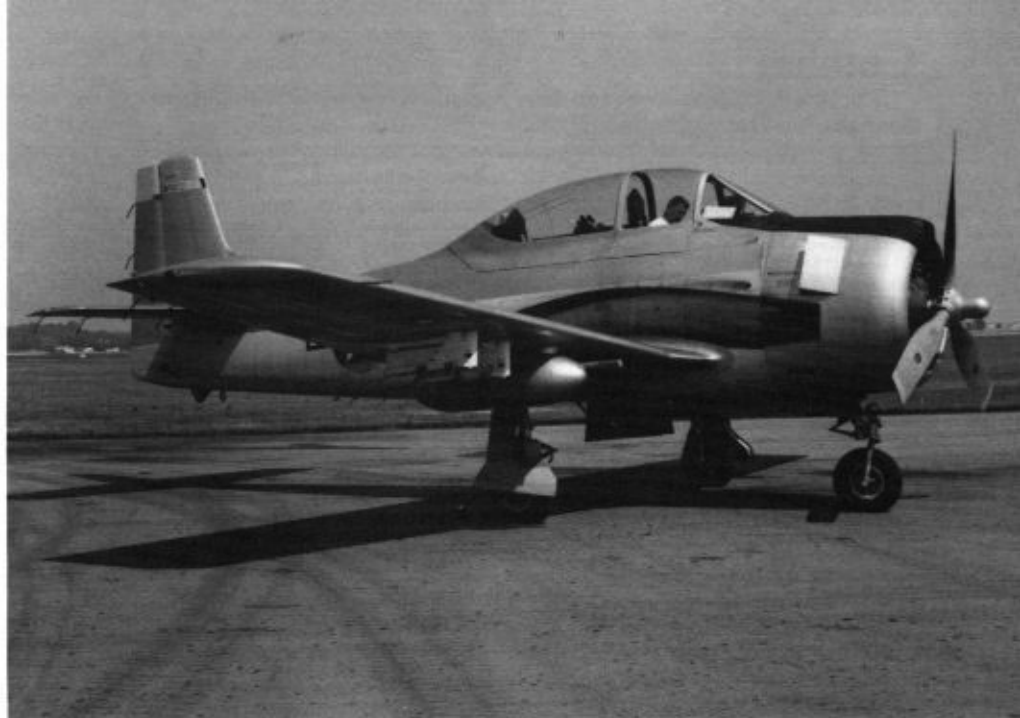
The majority of T-28Ds were remanufactured T-28As. This T-28D (52-12001) was rebuilt from a T-28A at North American's Inglewood, California plant. The aircraft is overall Natural Metal and carries two 100 round .50 caliber machine gun pods and four underwing pylons. (Norman Taylor)
