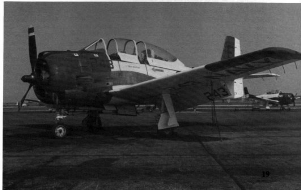
This T-28B of Training Wing 5 (TW-5) is tied down on the ramp at Saufley Field, NAS Pensacola, Florida. T-28s on the ground usually had the flaps in the full down position. (USN via Norm Hill)
