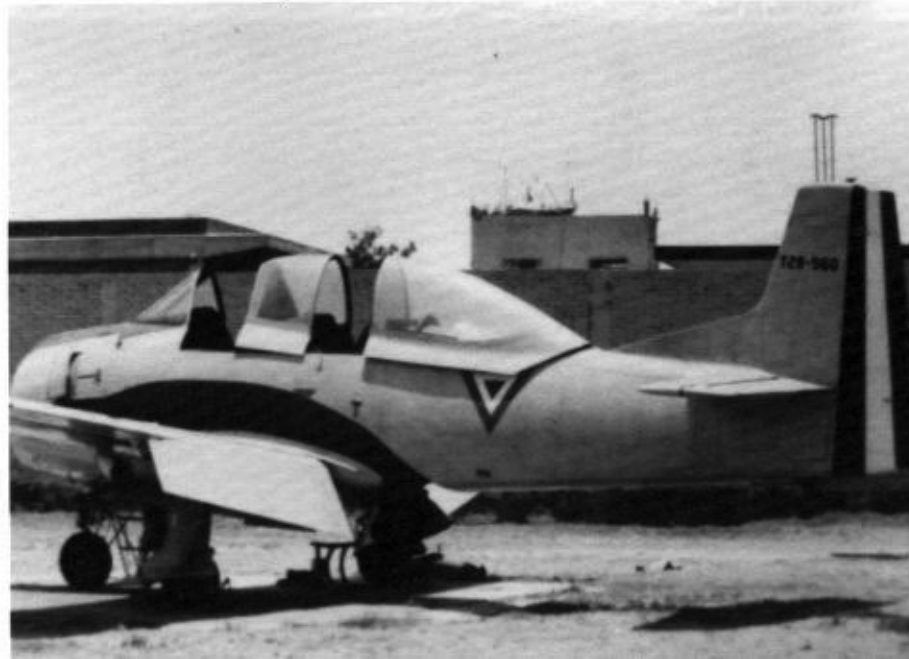
The Mexican Air Force received over eighty T-28As for use in both the training and internal security roles. This T-28A carries the locally assigned serial T-28-960 on the fin in Black. The national insignia and rudder stripes are Red, White, and Green. (D. Hagedorn via Nicholas J. Waters III)
