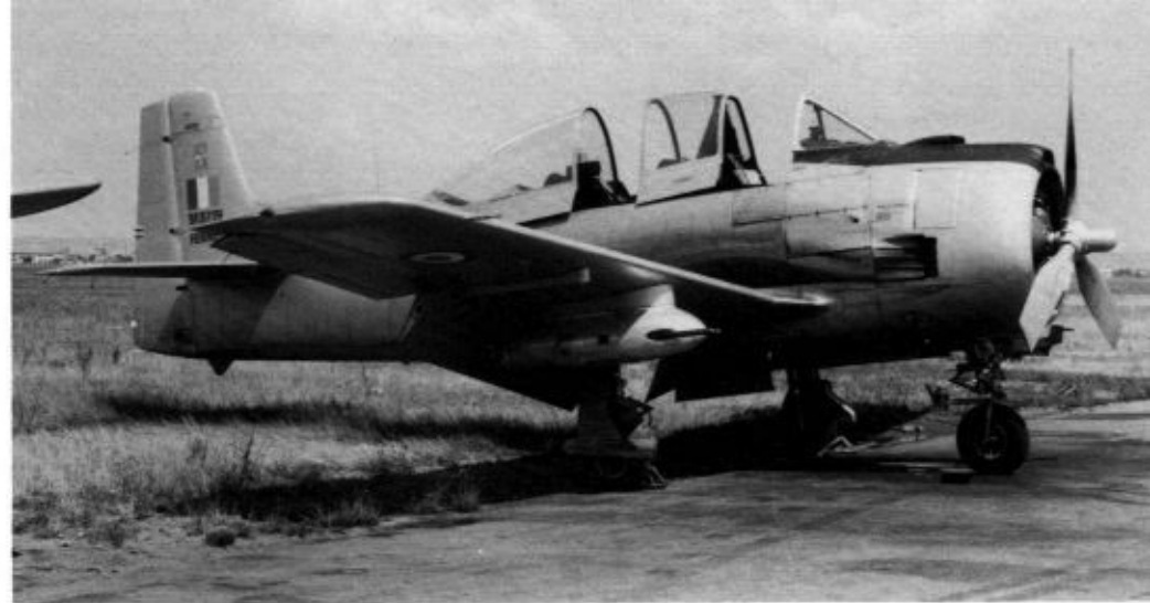
The gun pods carried on the Fennec were of French design and mounted two 12.7 MM machine guns and their ammunition. This Fennec of ERALA 01/39 at Lyon, France, was modified to see service in Algeria and was later sold to Argentina during 1967. (Norman Taylor)
