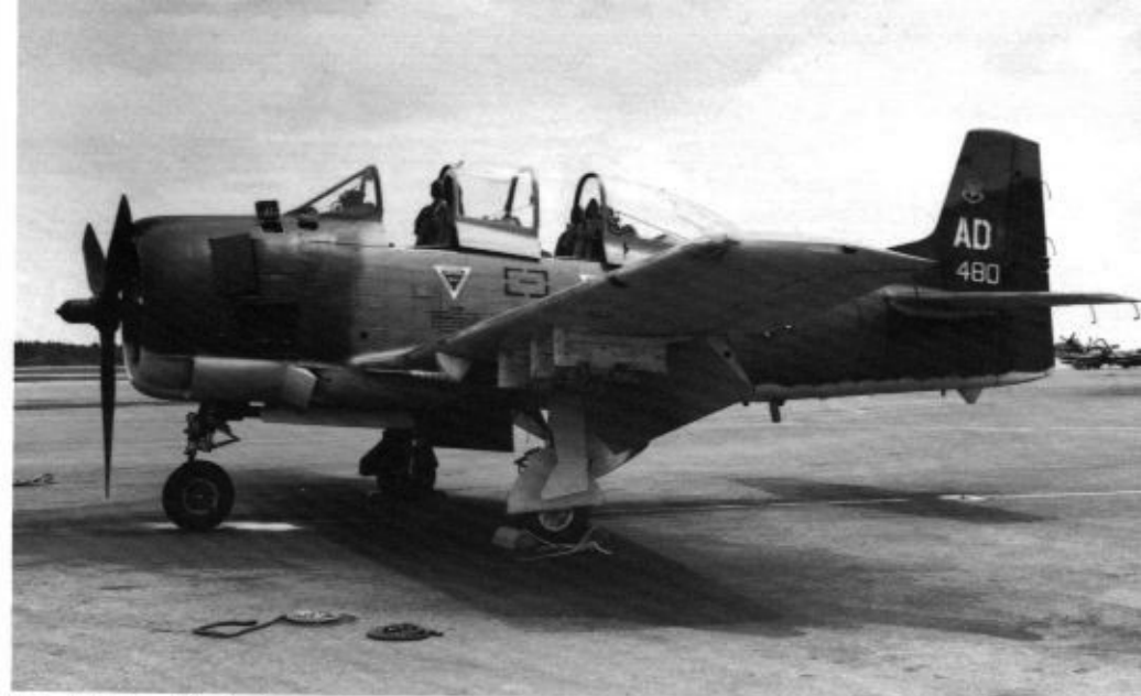
Fairchild Aircraft rebuilt seventy-two T-28As to T-28D-5 standards. A number of these aircraft were also fitted with a rocket propelled ejection seat designed especially for the T-28. The seat ejected through the canopy, and aircraft with the seats had a modified canopy with detonator chord imbedded in the plexiglass. (Norman Taylor)
