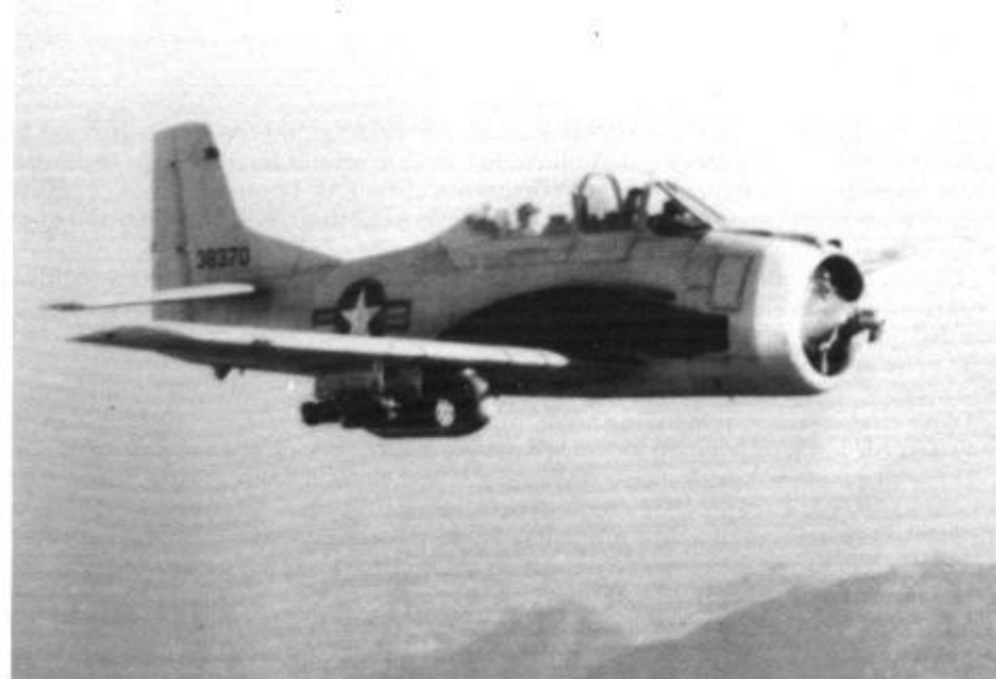
This Farm Gate T-28D (38370) over the Central Highlands near Pleiku during late 1962 is armed with the larger 500 round .50 caliber machine gun pods, seven shot rocket pods, and fragmentation bomb clusters on the outboard pylons. (C. Yarbrough)
