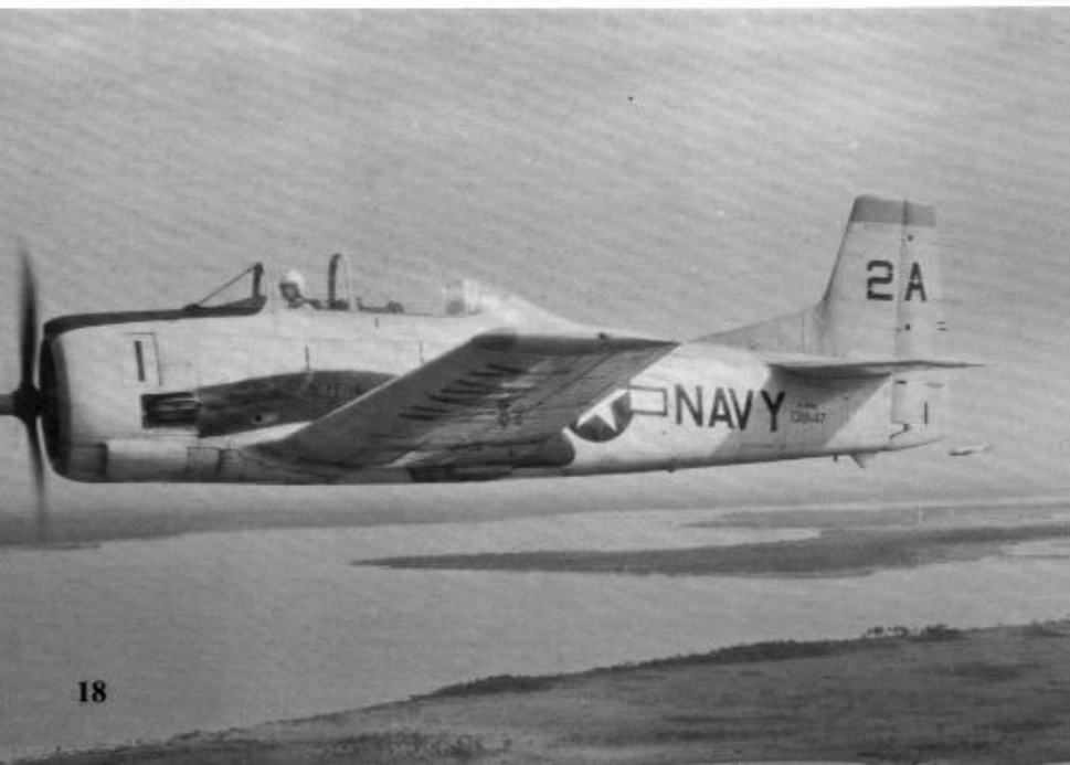
The tail code '2A' indicates that this overall Orange-Yellow T-28B (BuNo 0138147) is assigned to a Fleet Readiness Squadron (FRS) at NAS Pensacola for instrument training duties. (USN)
