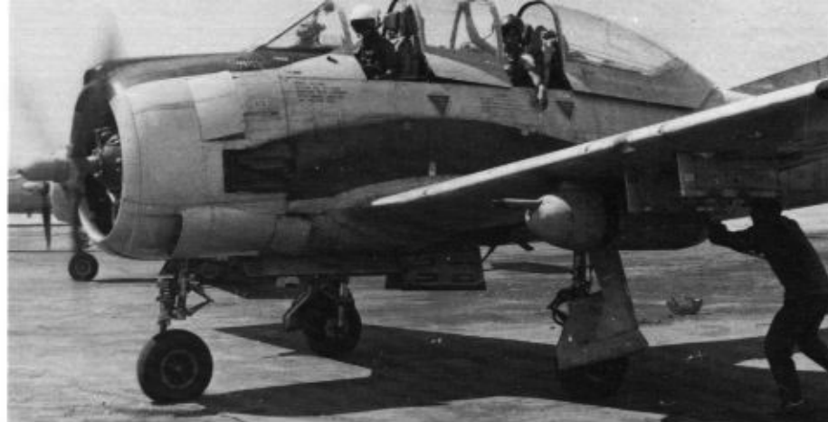
An armorer removes the safety pins from the .50 caliber machine gun pods on this AT-28D of the Philippine Air Force (PAF). The PAF received a number of Fairchild built AT-28Ds equipped with ejection seats, operating them in both the ground attack and training roles. (Carlos L. Agustin)
