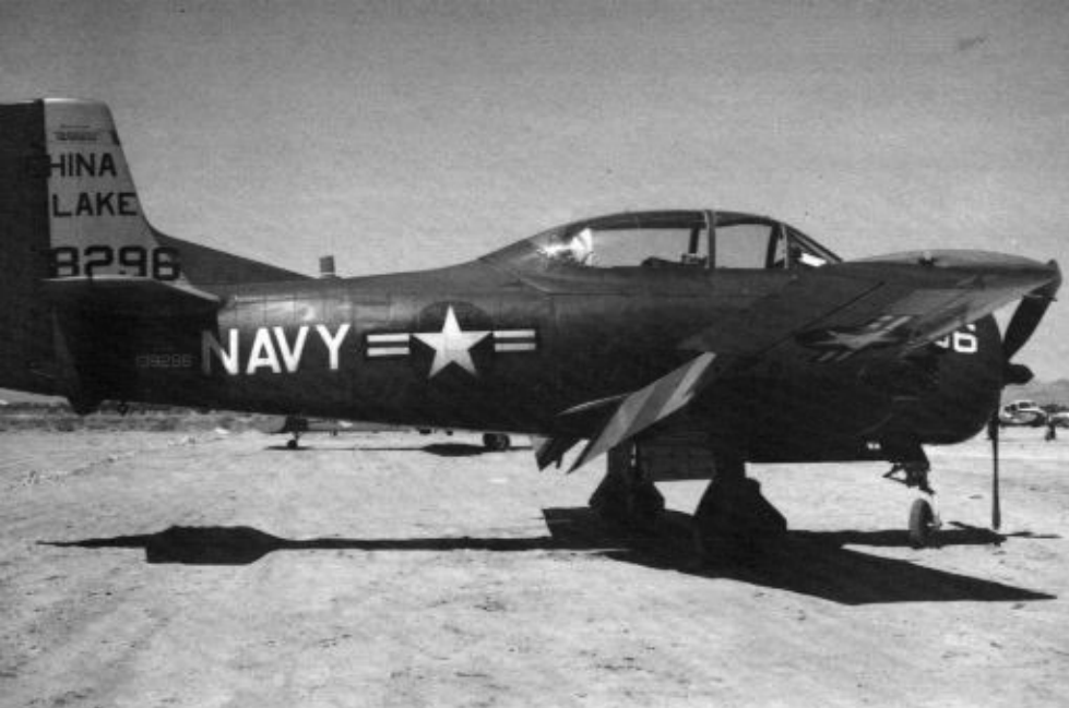
The Navy converted six T-28Bs to drone controllers under the designation T-28BD. This T-28BD (BuNo 138296) of the Naval Weapons Center, NAF China Lake, California, is painted in the standard drone controller scheme consisting of an Engine Gray fuselage; Orange-Yellow wings, horizontal and vertical stabilizers; with Red-Orange wing stripes and rudder. (L.S. Smalley via W.T. Larkins)
