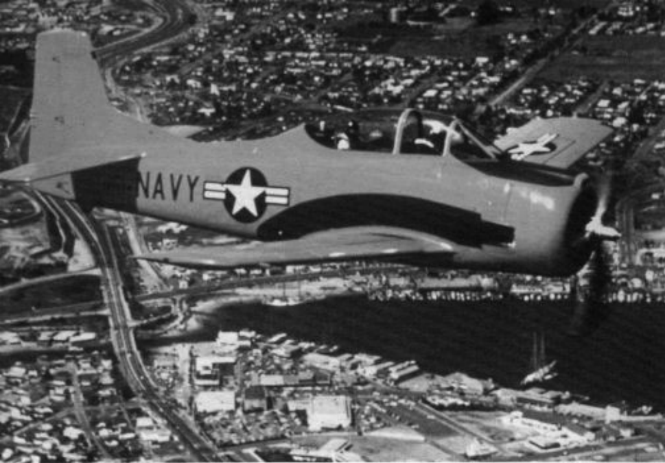
A new production T-28B (BuNo 137724) flies over Columbus, Ohio on an acceptance flight during 1954. The aircraft is overall Orange-Yellow with a non-standard Black anti-glare panel and exhaust area. (Norman Taylor)
