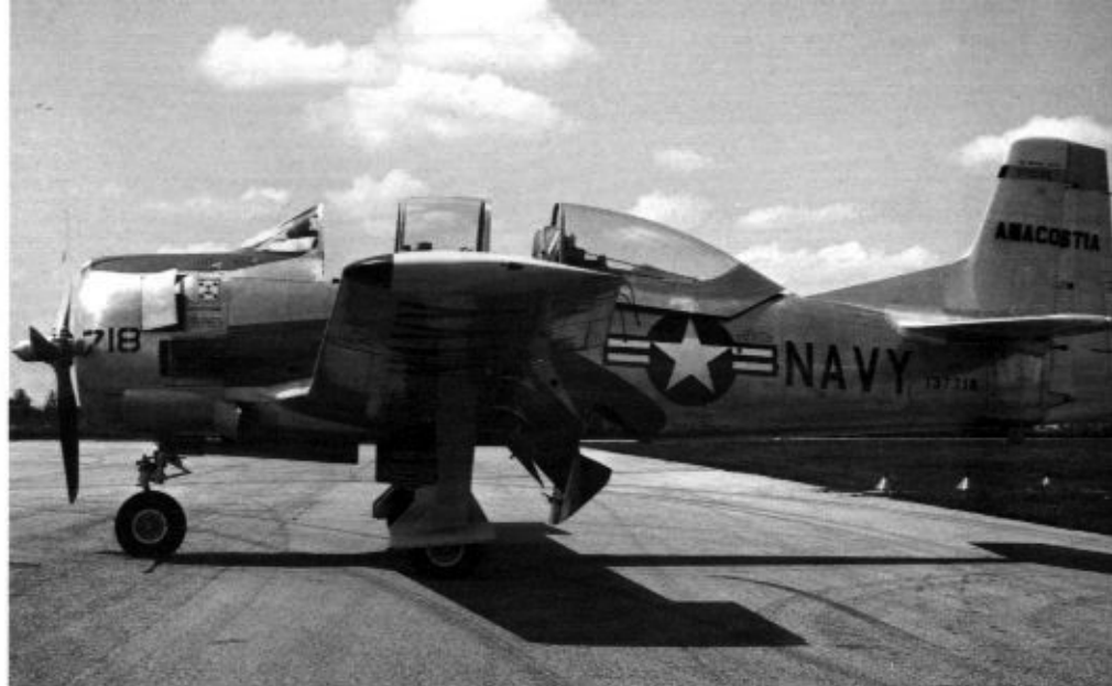
This T-28B (BuNo 137718) on the ramp at NAS Anacostia, Washington D.C., was the personal aircraft of the Assistant Secretary of the Navy for Air and carried his placard, consisting of a fouled anchor and four stars, on the cowling. The open door on the underside of the fuselage is the baggage compartment access door. (G. S. Williams via W.T. Larkins)
