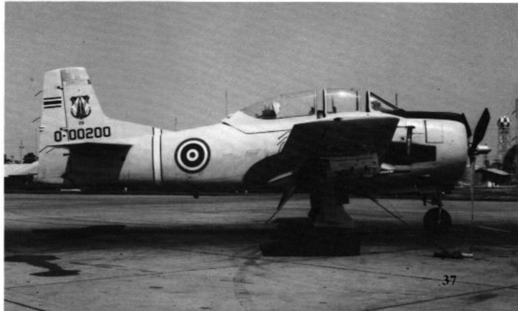
A T-28D-5 (ex-USAF 50-0200) of the 222th Tactical Fighter Squadron, Royal Thai Air Force (RTAF) parked on the ramp at Ubon Royal Thai Air Base. The Trojan is overall Light Gray with the fuselage stripe in White outlined in Dark Blue. The partially open canopy helped lessen the heat buildup in the cockpit under the relentless South East Asian Sun. (Norman Taylor)
