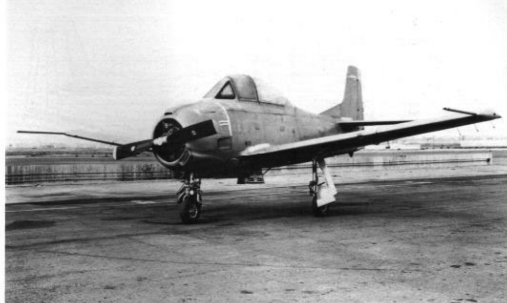
The first XBT-28 prototype (48-1371) was rolled out at the North American plant during September of 1949. The first prototype was fitted with air data probes on each wing tip and an underfuselage speed brake, a feature that would be removed on production aircraft. (National Archives)
