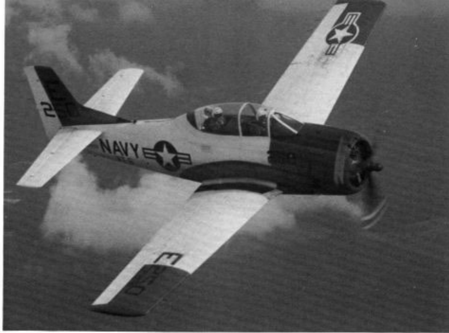
On 12 February 1959 the Navy issued MIL-C-18263B changing the color scheme for single engine trainers to overall Gloss Insignia White with Fluorescent Red Orange high visibility panels. This T-28B (BuNo 138206) of VT-6 at NAS Whiting Field, has been repainted to meet the new requirement. (USN via Norman Hill)
