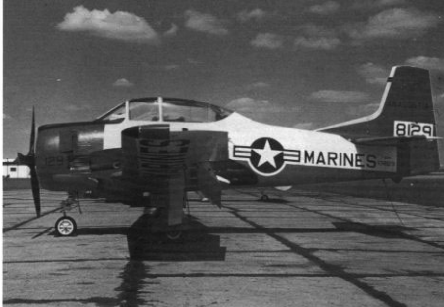
This T-28B (BuNo 138129) was used by the Marines at NAS Anacostia as a hack and carries a decidedly non-standard variation of the Gloss Insignia White and Fluorescent Red-Orange color scheme. The Trojan is also fitted with a sunshade inside the upper canopy. (W.J. Balogh Sr. via D. Menard)
