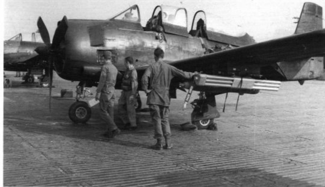
Accompanied by the crew chief, the pilot of this T-28D-5 of the 606th SOS conducts a pre-flight inspection of the Trojan prior to another mission. The T-28 is armed with SUU-14A bomblet dispensers, Mk 81 250 pound GP bombs, and LAU 32/A 2.75 inch rocket pods. (N. Crocker via N. Taylor)
