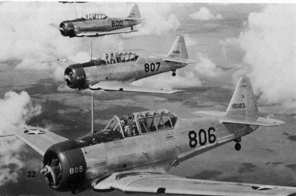
A flight of three Red nosed AT-6As fly formation over Kelly Field during 1943. By 1943 the Red, White, and Blue rudder stripes had been removed from US aircraft, including trainers. These aircraft are not equipped with a pilot's headrest which was normally installed on Army AT-6s. (Taylor)
