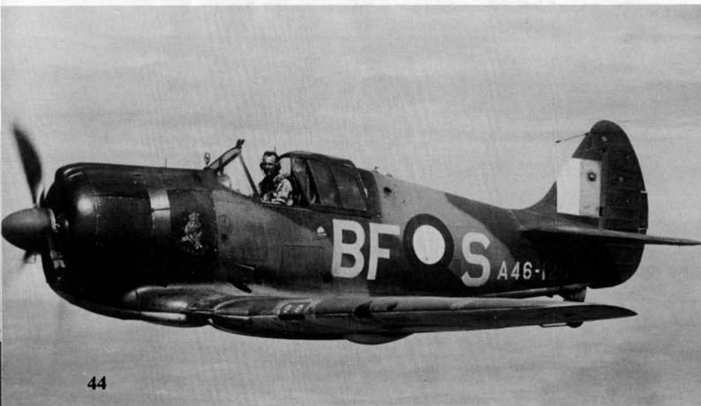
Sinbad II , a Commonwealth CA-13 Boomerang of No 5 Squadron Royal Australian Air Force during 1944. The Boomerang closely resembled the North American-designed P-64, and used a large amount of NA-16/Wirraway technology. It was armed with four .303 machine guns and two 20mm cannon. (AFM)
