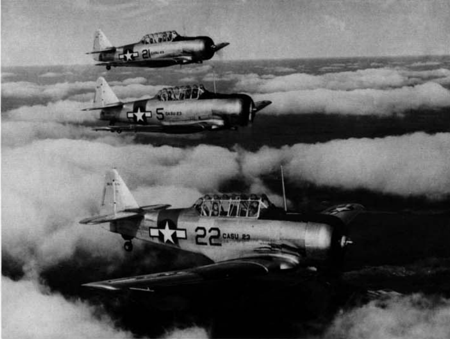
An SNJ-5 flies lead for a pair of SNJ-4s of CASU-23. SNJ-4s and -5s were identical except for their electrical systems and they often served together in the same units. The large Green bands on the wings and fuselage indicate that the Texans are used as instrument trainers. (Larkins)
