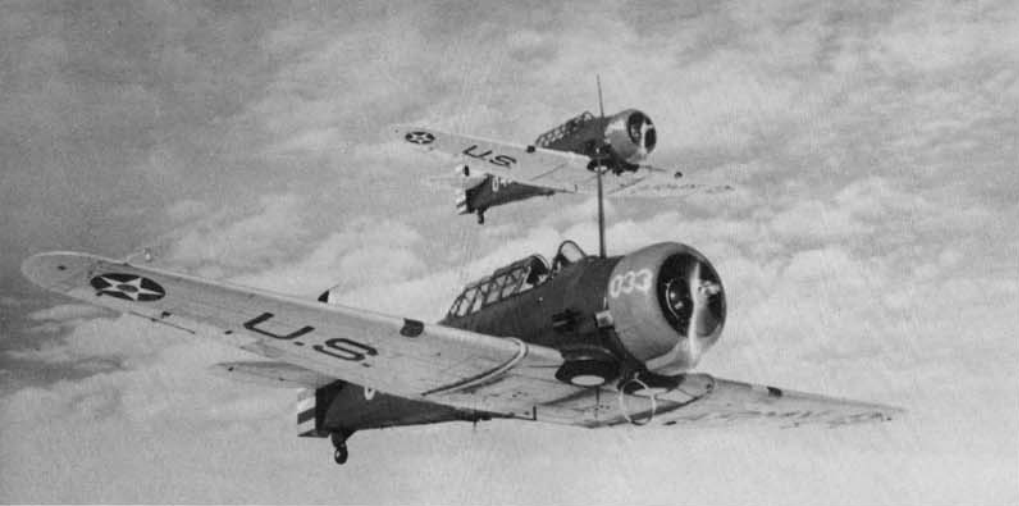
A pair of BC-1s from Randolph Field, Texas fly a practice formation flight during 1941. The distinctive ADF ring antenna just forward of the landing gear was a standard feature of BC-1 and BC-1A aircraft. Both aircraft carry Red cowlings with Yellow numbers. (AFM)
