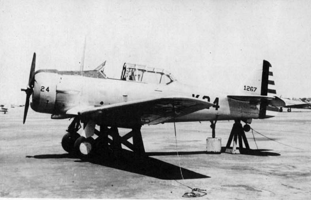
This AT-6A stationed at Stockton Field, California is mounted on jacks for use as an AT-6 cockpit orientation trainer. It was not unusual for a new cadet to pull the wrong handle and fold up the landing gear while sitting on the ramp. By using the cockpit orientation trainer, these incidents were reduced. (Dorr)
