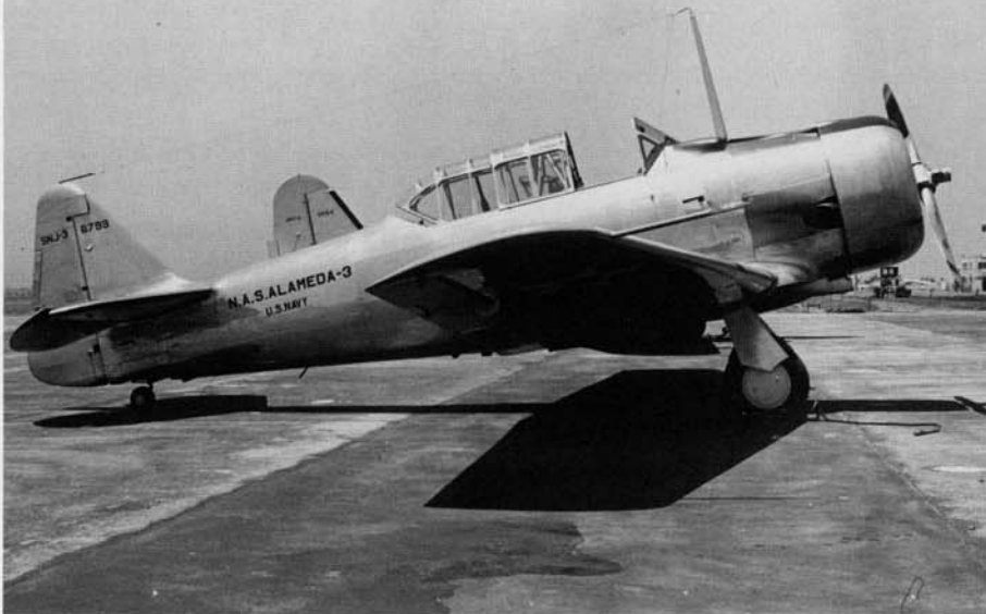
This SNJ-3 was assigned to the Naval Air Station at Alameda, California during 1940. The SNJ-3 was virtually identical to the AT-6A, and was the first T-6 variant to be powered by an -AN engine. The -AN designation meant that the engine was accepted as standard for both Army and Navy use. (Taylor)
