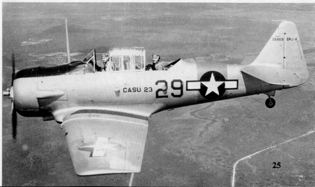
A Navy photographer readies his camera in the rear cockpit of an SNJ-4 of Carrier Air Service Unit (CASU) - 23. Most aircraft carriers had at least one SNJ assigned for use as a hack aircraft while in port. This SNJ has a Red fuselage band identifying it as an instrument trainer. (Dorr)
