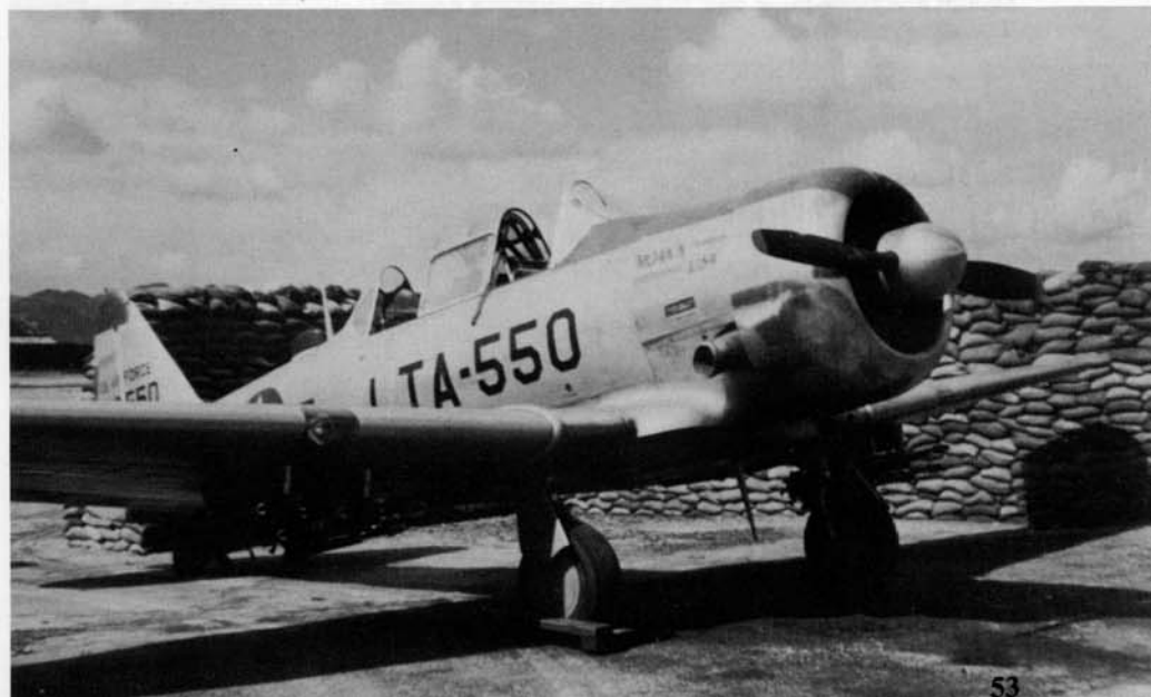
MOANN' LISA , was named because of the strange sounds that came from the air flow over the many patches in her skin. The LT-6G was flown by LT Gene Risedorph out of Chunchon during 1953. LT-6Gs were specially modified and armed T-6Gs built for the Mosquito mission in Korea. (Risedorph)
