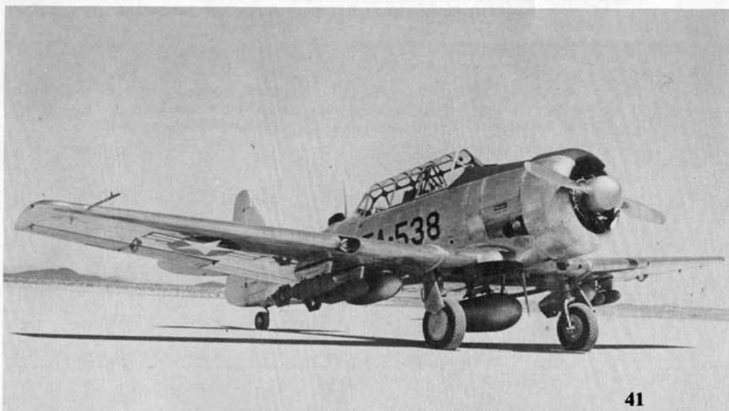
This T-6G (49-3538) was modified by North American for the counter-insurgency (COIN) role under the designation FT-6G. The aircraft mounted two .30 caliber machine gun pods under the wings and up to 400 pounds of ordnance on underwing racks. (Larkins)
