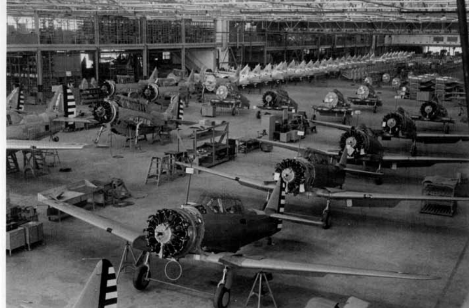
North American's plant at Inglewood, California was building BC-1 trainers and O-47A observation aircraft simultaneously. Between 1937 and 1940 North American built a total of 177 BC-1s and 239 O-47As. (AFM)
