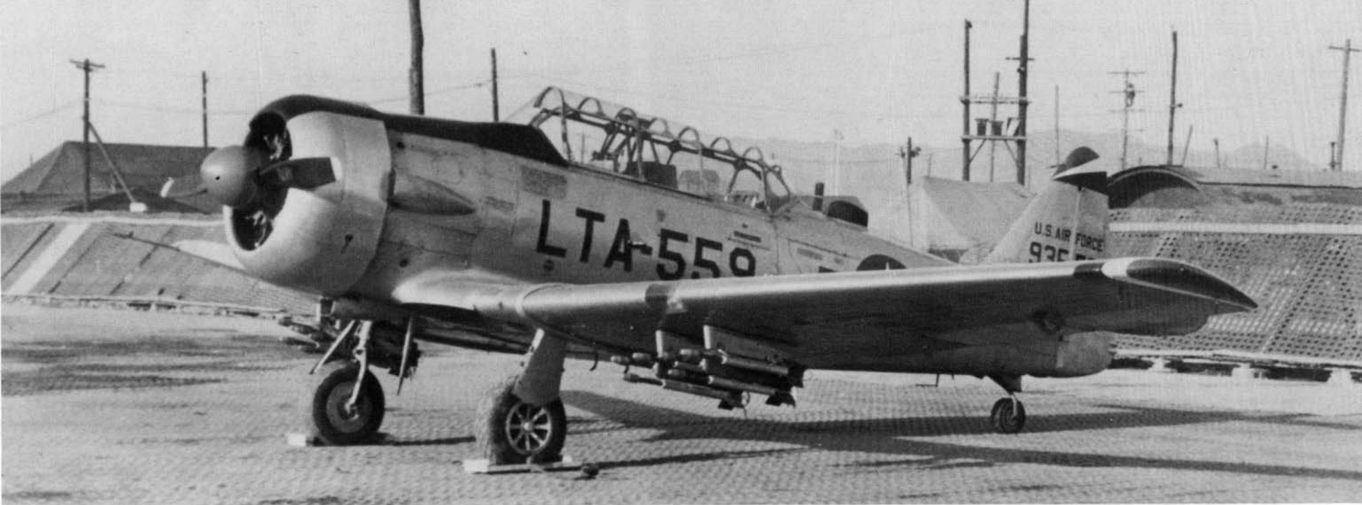
A fully armed LT-6G on the Chunchon ramp during 1953 ready for its next mission. The aircraft is fitted with multiple rocket launchers, a TACAN blade antenna behind the canopy, and another antenna mast between the landing gear wells. Wingtip and fin colors are Red, White, and Blue for the 6148th TCS(A). (NAA)
