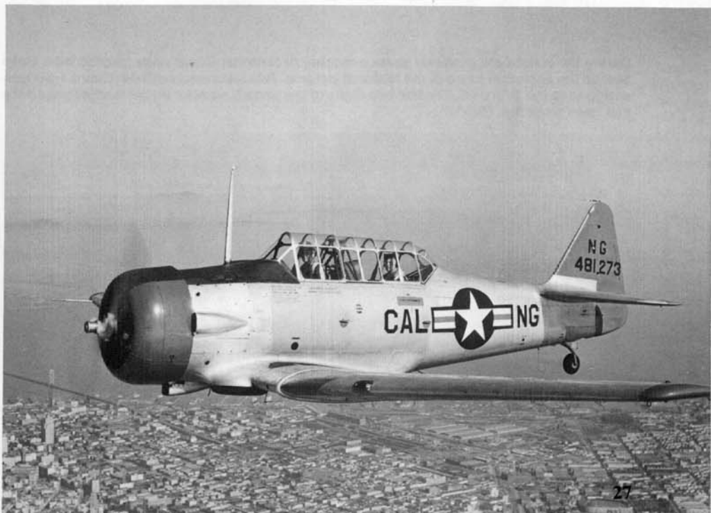
A T-6D instrument trainer of the California Air National Guard flies over San Francisco during October of 1949. Instrument trainers had canvas hoods that completely covered the pilot that was taking the instrument course. The aircraft is overall natural metal with the cowling, vertical tail, wingtips, and instrument trainer wing bands in Red. (Larkins)
