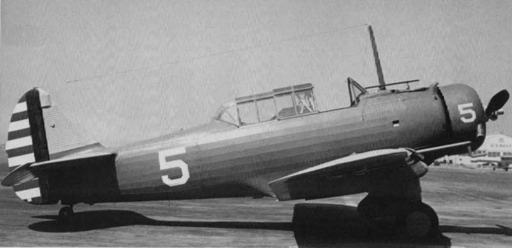
The BT-9C was an improved version of the BT-9A with wing leading edge slats, a single .30 caliber machine gun mounted in the cowl, and a telescopic gun sight for the pilot. North American built thirty-two BT-9Cs specifically for the U.S. Army Organized Reserve. (Larkins)
