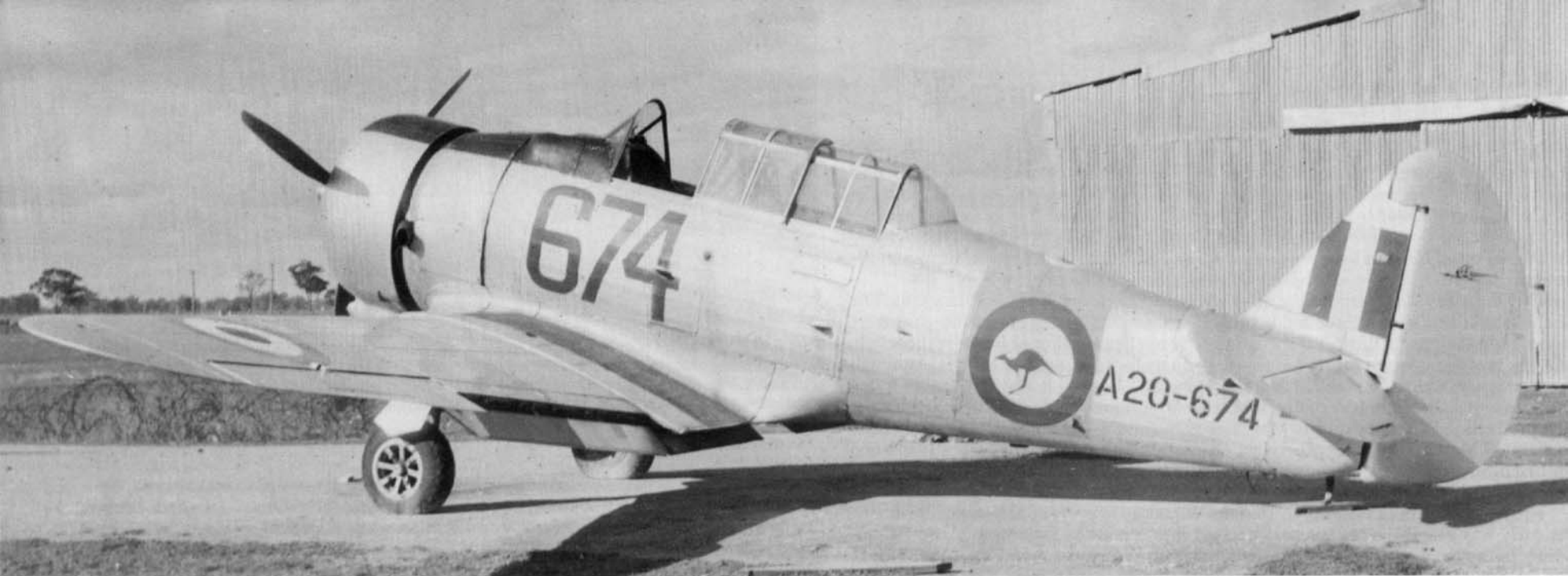
This Royal Australian Air Force CA-16 Wirraway at RAAF Toluwal during September of 1961 carries the post-war RAAF Kangaroo markings. Although rebuilt after the war and brought up to standards similar to those of the T-6G, the Wirraway retained its fabric-covered fuselage. (Dorr)
