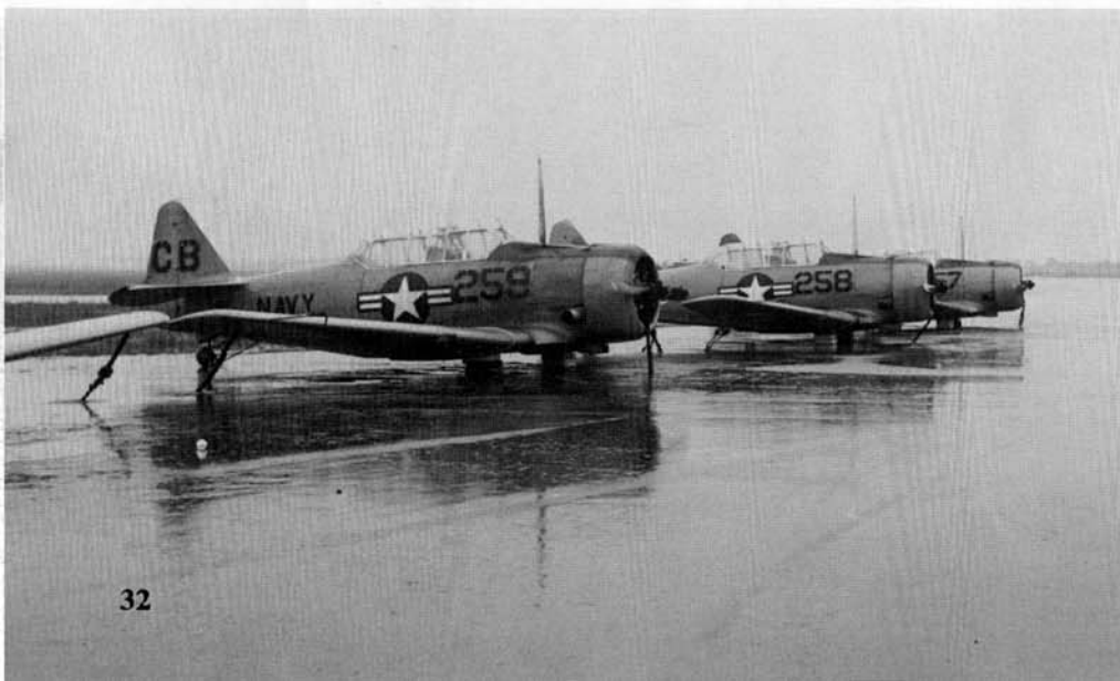
These SNJ-5s have been lowered onto stacks of tires, then lashed down to the ramp in preparation for a hurricane or tropical storm at NAS Corry Field, Florida. A crane would hoist the aircraft up while a mechanic retracted the landing gear, then the aircraft was lowered onto the tires and lashed down. (John Kirk)
