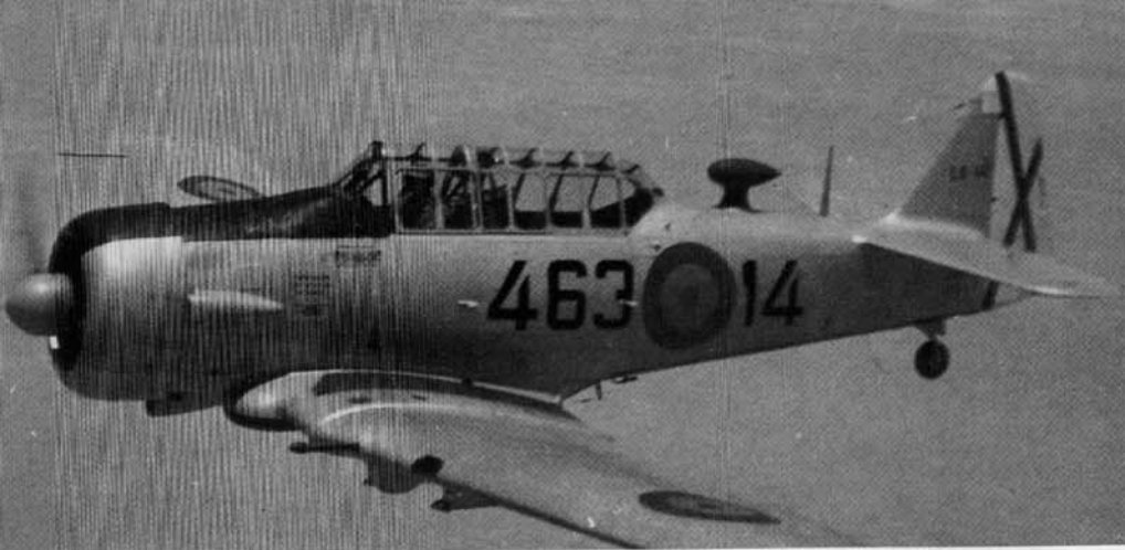
Spanish Air Force C.6 (T-6C/D) and E.16 (T-6G) flew armed anti-guerrilla missions over the Spanish Sahara desert provinces during the 1970s. Spanish aircraft were armed with .30 caliber machine guns in both wings, and underwing racks for rockets and bombs. (Luenco)
