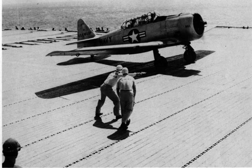
The flight deck officer gives the launch signal to the pilot of this SNJ-5C aboard USS WASP. Carriers had SNJs assigned as hacks/utility aircraft; however, they did not usually take them on deployment. The suffix C in the Texan's designation indicated that it was a tail hook equipped SNJ. (Larkins)
