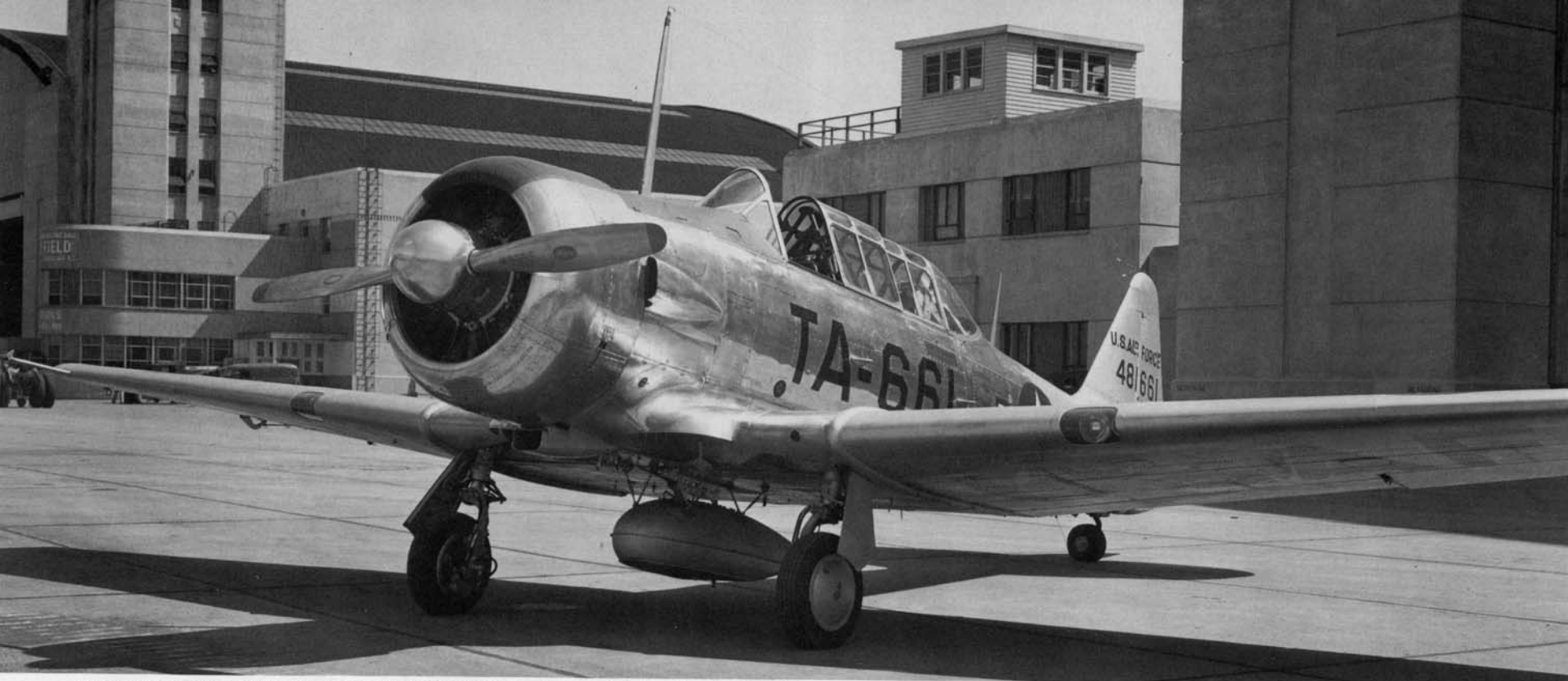
This well maintained T-6F was used at Wright Field to test several styles of centerline drop tanks. A twenty gallon tank was later adopted as a standard piece of equipment on the T-6G/LT-6G. This drop tank is an experimental fifty-five gallon tank. (Larkins)
