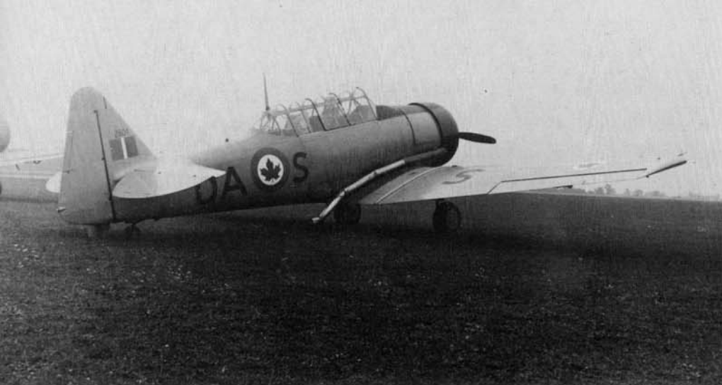
This CCF-built Royal Canadian Air Force Harvard IIB has an unusually long exhaust shroud which extends back over the wing trailing edge. The aircraft was painted in overall Trainer Yellow with the cowling in Red. (Balogh)
