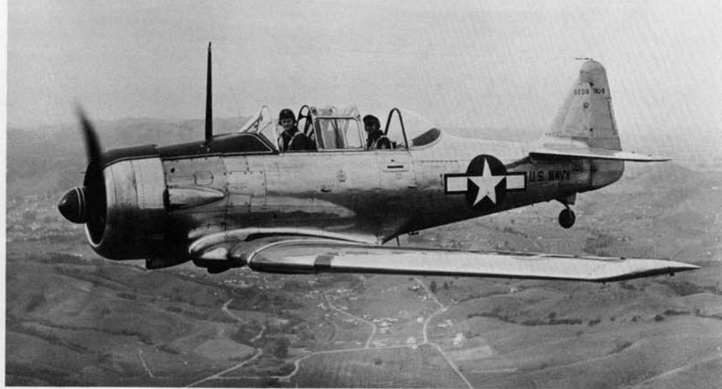
This highly polished SNJ-6 was the Commander's aircraft at Naval Air Station Alameda during 1947. The SNJ-6 was the Navy designation for the AT-6F. The propeller spinner and antiglare panel are gloss Dark Blue with Gold and Dark Blue striping. (Larkins)
