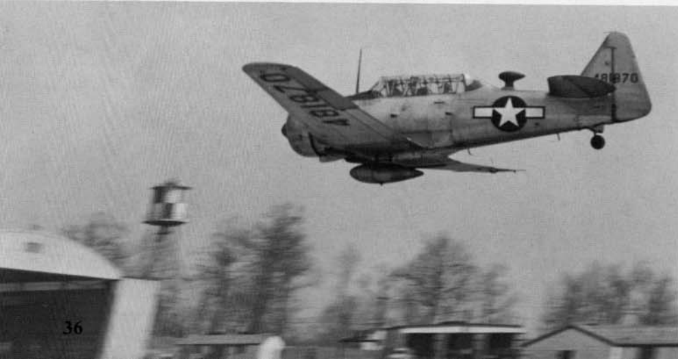
An AT-6F buzzes the ramp at Coreopolis Army Air Force Base during 1946. The AT-6F was the first variant to have provisions for carrying a belly tank and usually carried a twenty gallon tank on the fuselage centerline. (Balogh via Menard)
