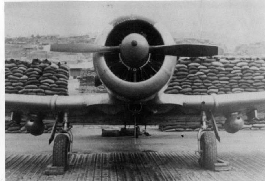
This T-6 at K-47 (Chunchon) during 1951 is armed with two underwing .30 caliber machine gun pods. The gun pods were usually removed to lighten the aircraft and improve performance. Additionally, senior officers did not want the FAC pilots engaging targets themselves instead of calling in strike aircraft. (Mosquito Association)
