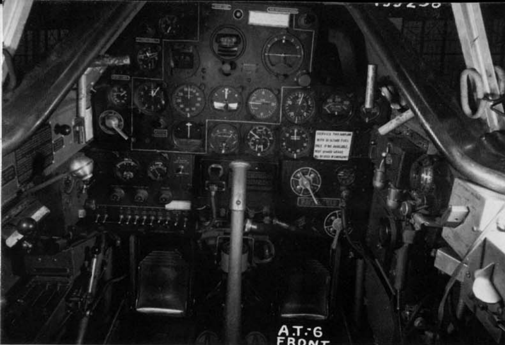
The front instrument panel of an AT-6C Texan. The placard on the right corner of the panel reads: "Service this airplane with 91 octane fuel only, if not available, next higher grade will be used in an emergency." (AFM)
