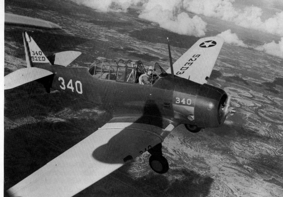
This BT-14 of the 52nd School Squadron carries a full set of school identification markings on the upper left and lower right wing in Black. These markings were displayed prominently so that civilians could identify any low flying aircraft over a populated area. This practice led to the term — buzz number. (Taylor)
