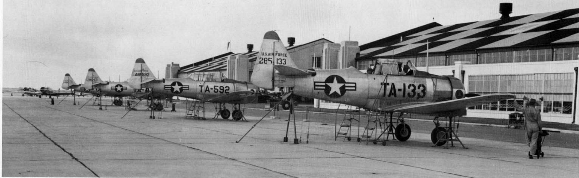
A quartet of T-6Ds assigned to Randolph AFB rest on jacks in preparation for cockpit orientation tests. When Congress created the U.S. Air Force during 1947, the Air Force immediately changed all the former Army Air Force designations, dropping the Advanced from AT-6 changing the designation to simply T-6D. (Ed Galbraith via Menard)
