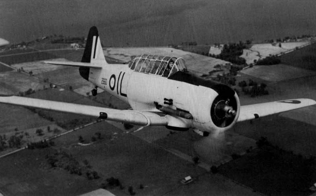
This Harvard Mk IIB of the Royal Canadian Air Force is painted overall Trainer Yellow. The aircraft is fitted with an extended exhaust shroud and two venturi tubes on the fuselage side above the exhaust. Unlike RAF Harvards, Noorduyn-built aircraft had American instruments and controls. (RCAF via Dorr)
