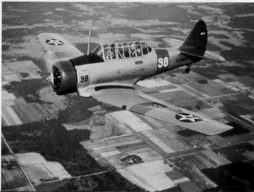
An SNJ-1 instrument trainer on a training mission during 1940. Navy trainer paint schemes were very colorful and consisted of a natural metal fuselage and wing undersurface, Yellow upper wing surfaces, Red cowling and tail, and a Black anti-glare panel. Instrument trainers carried a Red band around the fuselage and wings. (Starinchak)
