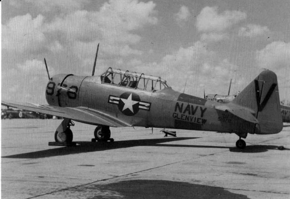
A pair of SNJ-5s parked on the ramp at NAS Glenview during 1956. Each naval air station was assigned a code letter which was painted on the vertical tail, upper starboard and lower port wings. Additionally, all Reserve units had International Orange bands around the rear fuselage. (Menard)
