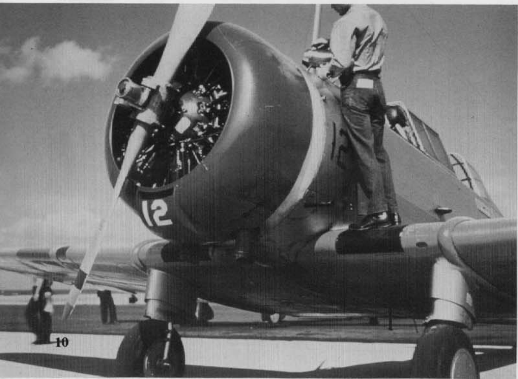
The BT-9 was selected by the Navy to be its standard trainer under the designation NJ-1. The NJ-1 differed from the BT-9 in having a Navy-specified 500 hp Pratt & Whitney R-1340-6 Wasp engine, and a modified cowl with the exhaust exiting through two stacks under the cowl. (Starinchak)
