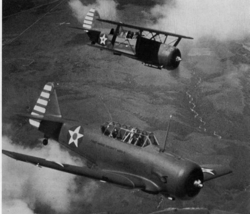
An SNJ-3 and SBC-4 Helldiver of the First Marine Aircraft Wing fly together near Quantico, Virginia. Both aircraft are camouflaged with Intermediate Blue Gray uppersurfaces over Light Gray undersurfaces. The SNJ-3 was used as a gunnery trainer, while the SBC-4 was used in the dive bomber training role. (Starinchak)
