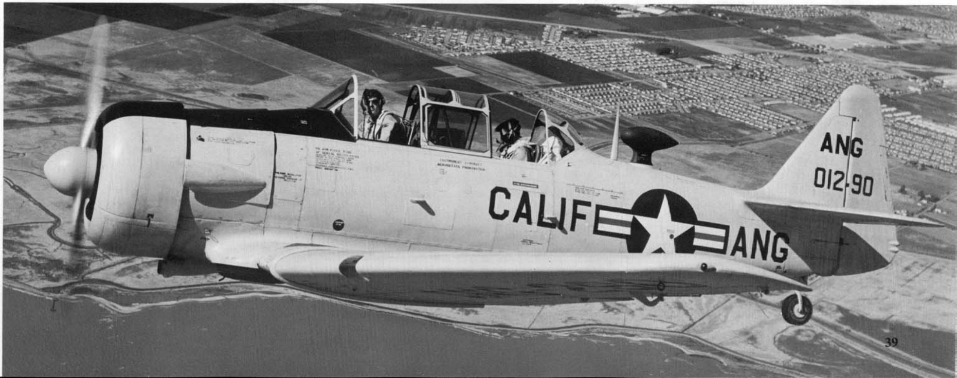
(Below) A T-6G of California Air National Guard flies over Hayward, California during 1953. The T-6G featured dual rear position lights on the lower rudder and a football ADF housing behind the cockpit. The lettering under the center canopy reads: Instrument Aircraft - Aerobatics Prohibited. (Larkins)
