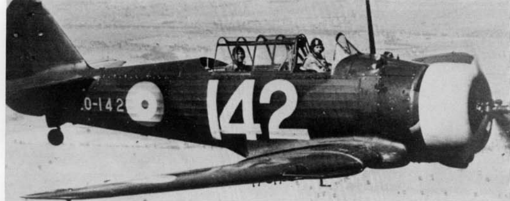
This RAAF Wirraway is camouflaged in Dark Earth and Foliage Green uppersurfaces with Aluminum undersurfaces. During the early days of the Pacific War, the Wirraway was pressed into service as a two seat fighter, fighter-bomber, and observation aircraft. One Wirraway pilot is credited with a kill, a Japanese Zero fighter. (IWM)
