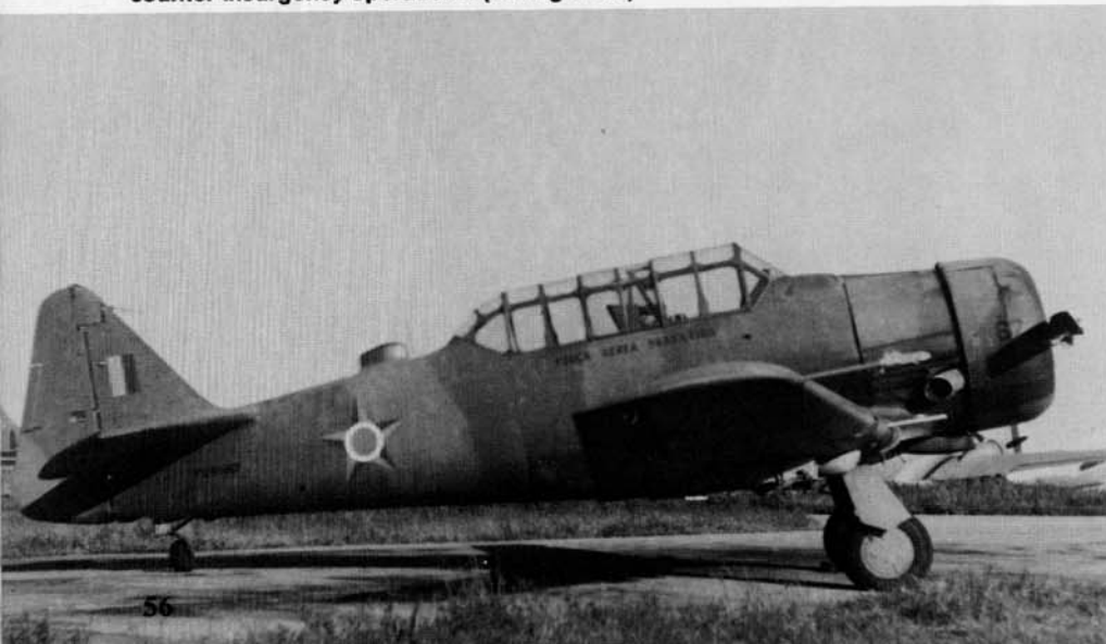
This camouflaged T-6 of the Brazilian Air Force is fitted with underwing racks for rockets and/or small bombs. The Brazilians used large numbers of T-6s, both in the training role and for counter-insurgency operations. (D. Hagedorn)
