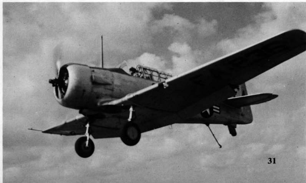
This SNJ pilot on final approach to USS WRIGHT during 1948 has the hook down to catch the carrier's arresting wire. Arrested landings were required as part of his Carrier Qualification. This SNJ has had the landing gear doors removed since they were often lost during carrier landings. (Ron Gerdes via Larkins)
