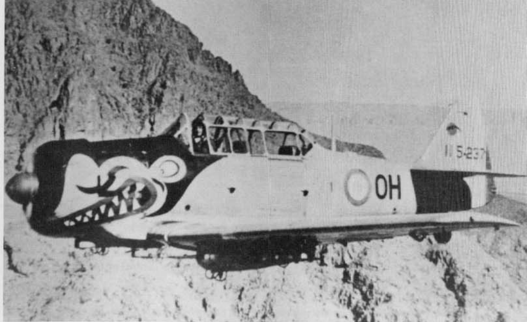
A French Air Force T-6G of 5/72 Ground Support Light Squadron (EALA) flies over Algeria during the late 1950s. The French used armed T-6s and Harvards for missions against Algerian guerrilla forces. French T-6s had underwing .30 caliber gun pods, and racks for bombs and/or rockets, a direct result of the FT-6G program. (Bertrand)
