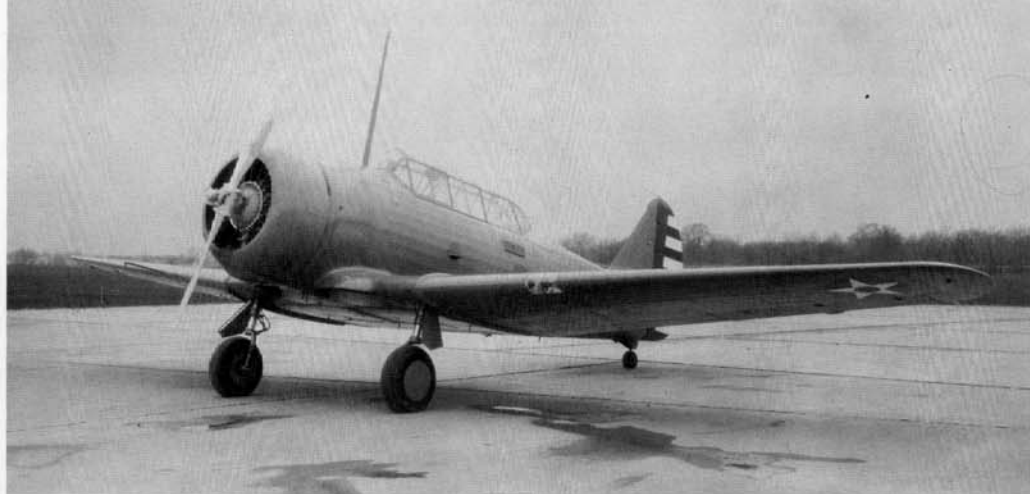
The North American NA-36 was the prototype for the BC-1 trainer series. It featured a fully retractable landing gear and was powered by a 600 hp Pratt and Whitney R-1340-S3H1 air cooled radial engine. The Army originally designated the prototype as the BT-9D. (AFM)
