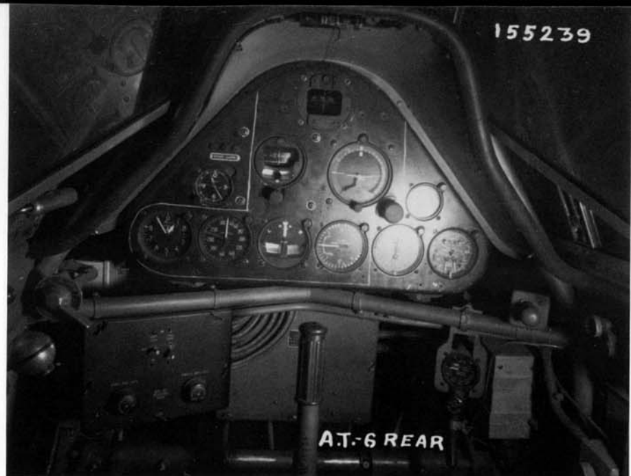
The instrument panel installed in the rear cockpit of the AT-6C. The cockpit color of the AT-6C was Interior Green with Black instrument panels, controls and radios. (AFM)
