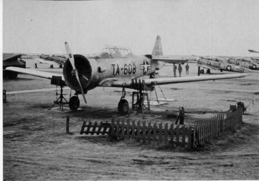
A "CAPTIVAIR" T-6D at Perrin Air Force Base. The "CAPTIVAIR" system allowed a cadet to literally "fly" the aircraft, getting a feel for everything in the cockpit, without actually leaving the ground. The enlarged cowling and cooling fan kept the engine from overheating during ground runups. (Merritt via Menard)
