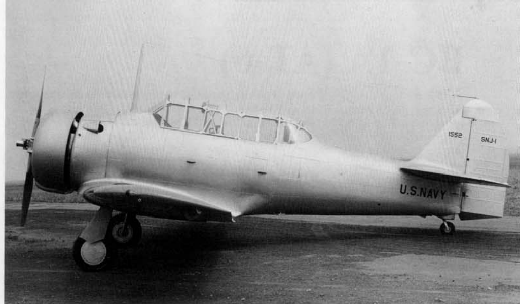
The SNJ-1 was the first variant to combine the all-metal fuselage of the BT-14, retractable landing gear, and 500 hp Pratt & Whitney R-1340 Wasp engine. This SNJ-1 (BuNo 1552) was the first of sixteen SNJ-1s built for the Navy. (Larkins)
