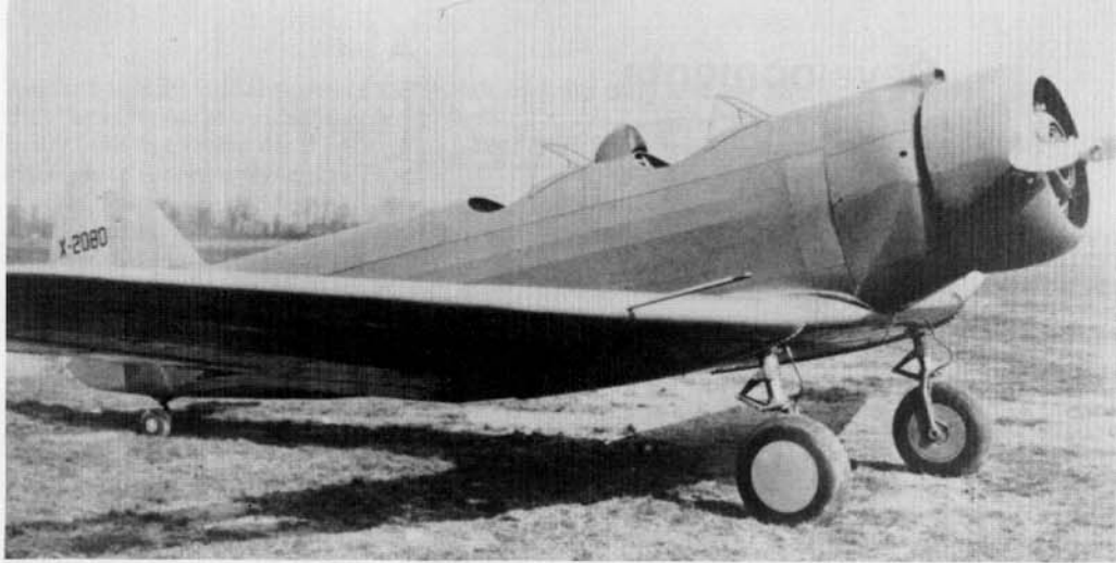
The North American NA-16 prototype featured open cockpits and fixed landing gear, which were traditional for Army basic trainers. The NA-16 prototype, registered X-2080, won the Army's 1935 Basic Trainer Competition. (NAA)
