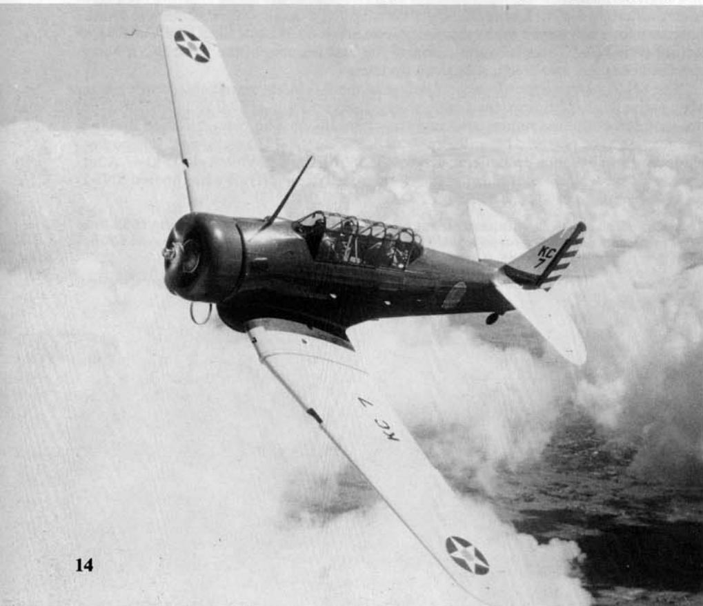
This BC-1 was assigned to the 3rd Air Base Squadron at Selfridge Field, Michigan. The distinctive shape of the NA-16 wing closely resembled that of a scaled down DC-2/3 airliner wing (which is understandable since its designers were ex-Douglas engineers). (AFM)
