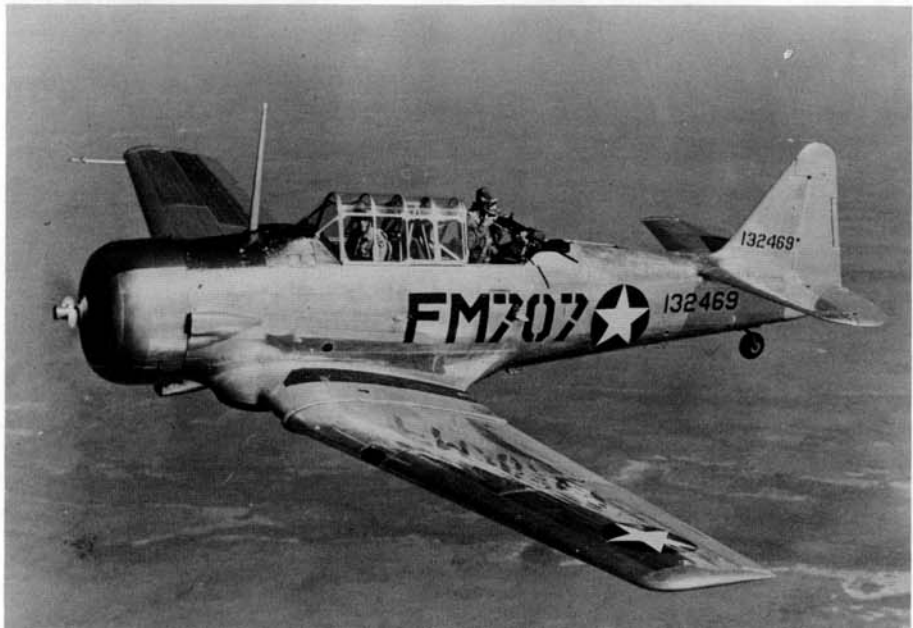
A student gunner takes aim from the rear cockpit of an AT-6C gunnery trainer based at Fort Myers (base code FM), Florida, during 1942. Bomber gunners trained in the rear cockpit of AT-6s before graduating to bombers. The slot in the upper rear fuselage was used to store the .30 caliber machine gun when not in use. (Larkins)
