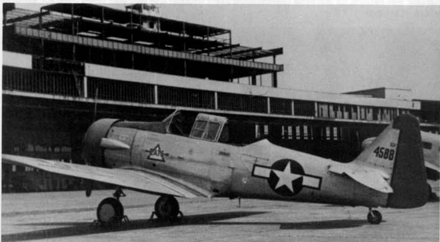
An AT-6D of the European Air Transport Service on the ramp at Berlin's Tempelhof Airport during 1946. The AT-6D was externally identical to the AT-6C, the main difference being the electrical system. The AT-6C had a 12 volt system while the T-6D had a 24 volt system. The cowling and rudder of this Texan is in Medium Blue. (AFM)
