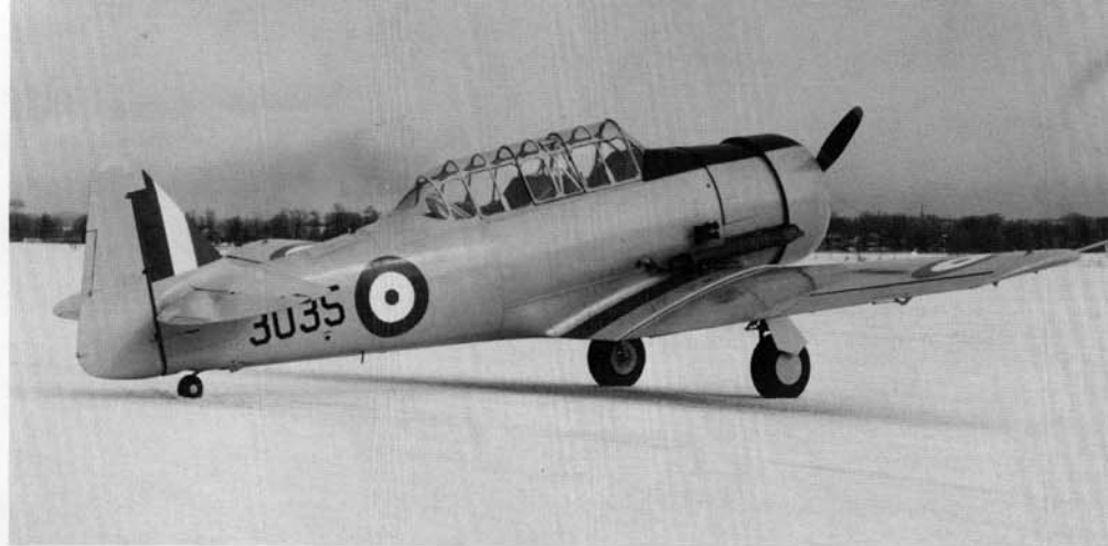
Noorduyn Aviation in Canada built a total of 2,910 Harvard Mk IIBs for the RAF, RCAF, and U.S. Army Air Force (under the designation AT-16). The extended exhaust shroud was designed to feed heated air into the cockpit to increase cabin heat in cold weather. (Noorduyn via Larkins)
