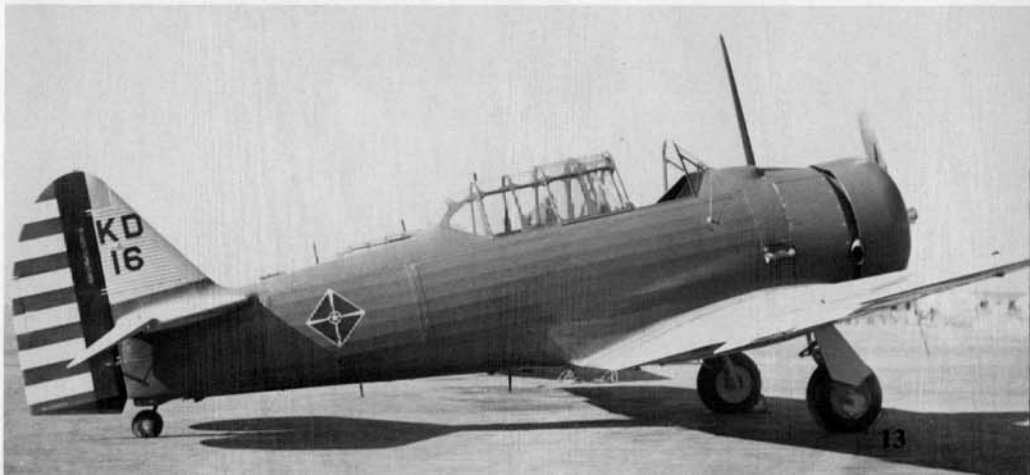
This BC-1 of the 4th Air Base Squadron was based at March Field, California during 1938. The BC-1 retained the fabric-covered fuselage of the BT-9 series and was powered by the 500 hp Pratt & Whitney Wasp engine. (Larkins)
