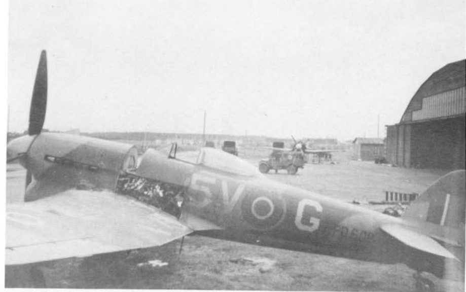
A Typhoon IB (PD608) of No 439 Squadron undergoes maintenance at a forward airfield during early 1945. The aircraft carries late war RAF markings with the Sky fuselage band being deleted and a four color upper wing roundel being used (this roundel was introduced on 3 January 1945).
