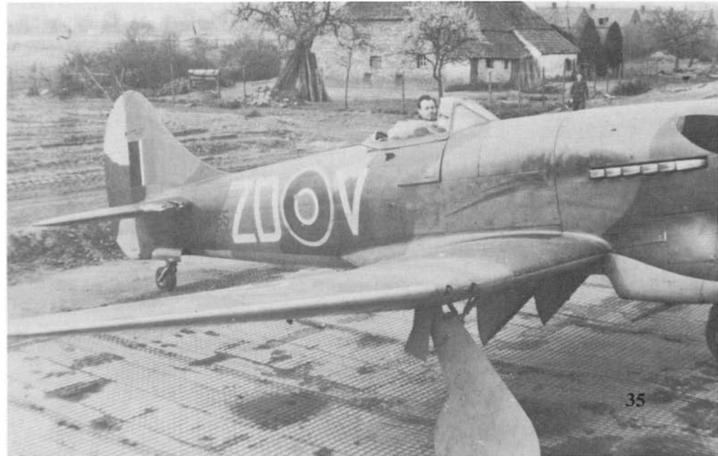
This Tempest V (SN165) of No 222 Squadron on the ramp at Quackenbruck, Germany, during 1945, has had the elevator and canopy damaged by flak. The aircraft already had a replacement rudder taken from an aircraft with a different camouflage pattern.
