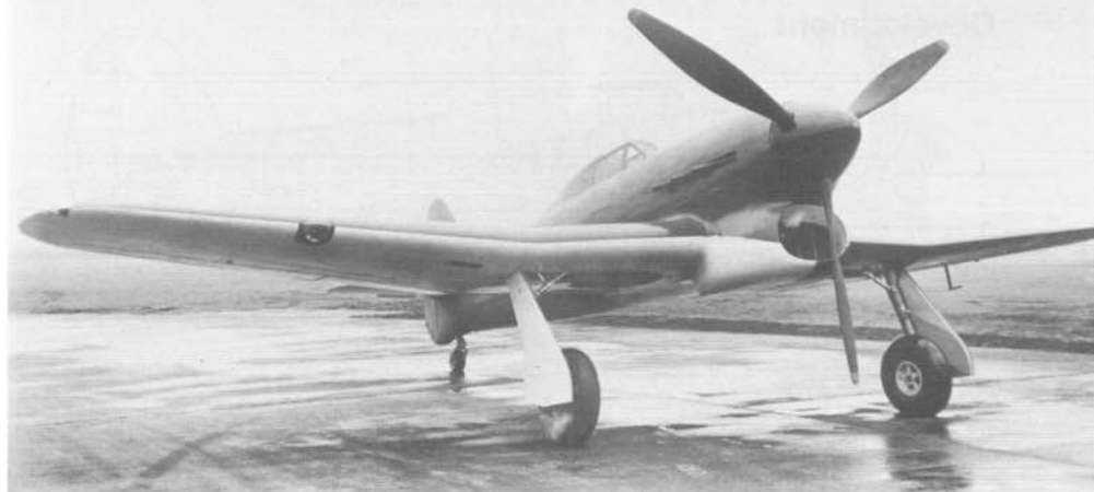
The first Typhoon prototype (P5212) was powered by a 2,020 hp Napier Sabre I engine and made its first flight on 24 February 1940 with Hawker test pilot Philip Lucas at the controls.
