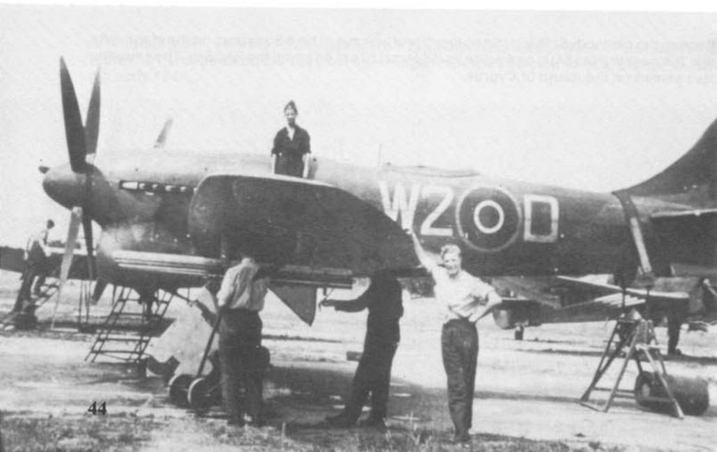
Ground crewmen work on a Tempest VI of No 80 Squadron. The men are aligning the four cannons of the Tempest to converge at a given range for ground attack missions.
