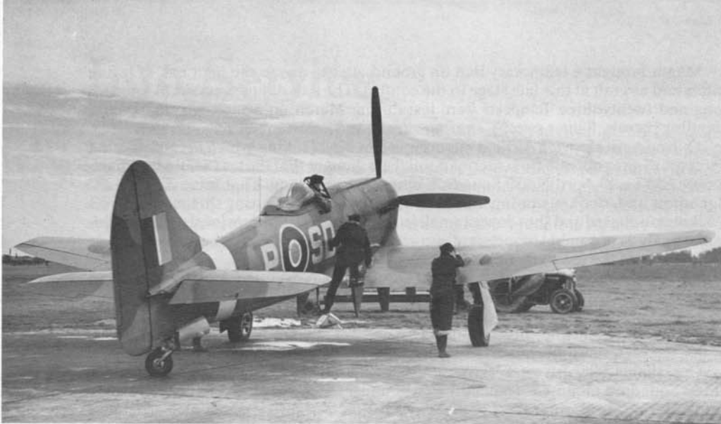
On 19 October 1944, the British public was informed by the newspapers that the RAF had a potent new fighter. This Tempest Mk V (EJ608) of No 501 Squadron at Bradwell Bay, was one of the aircraft featured in the announcements and carries the recently introduced forty-five gallon streamlined drop tanks.
