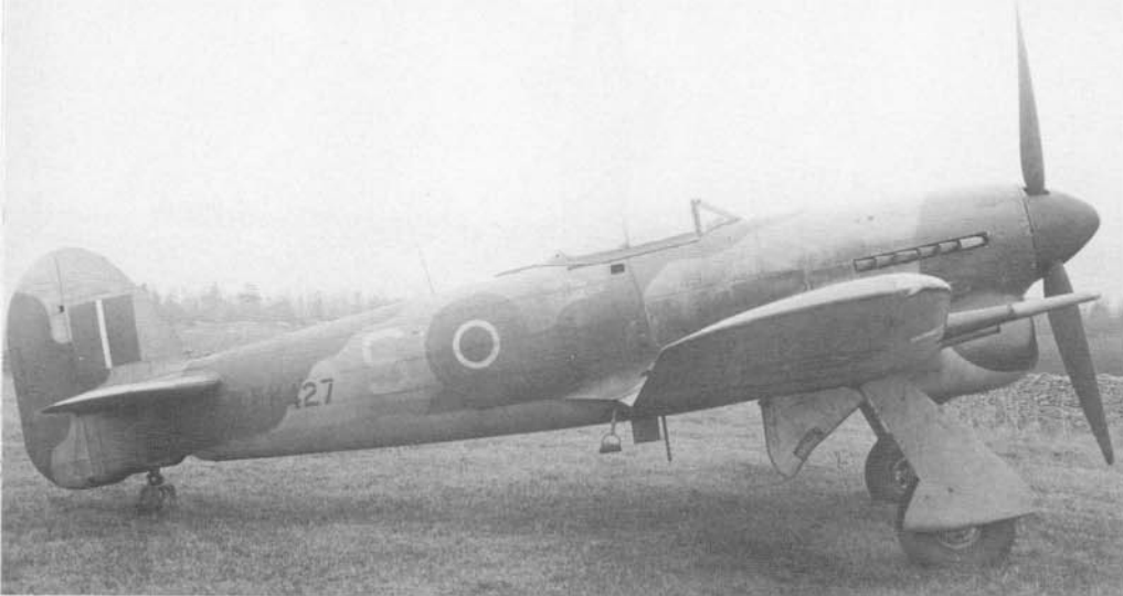
A number of Typhoons were modified for the reconnaissance role under the designation Typhoon PR Mk IB. This PR Mk IB (EK427) of No 4 Squadron during March of 1945 has a camera replacing the starboard inboard cannon.
