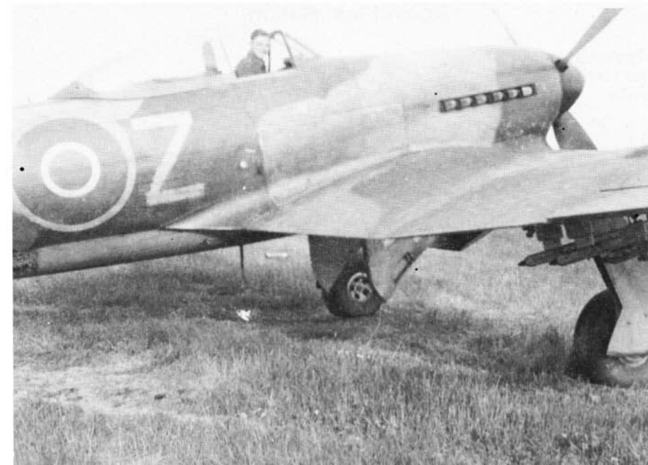
This Typhoon IB of No 137 Squadron is fitted with a four blade propeller and late style under wing rocket rails. Later, it was found that these long launch rails were unnecessary on high speed fighters.
