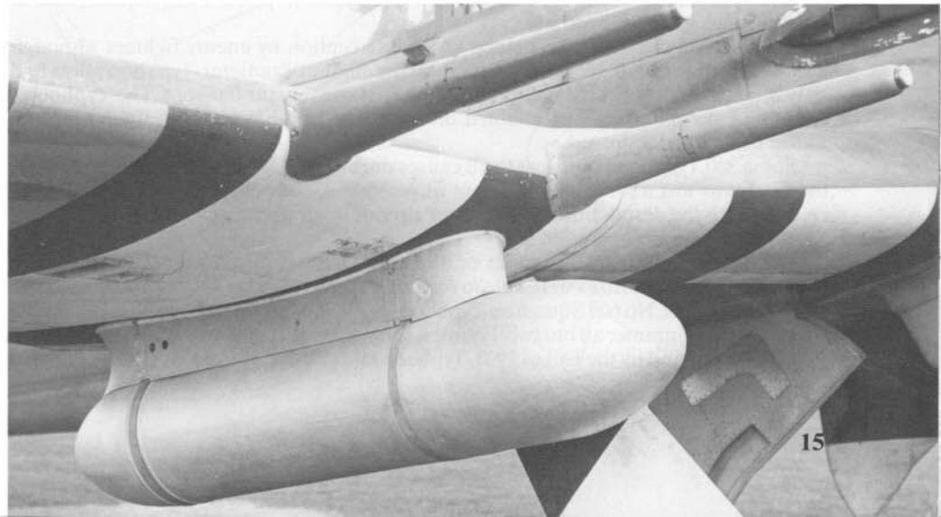
This forty-four gallon Hurricane type under wing drop tank was the first type of drop tank cleared to be carried on the Typhoon IB. The fully faired cannon barrels have two sections, with the front section being easily removed for servicing.
