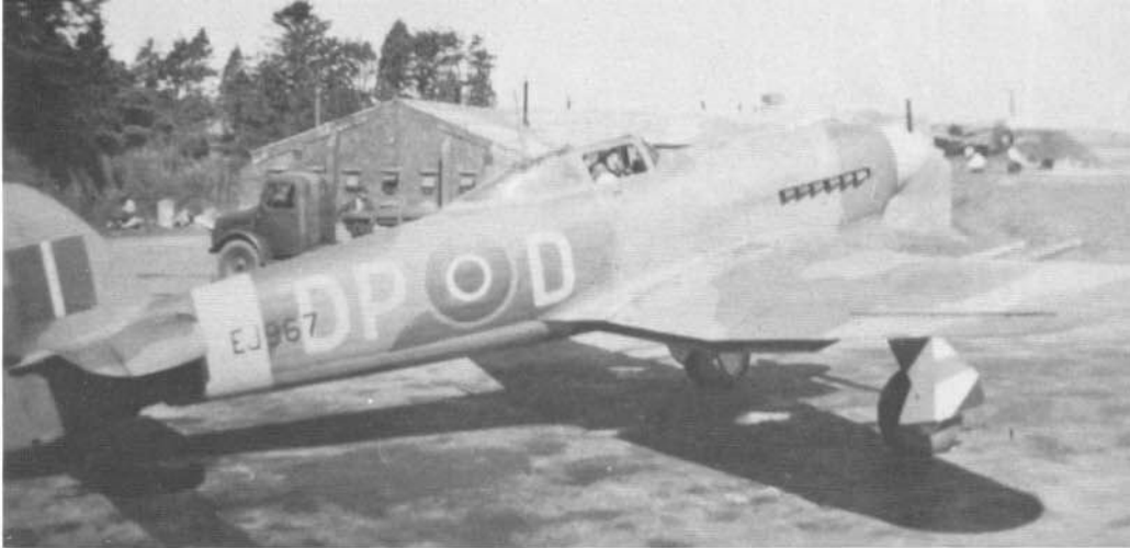
A Typhoon IB (EJ967) of No 193 Squadron prepares to taxi from its dispersal parking spot at Harrowbeer, Devon, during March of 1943. The aircraft has Black and White stripes on the wing undersurface which were added to the Typhoon as a recognition aid.
