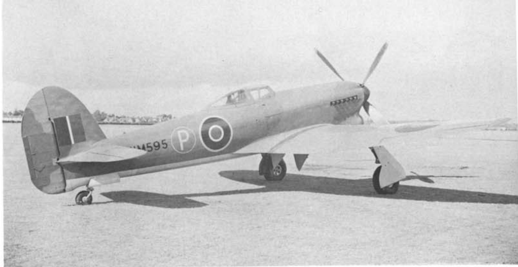
This Typhoon (HM595) was used as a prototype for the Tempest program. The aircraft has not yet been fully converted and retains the Typhoon's car door type pilot entry and early style canopy.
