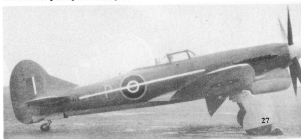
As part of the Tempest program HM595 was fitted with a fin fillet in front of the vertical stabilizer. The white line on the fuselage was a painted datum line used for photographic reference during filming of the test flights.
