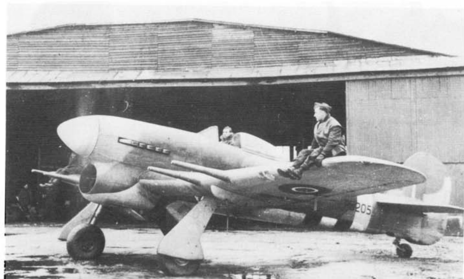
Wing Commander F. G. Grant, commander of No 143 Canadian Wing taxis in at Eindhoven during late 1944. The two ground crewmen riding on the wing directed the pilot, who could not see over the cowlings of the Typhoon. This aircraft (RB205) carried Grant's initials as its identification markings.
