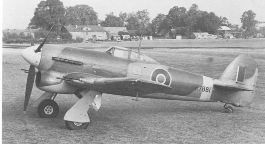
This early Typhoon IB is armed with four Hispano 20MM cannons with unfaired gun barrels, similar to the mounting found on the Hawker Hurricane IIC. The solid fairing behind the cockpit has been replaced by a fixed clear fairing which greatly improved the pilot's rearward view.
