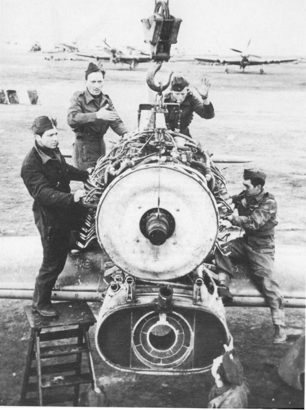
Five maintenance fitters lift the Sabre engine from a Typhoon IB at Eindhoven, Holland. The large pipe protruding above the radiator was the main connection line between the engine and the radiator.
