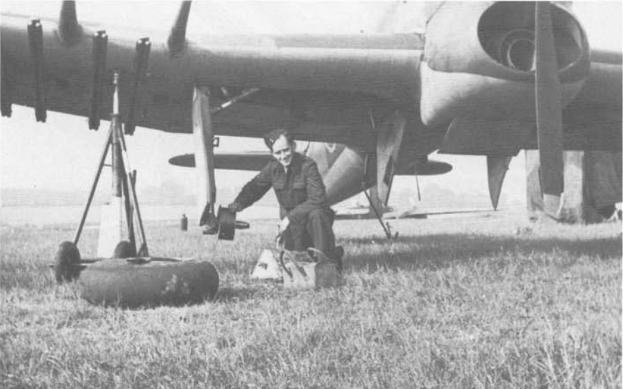
An RAF aircraftsman changes the starboard main landing gear wheel of a Typhoon IB. The rack stand point is between the two inner rocket racks. These racks are the early MK I type with two round launch rails below the rack.
