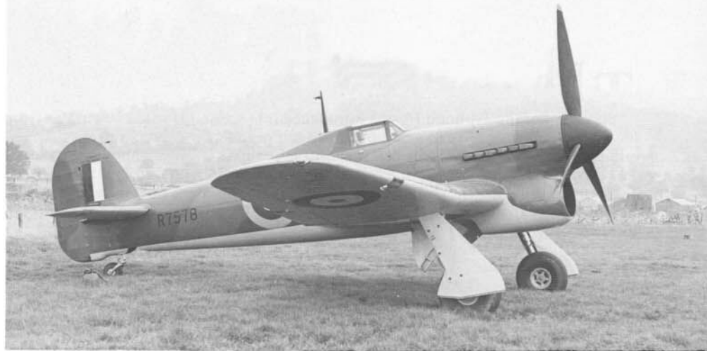
This early production Typhoon IA (R7578) lacks the small windows behind the cockpit found on the prototype Typhoon. The aircraft is armed with a total of twelve Browning .303 machine guns, six in each wing.
