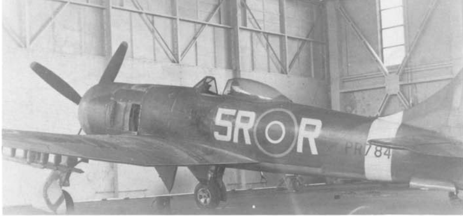
One of No. 33 Squadron's Tempest IIs (PR784) occupies a hangar at Fassberg, Germany. These aircraft carried their serial numbers in Black on the wing undersurface and part of the number can be seen on the wheel well door.
