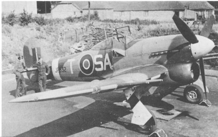
No 486 Squadron, Royal New Zealand Air Force was based at Tangmere during 1943 and was among the first Commonwealth units to receive the Typhoon IB. This Typhoon IB (JP532) was often flown as a fighter-bomber using removable underwing bomb racks.
