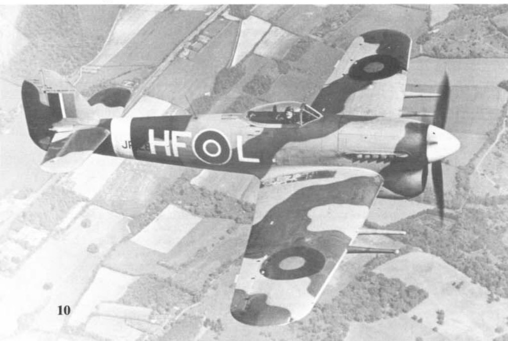
This Typhoon IB (JP128) of No 183 Squadron was flown by Merrick Hyman. The aircraft has the bubble canopy, fish plate reinforcements and whip antenna identifying it as a late production Typhoon IB.
