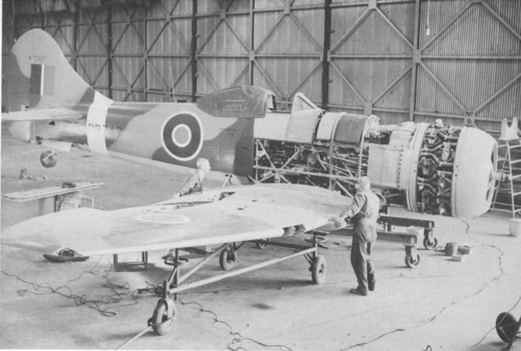
Workmen at Hawker's Langley facility mate the starboard wing to a Tempest II (PR747) fuselage. The wing mounted Hispano cannons have not been installed and all the forward fuselage access panels have been removed.
