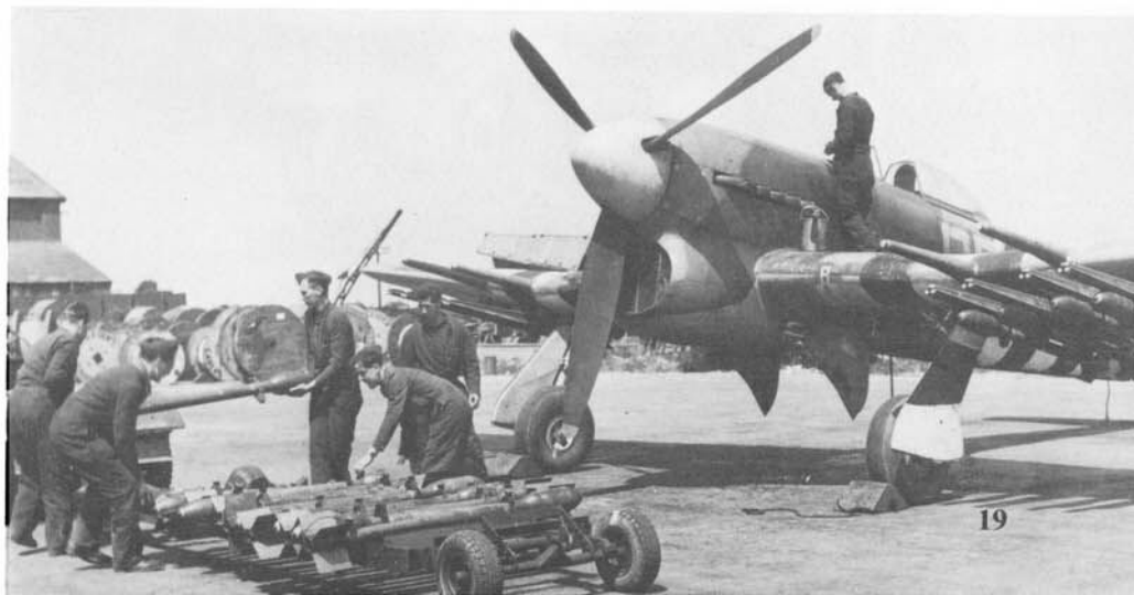
Ground crewmen load 60 pound rockets on the wing racks of a Typhoon IB of the 2nd Tactical Air Force. Each Typhoon could carry eight rockets, making them a potent ground attack weapon against German armor.
