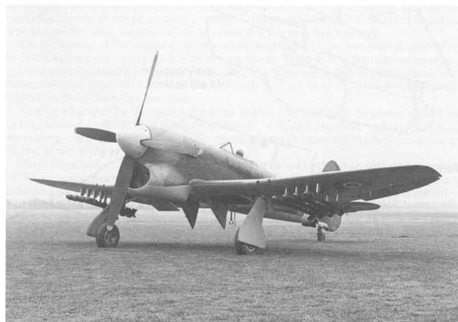
Although the Tempest, unlike the Typhoon, did not use rockets operationally during the war, the Tempest Mk V was tested and cleared to carry eight rockets on Mk VIII zero length launchers.
