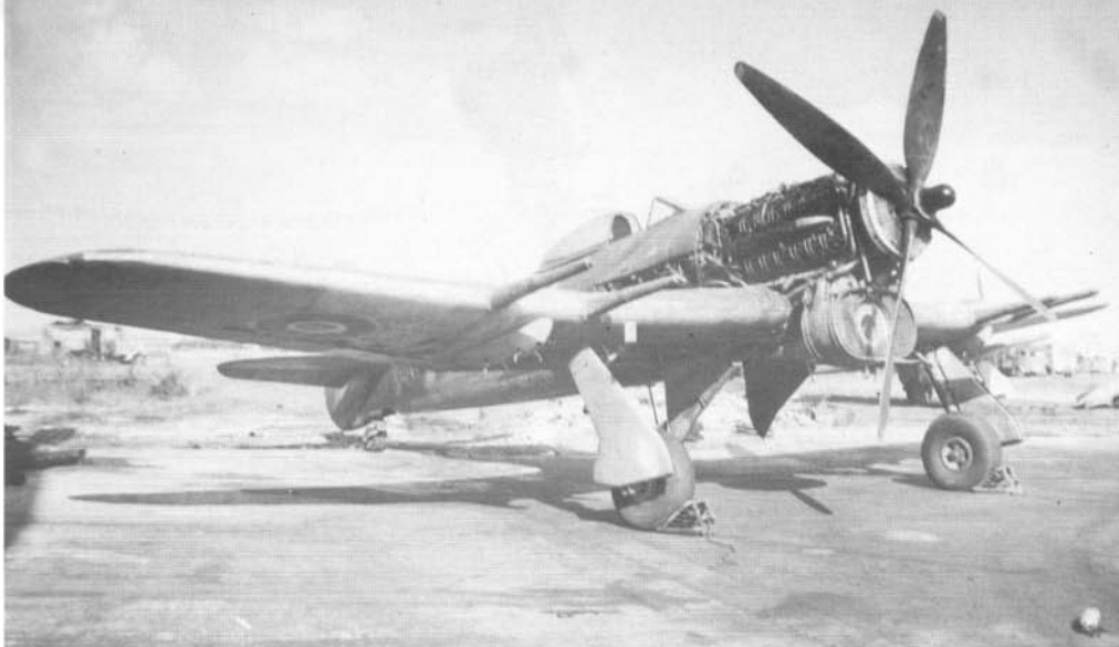
This late production Typhoon IB of No 440 Squadron has the cowling panels removed so that maintenance personnel can work on its engine at Eindhoven, Holland, during the Spring of 1945. The Sabre engine required a lot of preventive maintenance.
