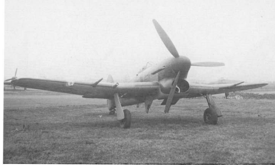
The starboard inboard cannon fairing of this Typhoon PR IB (EK427) reveals the lens of a five inch forward facing oblique camera. This camera was used to record the damage done to targets during strikes by rocket and bomb armed Typhoons.
