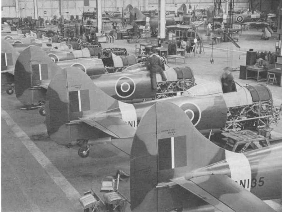
Tempests during final assembly at Langley reveal that the aircraft were painted with camouflage, national insignia, and serial numbers before the engines were mated to the fuselage. The aircraft in the foreground (SN135) served with No 274 Squadron, then with two others before being retired during 1950.
