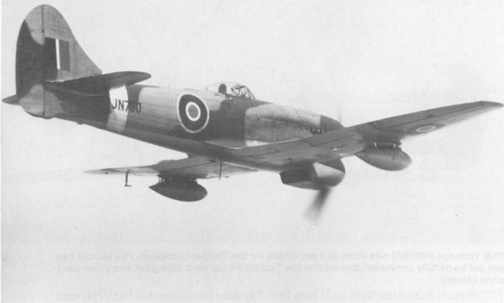
The second production Tempest V (JN730) was used to test fly the Hawker designed forty-five gallon teardrop shaped underwing fuel tanks. The tanks were approved for use and became a standard item of equipment for Tempest squadrons.
