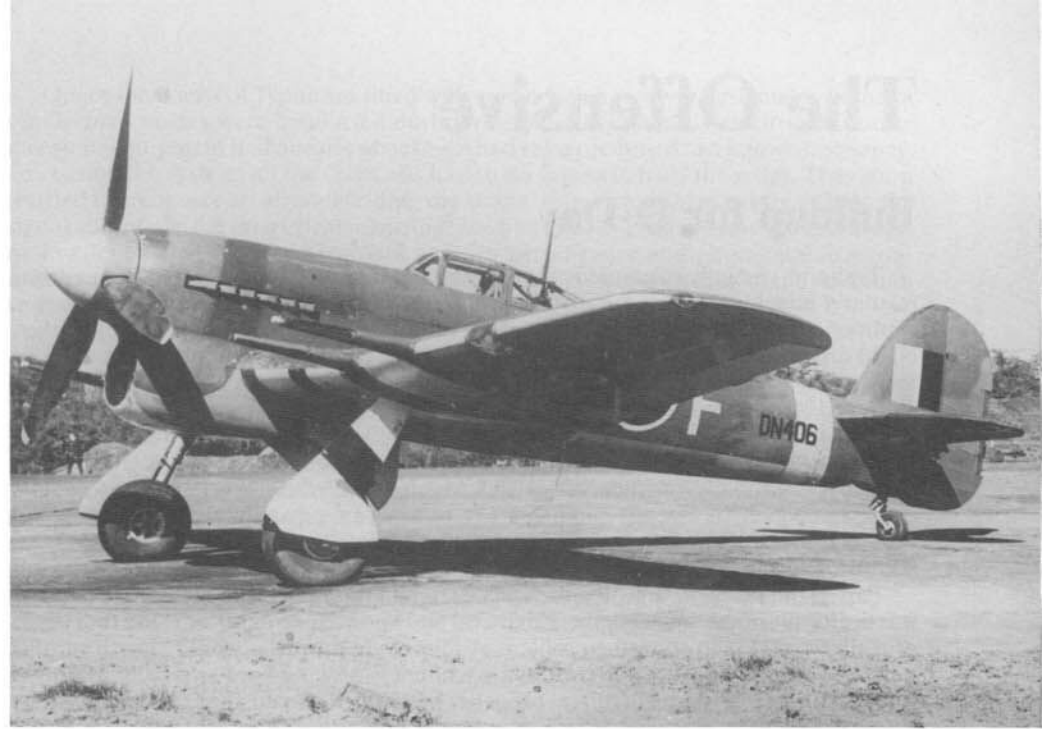
A Typhoon IB of No 609 Squadron (DN406/PR-F) parked in its dispersal spot at Tangmere during May of 1943. The aircraft has the later faired cannon barrels and carried a score of eighteen locomotive silhouettes on the starboard side under the cockpit.
