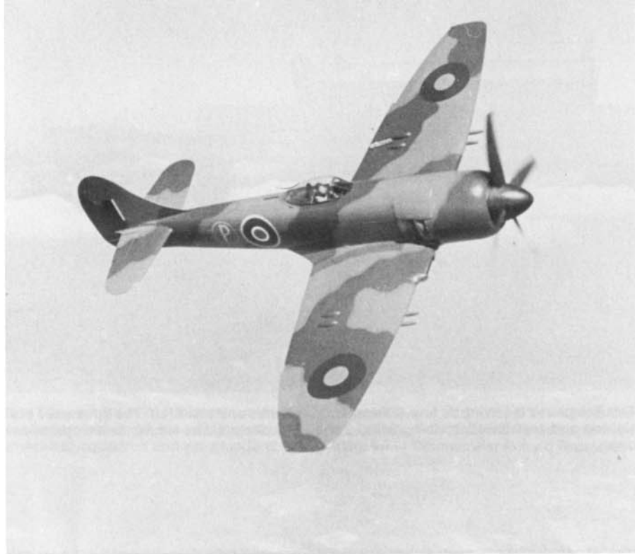
The prototype Tempest II (LA602) was armed with the early long barreled Hispano Mk II cannons that extended beyond the wing leading edge. Originally, the aircraft had been fitted with a Typhoon style tail.
