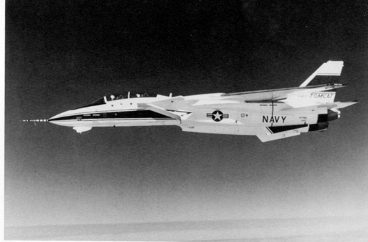
The F-14B test aircraft is fitted with General Electric F110-GE-400 engines and a dual infrared sensor/ECM chin pod under the nose. Although the aircraft was used as a testbed, it retained the M61 cannon. All leading edge surfaces were unpainted natural metal. (Grumman)
