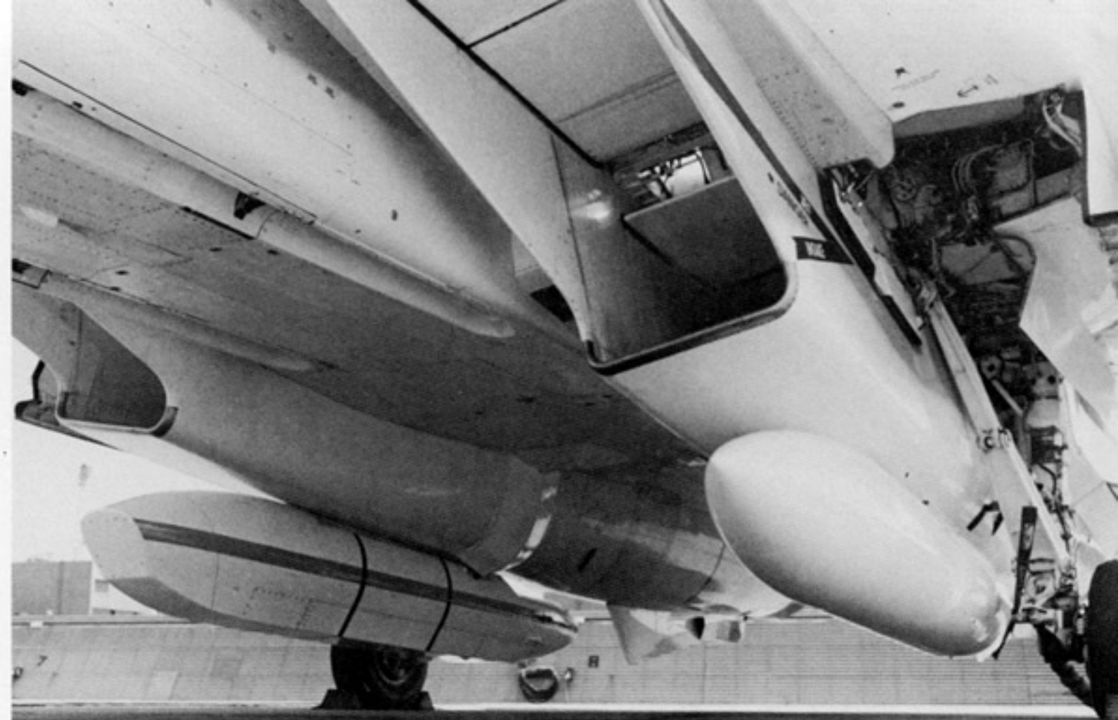
By 1980, the shape of the TARPS pod had evolved and the fins were removed. The fins were removed to make the pod closer in aerodynamic properties to the normal external fuel tanks carried by the Tomcat. The Black stripes on the TARPS pod are alignment reference markings. (Grumman)
