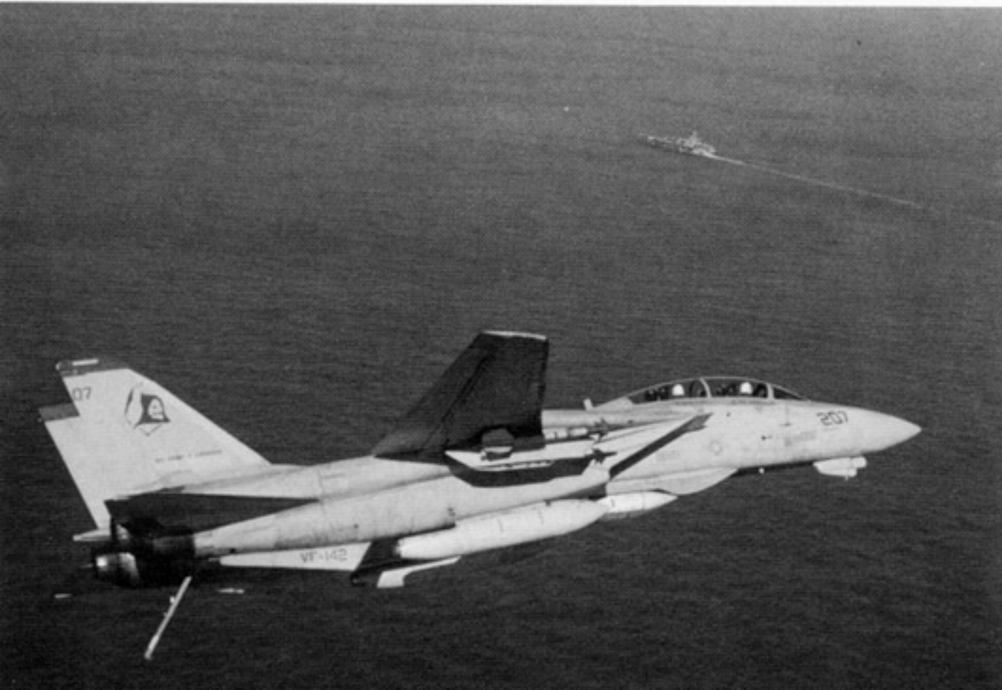
Hook down, an F-14A of VF-142 Ghostriders turns onto final approach for landing aboard USS DWIGHT D. EISENHOWER (CVN-69) in the Mediterranean Sea. The aircraft is armed with two AIM-9 Sidewinders and two AIM-54 Phoenix air-to-air missiles. (USN via LT J. Mizerak)
