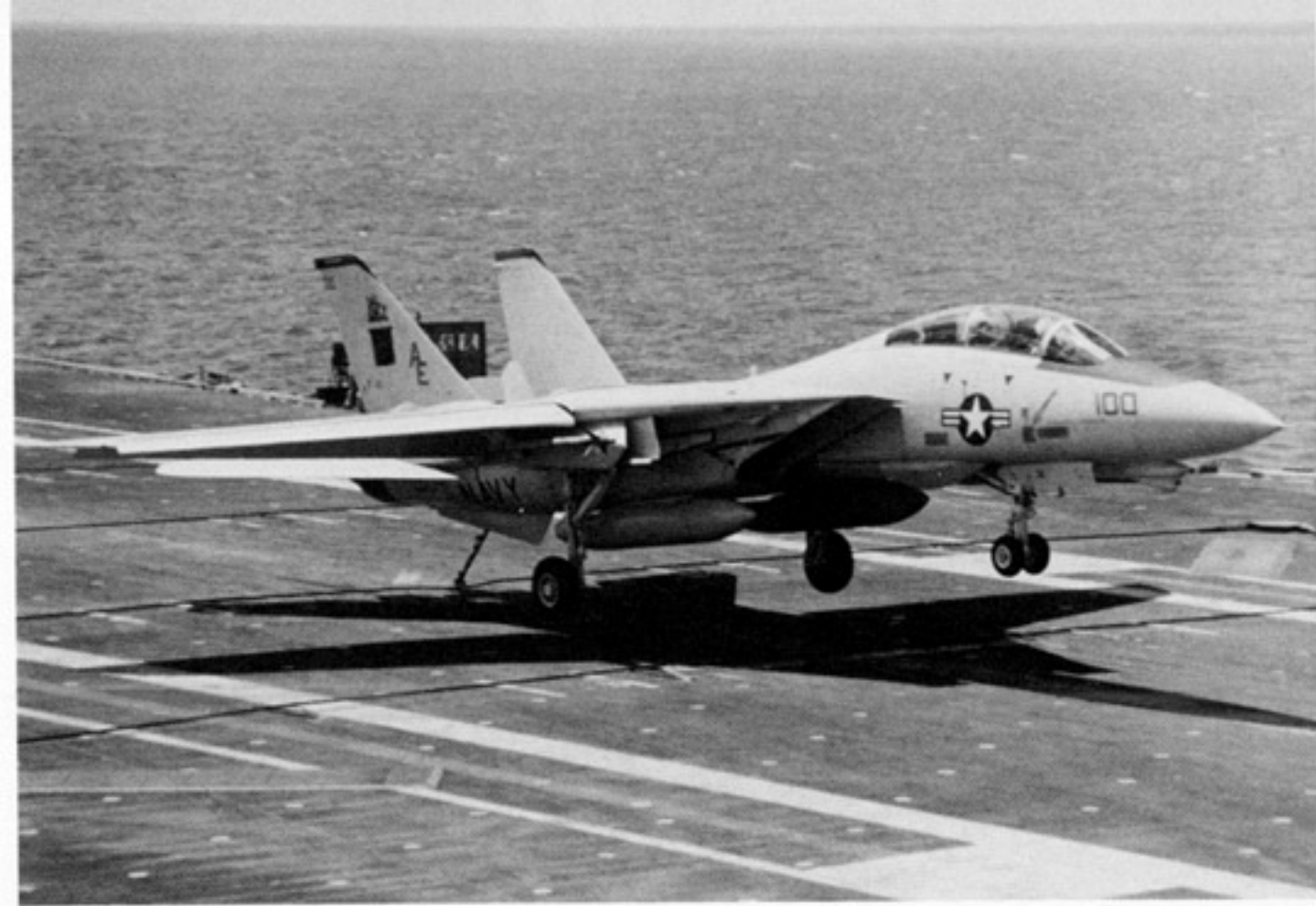
An F-14A of VF-11 Red Rippers engages the number 3 wire for a perfect arrested landing aboard USS FORRESTAL (CV-59) in the Mediterranean Sea with the U.S. Sixth Fleet. The tips of the vertical stabilizers are Red and the anti-glare panel is Dark Blue-Gray. (USN)
