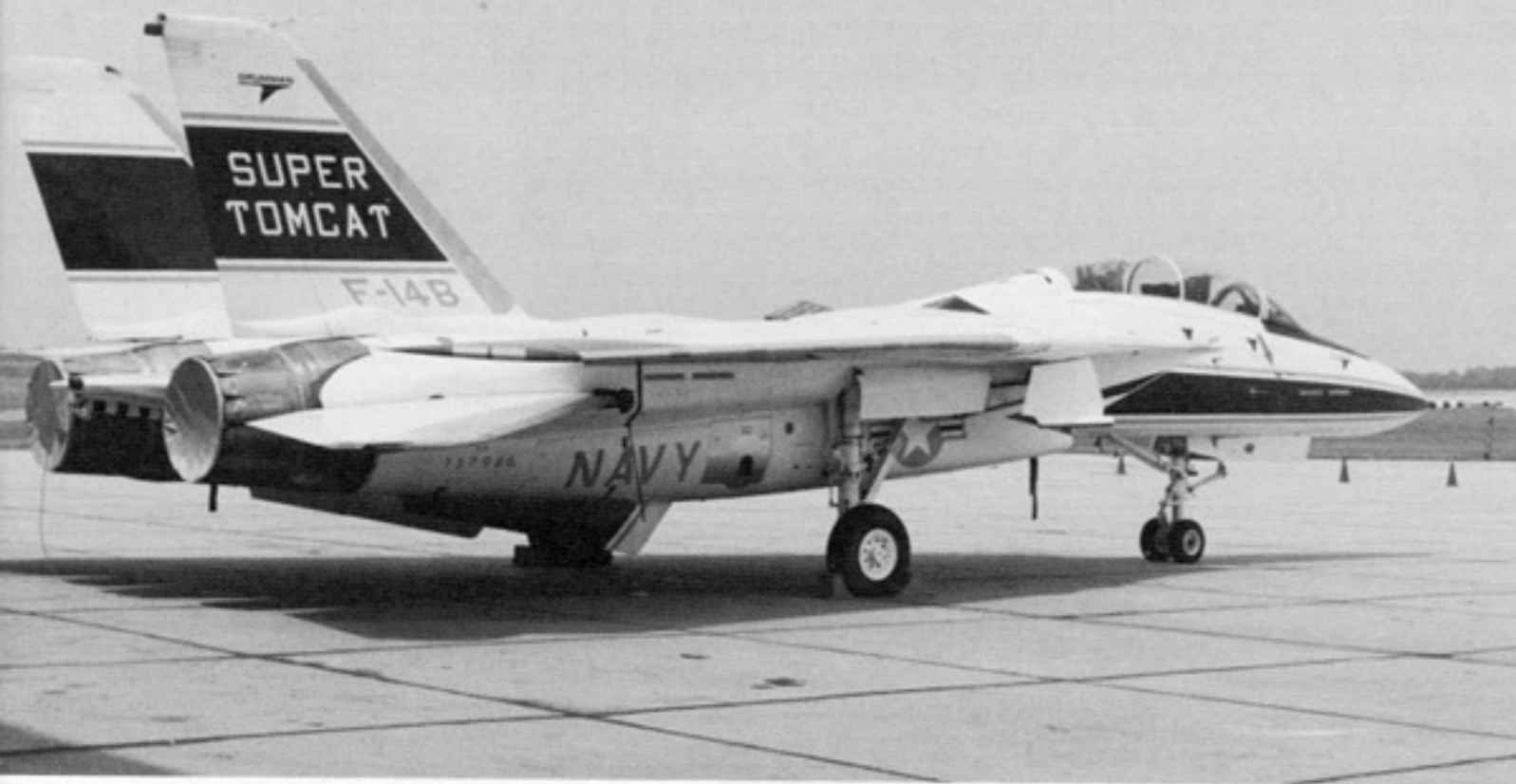
The F-14B Super Tomcat on the ramp at the Grumman facility during 1976. The natural metal APU (Auxiliary Power Unit) exhaust area is visible just forward of NAVY on the lower fuselage side. Once flight testing with the F-401 engine was completed, the F-14B was put into long term storage. (Grumman)
