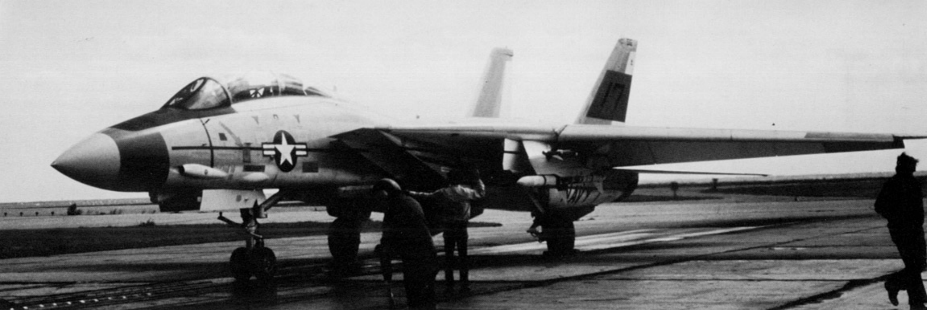
F-14A Number 12 (BuNo 158616) was used for catapult tests at the Naval Air Test Center, Pax River, Maryland, during 1972. The tests included launches at various weights and with various missiles carried on the wing pylons. The aircraft carries a Red identification band on the nose and Black photographic reference stripes on the fuselage. (USN)
