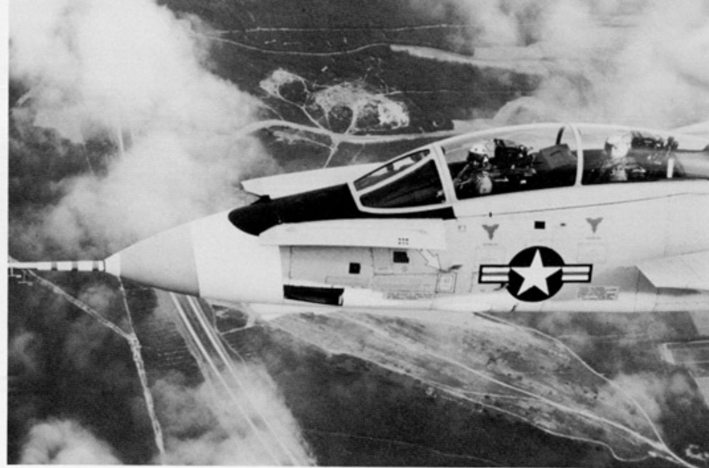
The ARI modifications included a set of moveable canards mounted on the nose section and software changes to the aircraft's basic analog flight control system. The canards, when not in use, were hydraulically folded flush along the side of the nose. (Grumman)
