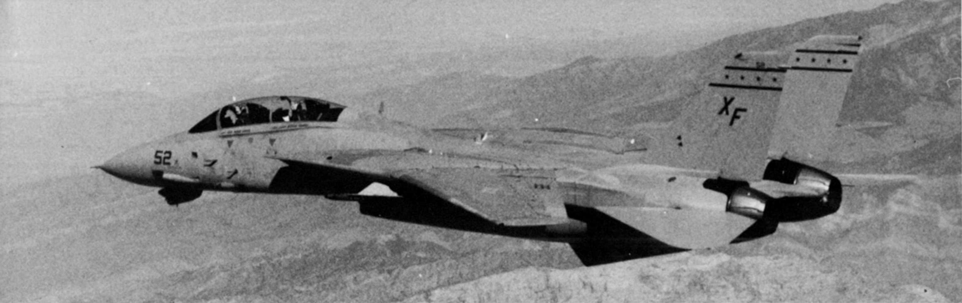
XF-52 is an F-14A (Plus) of the Pacific Missile Test Center, Point Mugu, California. Weapons testing with the F-14A (Plus) began at PMTC during January of 1988. Tests included firing air-to-air missiles, carrying Mk-82 500 pound bombs, and both air-to-air and air-to-ground firing of the internal cannon. (General Electric)
