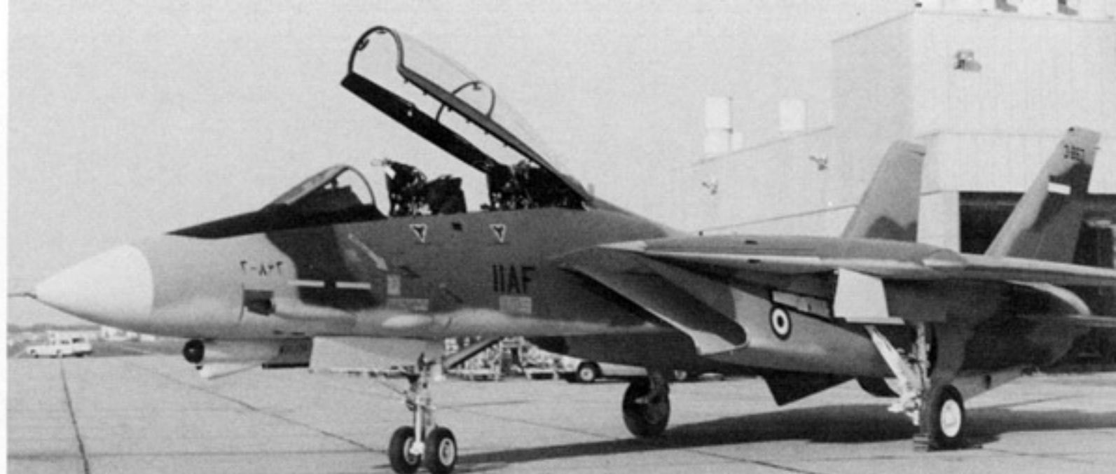
An F-14 of the Imperial Iranian Air Force parked on the ramp at the Grumman plant at Calverton, New York, awaiting a flight crew to make the delivery flight to Iran. Aircraft was finished in a Tan, Brown and Green upper surface camouflage over a Light Gray undersurface. (Grumman)
