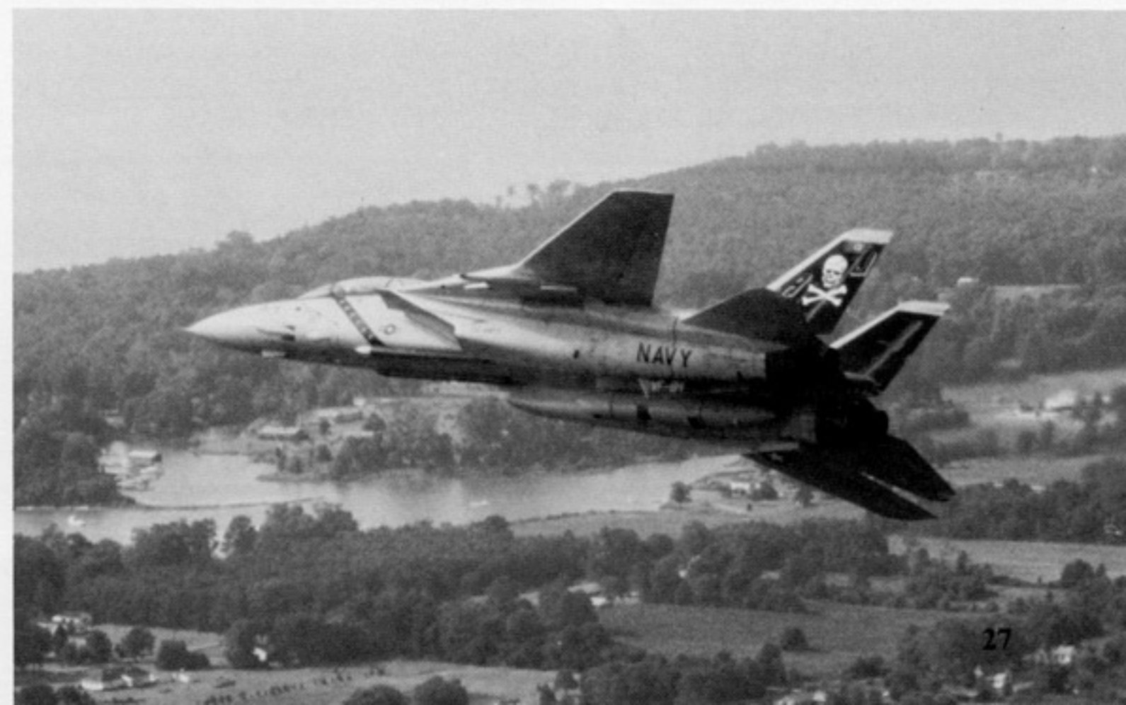
TARPS equipped aircraft made their first cruise aboard USS NIMITZ (CVN-68) with VF-84 Jolly Rogers during 1982. When carrying a TARPS pod, the Tomcat can still carry other weapons for self defense. The pod utilizes cooling from the mother aircraft, similar to the system utilized by the AIM-54 Phoenix. (Grumman)
