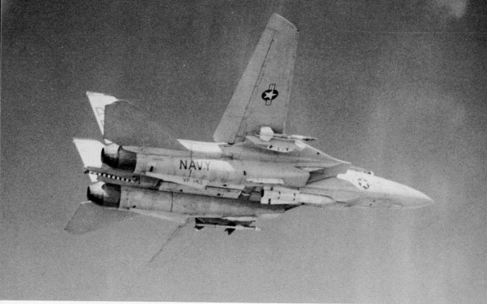
This F-14A of VF-143 Pukin' Dogs is armed with an AIM-54 Phoenix missile on the forward pallet, an AIM-9 Sidewinder on the starboard wing pylon and an AIM-7 Sparrow on the port pylon. VF-143 was stationed aboard USS DWIGHT D. EISENHOWER (CVN-69) as part of Carrier Air Wing Seven (CVW-7). (USN)
