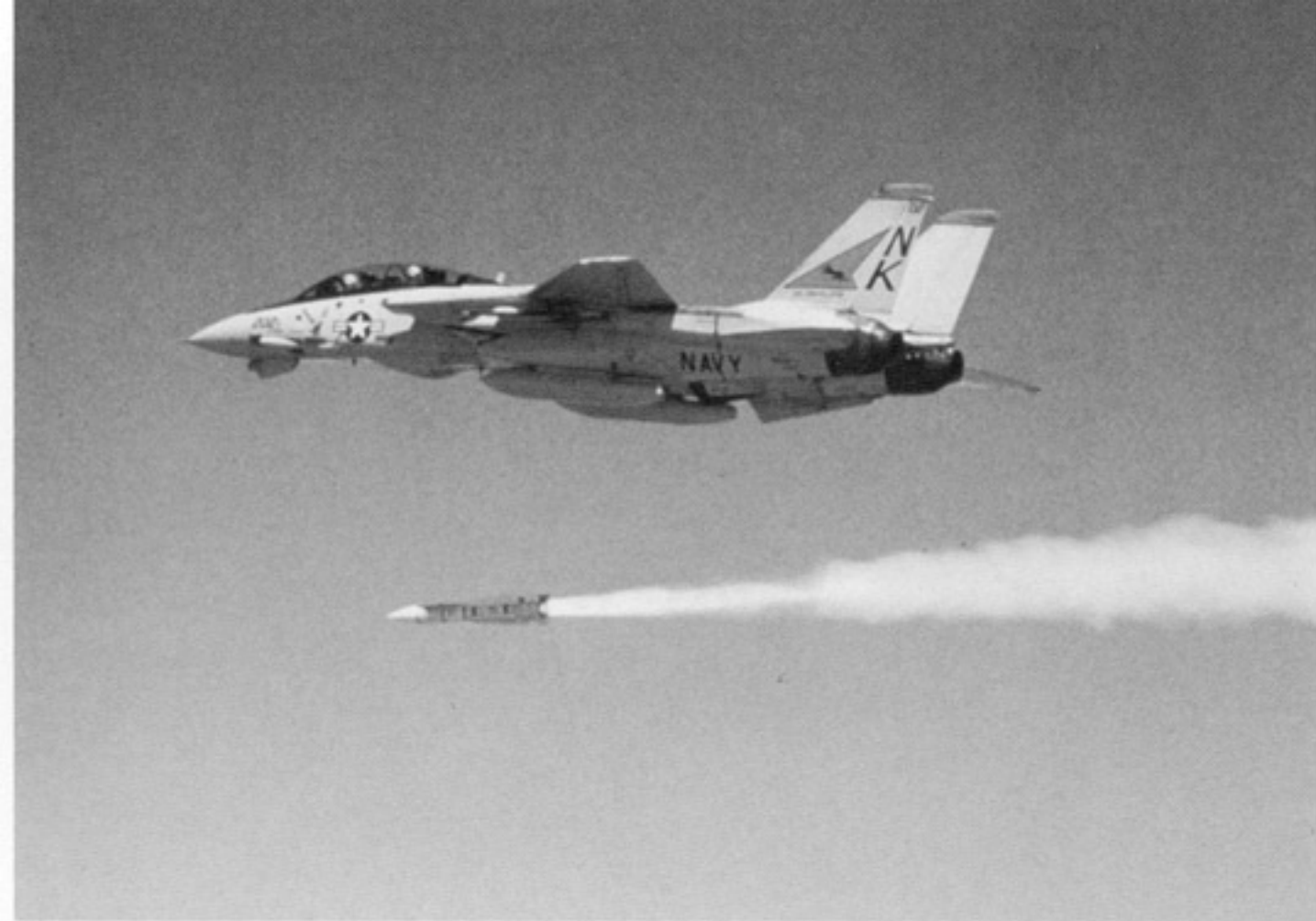
An F-14A of VF-21 Freelancers launches an AIM-54 Phoenix air-to-air missile during a live fire exercise. The Tomcat is equipped with a TCS chin pod and two 270 gallon fuel tanks. VF-21 was attached to Carrier Air Wing Fourteen (CVW-14) aboard USS CONSTELLATION (CV-64). (Hughes Aircraft)
