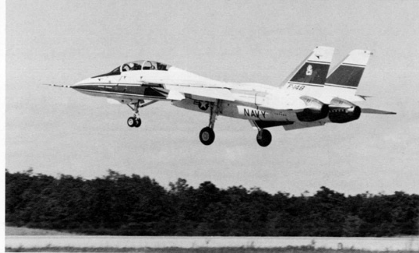
The F-14B prototype (BuNo 157986) differed externally from the F-14A in the shape of the engine exhaust nozzles of the Pratt and Whitney F-401 turbofans. The F-14B prototype would later serve in the development programs for both the F-14A (Plus) and F-14D. (Grumman)
