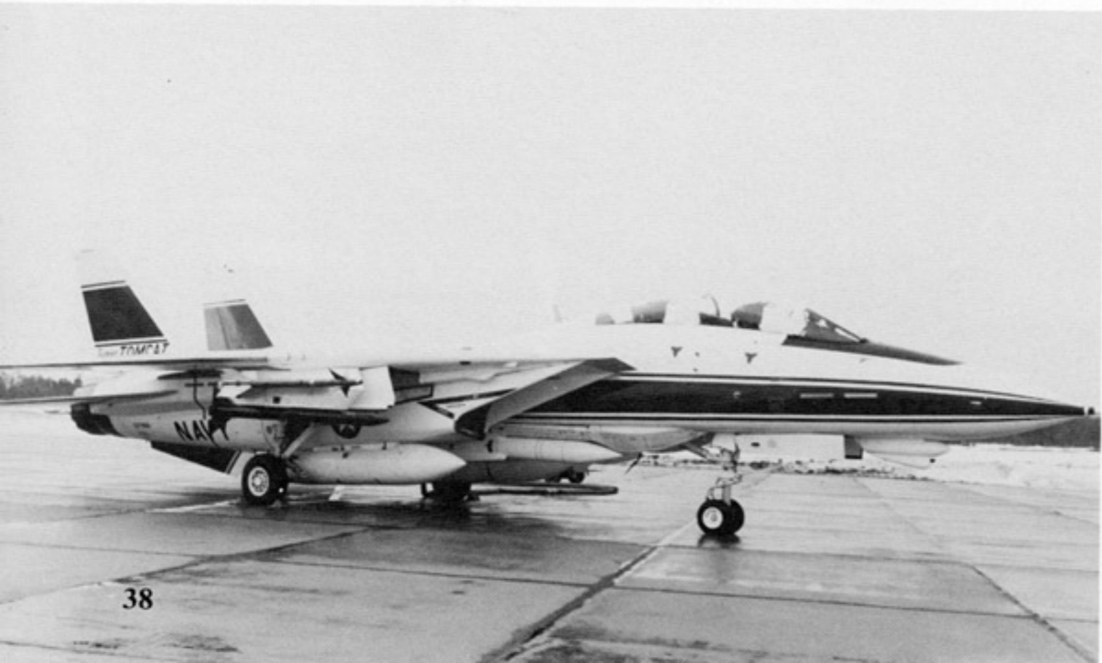
The F-14B prototype carries Phoenix missiles on the fuselage pallets, Sparrows on the wing pylons, and Sidewinders on the wing shoulder pylons during early 1987. The aircraft was also equipped with two 270 gallon fuel tanks. Even though it is carrying Phoenix missiles, the aircraft could not fire them, since it had no AWG-9 radar installed. (Grumman)
