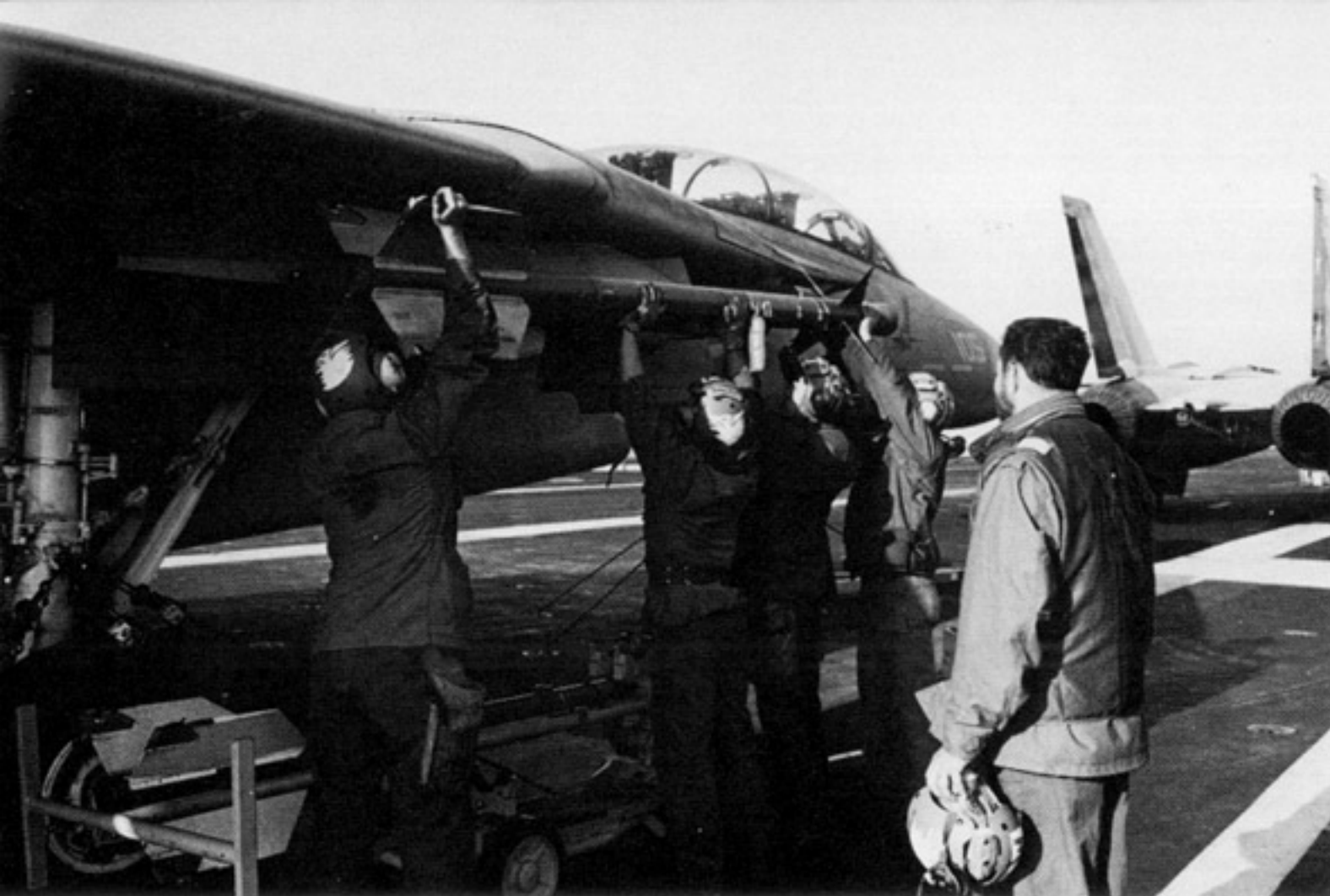
Red shirted Ordnancemen of VF-1 Wolfpack load an AIM-9D Sidewinder on the starboard wing rail of an F-14A aboard USS JOHN F. KENNEDY (CV-67) while another AIM-9D sits on the weapons dolly. The deck crew all have the Wolfpack insignia on their head/ear protection equipment known to the crews as the brain box. (USN by M. Langway)
