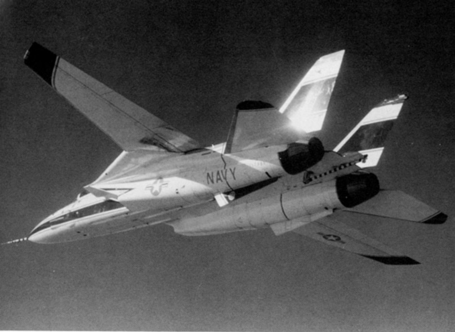
During 1981 the F-14B was removed from storage and fitted with General Electric F-101-GE-400 Derivative Fighter Engines (DFE). During the short flight test program (between July and September 1981) Grumman made twenty-two flights and the Navy conducted three test flights. The aircraft carried a General Electric logo on the ventral fin. (Grumman)
