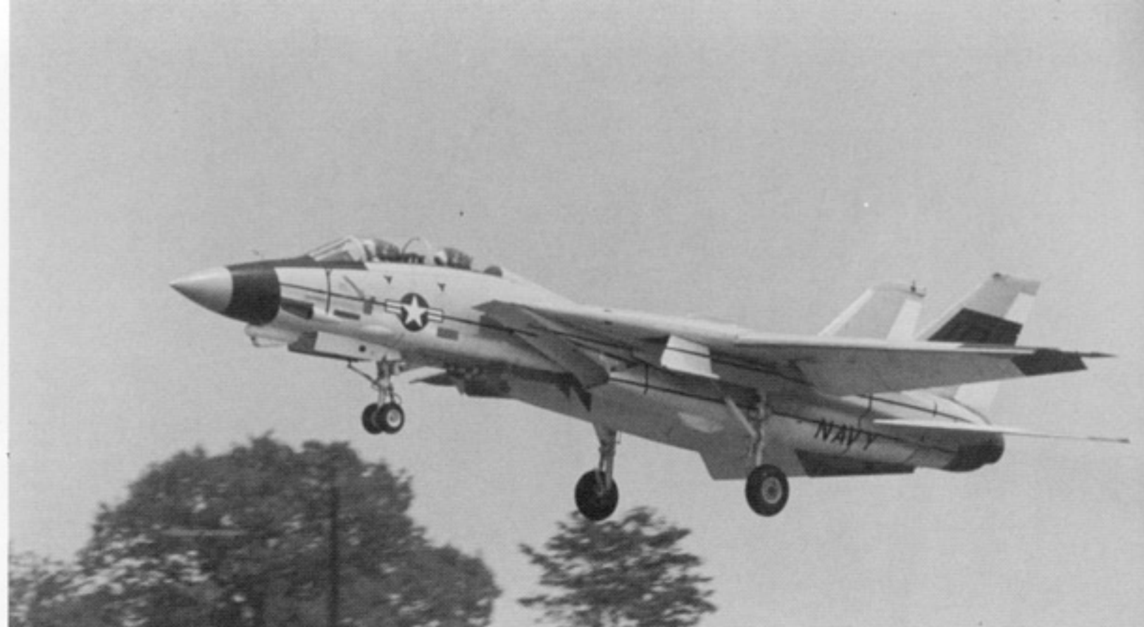
This pre-production F-14A (aircraft number 10, BuNo 167989) carries Black photographic reference stripes on the fuselage. Aircraft number 10 was used for flight tests to determine the flight envelope of the F-14A and was later lost while conducting spin tests. (Grumman)
