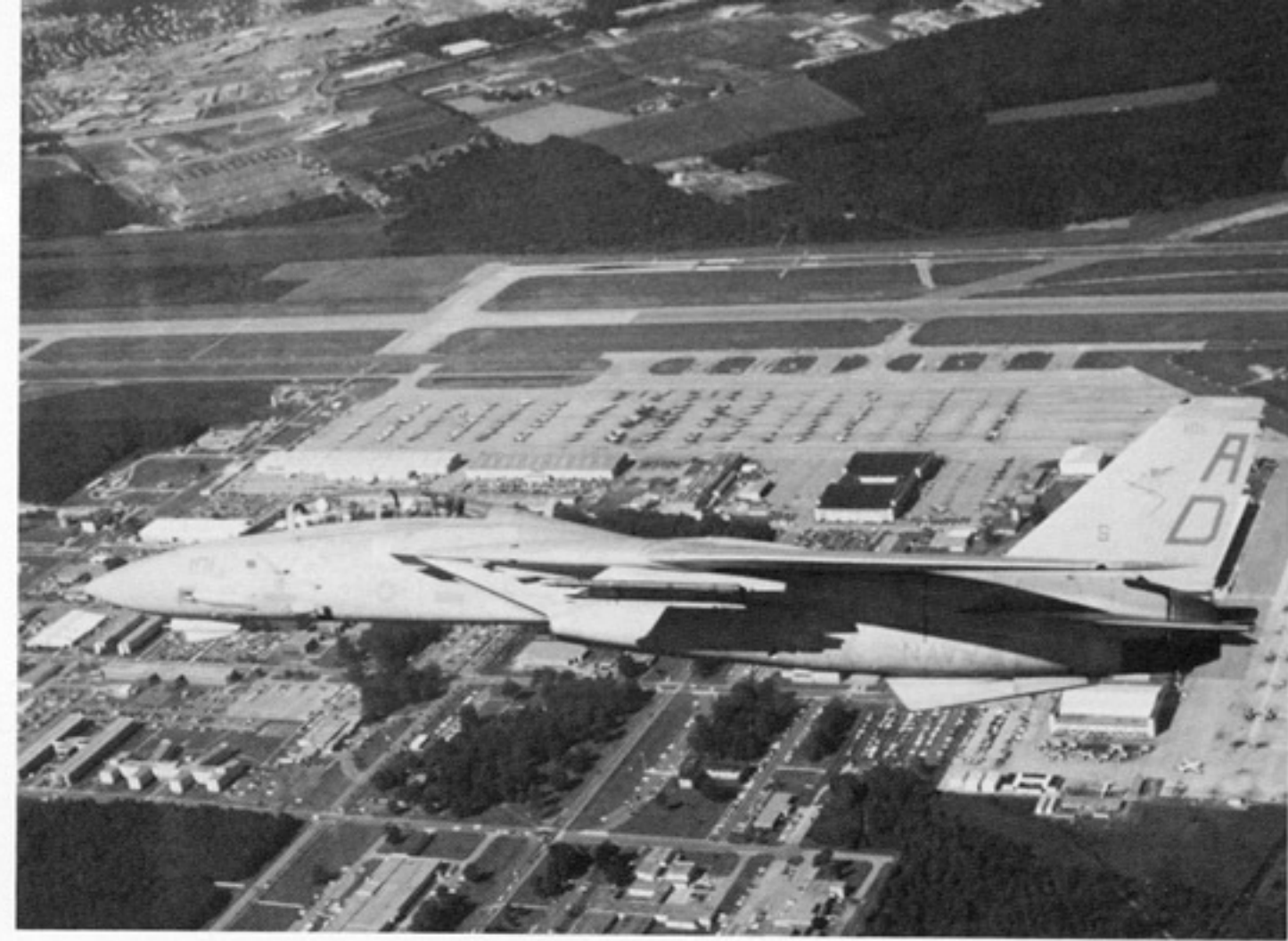
An F-14A (Plus) flies over NAS Oceana, Virginia, the home base of VF-101 Grim Reapers. Pilots report that the F-14A (Plus) has a much better acceleration and can perform vertical maneuvers that were impossible in the TF-30 powered F-14A. The two fairings under the wing glove are ECM antennas. (Grumman)
