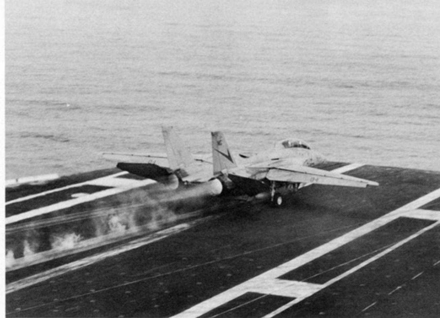
An F-14A of VF-24 Fighting Renegades launches from the waist catapult of USS KITTY HAWK (CV-63) during February of 1987. While the F-14A requires the use of afterburner during launch, the newer, re-engined F-14A (Plus) and F-14D do not. Currently, the KITTY HAWK is scheduled to replace the USS LEXINGTON (AVT-16) as the Navy's training carrier. (USN by J.D. Bunting)
