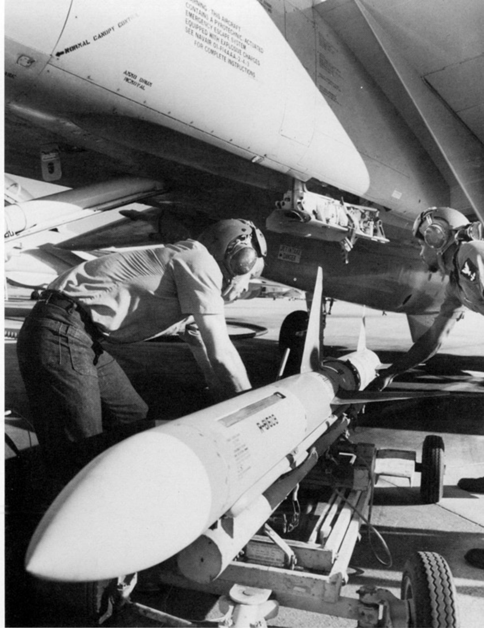
Ordnancemen load an AIM-7M Sparrow onto the port fuselage weapons bay on this F-14A. This version of the Sparrow was credited with shooting down one of the two MiG-23 Floggers credited to VF-32 Swordsmen on 5 January 1989. The AIM-7M has an improved monopulse seeker and digital processor giving it a greater look-down capability. (General Dynamics)
