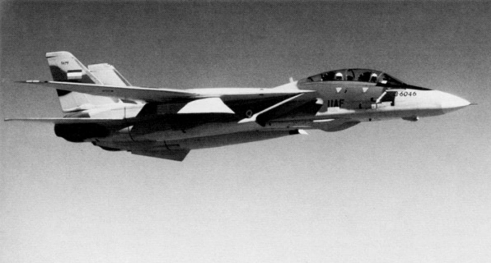
This Iranian F-14A (serial number 3-6046) was one of the last purchased by Iran. The aircraft carries pallets for Phoenix missiles on fuselage as well as wing missile pylons. During the Iran-Iraq war the aircraft were mainly flown armed with AIM-7 Sparrow and AIM-9 Sidewinder missiles. (Grumman)
