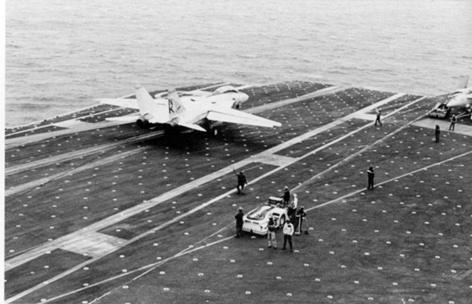
An F-14A of VF-21 Freelancers comes to a halt on the angle deck of USS CONSTELLATION (CV-64). The White dots on the deck are tie-down locations and the vehicle in the foreground is an MD-3A tow vehicle modified for fire fighting duties. (USN via M. Tamberg)
