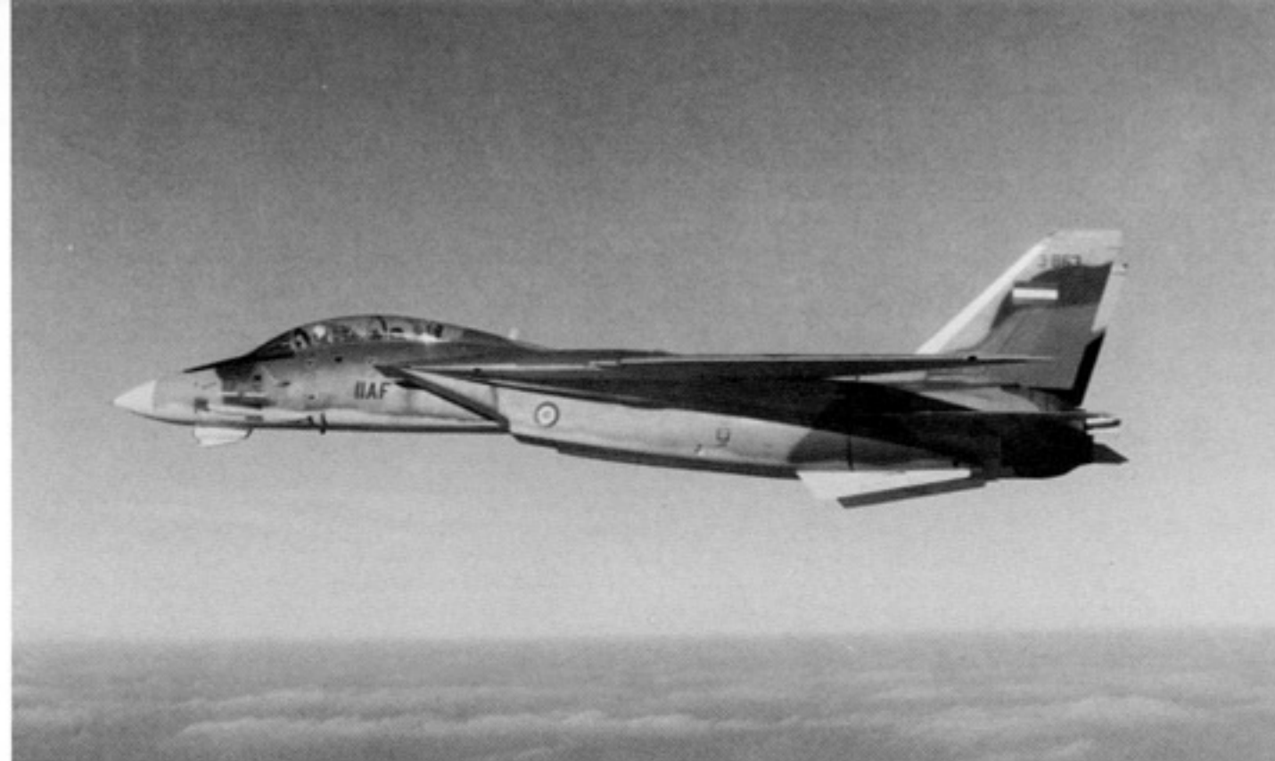
Iranian Air Force F-14As retained all of the aircraft's carrier equipment, such as catapult launch bar and arresting hook, although the hook was now used for airfield arresting gear. Iran purchased the F-14A to counter overflights by Soviet MiG-25 Foxbats. The leading edges of the wings, horizontal stabilizers and vertical stabilizers were unpainted. (Grumman)
